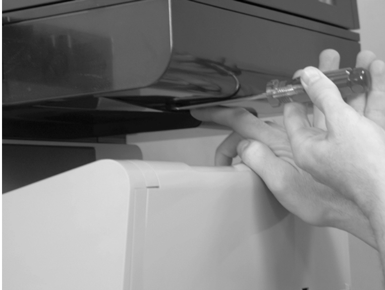
Figure 1-84 Remove the scanner (1 of 7)
