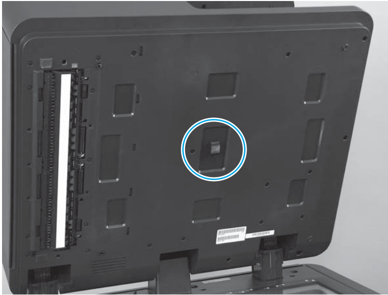
Figure 1-15 Remove the document feeder white backing (3 of 3)
