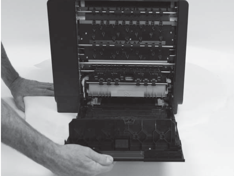
Figure 1-47 Remove left door (1 of 5)
