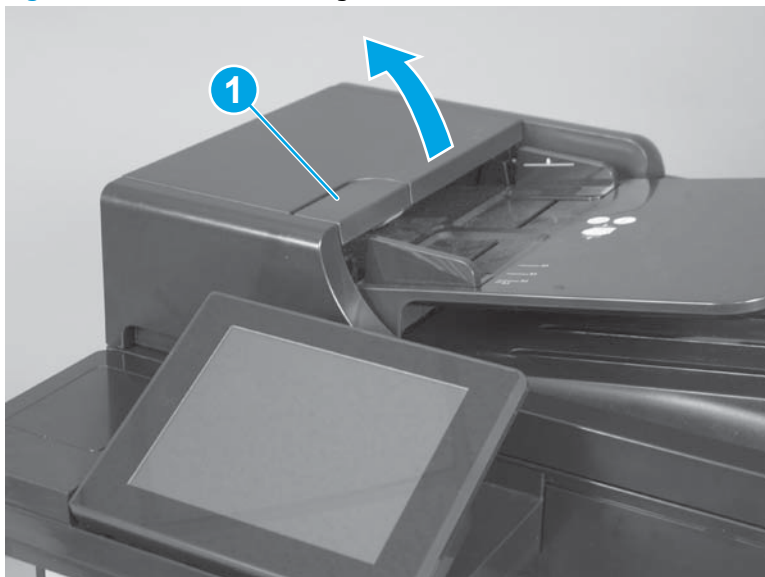
Figure 1-22 Remove the background selector (1 of 4)
