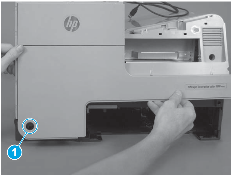
Figure 1-63 Remove the front cover (2 of 2)
