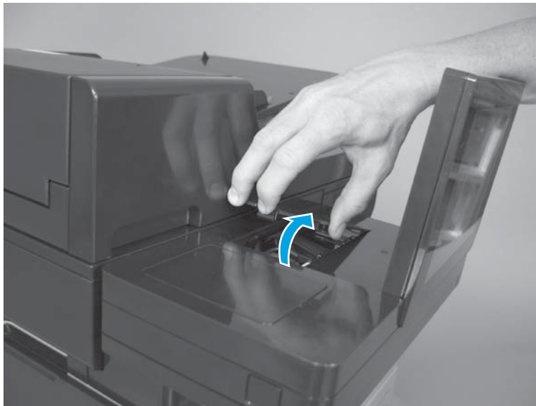
Figure 1-31 Remove the control panel — X585 models (1 of 4)
