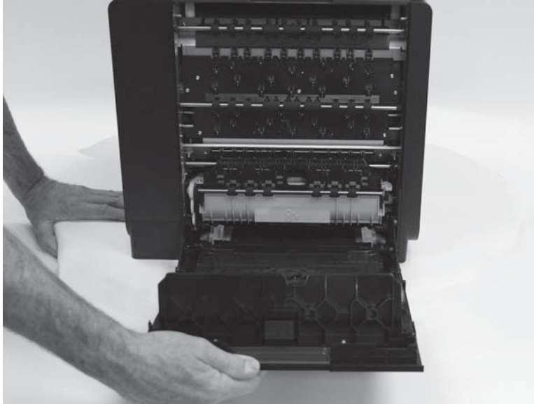
Figure 1-60 Remove the top cover cap (1 of 2)
