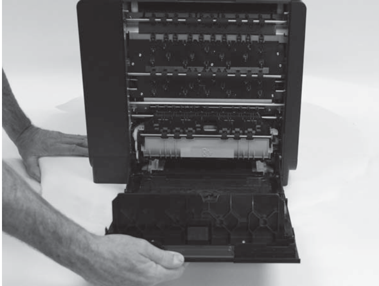
Figure 1-2 Remove the ink collection unit (1 of 2)
