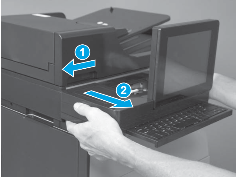
Figure 1-34 Remove the control panel — X585 models (4 of 4)
