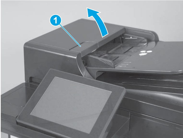
Figure 1-66 Remove the document feeder mylar strip (1 of 4)
