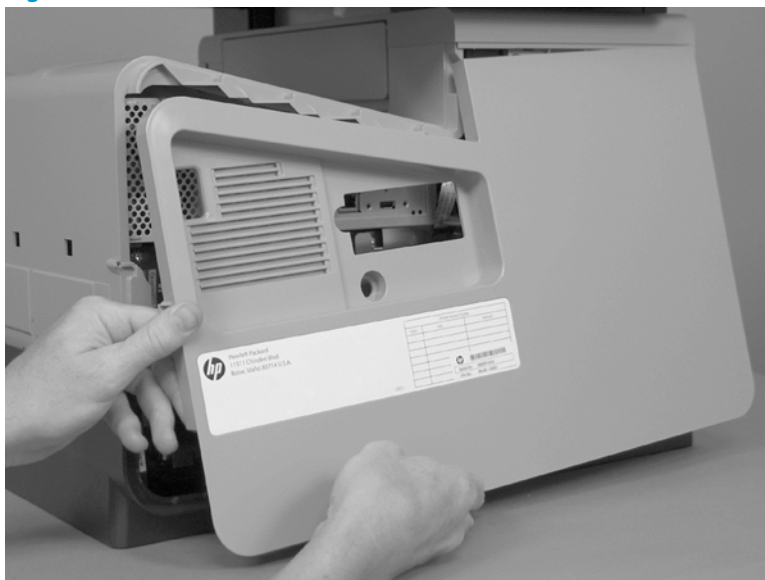
Figure 1-46 Remove the rear cover (2 of 2)
