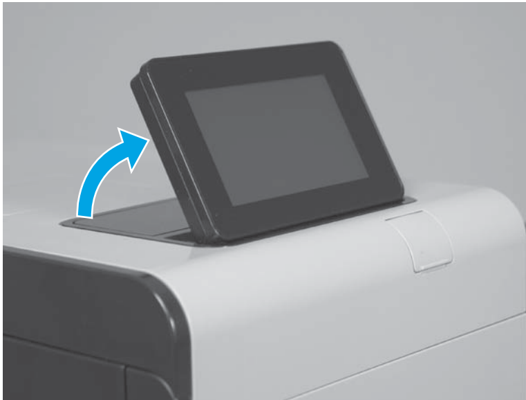
Figure 1-27 Remove the control panel — X555 models (1 of 4)
