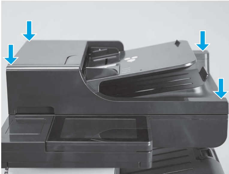
Figure 1-19 Install a replacement document feeder white backing (4 of 6)
