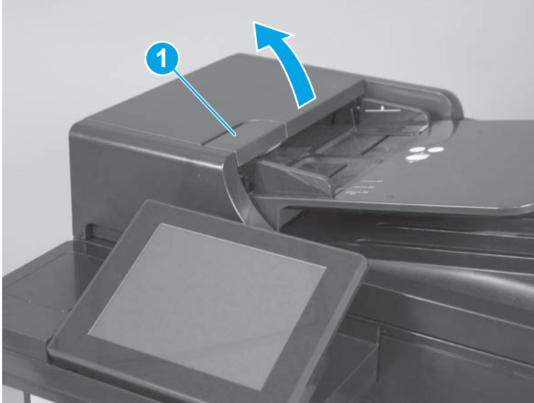
Figure 1-6 Remove the document-feeder roller (1 of 3)
