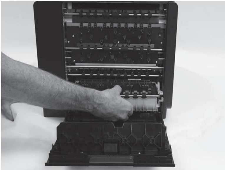
Figure 1-3 Remove the ink collection unit (2 of 2)
