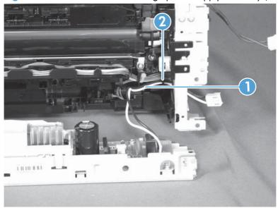
Disconnect three connectors (callout 1) and remove the low-voltage power supply assembly (callout 2).
