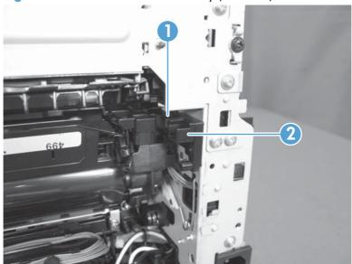
12. Release the hook end (callout 1) of the ITB fixing spring (callout 2), and then pull the wire harness (callout 3) through the hole in the chassis.
