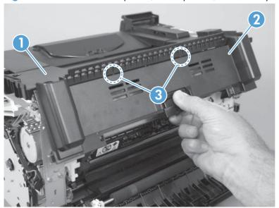
5. Open the top door (callout 1), rotate the delivery cover and rear-top cover (callout 2) away from the product, and then slide the door and covers towards the front of the product to release the assembly.
