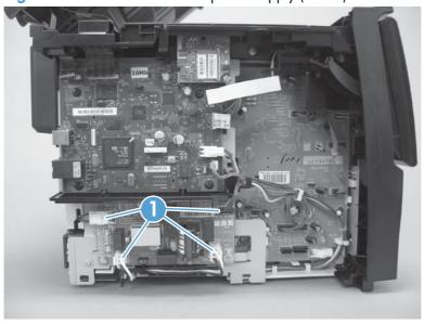
2. Remove three screws (callout 1), and then remove the fuser power supply.
