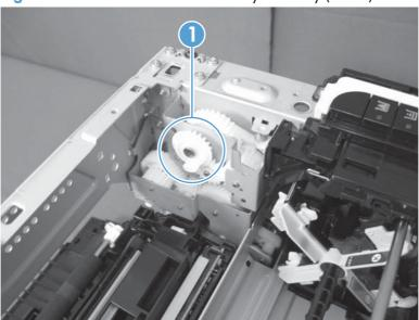
Figure 1-72 Reinstall the fuser delivery assembly (2 of 2)
