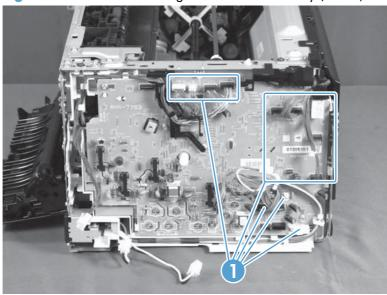
Remove six screws (callout 1), release two tabs (callout 2), and then remove the engine controller assembly.
