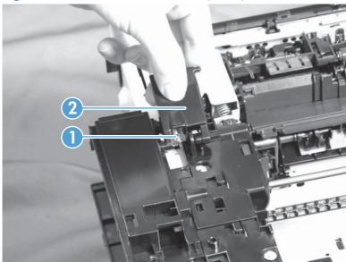
2. Remove three machine screws (callout 1), and then remove one self-tapping screw (callout 2).
