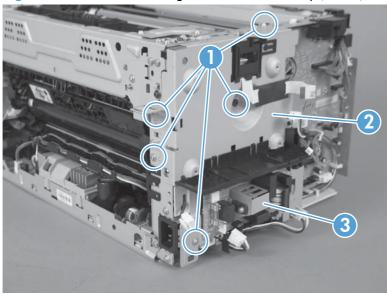
3. Disconnect one FFC (Callout 1), and then remove the sheet-metal plate and fuser power supply assembly.
