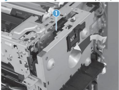
4. Release one tab (callout 1) and remove the cable cover (callout 2).
