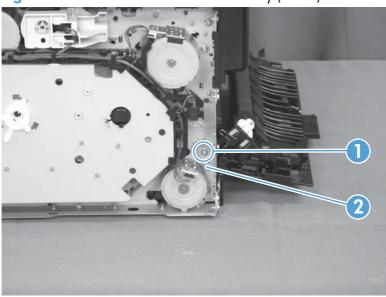
2. Pull out the shaft (callout 1) and remove the rear door assembly (callout 2).
