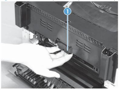
4. Push up on the rear-top cover (callout 1) to slightly raise the delivery cover (callout 2) to release two rear-top cover tabs (callout 3) along the rear edge of the product.
