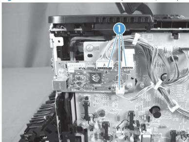
2. Remove two screws (callout 1), and then remove the formatter PCA.
