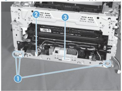
8. Release the wire harness (callout 1) from the guide (callout 2), and then pull the wire harness through the hole in the chassis.
