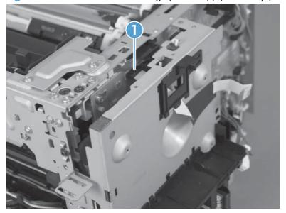
4. Release one cable from the cable guide (callout 1), and then remove two screws (callout 2).
