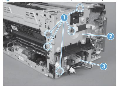
Disconnect one FFC (Callout 1), and then remove the sheet-metal plate and fuser power supply assembly.
