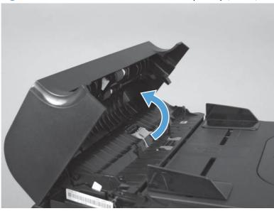
2. Hold the scanner cover down, and then pull up on the document feeder tray to release two tabs, lift the document feeder tray up, and then remove it.
