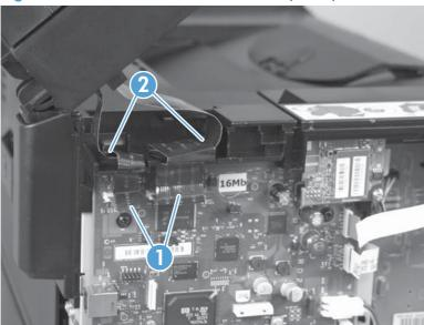
Release the tabs inside the hinges (callout 1) to allow the scanner assembly to slide down on the hinges.
