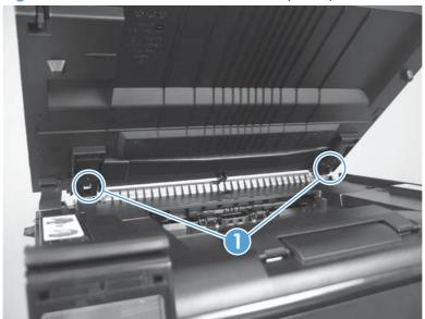
4. Lift and rotate the scanner assembly up and away from the hinges.
