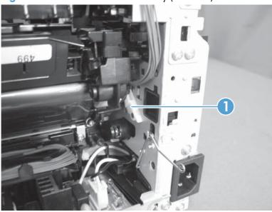
Figure 1-63 Remove the ITB assembly (16 of 17)
