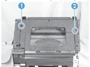
2. Open the top door, release the door retainer arm (callout 1), and then close the top door.
