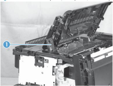
3. Open the rear door, and then release two tabs on the rear-top cover (callout 1).
