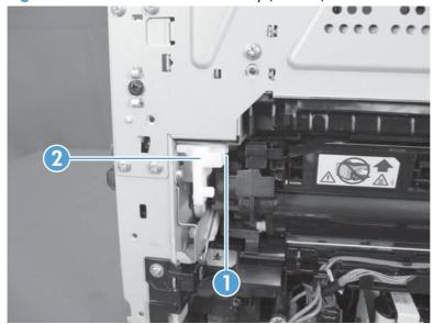
7. Release the hook end (callout 1) of the ITB fixing spring (callout 2).
