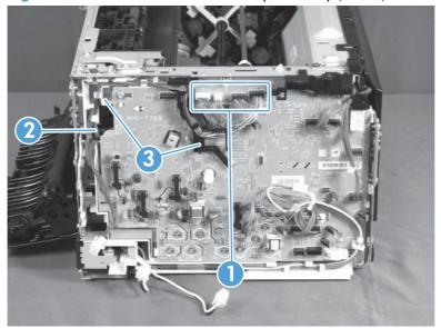
**6.** Remove six screws (callout 1), and then remove the fuser delivery assembly (callout 2).
