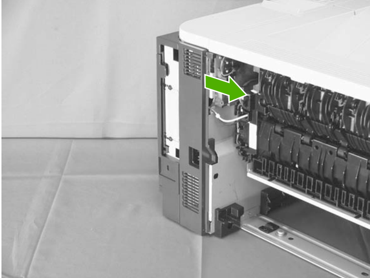
Figure 2-32 Remove the right-rear cover (1 of 2)
