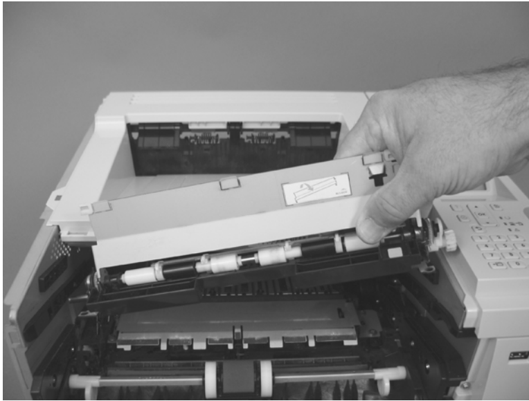
Figure 2-87 Removing the registration assembly (3 of 3)
