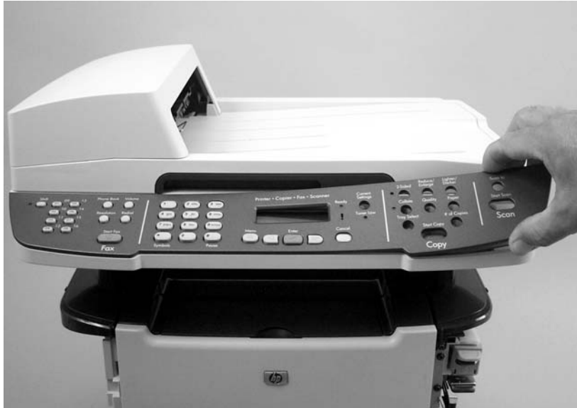
Figure 5-38 Remove the bezel and control panel (1 of 4)
