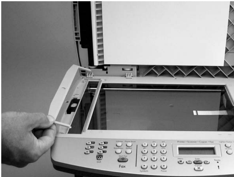
Figure 5-29 Removing the ADF scanner glass (2 of 3)
