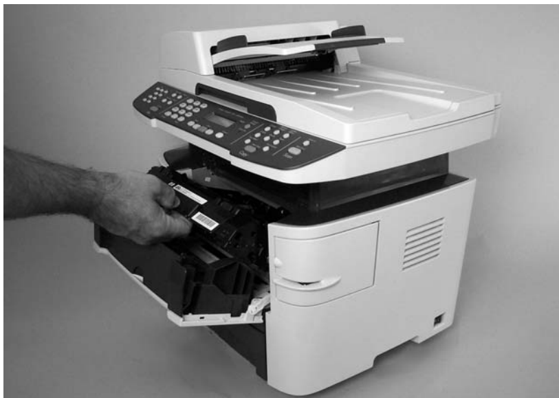
Figure 5-4 Remove the print cartridge (2 of 2)
