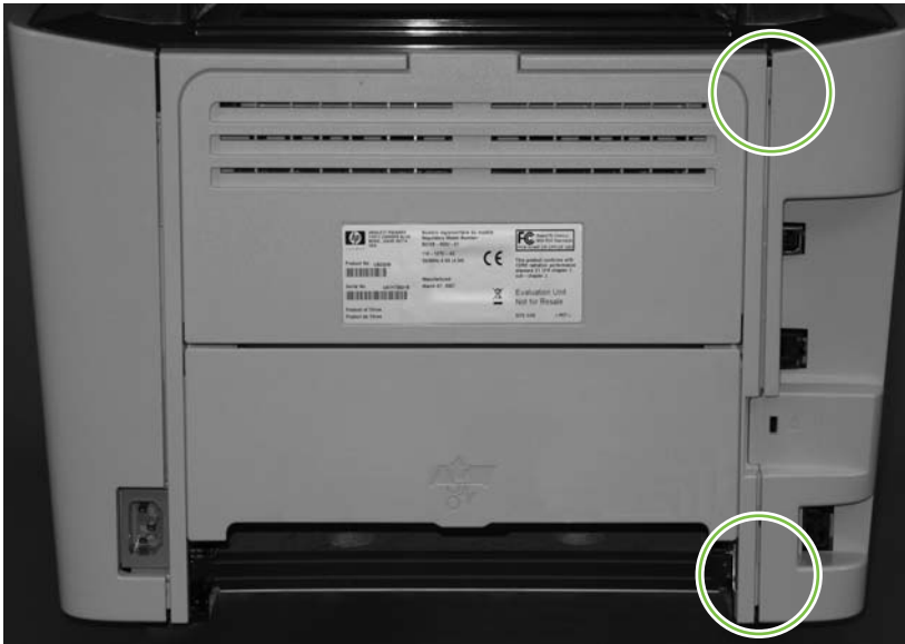
Figure 5-9 Remove the left cover (1 of 3)
