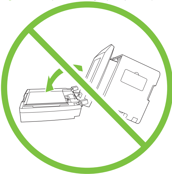
Figure 3-1 Replace the tray 2 pickup roller (1 of 7)
