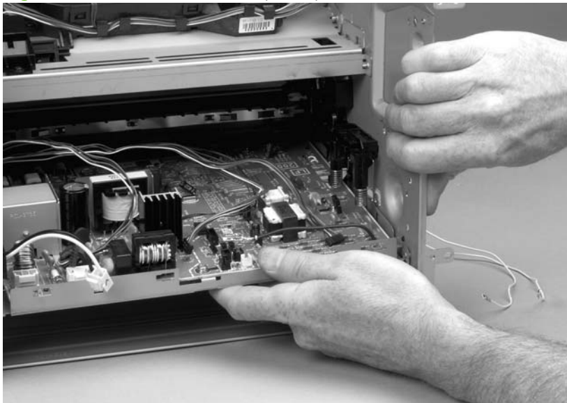
Figure 5-85 Remove the ECU (6 of 7)
