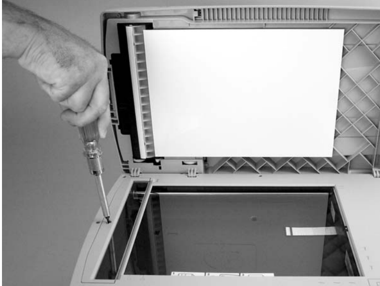
Figure 5-28 Removing the ADF scanner glass (1 of 3)
