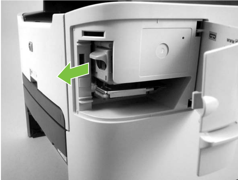
Figure 5-5 Remove the right cover (1 of 4)
