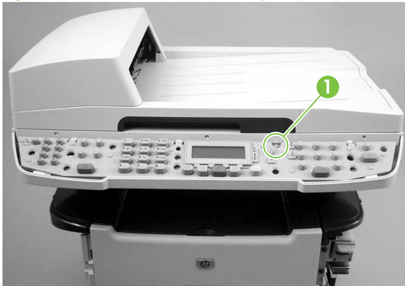
Figure 5-39 Remove the bezel and control panel (2 of 4)
