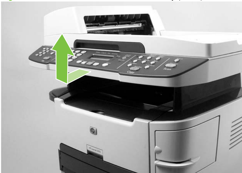
Figure 5-37 Remove the scanner/ADF assembly (4 of 4)
