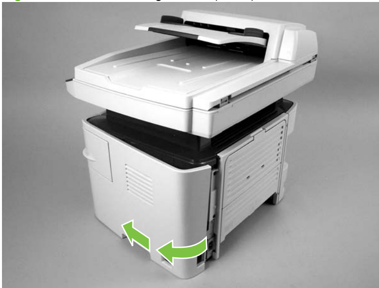
Figure 5-8 Remove the right cover (4 of 4)
