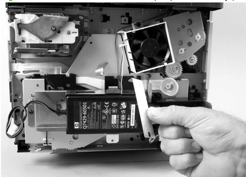
Figure 5-45 Remove the convenience-stapler power assembly (2 of 3)
