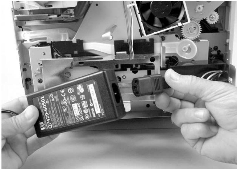
Figure 5-46 Remove the convenience-stapler power assembly (3 of 3)
