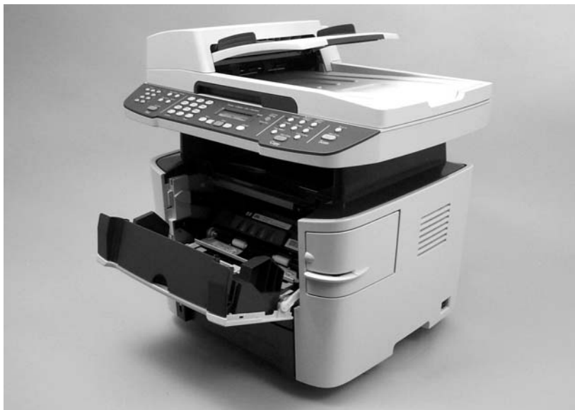
Figure 5-3 Remove the print cartridge (1 of 2)
