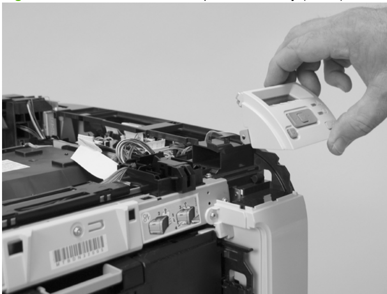
Figure 6-71 Remove the control-panel assembly (3 of 3)
