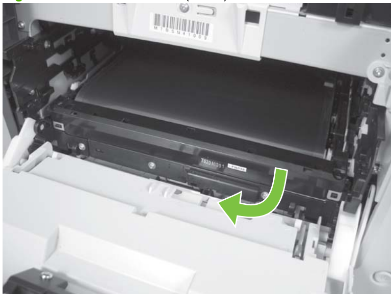
Figure 6-22 Remove the ITB (2 of 6)
