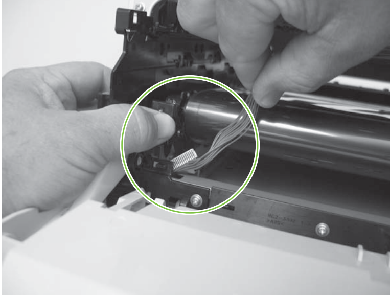
Figure 6-87 Reinstall the color-misregistration sensor assembly PCA (1 of 2)
