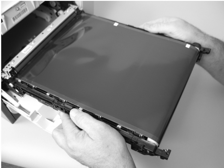
Figure 6-26 Remove the ITB (6 of 6)
