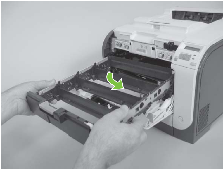
Figure 6-19 Remove the print-cartridge drawer (2 of 3)
