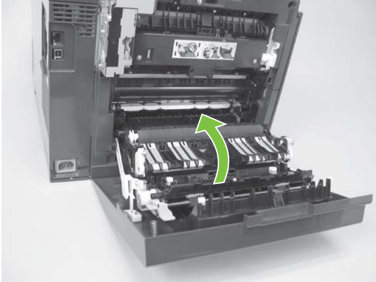
Figure 6-36 Remove the rear door (duplex product) (1 of 4)
