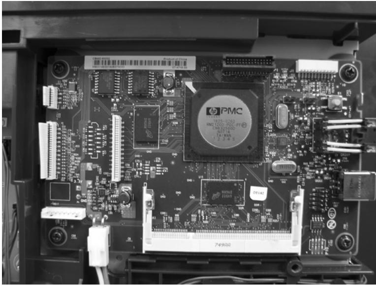
Figure 6-102 Remove the formatter PCA (1 of 2)
