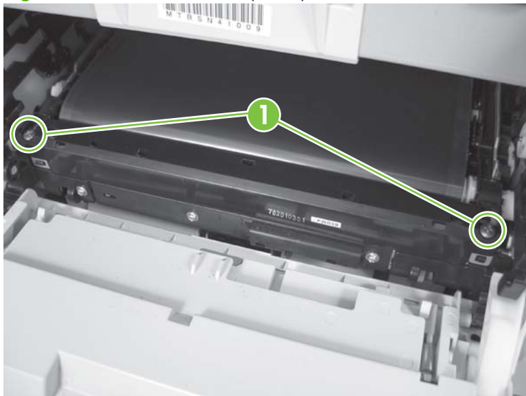
Figure 6-21 Remove the ITB (1 of 6)
