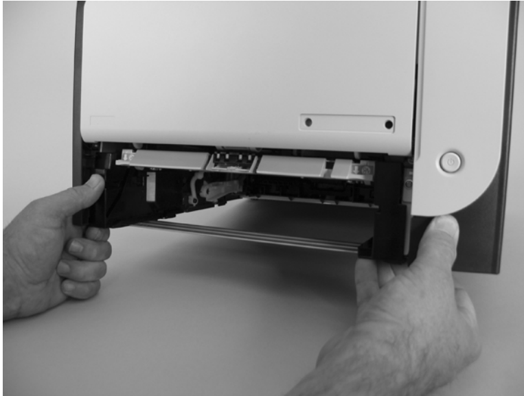
Figure 6-11 Remove the Tray 1 paper-pickup roller (2 of 3)
