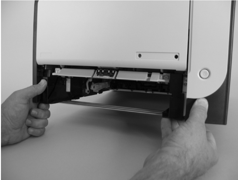
Figure 6-4 Remove the pickup roller (1 of 2)
