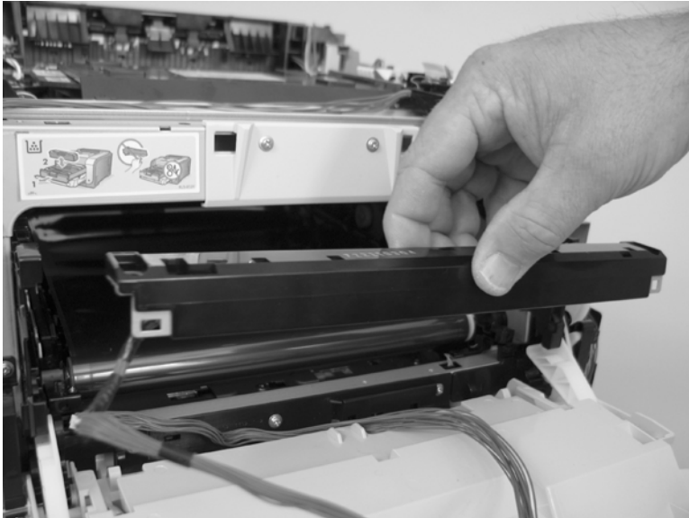
Figure 6-86 Remove the color-misregistration sensor assembly PCA (5 of 5)
