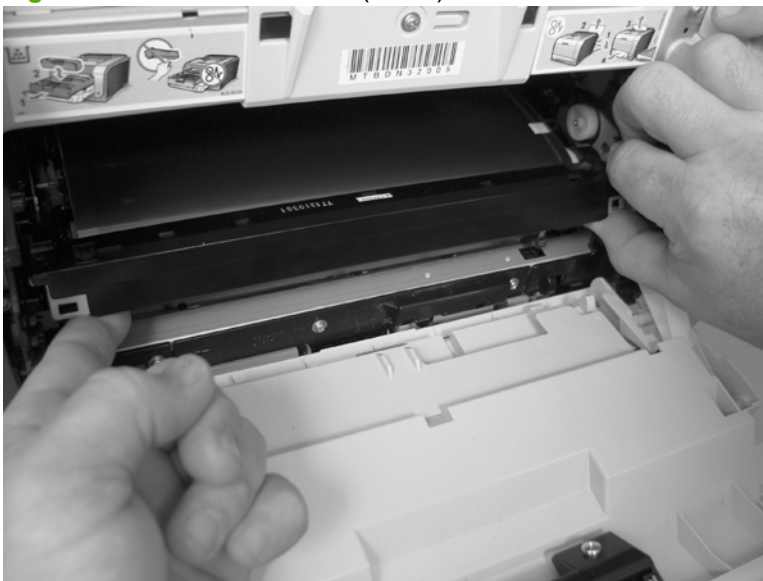
Figure 6-24 Remove the ITB (4 of 6)
