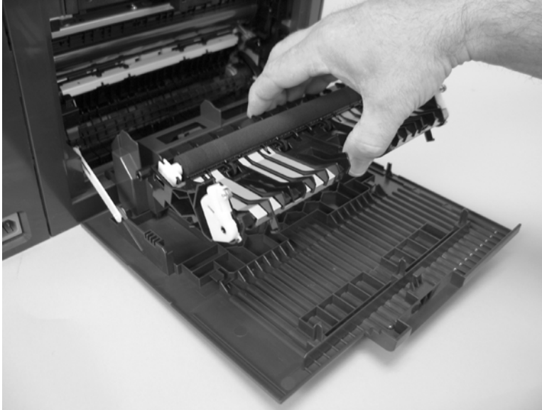
Figure 6-29 Remove the feed assembly (2 of 2)
