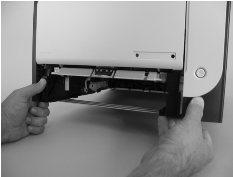
Figure 6-6 Remove the separation roller (1 of 3)
