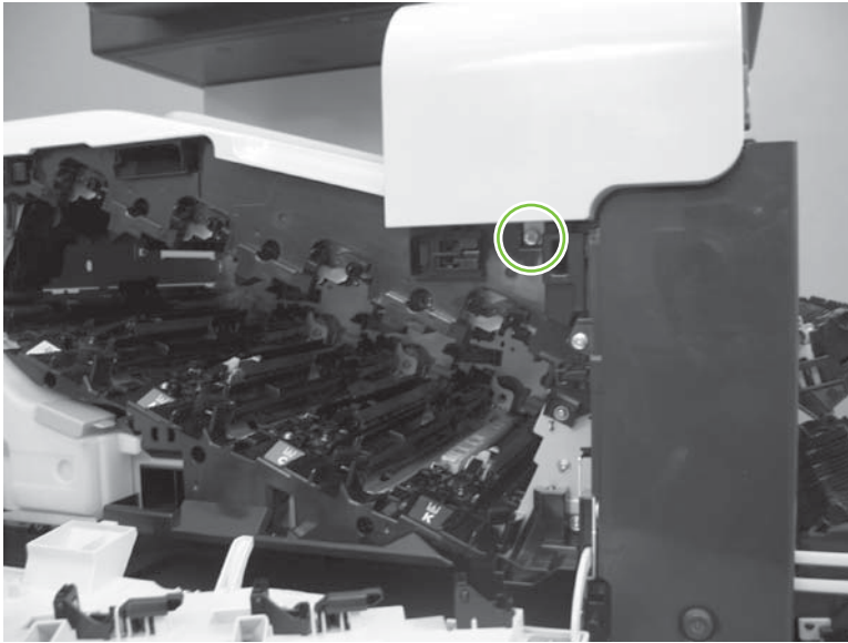
Figure 6-67 Remove the front-upper cover (3 of 4)
