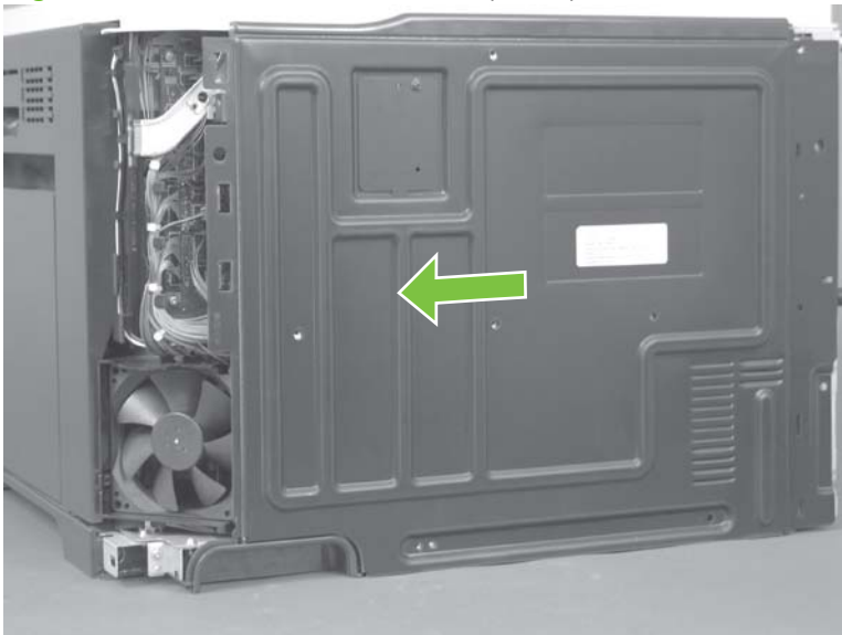
Figure 6-90 Remove the rear cover (2 of 2)
