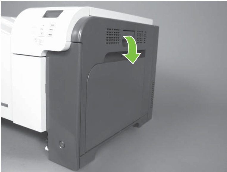
Figure 6-24 Remove the fuser (1 of 2)
