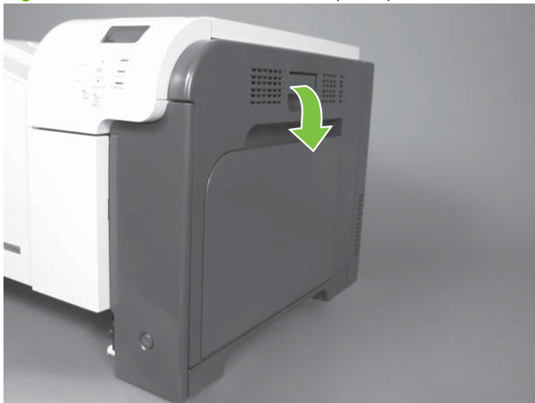
Figure 6-33 Remove the transfer roller (1 of 3)
