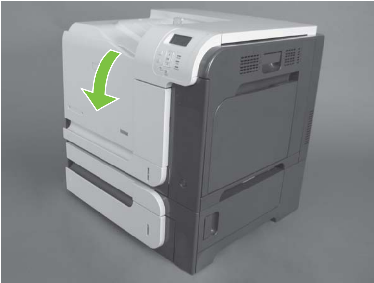
Figure 6-5 Remove the print cartridge (1 of 2)
