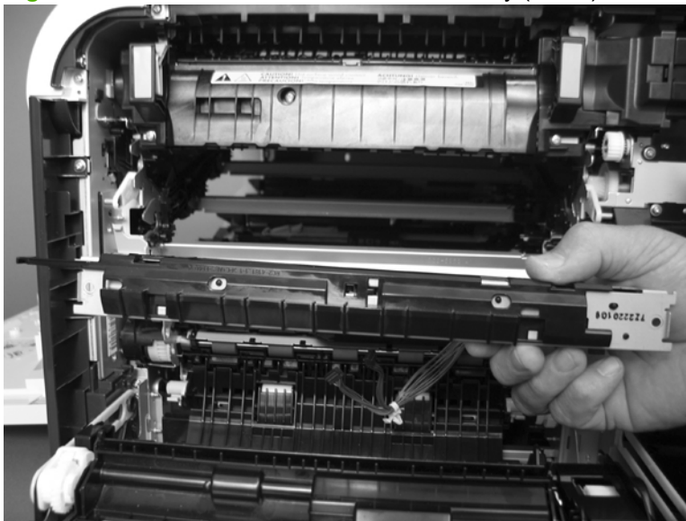
Figure 6-192 Remove the RD sensor assembly (6 of 6)
