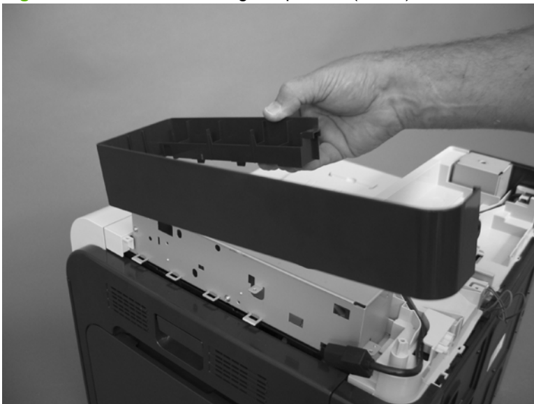
Figure 6-128 Remove the right-top cover (5 of 5)
