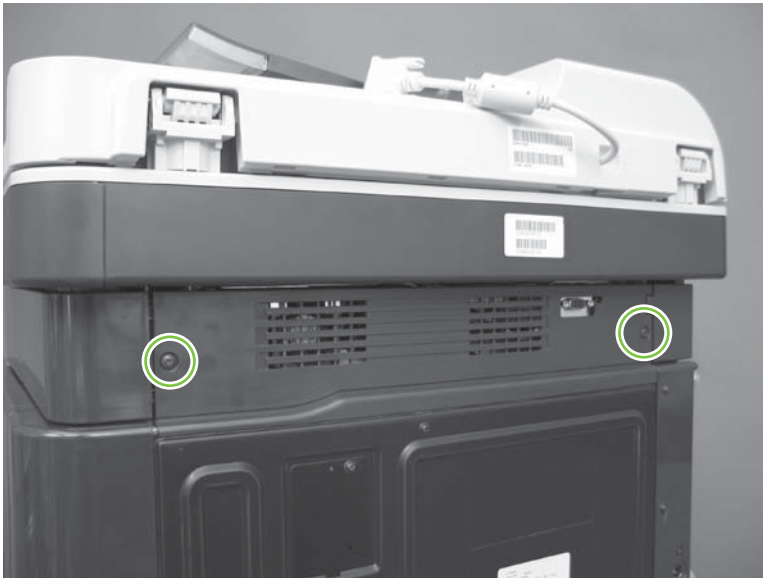
Figure 6-86 Remove the rear-upper cover (2 of 4)
