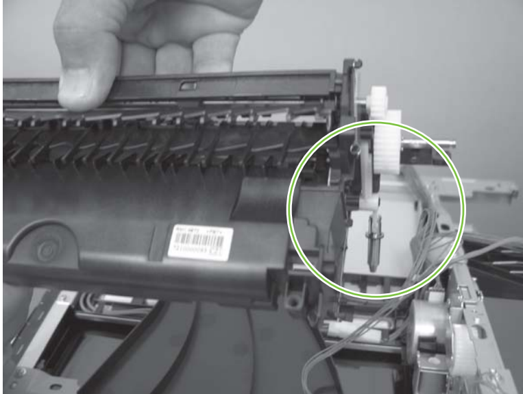
Figure 6-294 Reinstall the delivery assembly (1 of 2)
