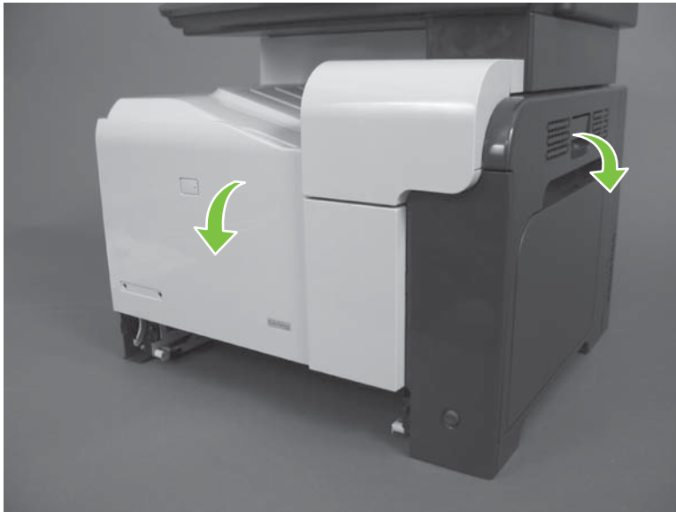
Figure 6-65 Remove the front-upper cover (1 of 4)
