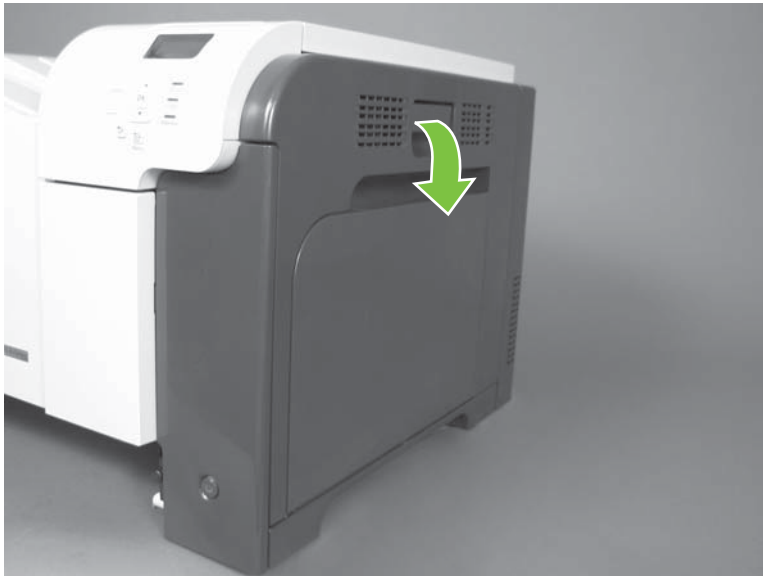
Figure 6-77 Remove the right-rear cover (1 of 3)
