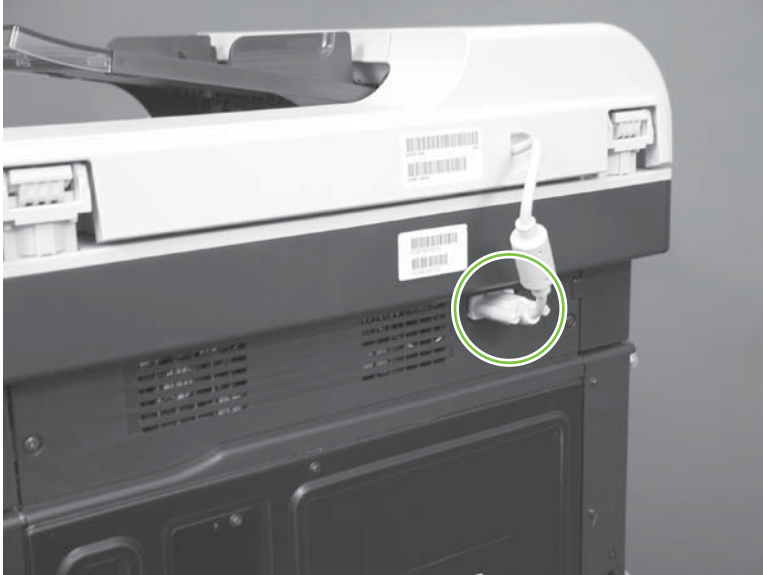
Figure 6-46 Remove the ADF assembly (1 of 4)
