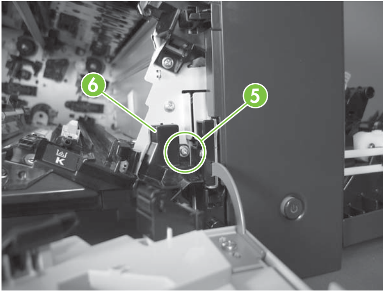
Figure 6-246 Remove the laser/scanner assembly (C/Bk) (4 of 7)
