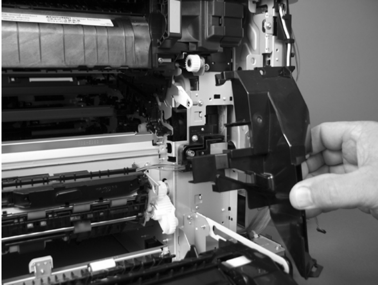
Figure 6-198 Remove the registration assembly (2 of 8)
