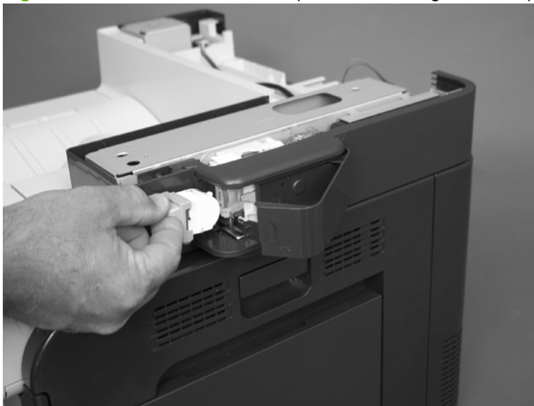
Figure 6-108 Remove the front stapler cover and right-side stapler cover (1 of 13)
