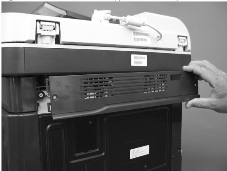
Figure 6-88 Remove the rear-upper cover (4 of 4)
