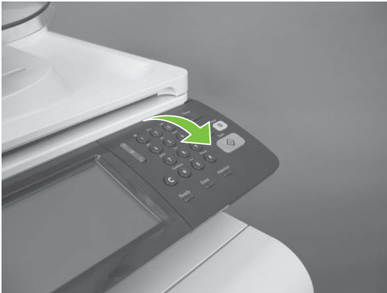
Figure 6-56 Remove the control-panel overlay (1 of 2)
