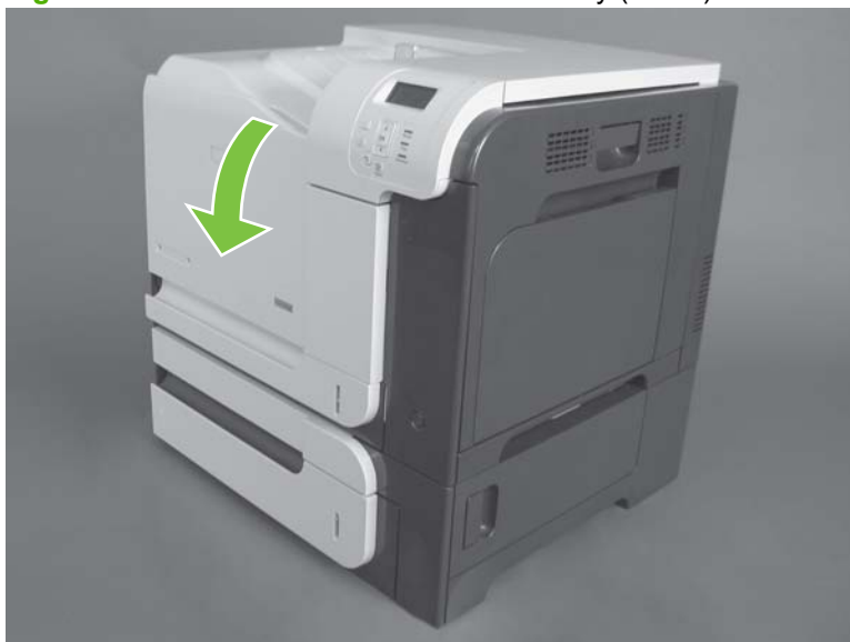
Figure 6-44 Remove the front-door assembly (1 of 2)
