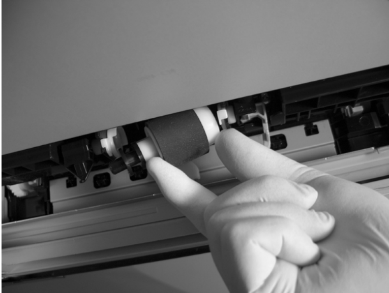
Figure 6-28 Remove the pickup roller (Tray 2) (3 of 4)
