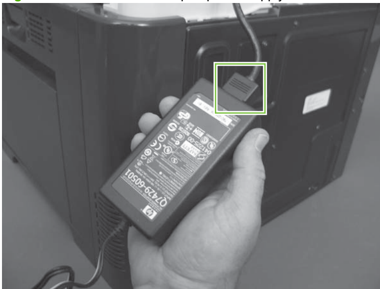
Figure 6-136 Remove the stapler power supply
