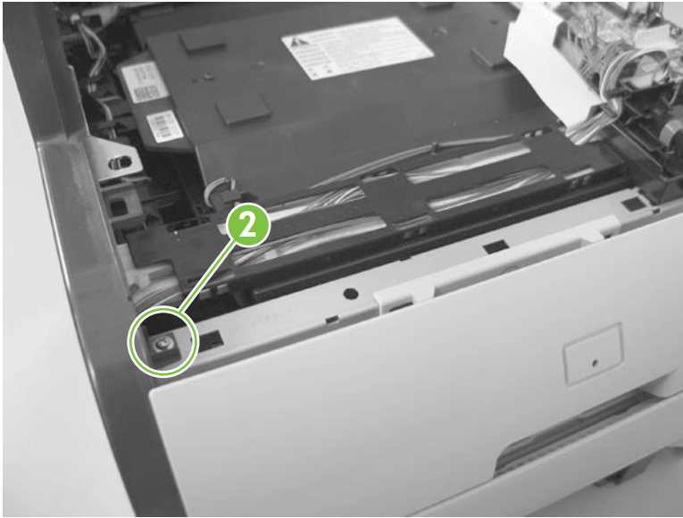
Figure 6-101 Remove the left cover (2 of 4)
