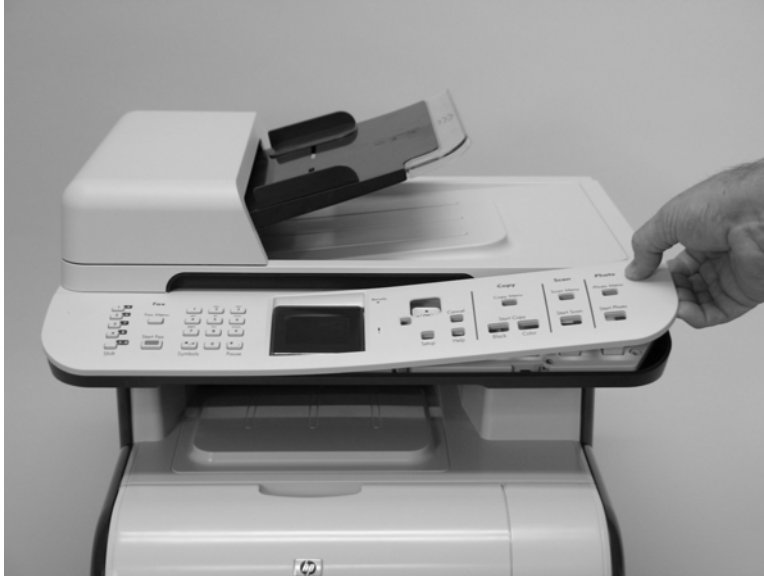
Figure 6-8 Remove the control-panel bezel (fax/memory-card models)
