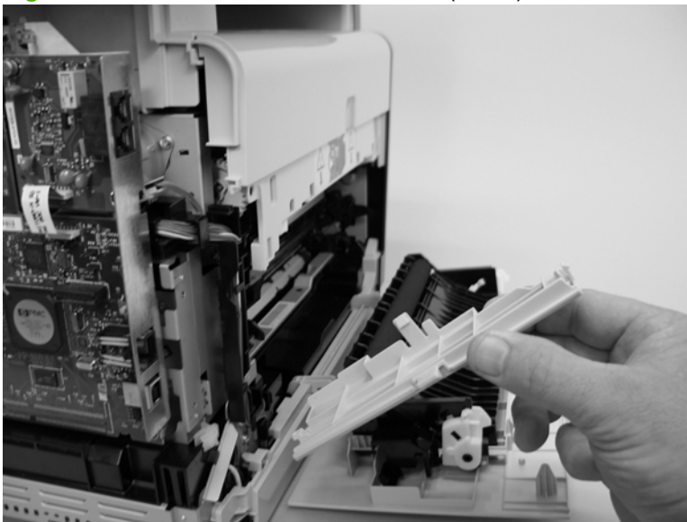
Figure 6-52 Remove the rear-side cover (2 of 2)
