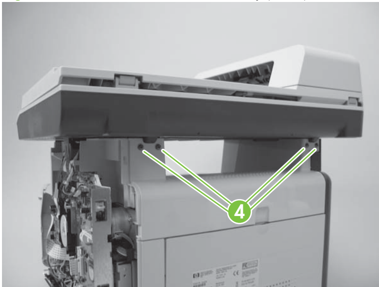
Figure 6-60 Remove the scanner assembly (2 of 4)
