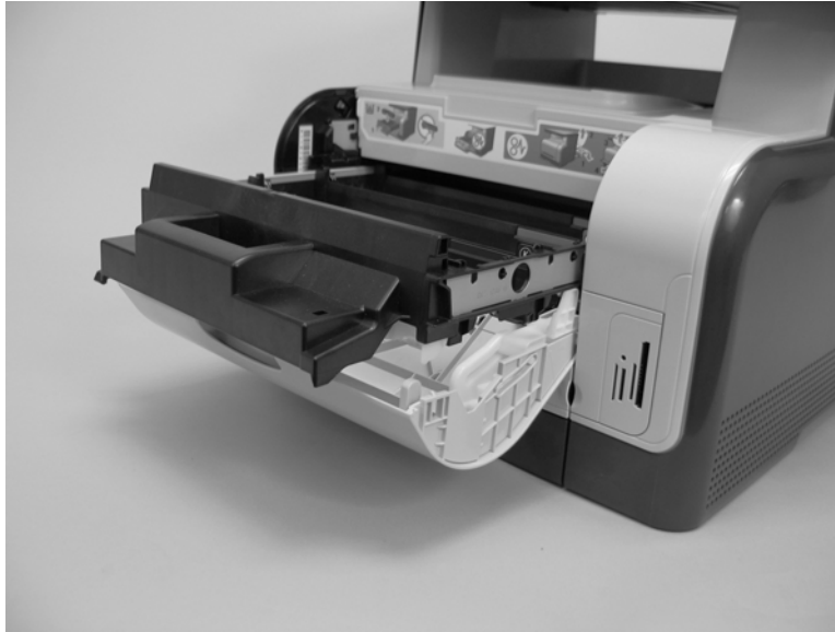
Figure 6-66 Remove the print-cartridge drawer (1 of 5)
