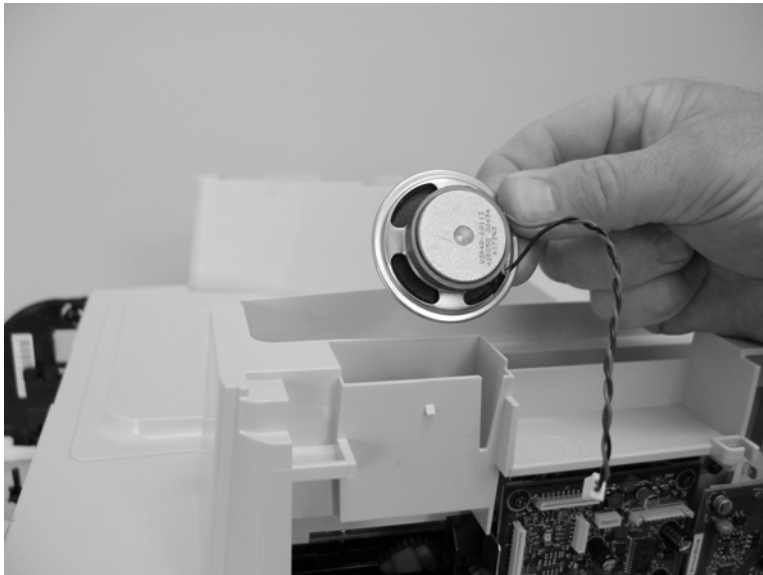
Figure 6-74 Remove the speaker (2 of 2)
