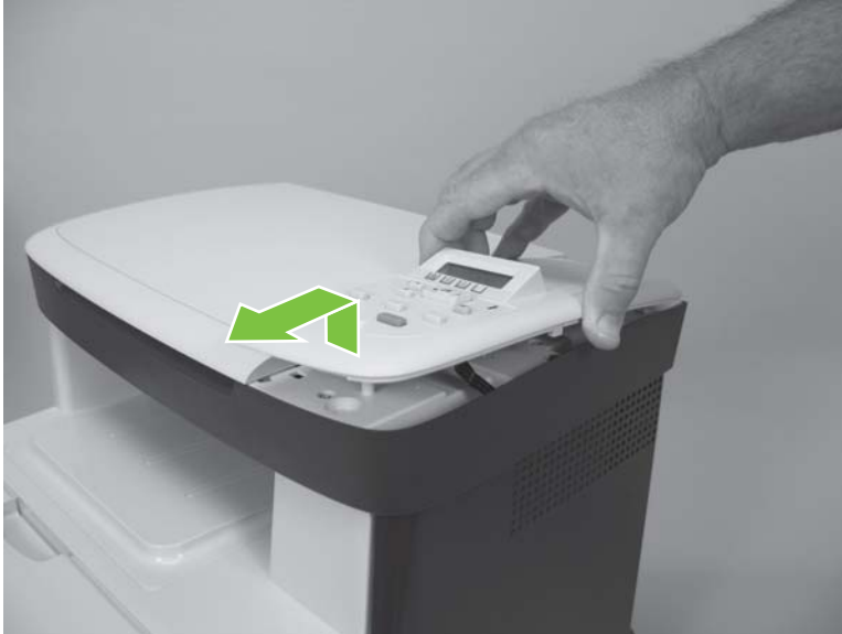
Figure 6-6 Remove the control-panel (2 of 3; base model)
