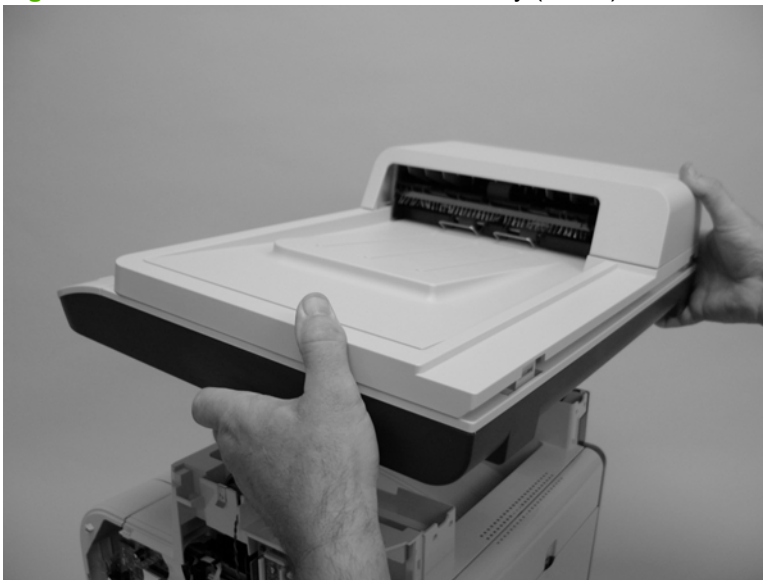
Figure 6-62 Remove the scanner assembly (4 of 4)
