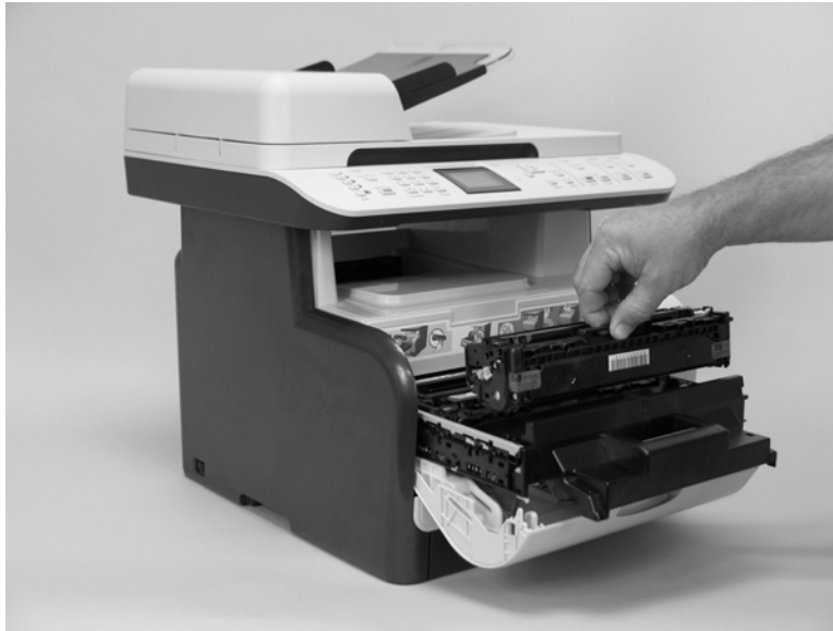
Figure 6-3 Remove the print cartridge
