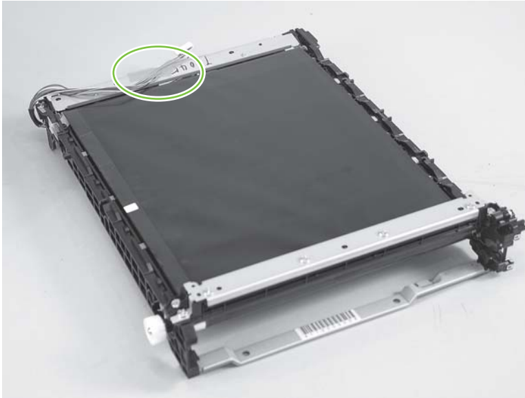
Figure 6-81 Reinstall the ITB (2 of 2)
