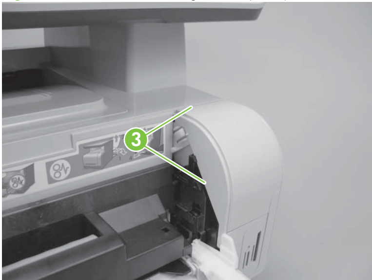
Figure 6-45 Remove the front-right cover (2 of 3)
