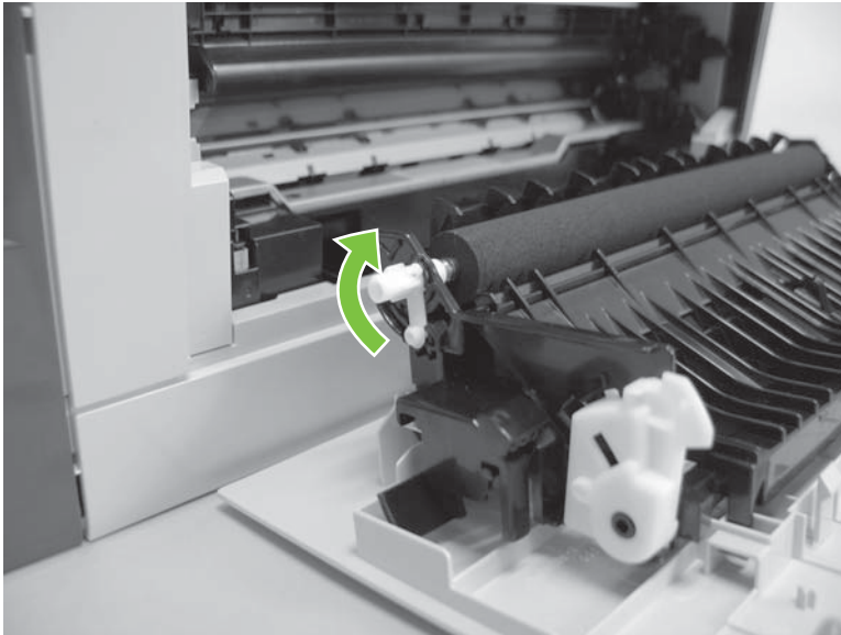
Figure 6-17 Remove the transfer roller (1 of 3)
