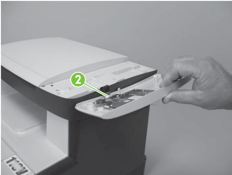
Figure 6-7 Remove the control-panel (3 of 3; base model)
