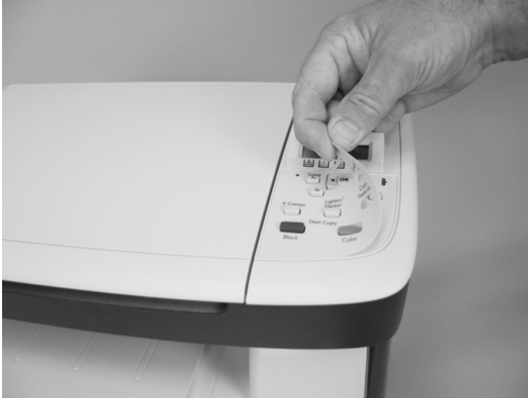
Figure 6-4 Remove the control-panel overlay (base model)
