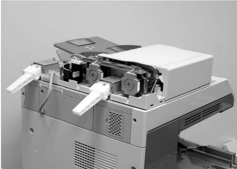
Figure 6-325 Remove the ADF hinges (1 of 3)
