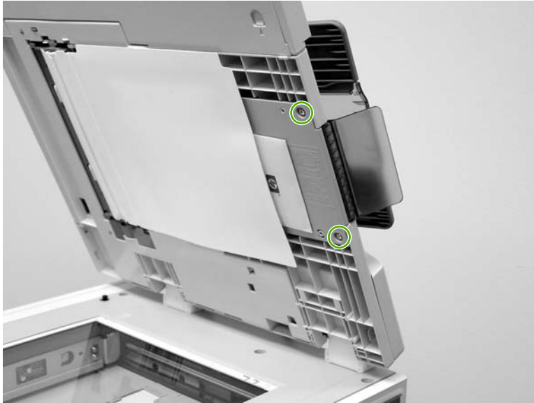
Figure 6-306 Remove the ADF output bin extension (1 of 2)
