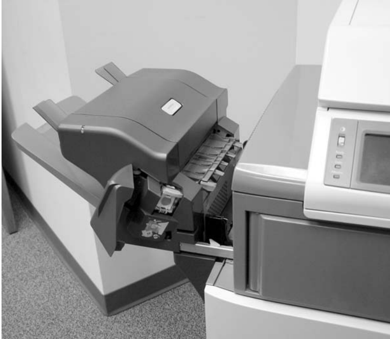
Figure 6-17 Replace the staple cartridge (1 of 3)
