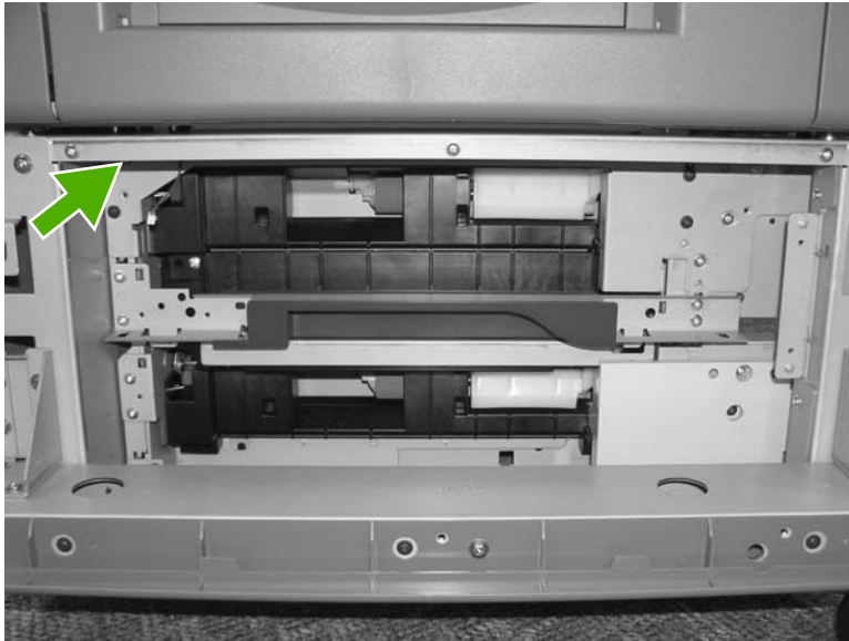
Figure 6-354 Remove the upper pickup assembly (6 of 10)
