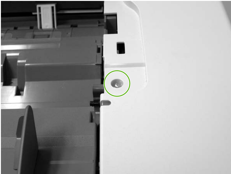
Figure 6-316 Remove the ADF rear cover (2 of 3)
