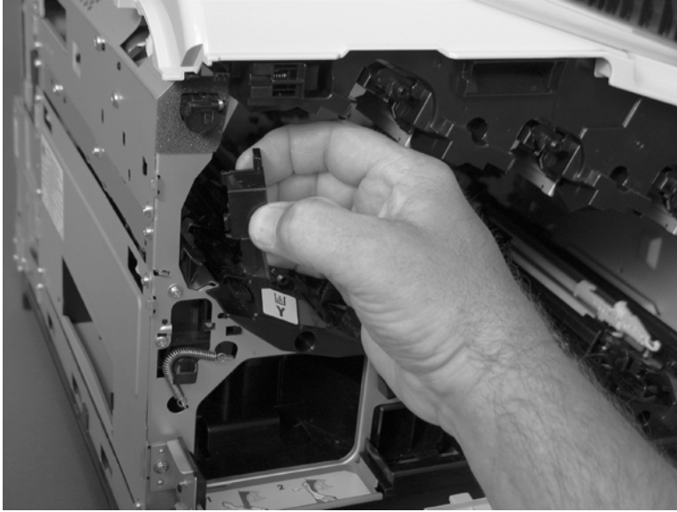
Figure 1-145 Remove the residual-toner-feed motor (2 of 7)
