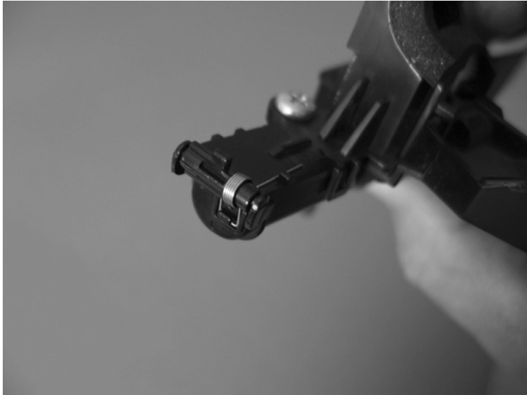
Figure 1-151 Reinstall the residual-toner collection door
