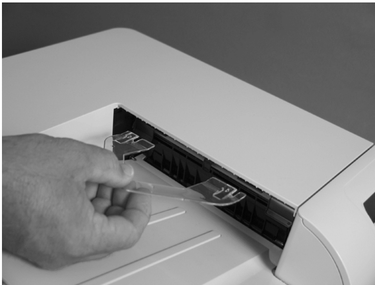
Figure 1-6 Remove the duplex-reverse guide (2 of 2)
