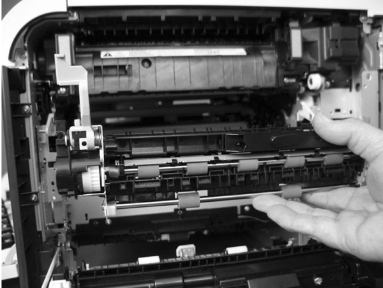
Figure 1-177 Remove the registration assembly (8 of 8)
