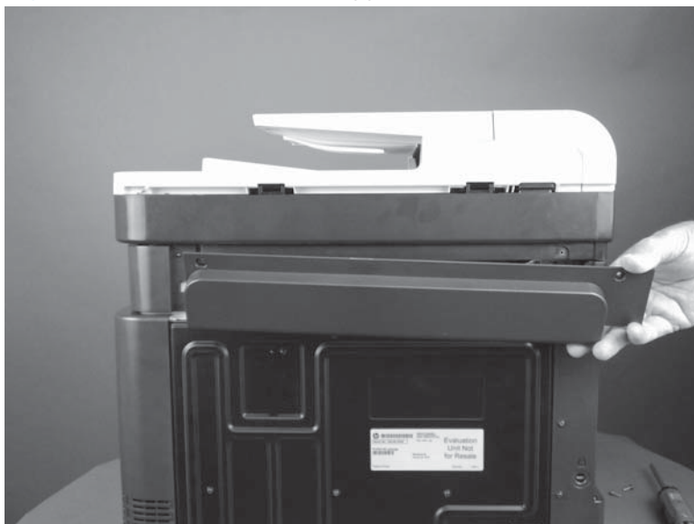
Figure 1-75 Remove the rear-upper cover (2 of 2)
