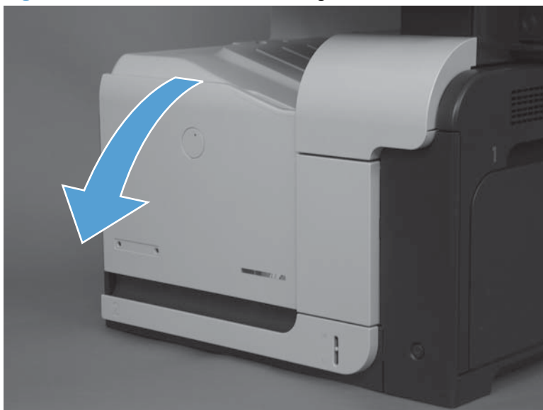
Figure 1-3 Remove the toner cartridge (1 of 2)
