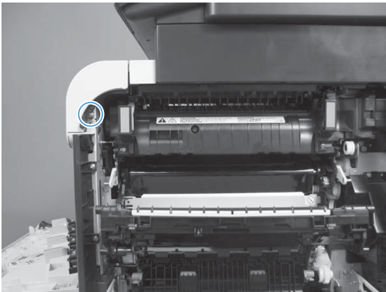
Figure 1-55 Remove the front-upper cover (2 of 4)
