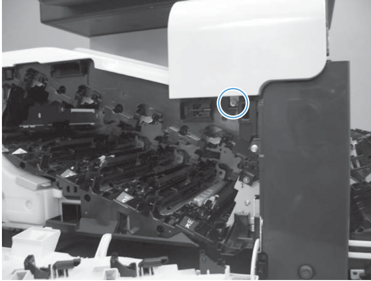
Figure 1-56 Remove the front-upper cover (3 of 4)
