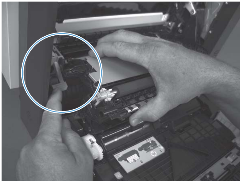
Figure 1-155 Reinstall the secondary transfer assembly
