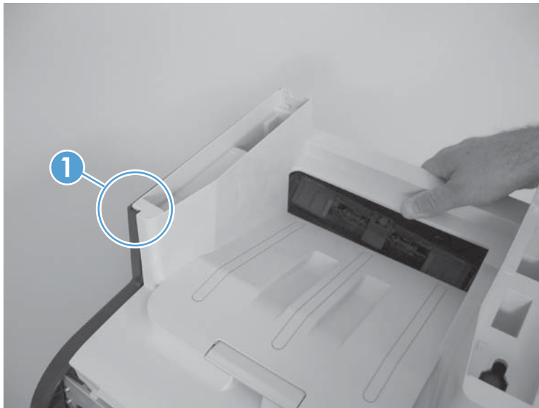
Figure 1-68 Reinstall the upper-cover assembly (1 of 3)
