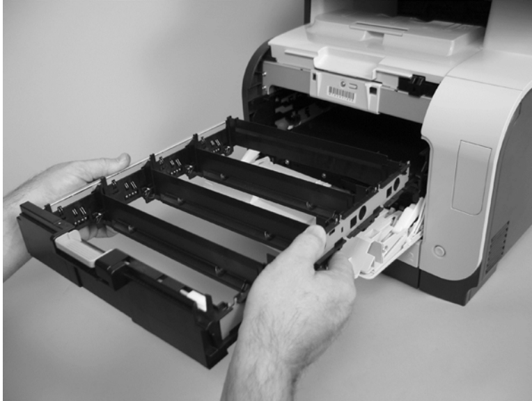
Figure 1-18 Remove the print-cartridge drawer (3 of 3)
