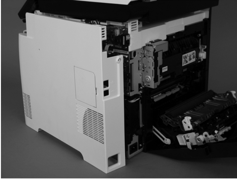
Figure 1-22 Remove the right cover (3 of 3)
