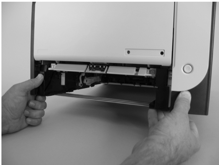
Figure 1-6 Remove the pickup roller (1 of 3)
