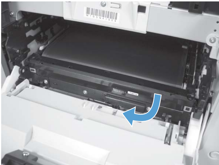
Figure 1-89 Remove the ITB (2 of 6)
