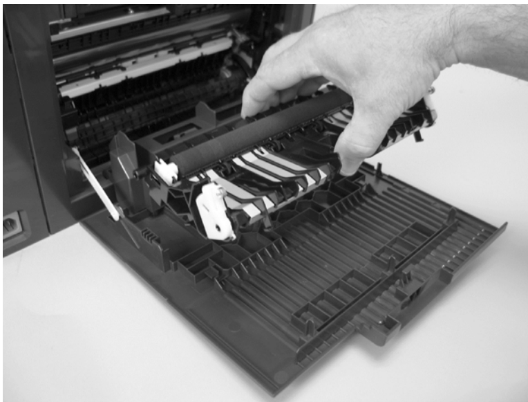
Figure 1-32 Remove the feed assembly (2 of 2)
