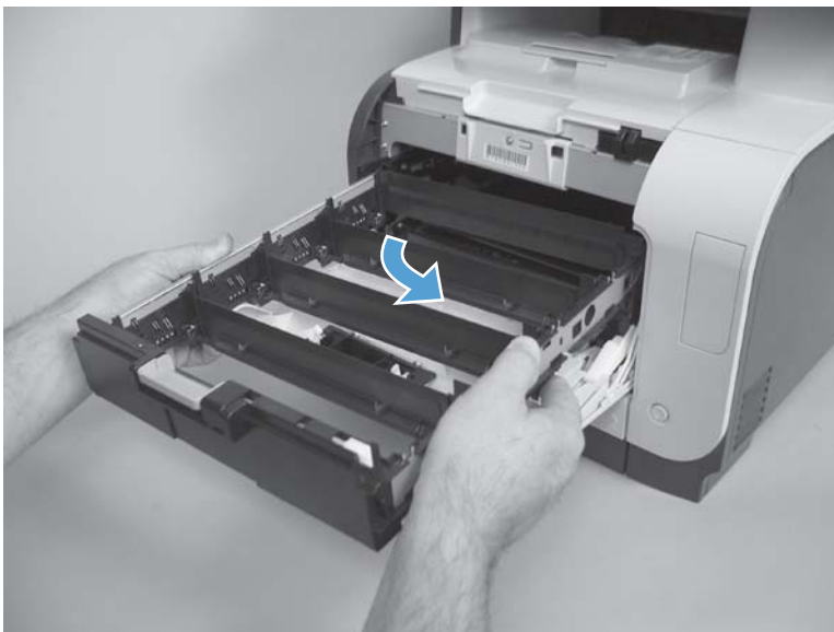
Figure 1-17 Remove the print-cartridge drawer (2 of 3)
