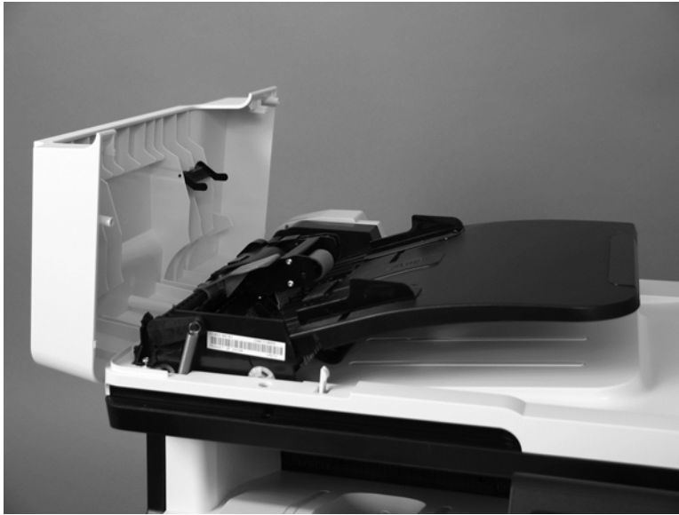
Figure 1-23 Remove the document feeder input tray (2 of 2)
