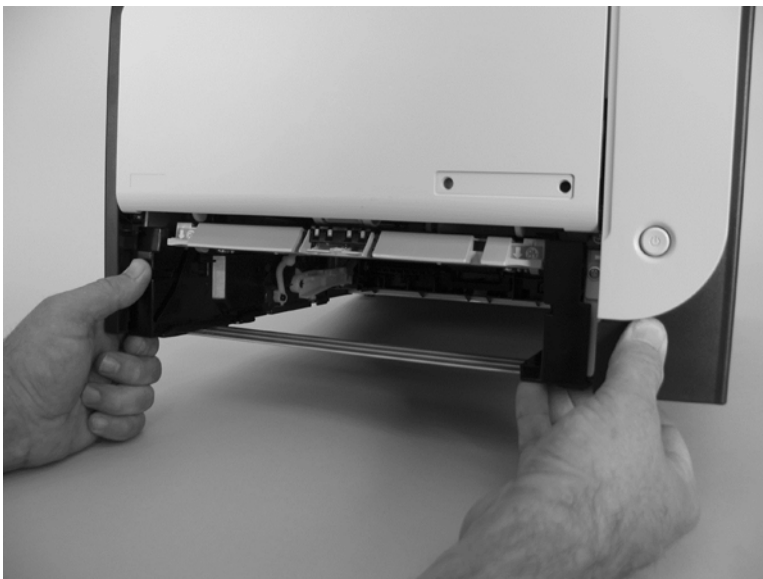
Figure 1-13 Remove the Tray 1 pickup roller (2 of 3)
