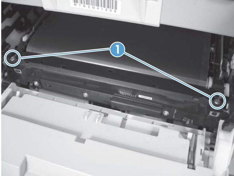
Figure 1-88 Remove the ITB (1 of 6)
