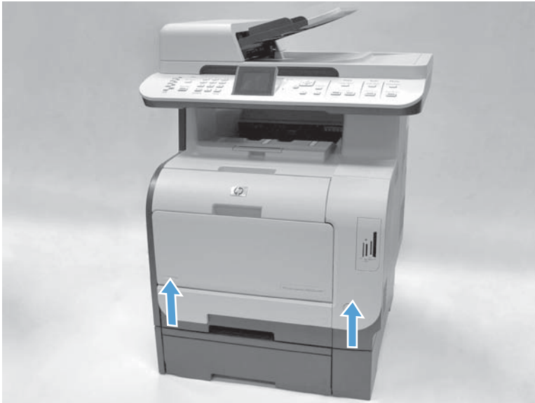
Figure 1-151 Remove the tray cassettes and optional Tray 3 assembly (2 of 2)
