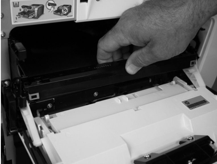
Figure 1-127 Remove the color-misregistration sensor assembly PCA (4 of 4)
