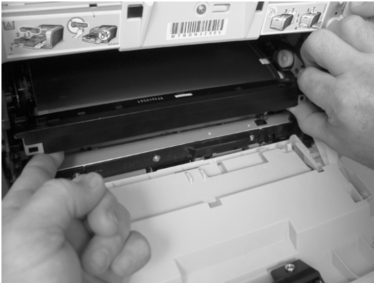
Figure 1-91 Remove the ITB (4 of 6)
