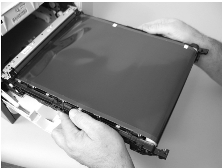
Figure 1-93 Remove the ITB (6 of 6)
