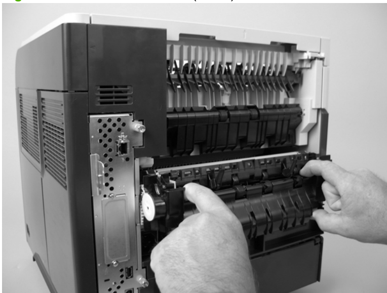
Figure 6-24 Remove the fuser (2 of 2)
