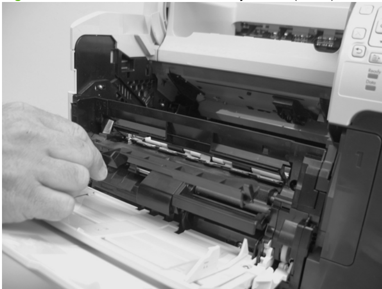
Figure 6-15 Remove the front accessory covers (1 of 2)
