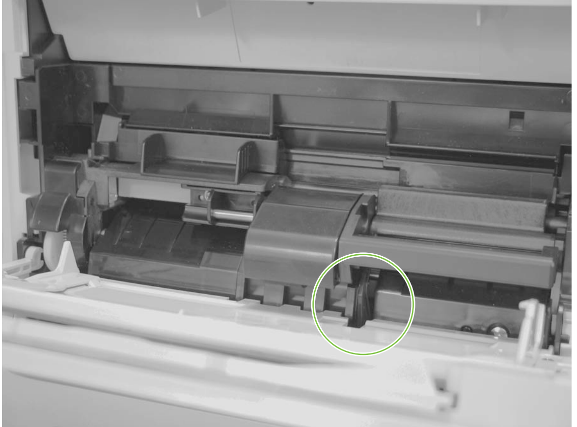
Figure 7-4 Checking the Tray 1 paper present sensor
