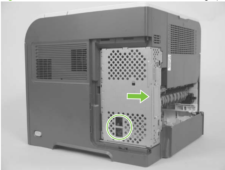
Figure 6-26 Remove the formatter cover and formatter cage (2 of 2)
