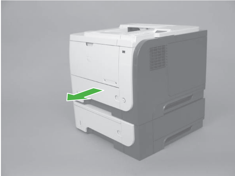
Figure 2-6 Remove the tray cassette (1 of 2)
