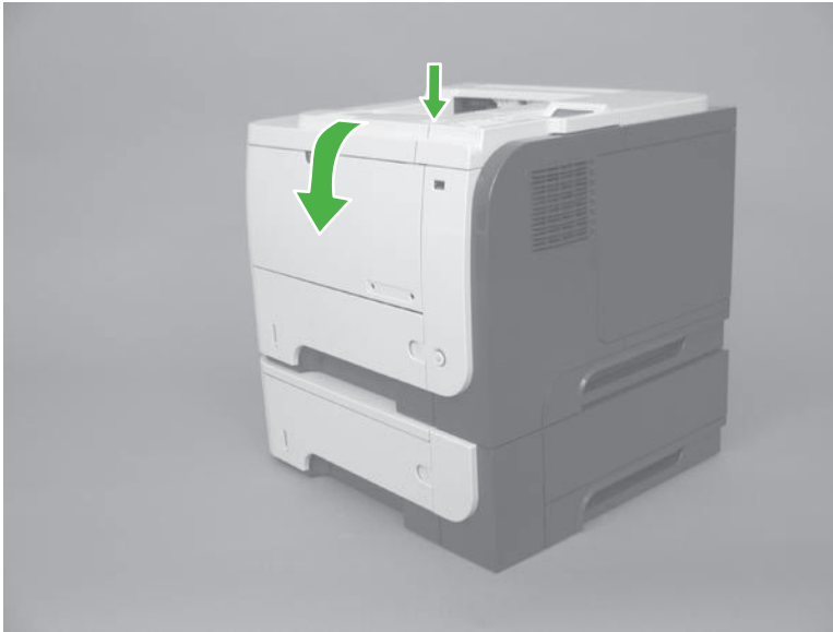
Figure 2-60 Remove the Tray 1 (MP tray) pickup roller (1 of 2)
