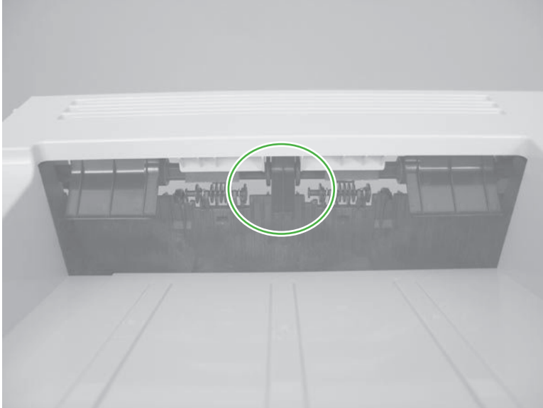
Figure 3-9 Test the face-down media tray media-full sensor
