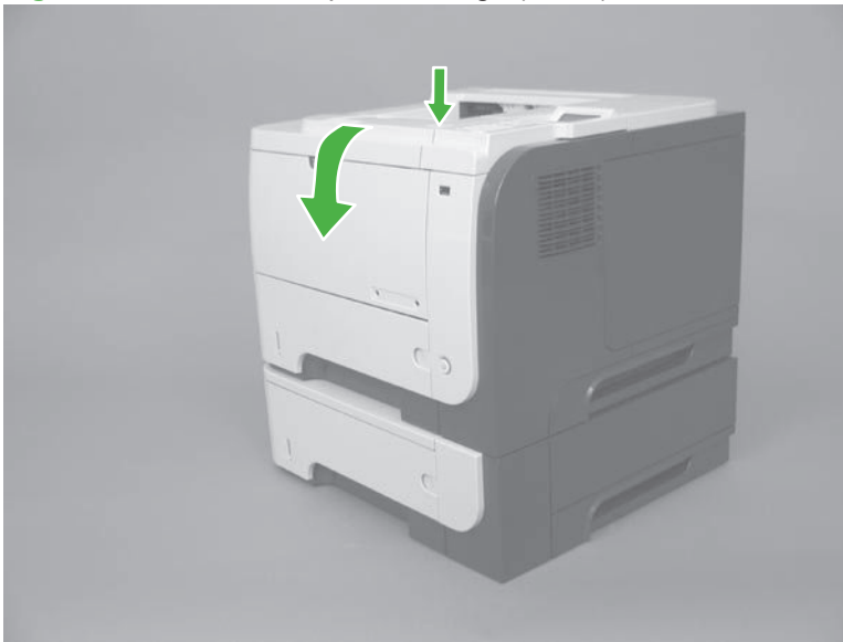
Figure 2-4 Remove the print cartridge (1 of 2)
