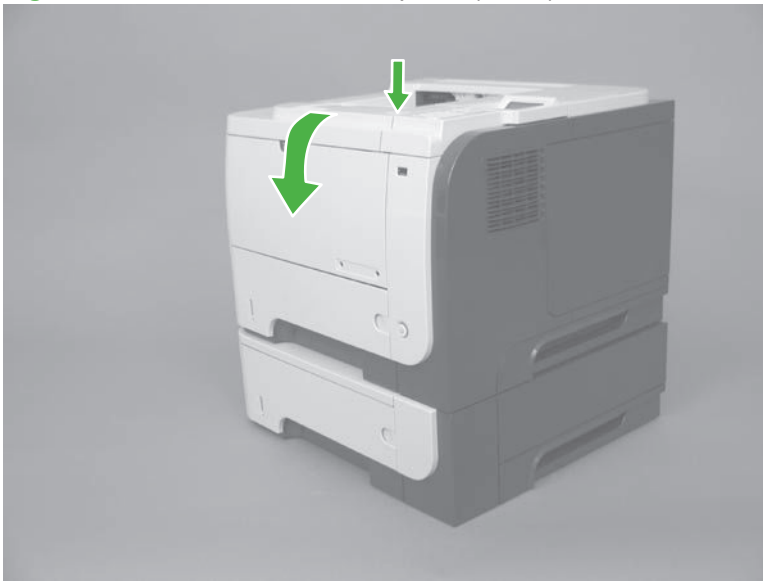
Figure 2-42 Remove the control panel (1 of 4)
