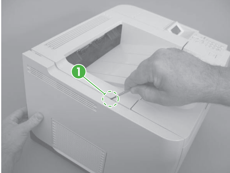
Figure 2-30 Remove the left cover (3 of 4)
