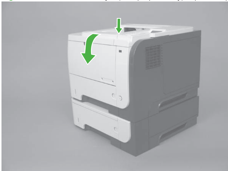
Figure 2-62 Remove the Tray 1 (multipurpose tray) separation pad (1 of 2)
