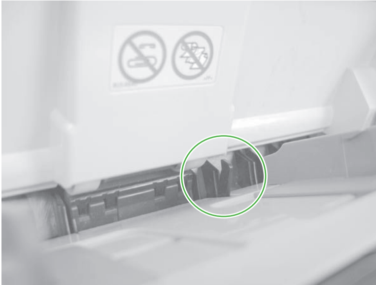
Figure 3-14 Test the Tray 1 (multipurpose tray) media-presence sensor
