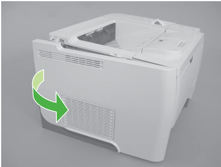
Figure 2-31 Remove the left cover (4 of 4)
