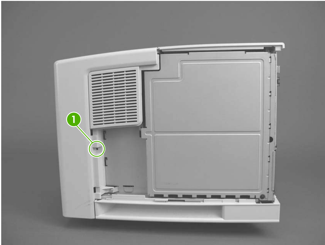
Figure 6-3 Locating the engine-test-page switch
