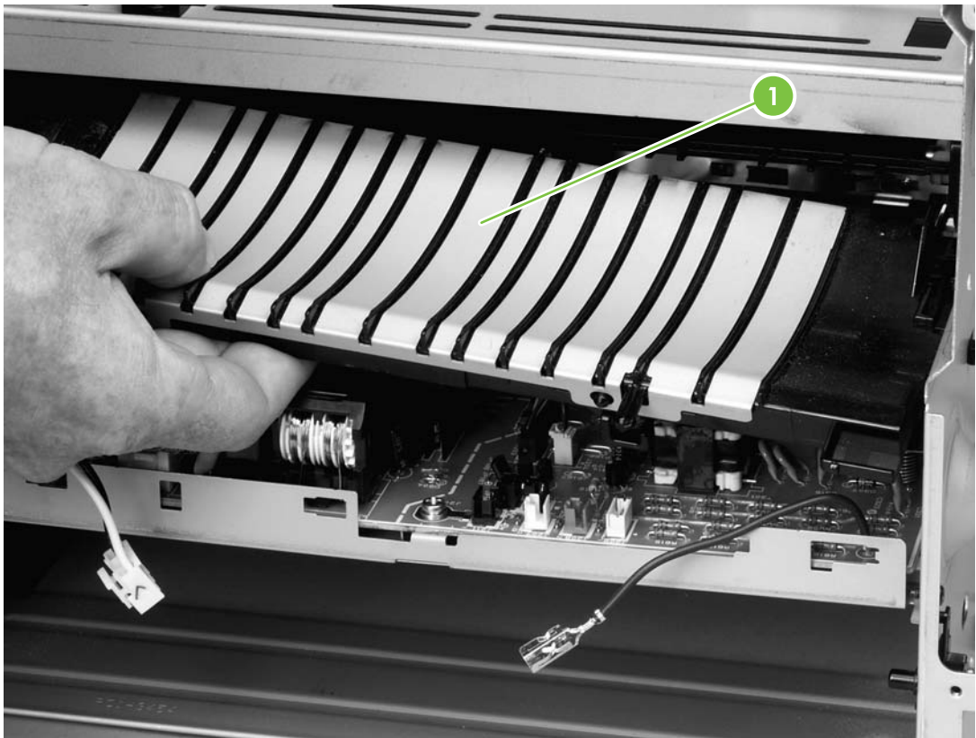
Figure 6-27 Removing the ECU (1 of 7)
