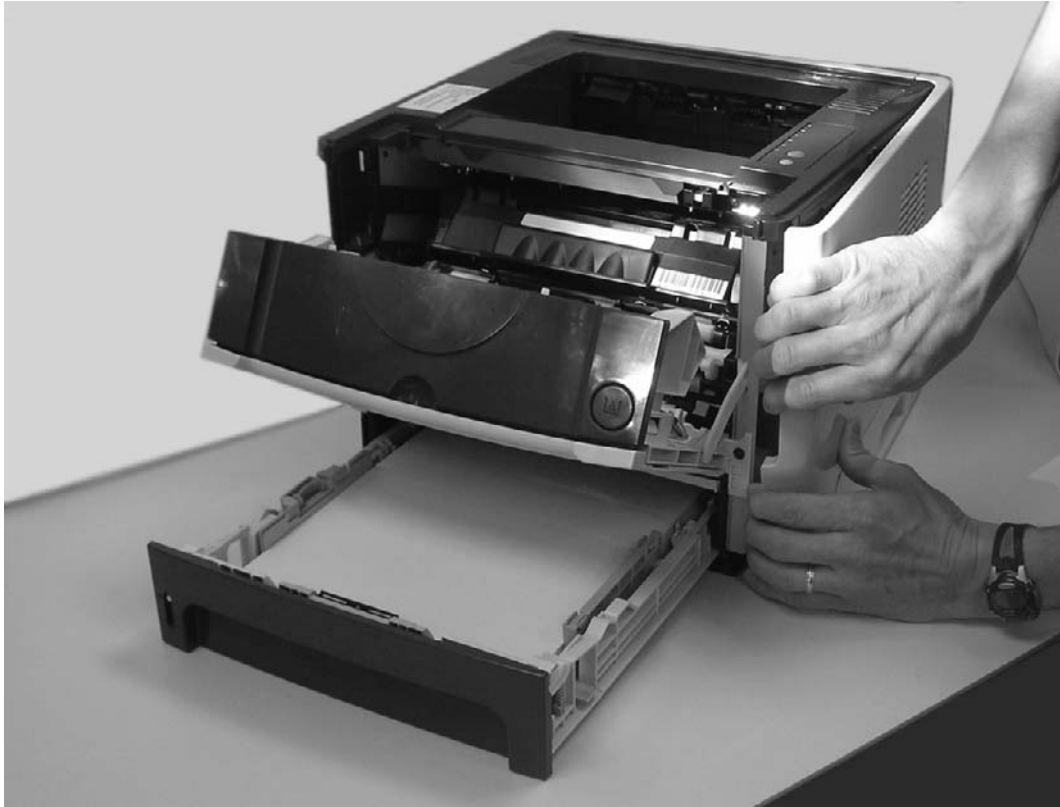
Figure 6-2 Removing the right-side cover
