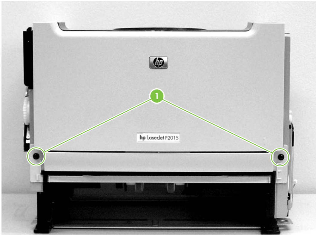
Figure 6-46 Removing the print-cartridge door (2 of 2)
