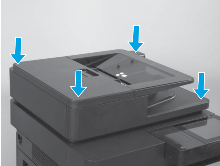
Figure 1-41 Install a replacement document feeder white backing (M830; 4 of 6)
