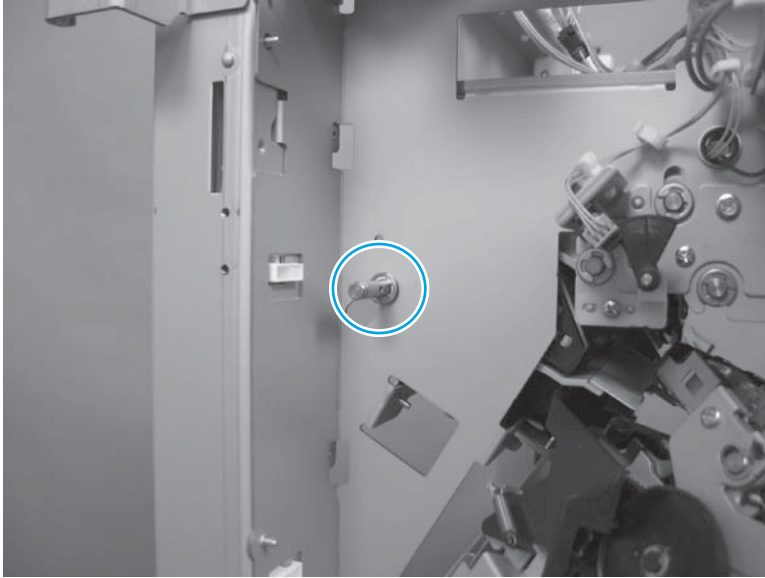
Figure 1-642 Remove the operation tray assembly (3 of 11)
