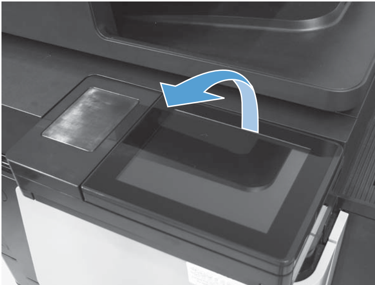
Figure 1-60 Remove the control-panel assembly (M830; 1 of 7)
