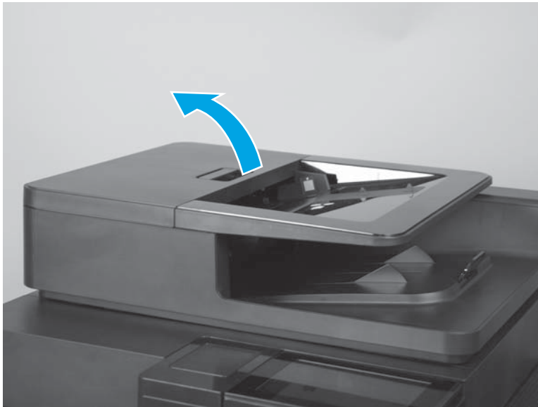
Figure 1-29 Remove the document feeder mylar strip (M830; 1 of 3)
