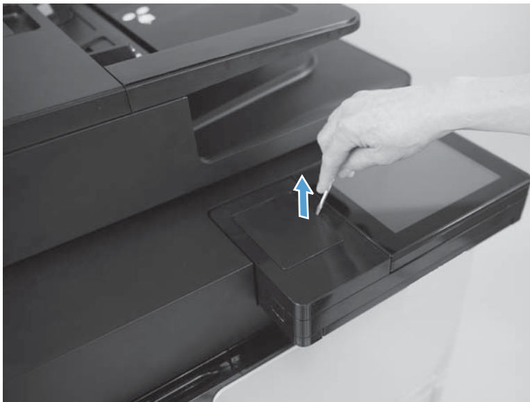
Figure 1-136 Remove the HIP cover (M830; 2 of 3)
