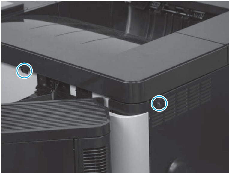
Figure 1-148 Remove the right top cover (M806; 3 of 4)
