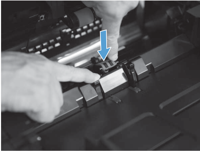
Figure 1-94 Reinstall the document-feeder separation pad (M830; 3 of 5)
