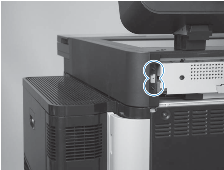
Figure 1-115 Remove the scanner right cover (M830; 2 of 4)
