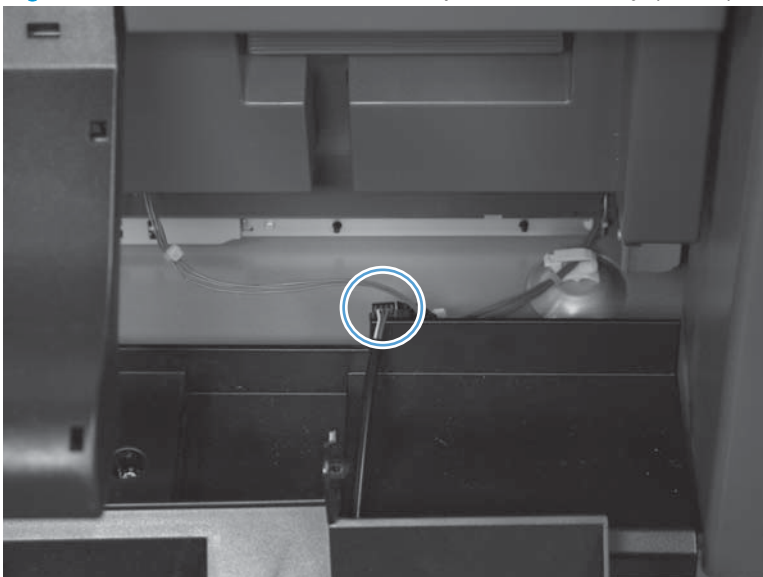
Figure 1-718 Remove the saddle output bin assembly (2 of 2)
