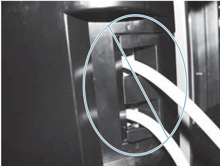
Figure 1-484 Bin cable guide cover incorrectly installed
