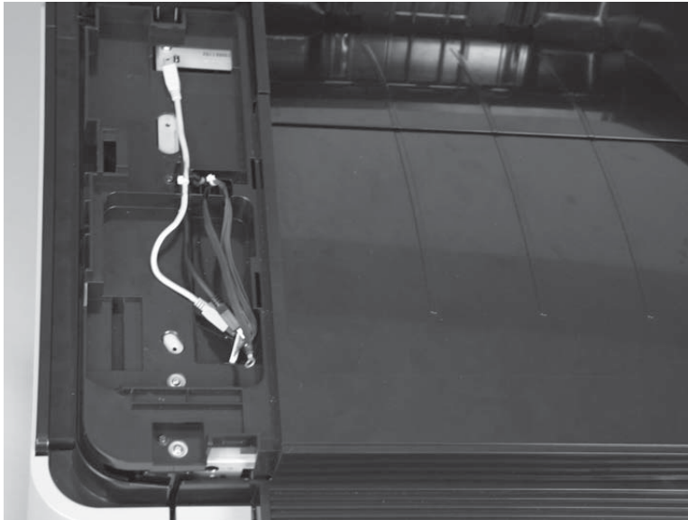
Figure 1-152 Reinstall the right top cover (M806; 3 of 3)
