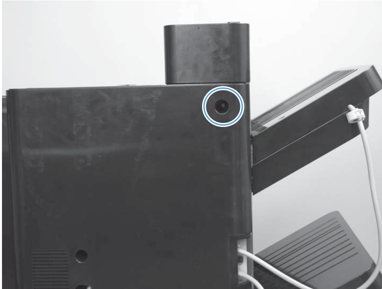
Figure 1-492 Remove the lower stepped cover assembly (2 of 5)
