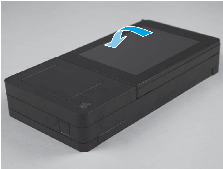
Figure 1-73 Remove the keyboard assembly (M830; 4 of 7)
