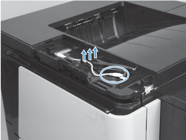
Figure 1-146 Remove the right top cover (M806; 1 of 4)
