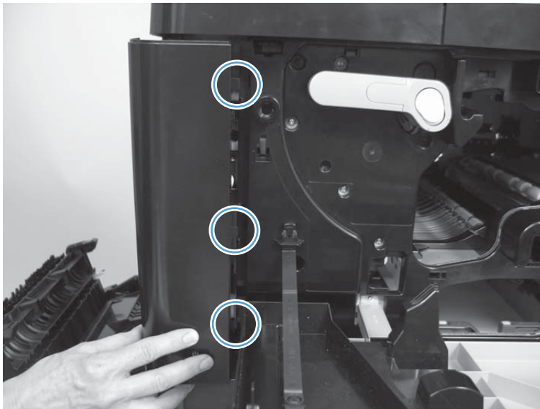
Figure 1-185 Remove the left front cover (2 of 2).
