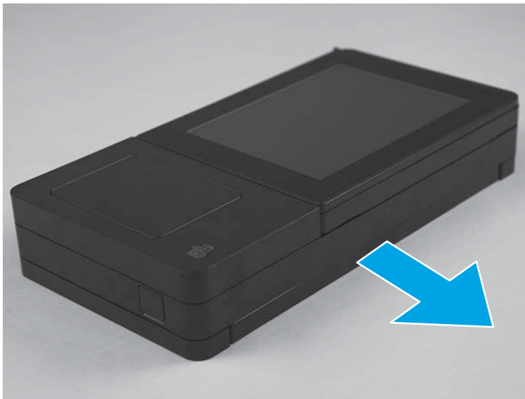
Figure 1-74 Remove the keyboard assembly (M830; 5 of 7)
