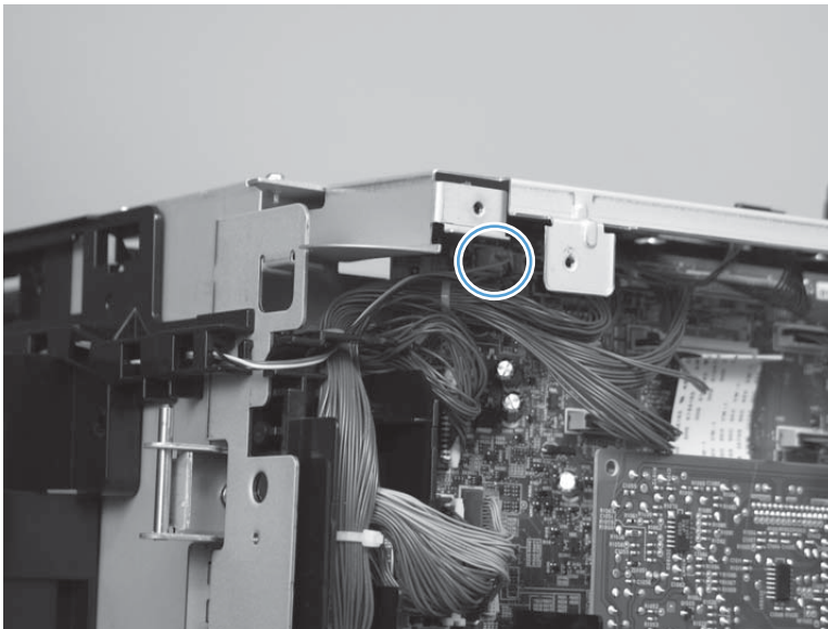
Figure 1-239 Remove the cartridge fan (1 of 5)
