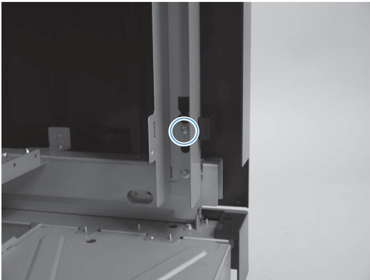
Figure 1-473 Remove the rear reverse cover assembly (2 of 3)
