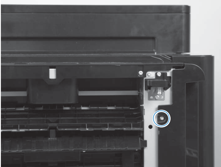
Figure 1-472 Remove the rear reverse cover assembly (1 of 3)
