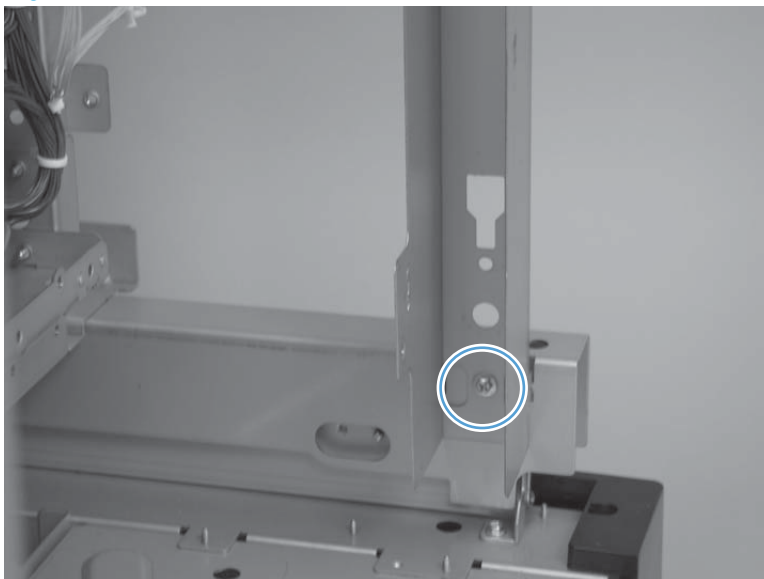
Figure 1-794 Remove the saddle assembly (6 of 15)
