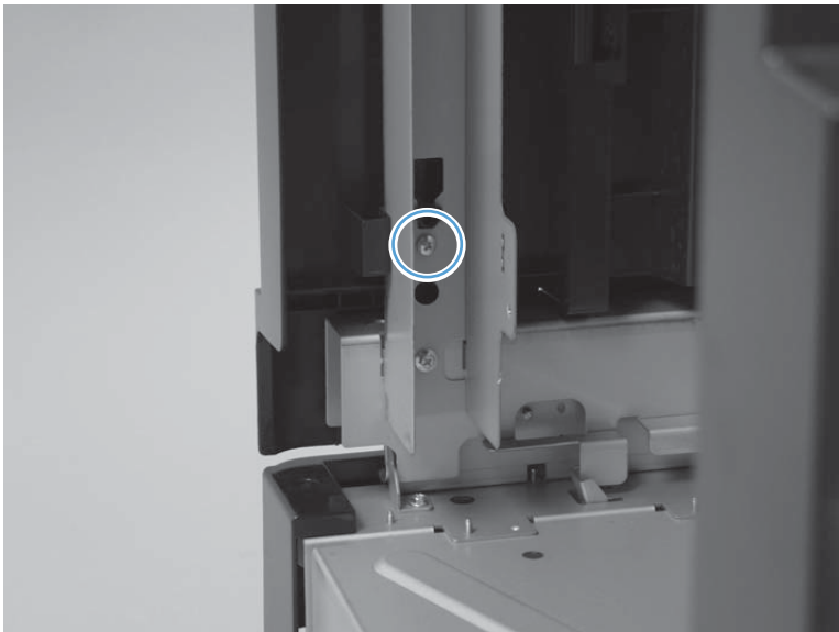
Figure 1-470 Remove the pre-reverse cover assembly (2 of 3)
