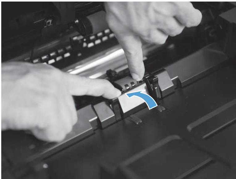
Figure 1-95 Reinstall the document-feeder separation pad (M830; 4 of 5)
