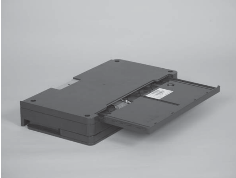
Figure 1-75 Remove the keyboard assembly (M830; 6 of 7)
