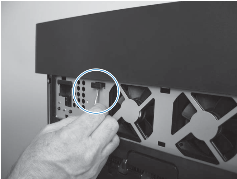
Figure 1-218 Remove the scanner assembly (M830; 1 of 4)
