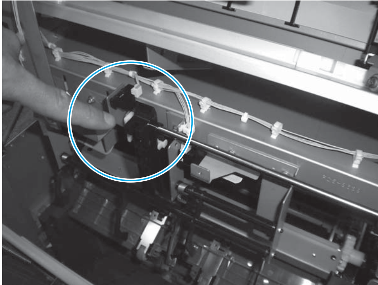
Figure 1-612 Reinstall the height wall assembly
