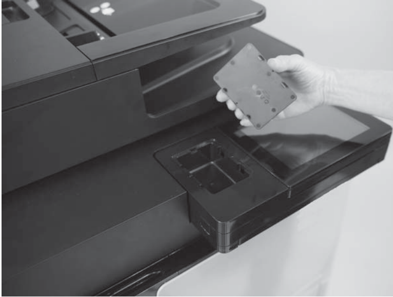
Figure 1-137 Remove the HIP cover (M830; 3 of 3)
