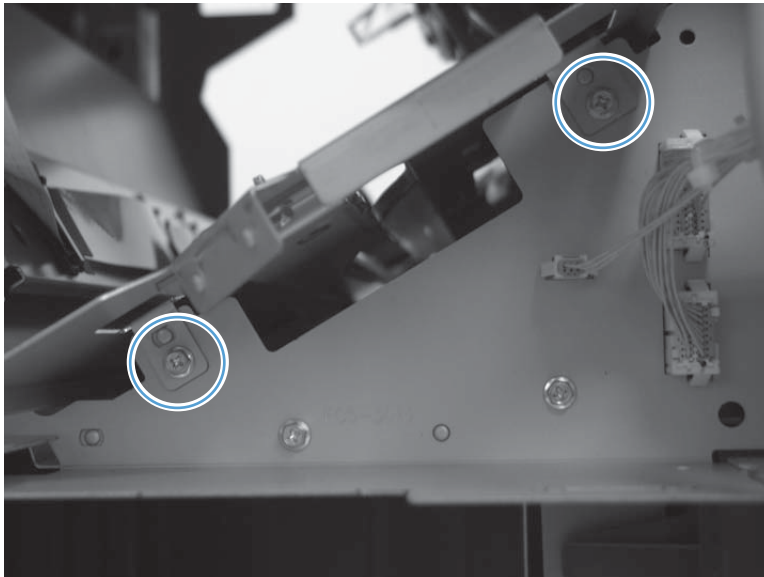
Figure 1-630 Remove the staple assembly (1 of 7)
