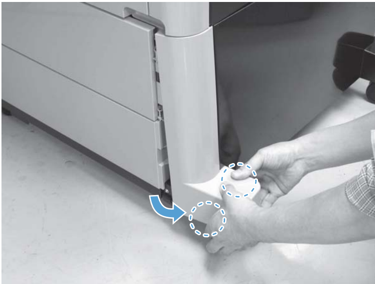
Figure 1-418 Remove the HCI rear and right-rear corner covers (2 of 4)
