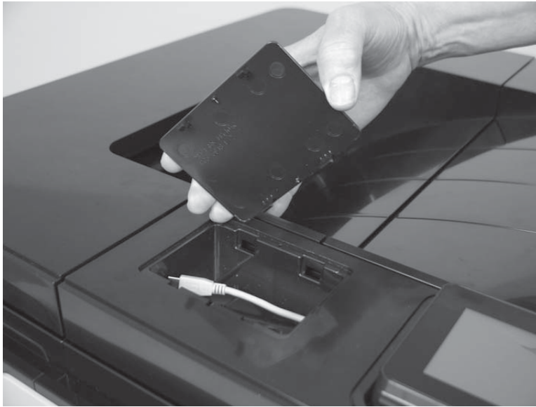
Figure 1-132 Remove the HIP cover (M806; 3 of 3)
