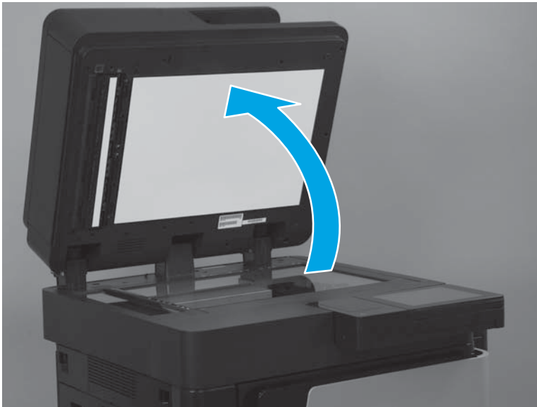
Figure 1-35 Remove the document feeder white backing (M830; 1 of 3)
