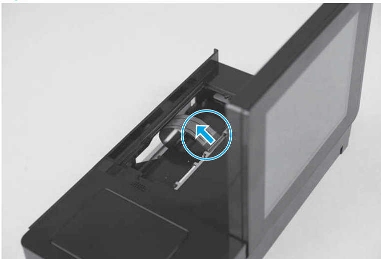
Figure 1-72 Remove the keyboard assembly (M830; 3 of 7)
