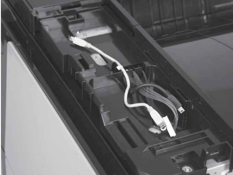
Figure 1-143 Reinstall the control-panel base cover (M806; 1 of 3)
