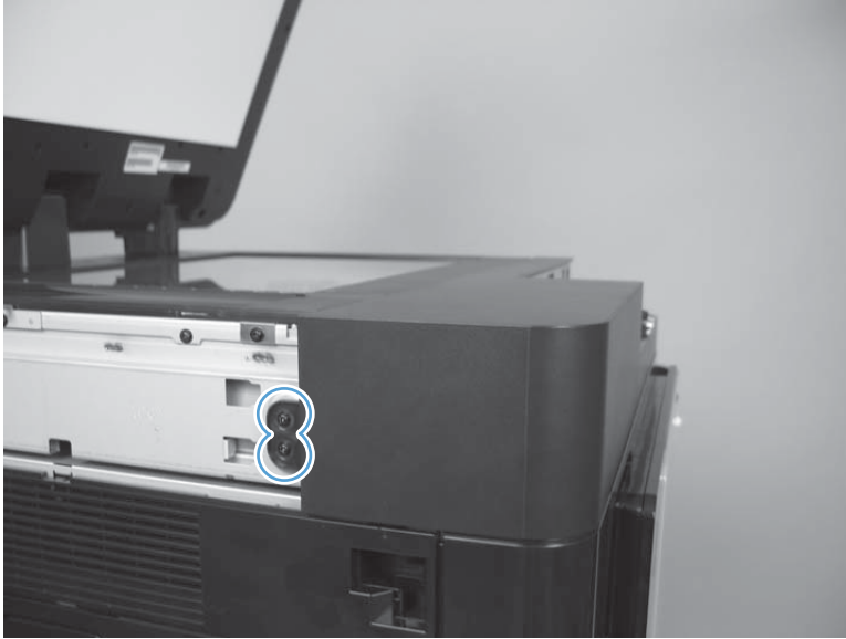
Figure 1-121 Remove the scanner front cover (M830; 4 of 7)
