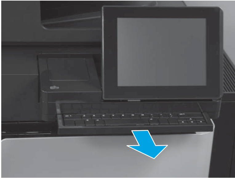
Figure 1-62 Remove the control-panel assembly (M830; 3 of 7)
