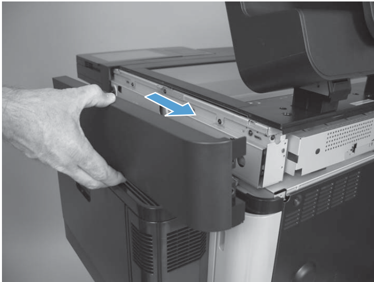
Figure 1-117 Remove the scanner right cover (M830; 4 of 4)
