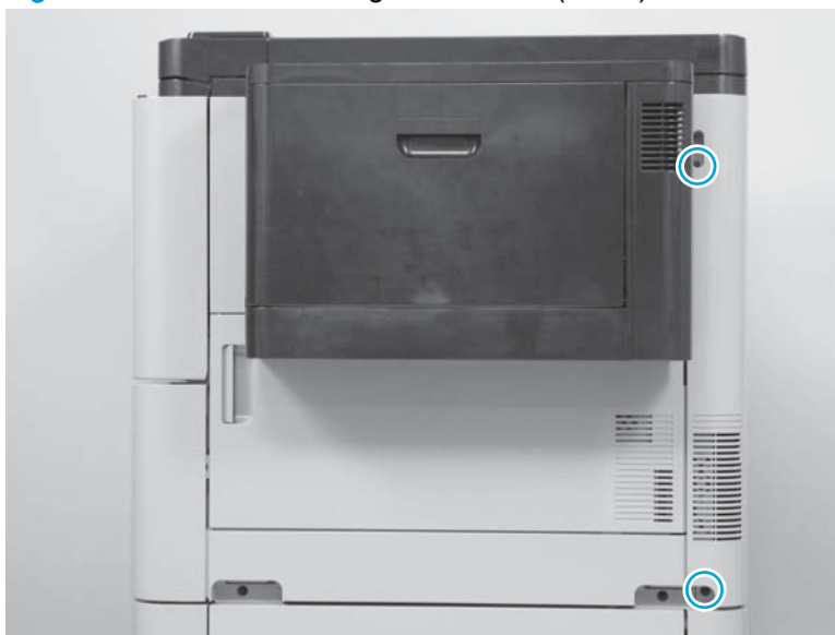
Figure 1-170 Remove the right rear cover (1 of 5)
