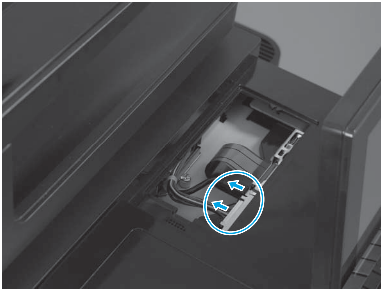
Figure 1-63 Remove the control-panel assembly (M830; 4 of 7)
