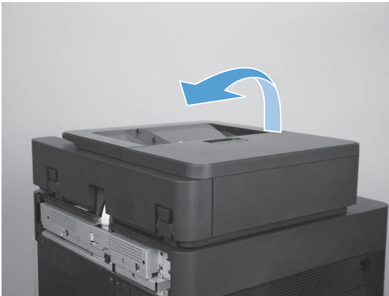
Figure 1-118 Remove the scanner front cover (M830; 1 of 7)
