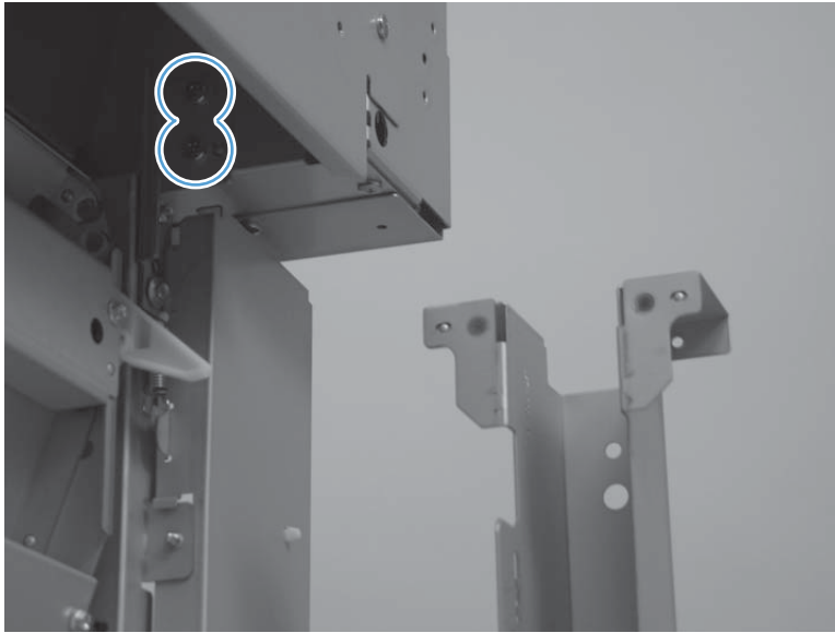
Figure 1-714 Remove the paper pass assembly (6 of 7)
