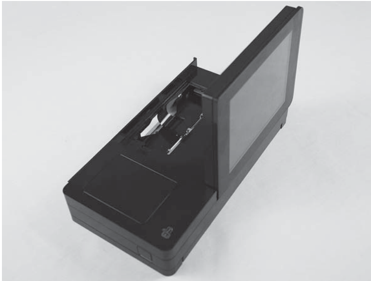
Figure 1-70 Remove the keyboard assembly (M830; 1 of 7)
