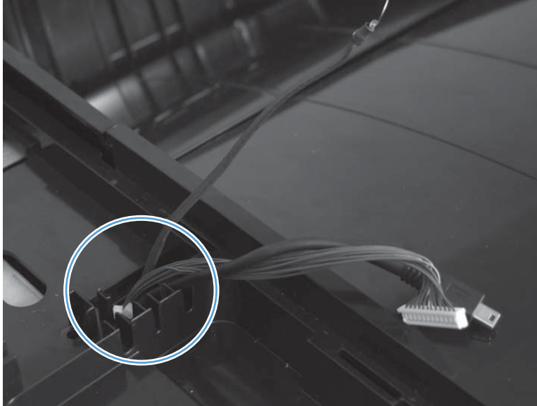
Figure 1-151 Reinstall the right top cover (M806; 2 of 3)
