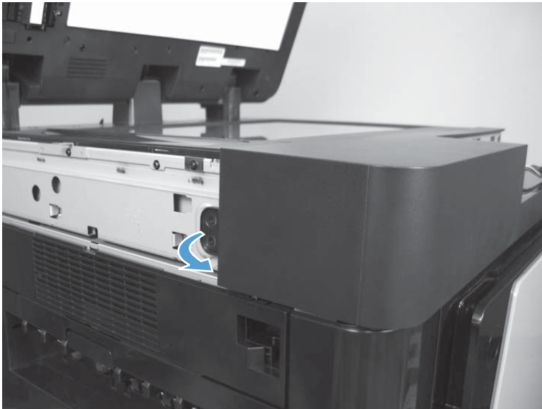
Figure 1-122 Remove the scanner front cover (M830; 5 of 7)
