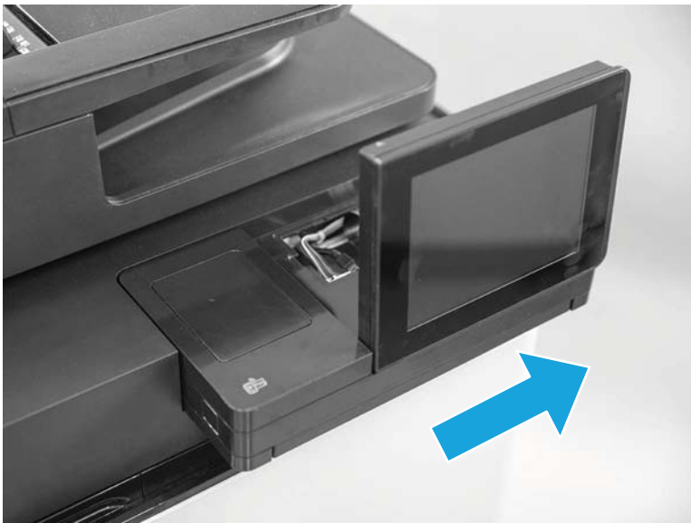
Figure 1-65 Remove the control-panel assembly (M830; 6 of 7)
