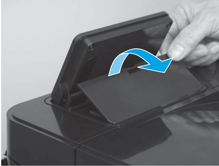
Figure 1-51 Remove the control-panel assembly (M806; 3 of 10)
