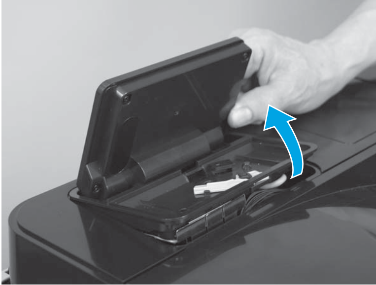
Figure 1-53 Remove the control-panel assembly (M806; 5 of 10)
