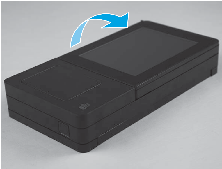
Figure 1-80 Reinstall the keyboard assembly (M830; 4 of 7)
