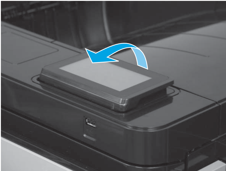
Figure 1-49 Remove the control-panel assembly (M806; 1 of 10)
