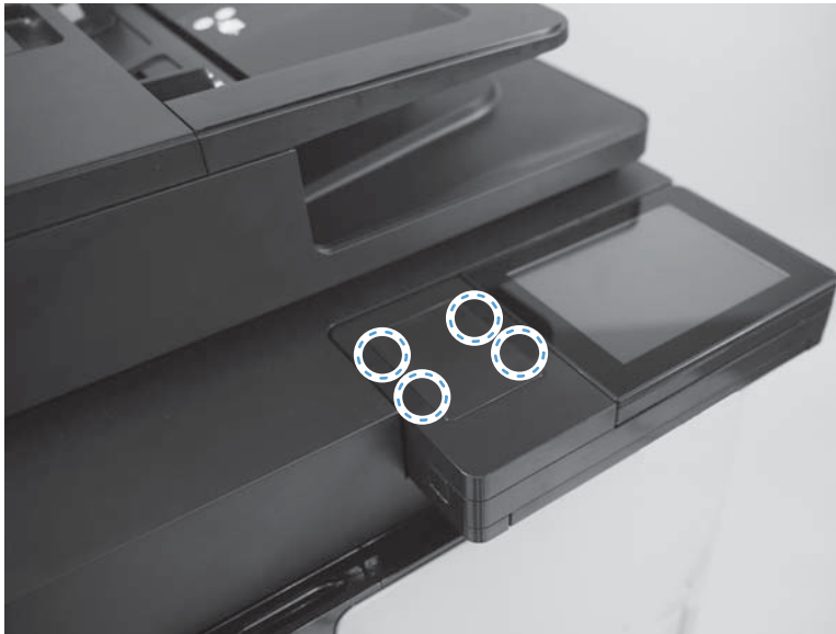
Figure 1-135 Remove the HIP cover (M830; 1 of 3)
