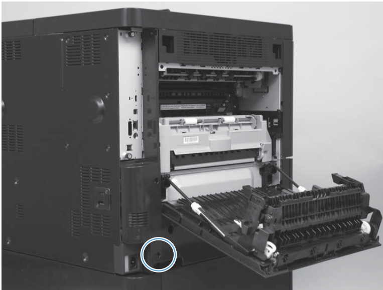
Figure 1-165 Remove the rear cover (1 of 3)
