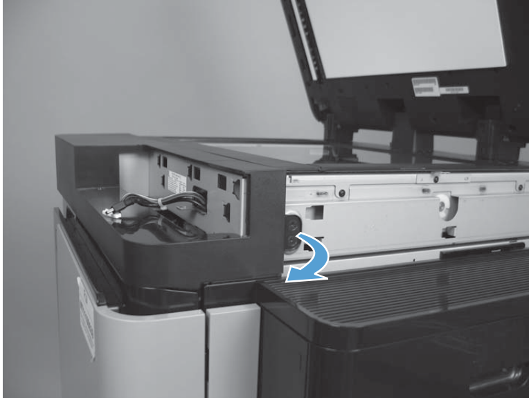
Figure 1-123 Remove the scanner front cover (M830; 6 of 7)
