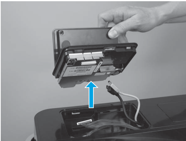
Figure 1-58 Remove the control-panel assembly (M806; 10 of 10)
