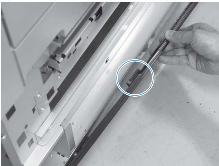
Figure 1-430 Remove the HCI lower right cover (2 of 3)
