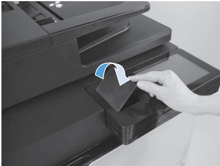
Figure 1-139 Reinstall the HIP cover (M830; 2 of 2)
