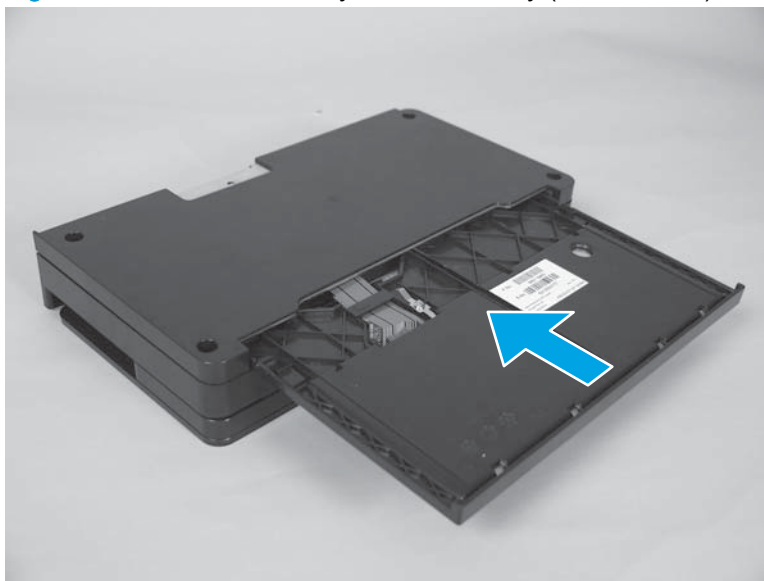
Figure 1-78 Reinstall the keyboard assembly (M830; 2 of 7)
