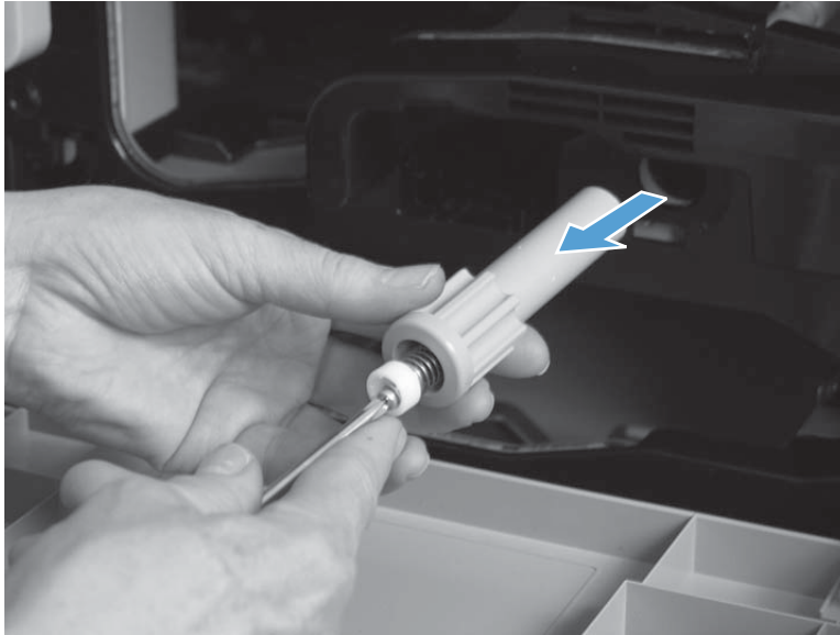
Figure 1-230 Remove the registration-jam-removal knob (3 of 3)
