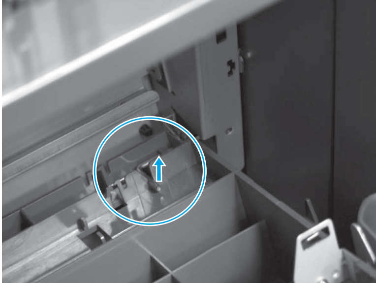
Figure 1-813 Remove the saddle paper delivery assembly (6 of 8)
