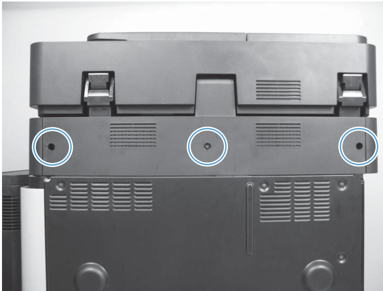
Figure 1-109 Remove the scanner back cover (M830; 1 of 2)
