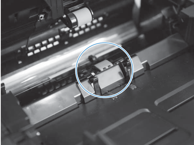
Figure 1-96 Reinstall the document-feeder separation pad (M830; 5 of 5)
