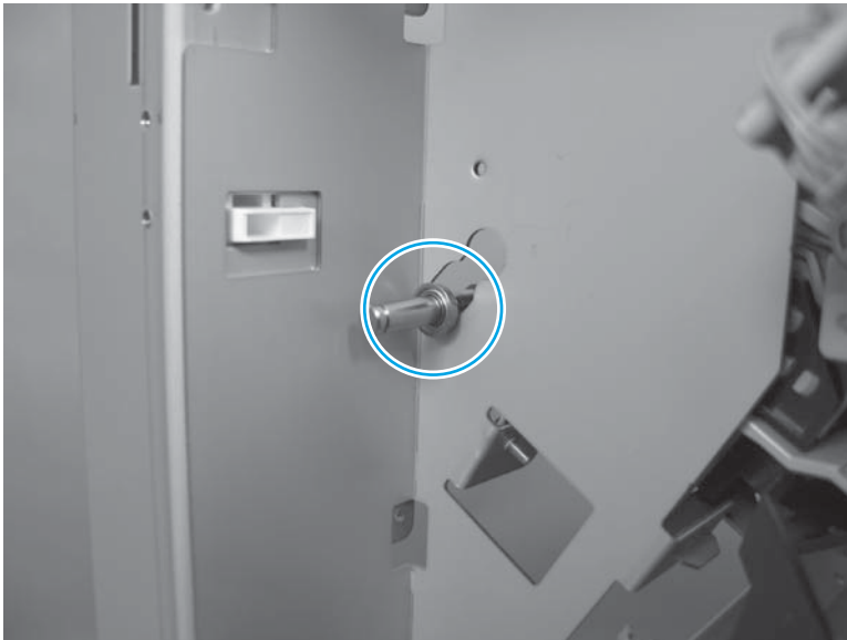
Figure 1-643 Remove the operation tray assembly (4 of 11)
