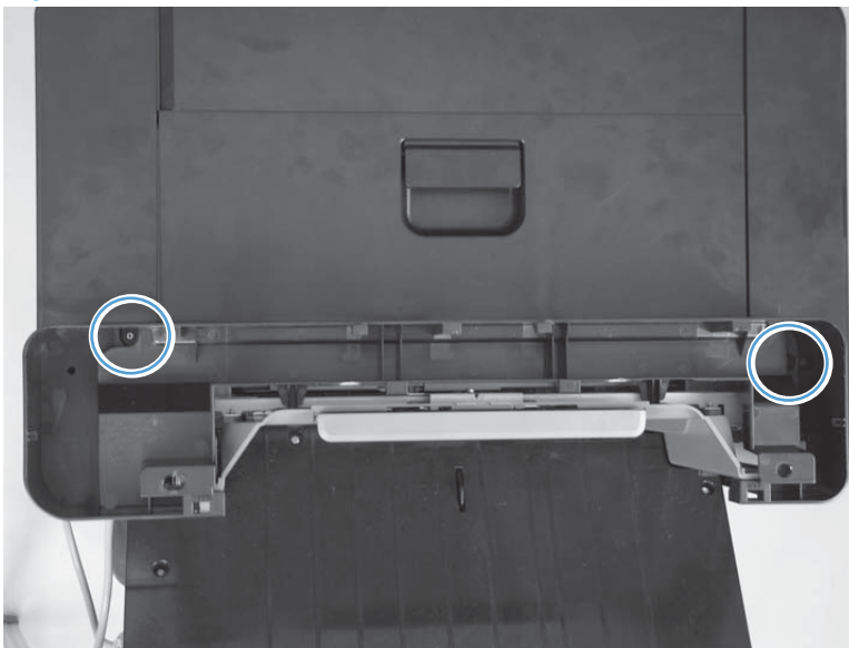
Figure 1-491 Remove the lower stepped cover assembly (1 of 5)
