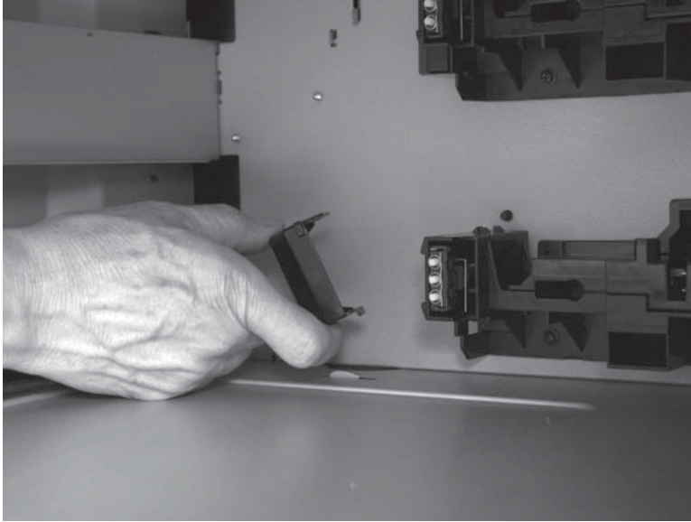
Figure 1-261 Remove the auto-close assembly (2 of 5)
