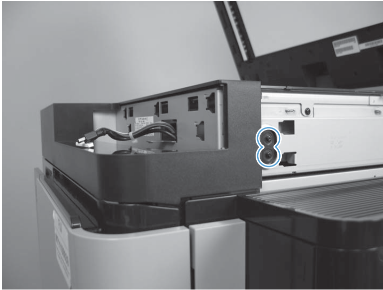
Figure 1-119 Remove the scanner front cover (M830; 2 of 7)
