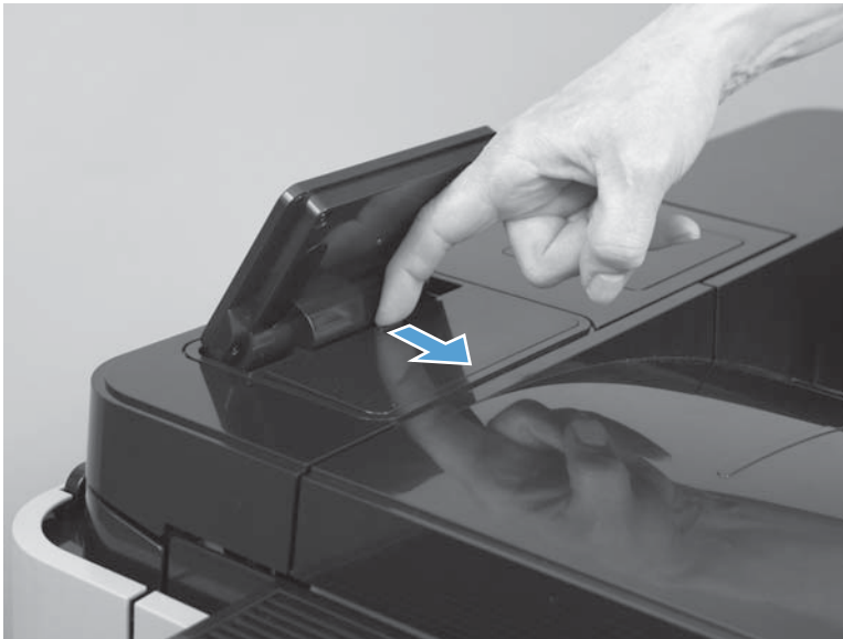
Figure 1-50 Remove the control-panel assembly (M806; 2 of 10)
