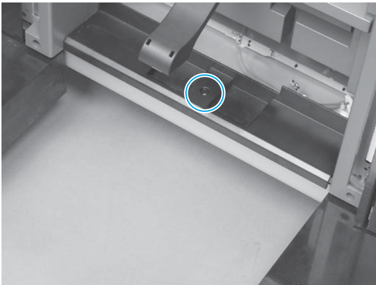
Figure 1-808 Remove the saddle paper delivery assembly (1 of 8)
