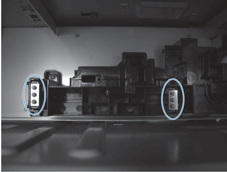
Figure 2-21 Tray 4 paper size switches
