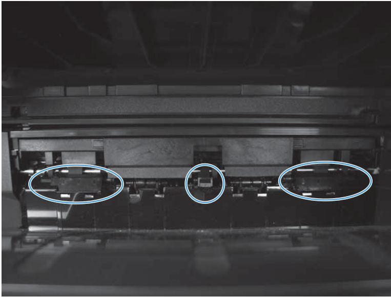
Figure 2-18 Output bin full sensor
