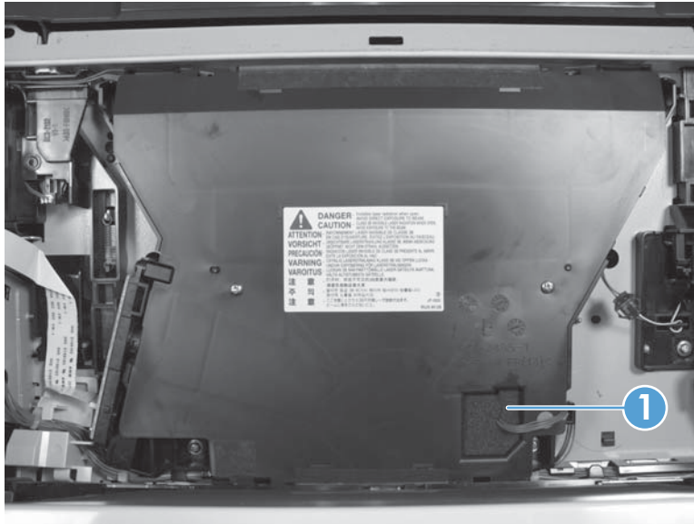
Figure 1-67 Remove the laser scanner (1 of 3)
