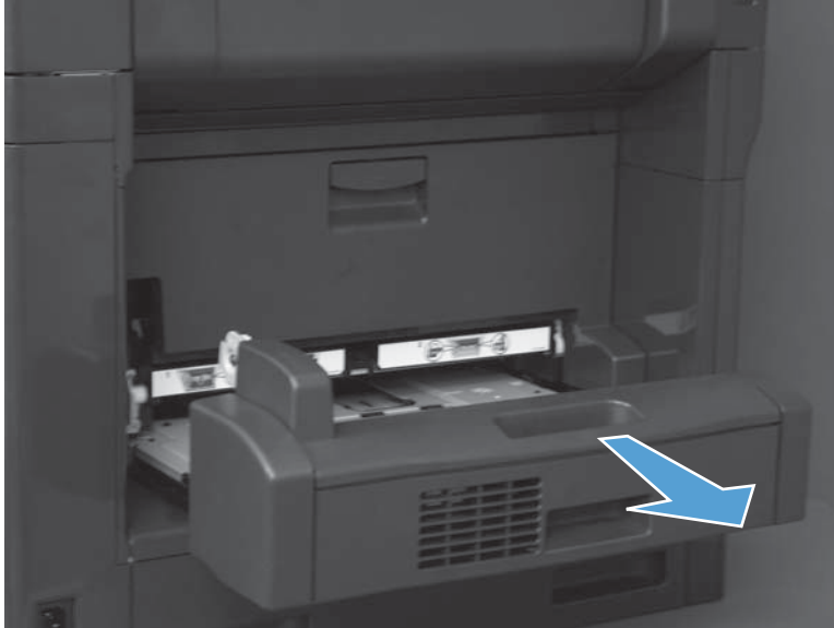
Figure 1-43 Remove the duplexer (1 of 2)
