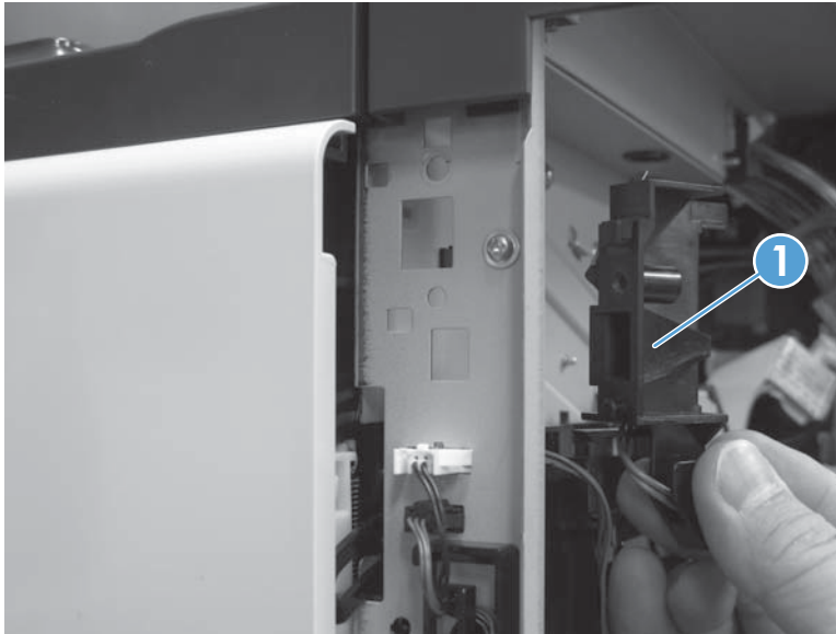
Figure 1-112 Remove the cartridge door interlock switch (3 of 4)
