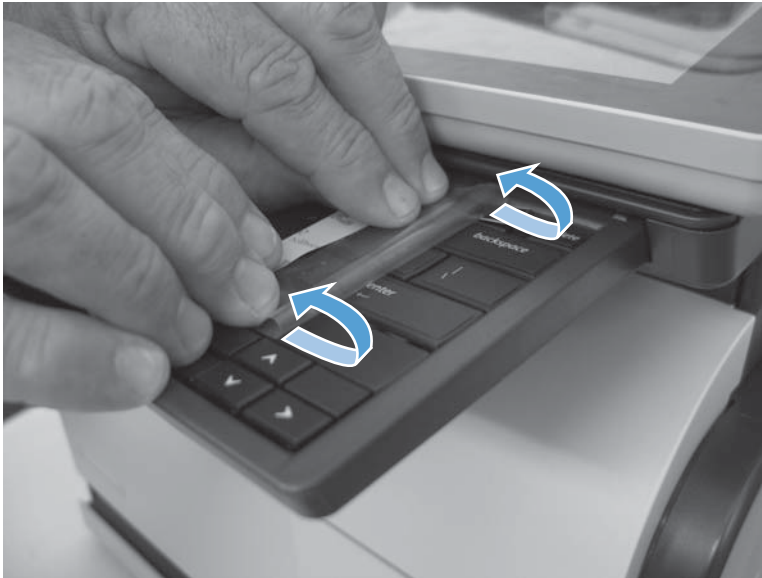
Figure 1-68 Install a keyboard overlay (6 of 6)
