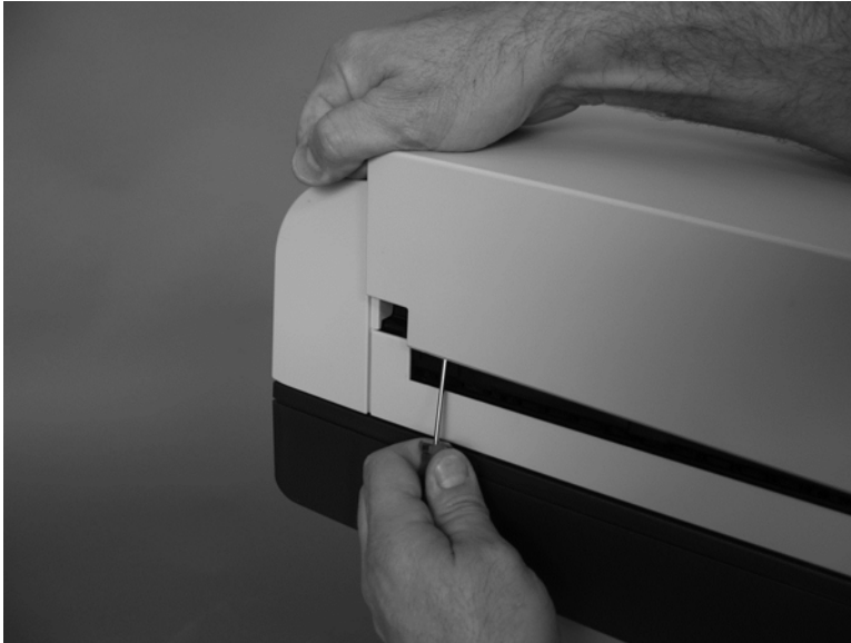
Figure 1-170 Remove the document feeder jam-access cover (5 of 5)
