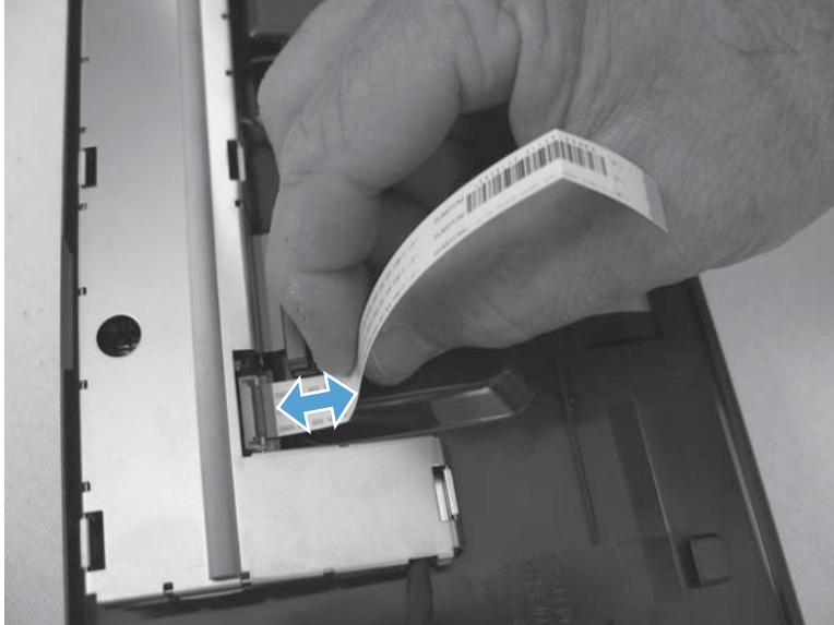
Figure 1-55 Reinstall the control-panel assembly to keyboard FFC (4 of 4)
