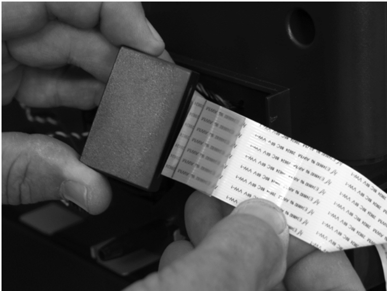
Figure 1-215 Separate the ISA assemblies (525c model; 4 of 7)
