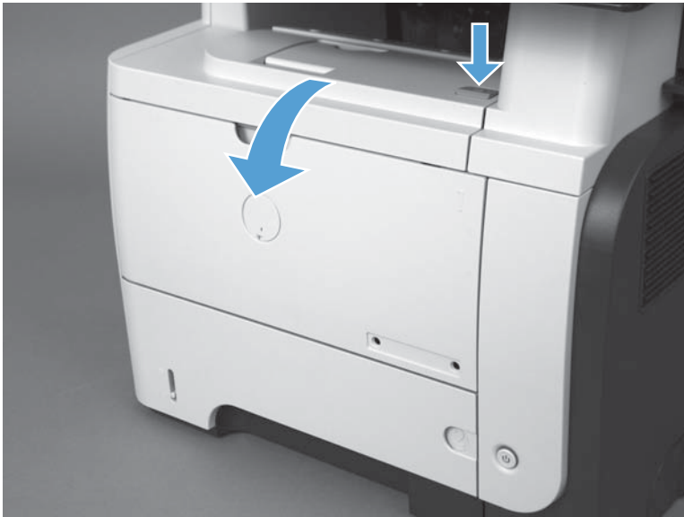
Figure 1-7 Remove the toner cartridge (1 of 2)
