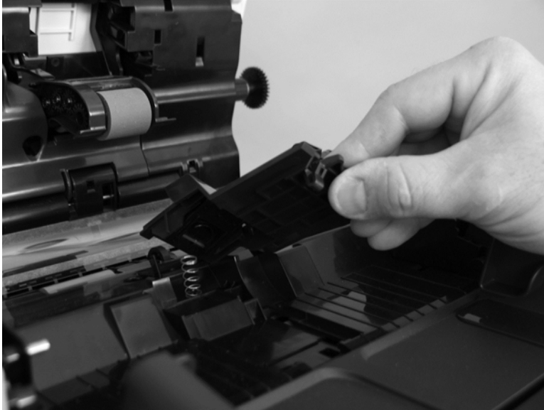
Figure 1-90 Remove the document feeder separation pad (5 of 5)
