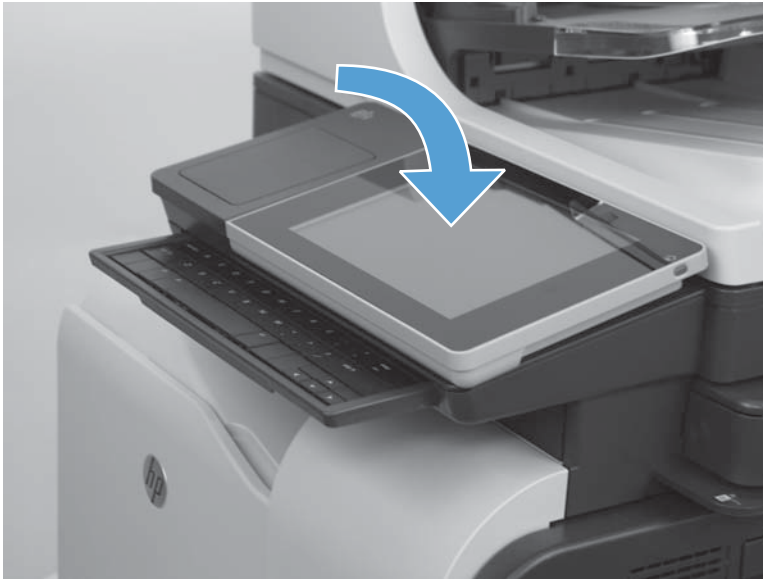
Figure 1-46 Reinstall the control-panel assembly (12 of 13)
