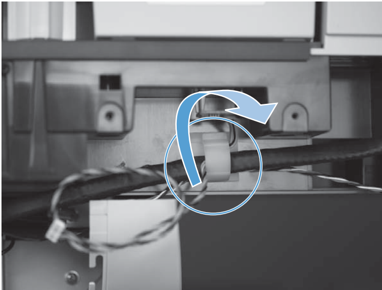
Figure 1-179 Remove the scanner memory PCA (4 of 4)
