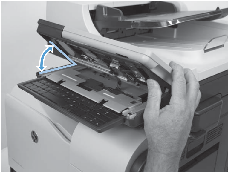
Figure 1-36 Reinstall the control-panel assembly (2 of 13)
