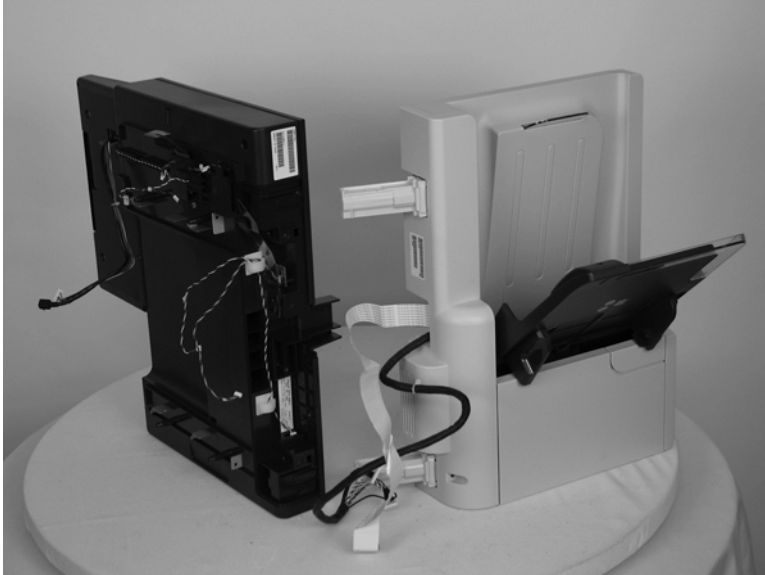
Figure 1-218 Separate the ISA assemblies (525c model; 7 of 7)
