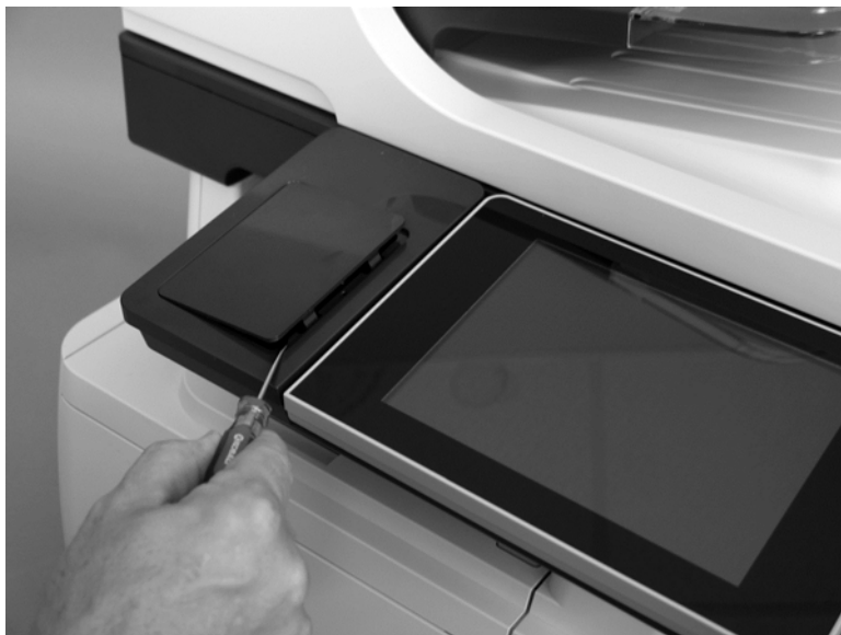
Figure 1-10 Remove the control-panel HIP cover
