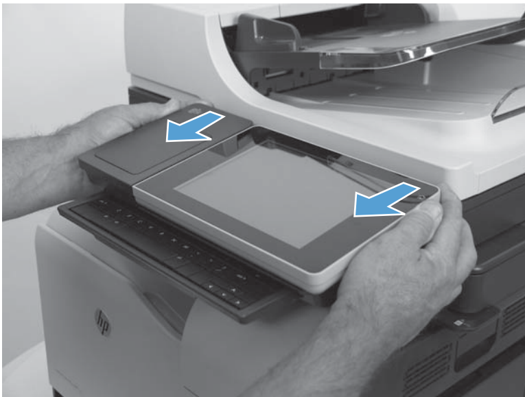
Figure 1-28 Remove the control-panel assembly (7 of 13)
