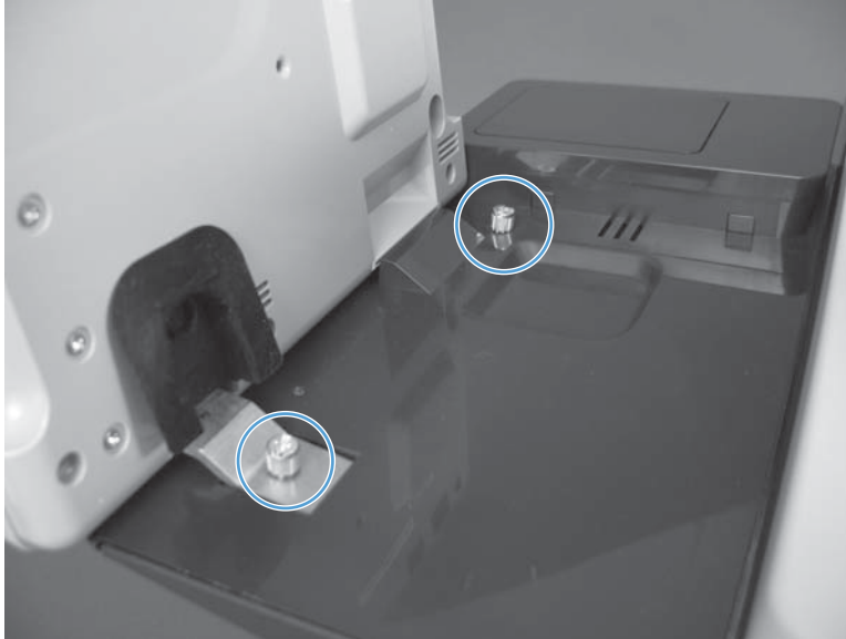
Figure 1-14 Remove the control-panel assembly (3 of 5)
