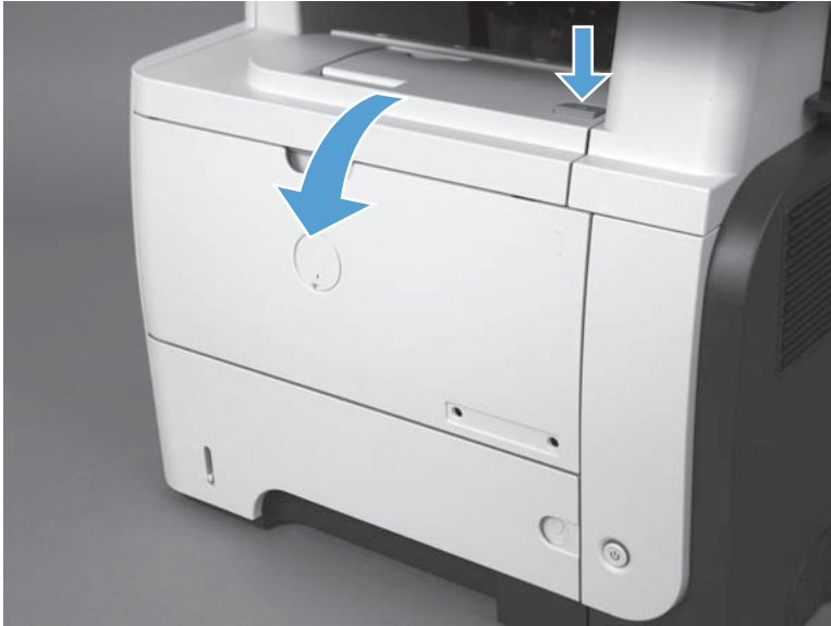
Figure 1-224 Remove the Tray 1 separation pad (1 of 2)
