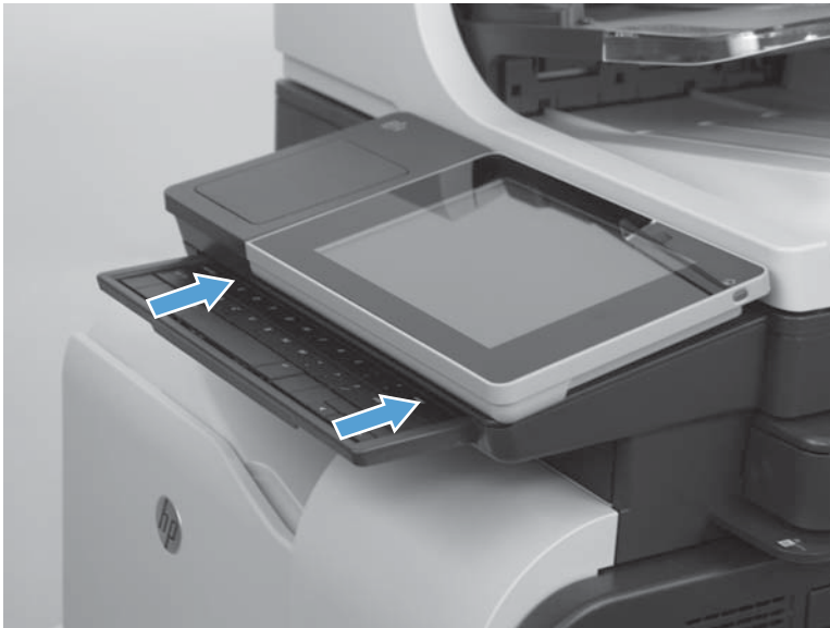
Figure 1-47 Remove the control-panel assembly (13 of 13)
