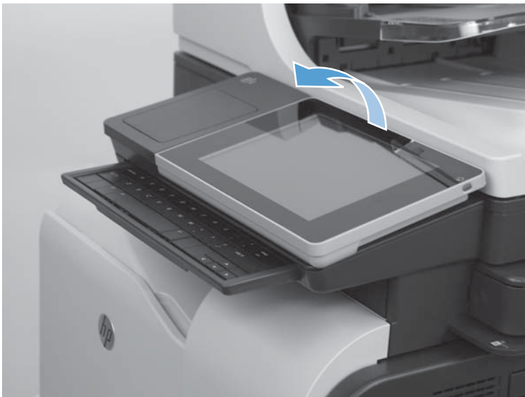
Figure 1-24 Remove the control-panel assembly (3 of 13)
