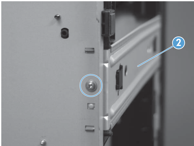
Figure 1-301 Remove the Tray 2 paper pickup assembly (2 of 10)
