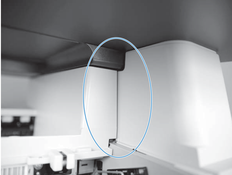
Figure 1-151 Reinstall the right cover assembly: incorrect alignment
