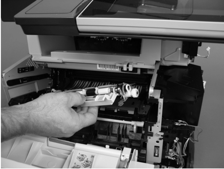
Figure 1-261 Removing the registration roller assembly (3 of 3)
