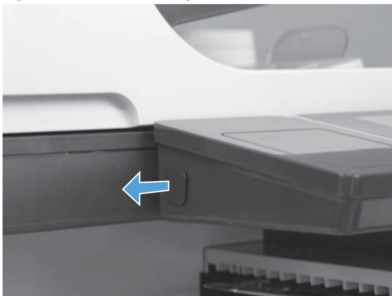
Figure 1-11 Remove control-panel USB cover
