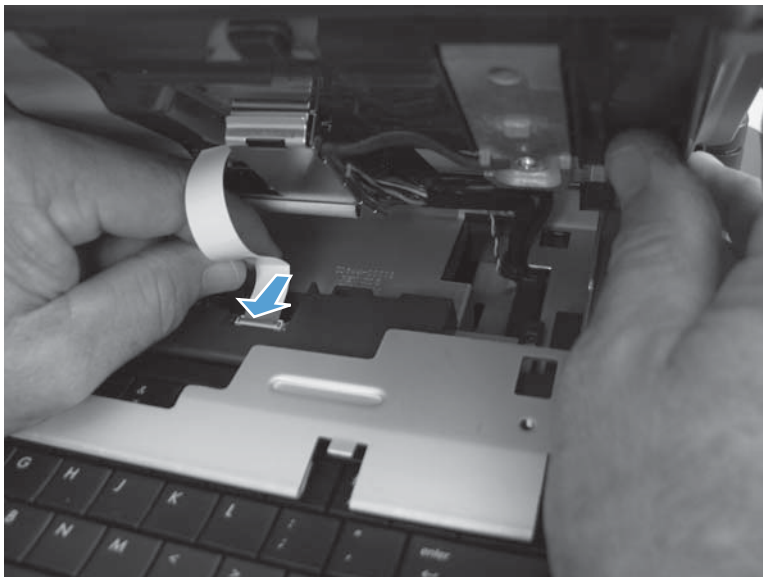
Figure 1-37 Reinstall the control-panel assembly (3 of 13)
