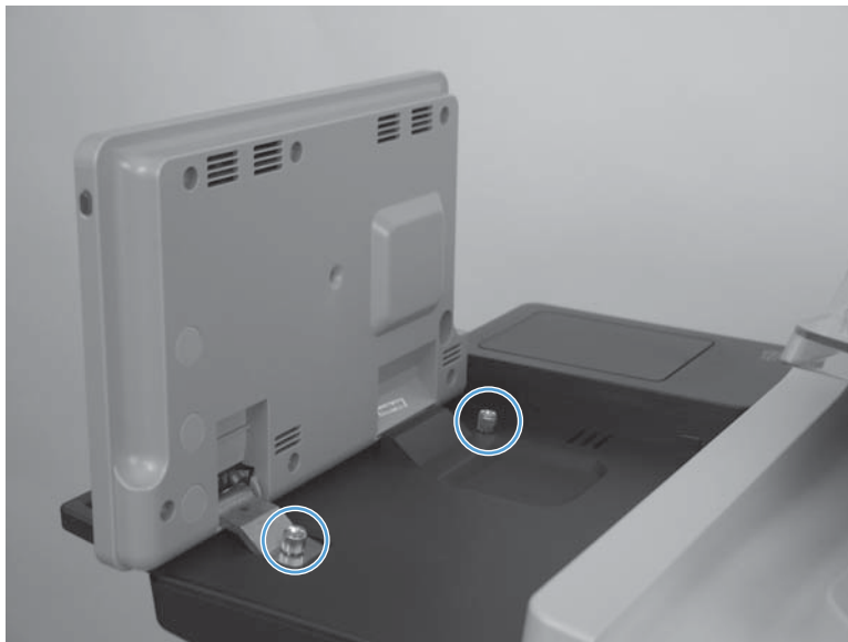
Figure 1-26 Remove the control-panel assembly (5 of 13)
