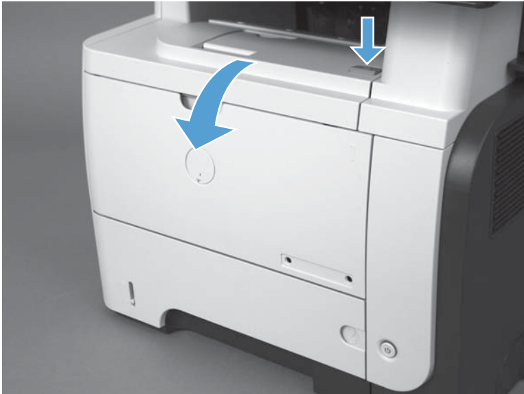
Figure 1-222 Remove the Tray 1 pickup roller (1 of 2)
