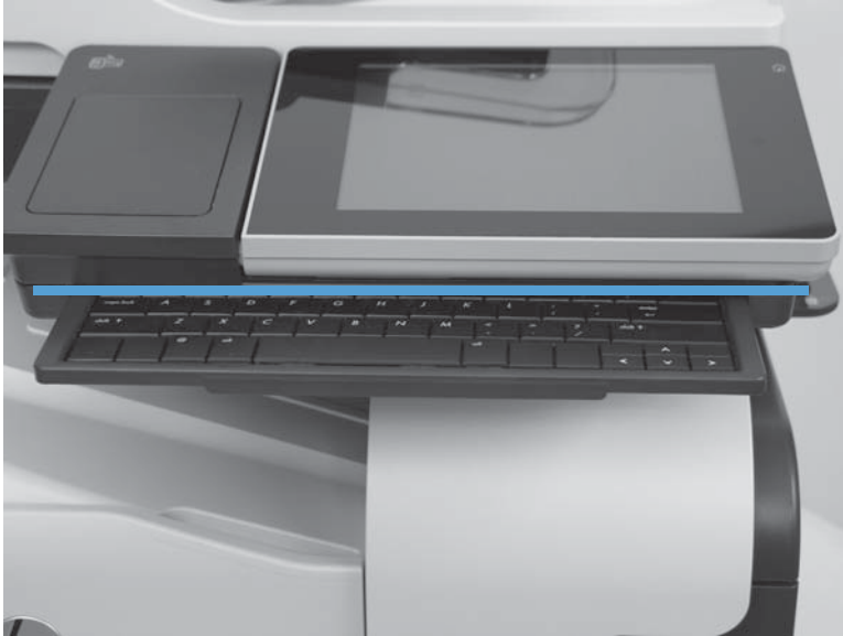
Figure 1-23 Remove the control-panel assembly (2 of 13)
