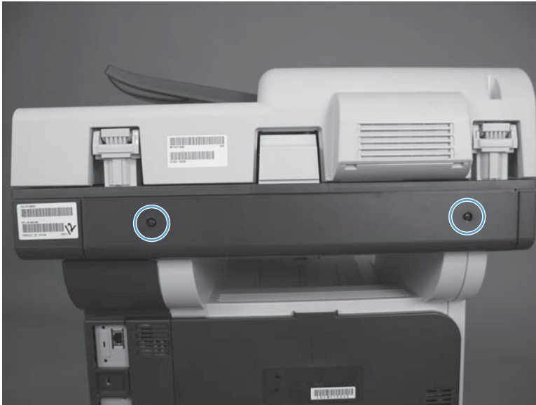
Figure 1-137 Remove the Rear scanner cover
