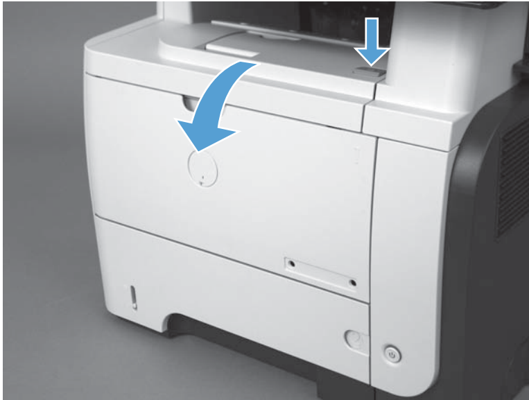
Figure 1-247 Remove the transfer roller (1 of 3)
