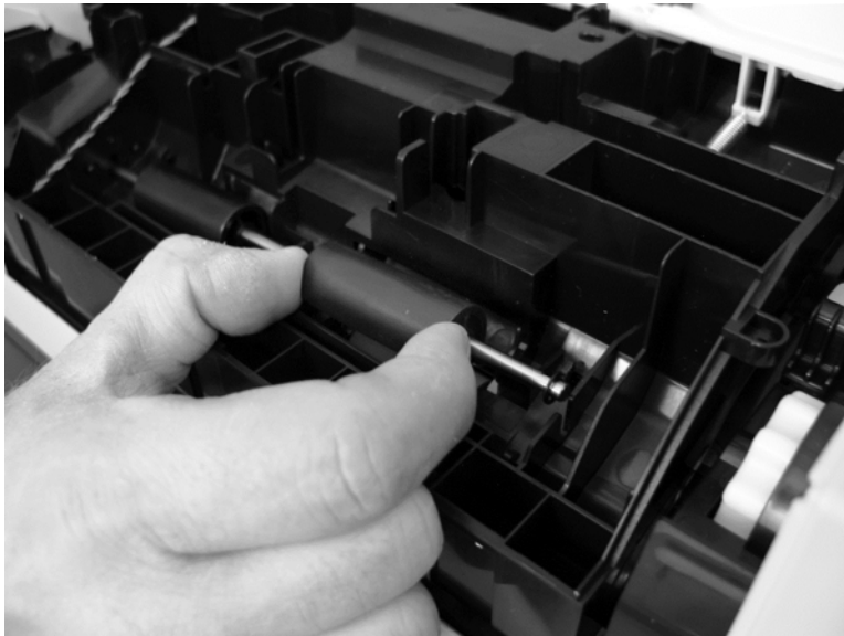
Figure 1-172 Remove the document feeder roller cover (2 of 4)
