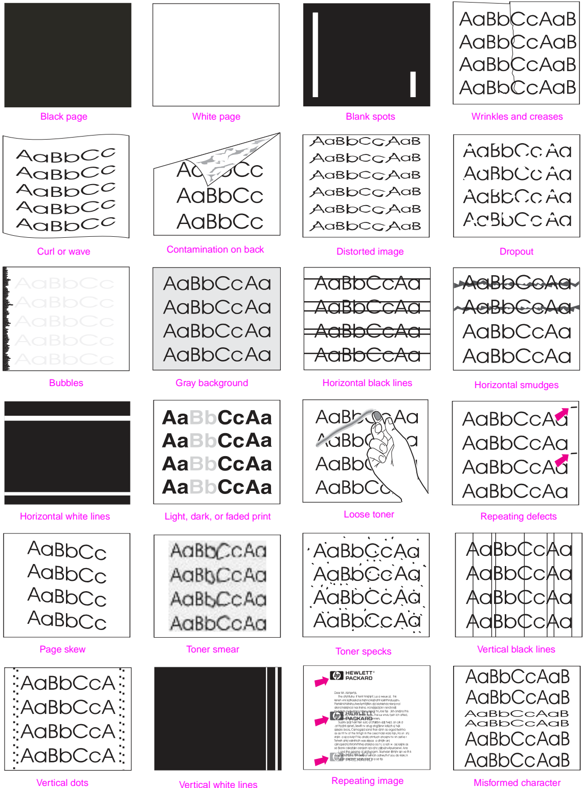
Figure 129. Image defect examples
