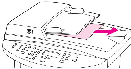
Figure 6-7. Clearing output bin jams (HP LaserJet 3020 and 3030)
