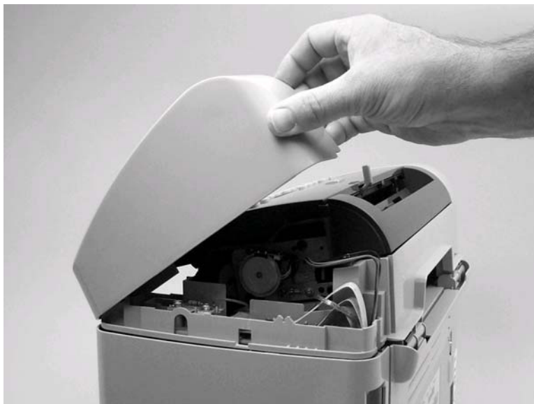
Figure 5-12. Remove the scanner side covers (3 of 3)
