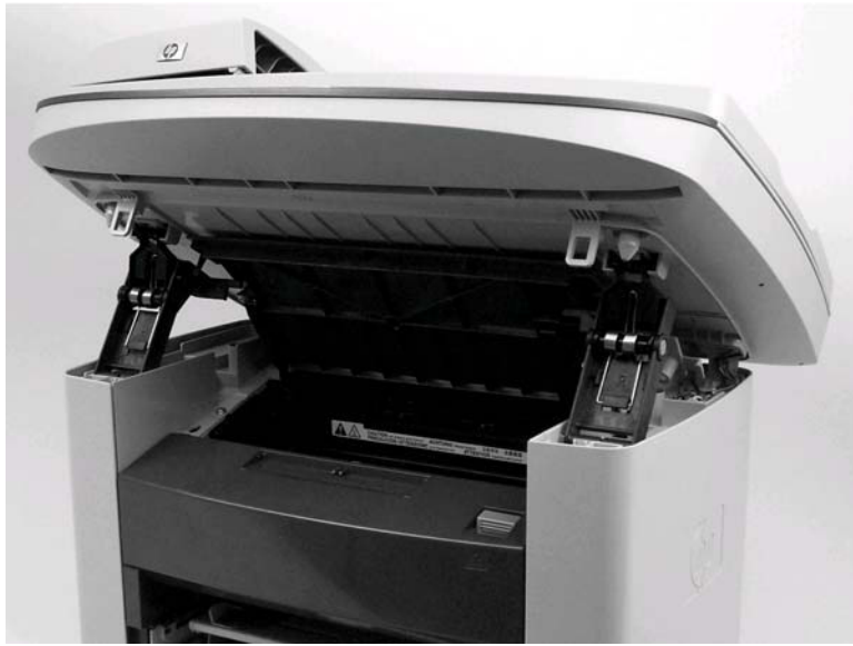
Figure 5-91. Remove the print cartridge (1 of 2)
