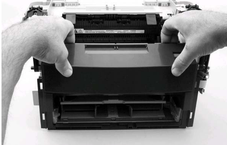
Figure 5-115. Remove the front cover (3 of 3)
