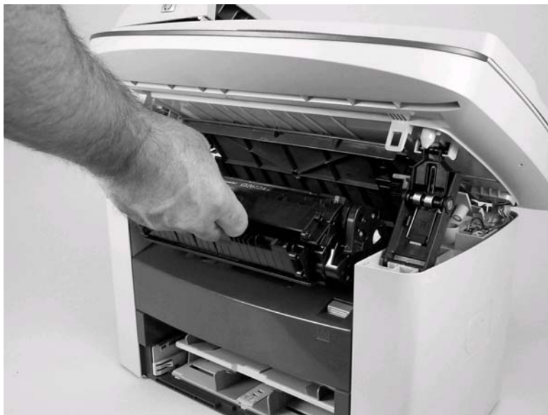
Figure 5-92. Remove the print cartridge (2 of 2)
