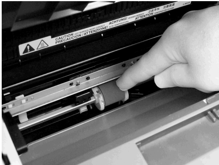
Figure 5-97. Remove the printer pickup roller (5 of 5)
