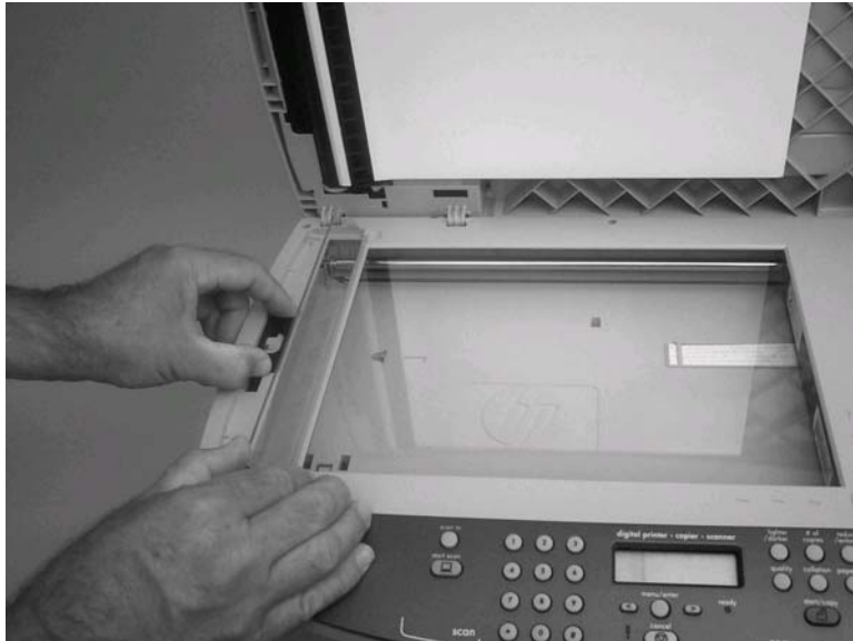
Figure 5-73. Remove the ADF scanner glass (3 of 3)
