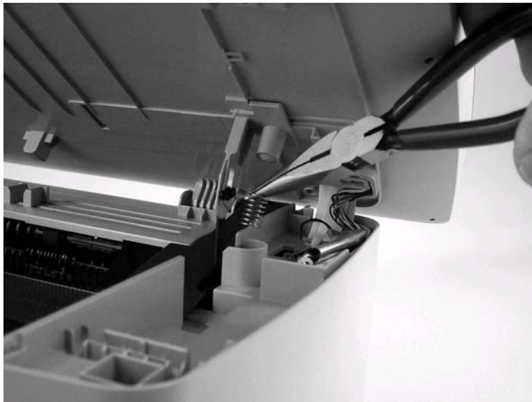
Figure 5-62. Remove the link assemblies and scanner support frame springs (4 of 4)
