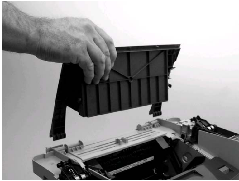
Figure 5-109. Remove the print-cartridge door (2 of 2)
