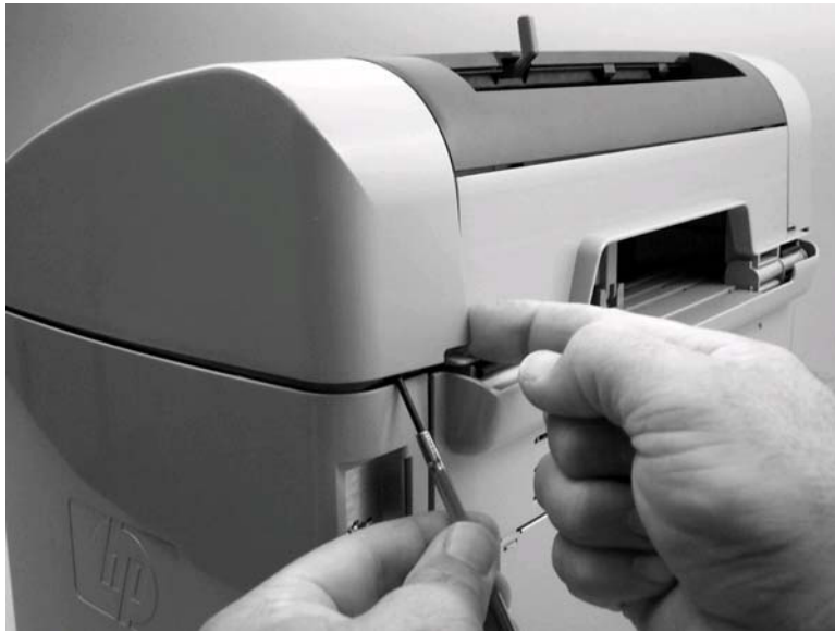
Figure 5-10. Remove the scanner side covers (1 of 3)
