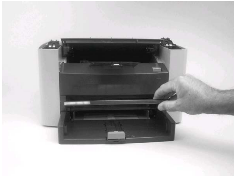
Figure 5-98. Remove the media input tray (1 of 3)
