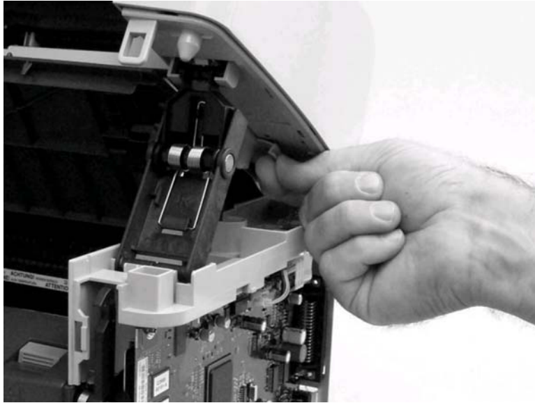
Figure 5-32. Remove the scanner assembly (9 of 15)
