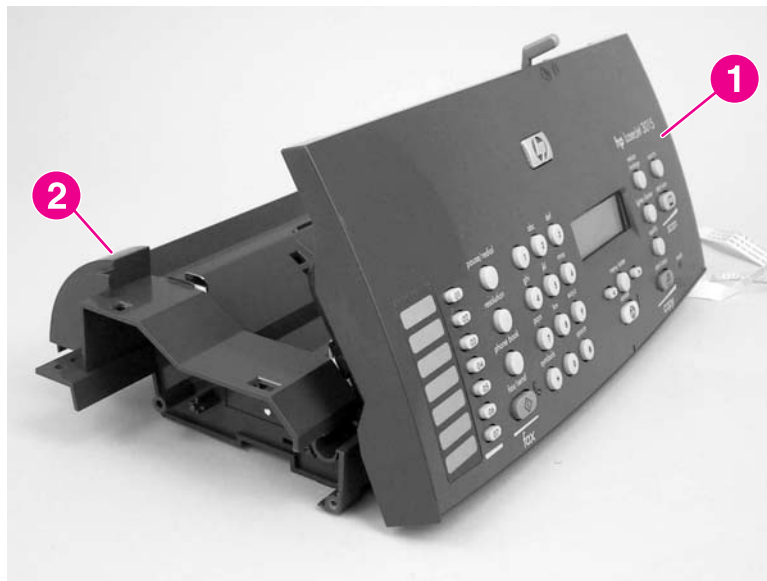
Figure 5-45. Remove the top-cover assembly (1 of 2)
