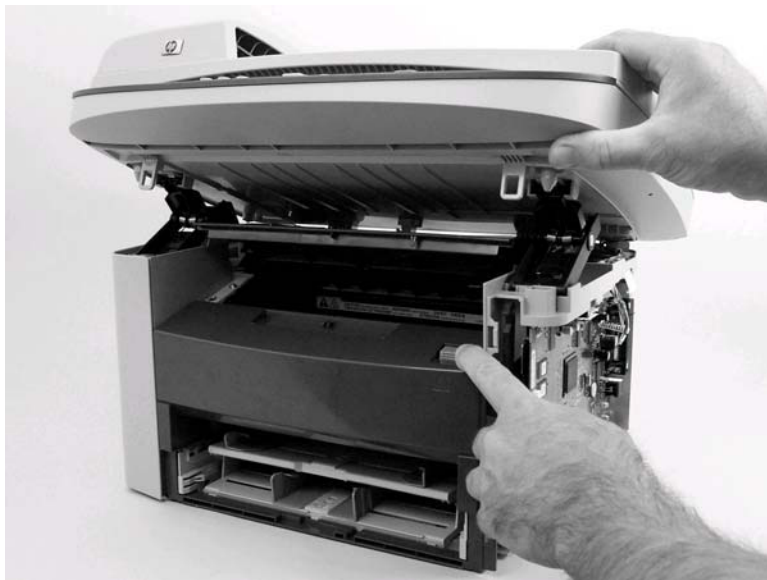
Figure 5-80. Remove the scanner assembly (6 of 13)
