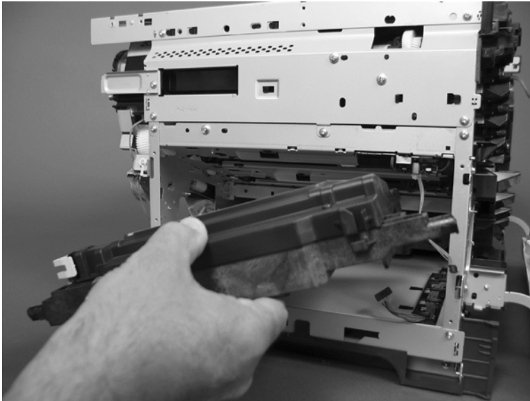
Figure 1-215 Remove the laser/scanner assembly (Y/M) (12 of 12)
