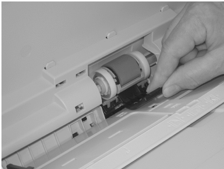
Figure 1-38 Remove the Tray 1 separation pad (4 of 4)
