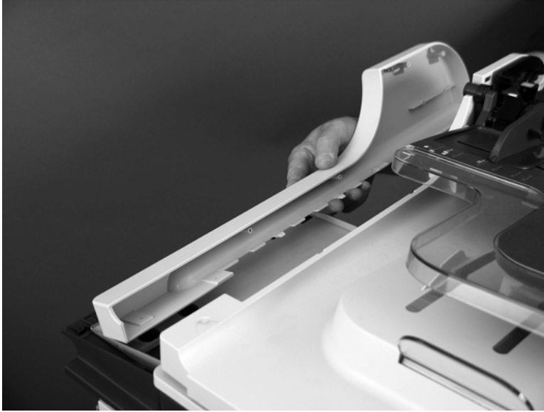
Figure 1-62 Remove the document feeder front cover (8 of 8)
