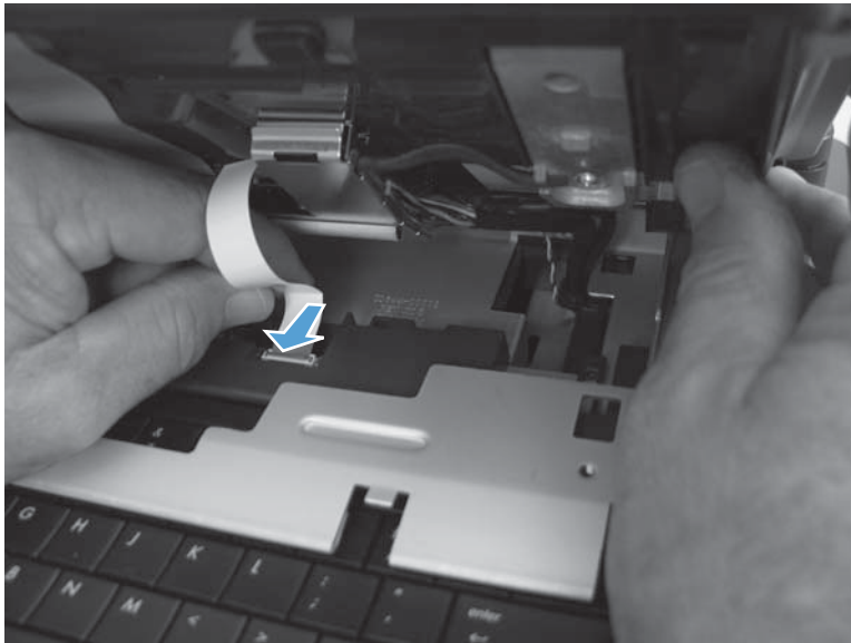
Figure 1-81 Reinstall the control-panel assembly (3 of 13)
