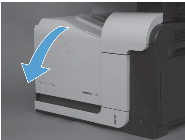
Figure 1-6 Remove the toner cartridge (1 of 2)
