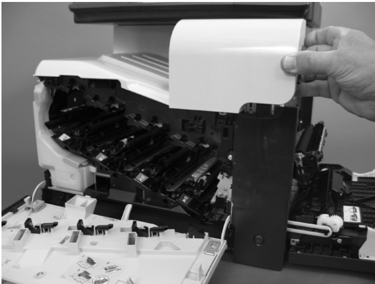
Figure 1-125 Remove the front-upper cover (4 of 4)
