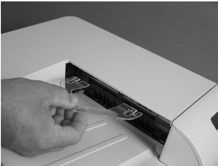
Figure 1-10 Remove the duplex-reverse guide (2 of 2)
