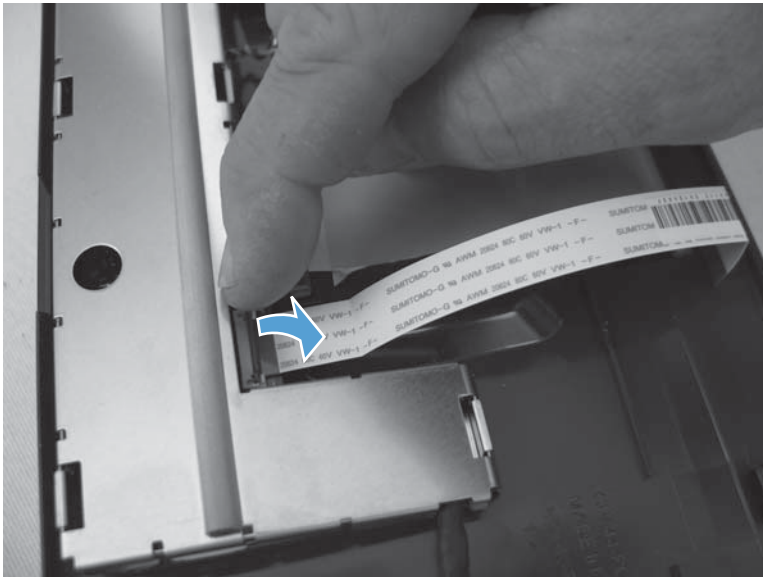
Figure 1-98 Reinstall the control-panel assembly to keyboard FFC (3 of 4)
