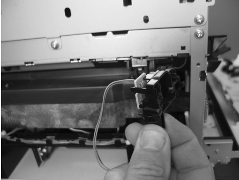
Figure 1-240 Remove the toner-collection sensor (4 of 4)
