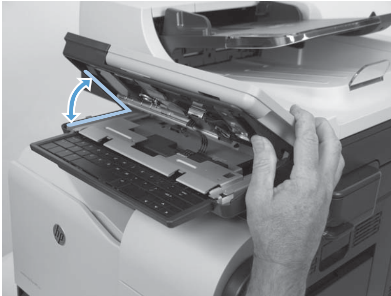
Figure 1-80 Reinstall the control-panel assembly (2 of 13)
