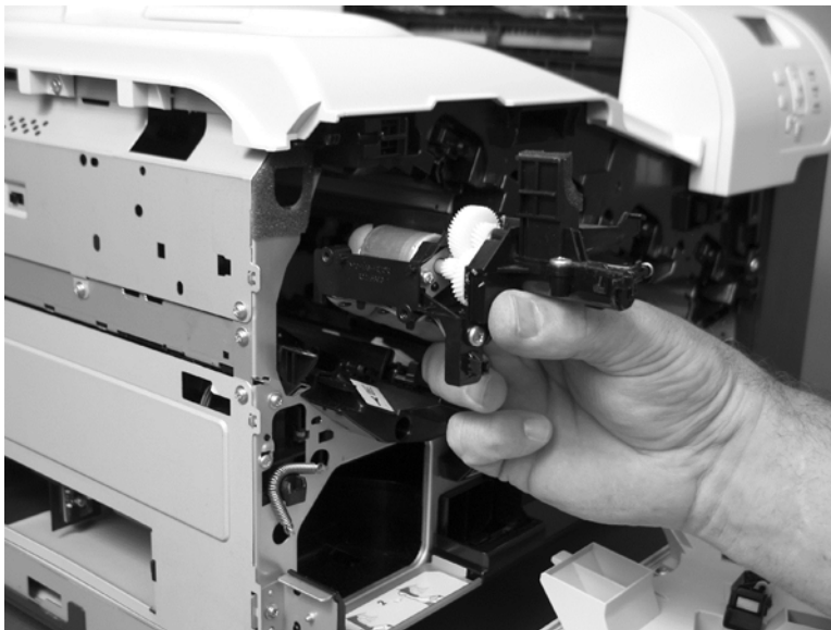
Figure 1-247 Remove the residual-toner-feed motor (7 of 7)
