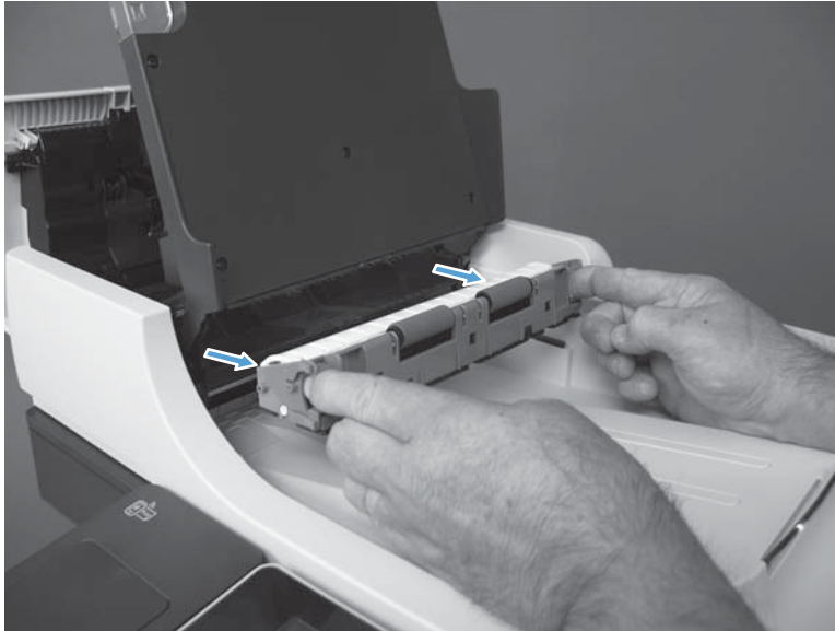
Figure 1-115 Remove the back-side background selector assembly (3 of 3)
