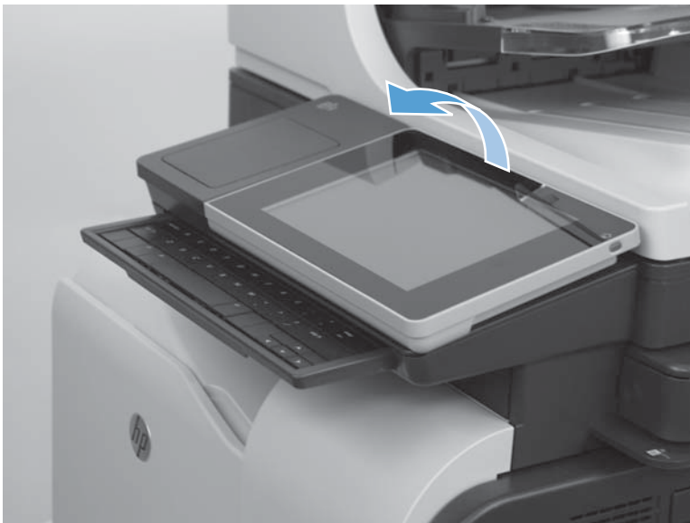
Figure 1-68 Remove the control-panel assembly (3 of 13)
