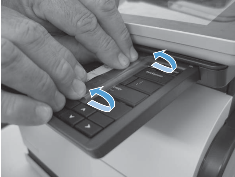
Figure 1-112 Install a keyboard overlay (6 of 6)
