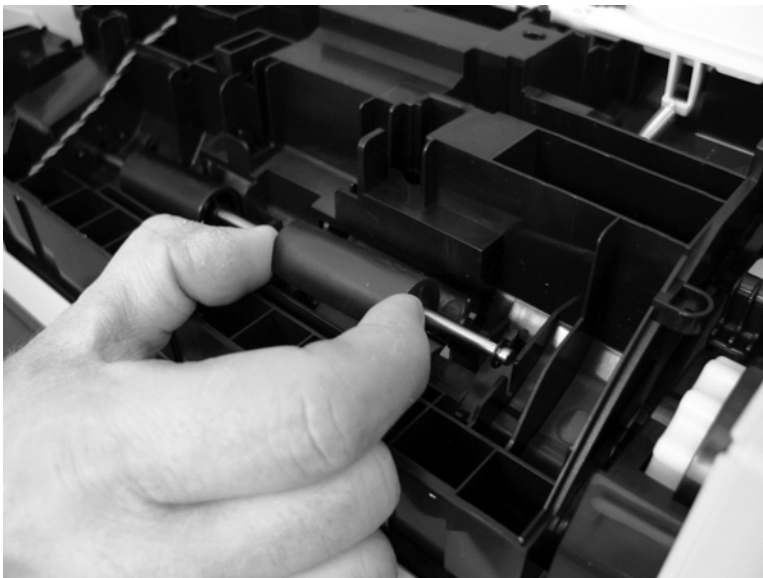
Figure 1-185 Remove the document feeder roller cover (2 of 4)
