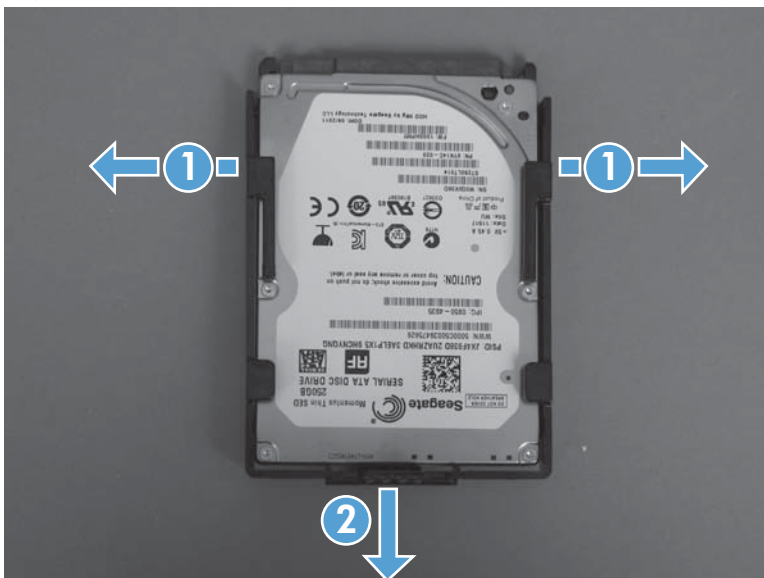
Figure 1-20 Remove the HDD (3 of 3)
