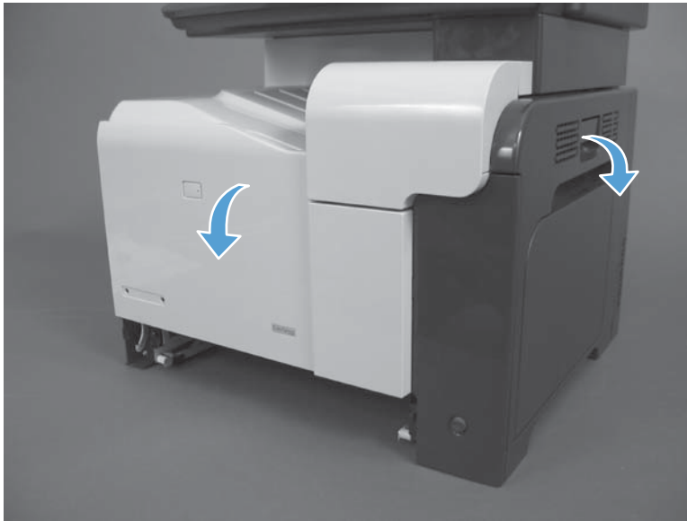
Figure 1-122 Remove the front-upper cover (1 of 4)
