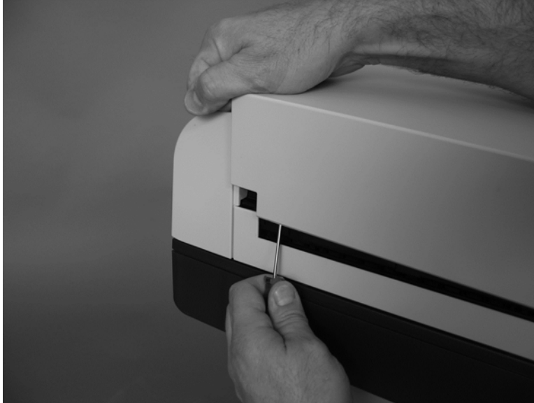
Figure 1-183 Remove the document feeder jam-access cover (5 of 5)
