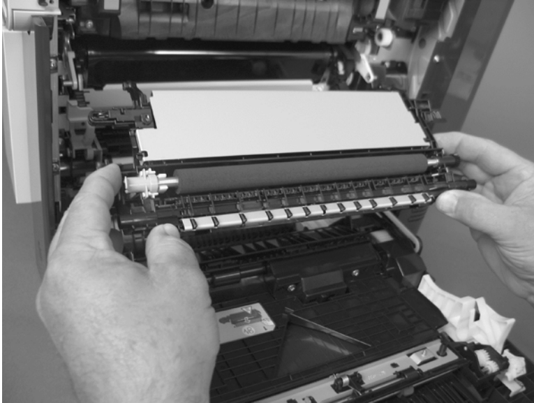
Figure 1-251 Remove the secondary transfer assembly (3 of 3)
