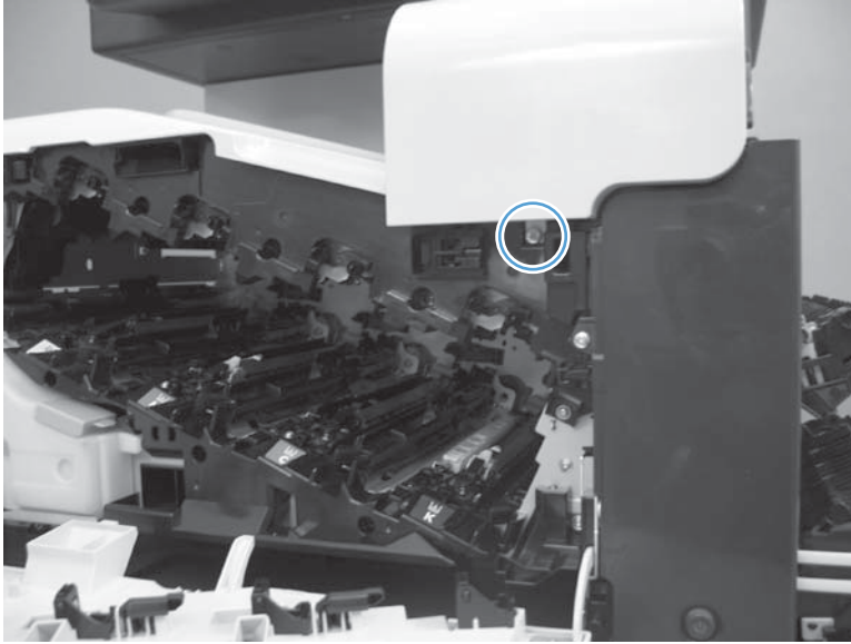
Figure 1-124 Remove the front-upper cover (3 of 4)
