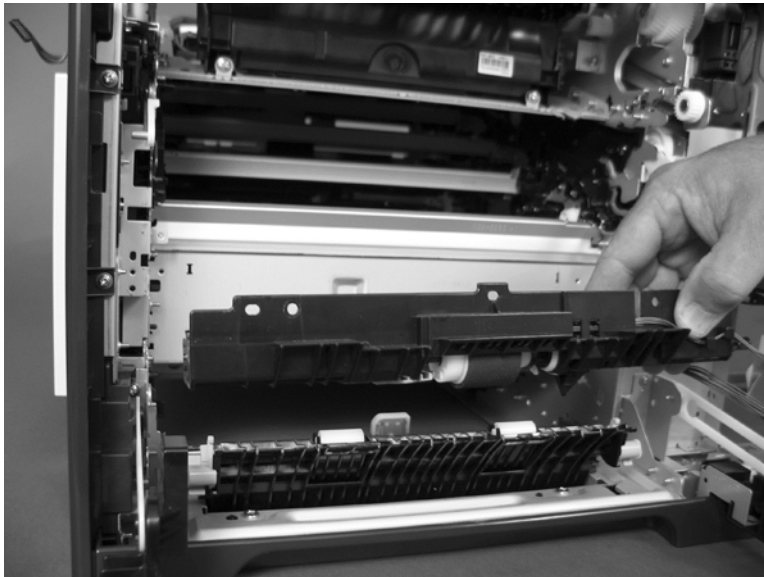
Figure 1-300 Remove the tray-pickup assembly (3 of 3)
