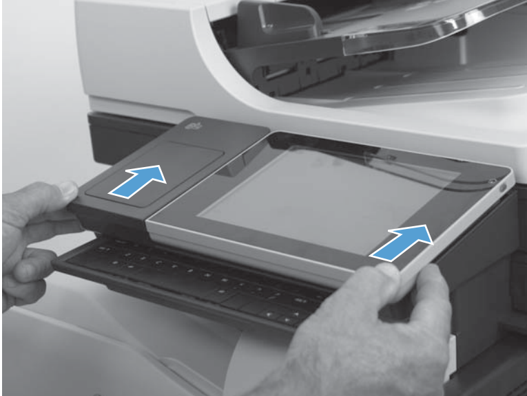
Figure 1-86 Reinstall the control-panel assembly (8 of 13)
