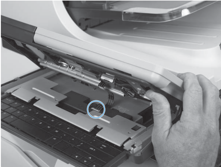
Figure 1-74 Remove the control-panel assembly (9 of 13)
