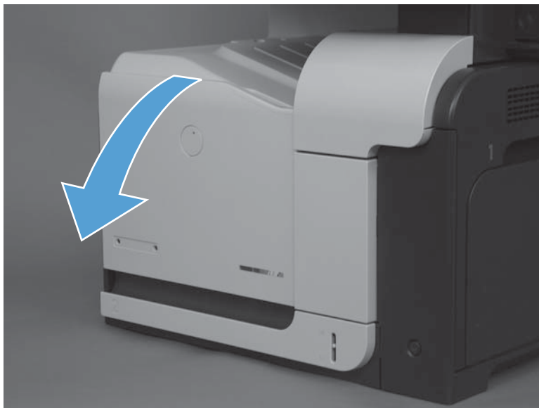
Figure 1-43 Remove the front-door assembly (1 of 2)
