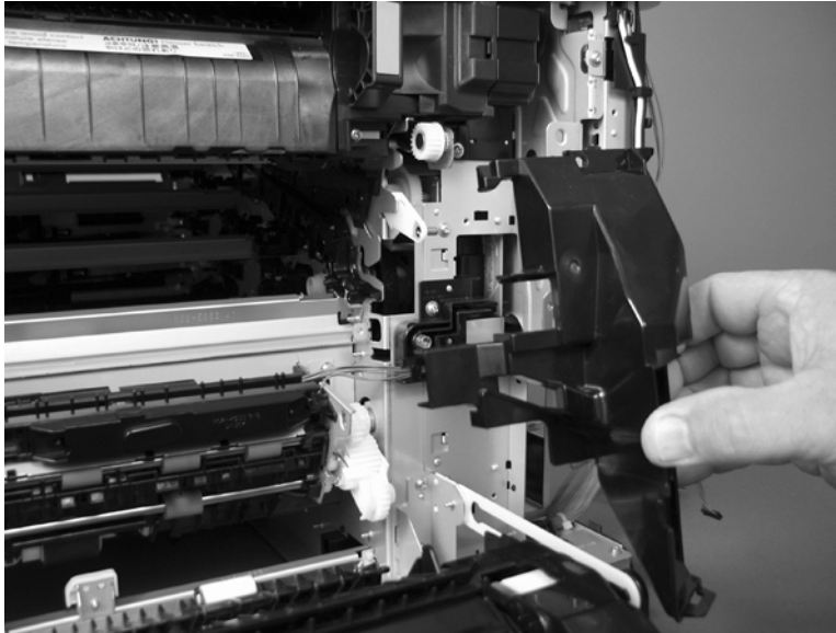
Figure 1-268 Remove the registration assembly (2 of 8)
