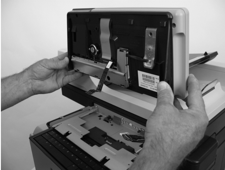
Figure 1-78 Remove the control-panel assembly (13 of 13)
