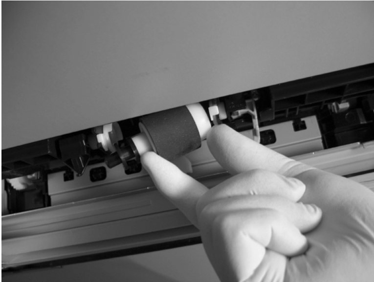
Figure 1-30 Remove the pickup roller (Tray 2; 3 of 4)
