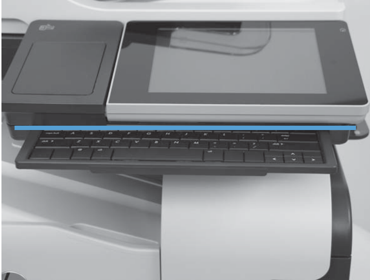
Figure 1-67 Remove the control-panel assembly (2 of 13)
