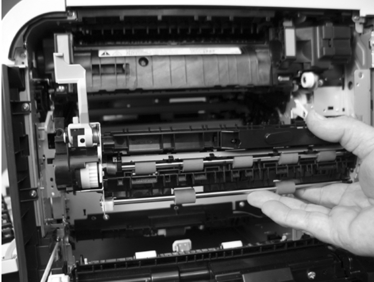
Figure 1-274 Remove the registration assembly (8 of 8)
