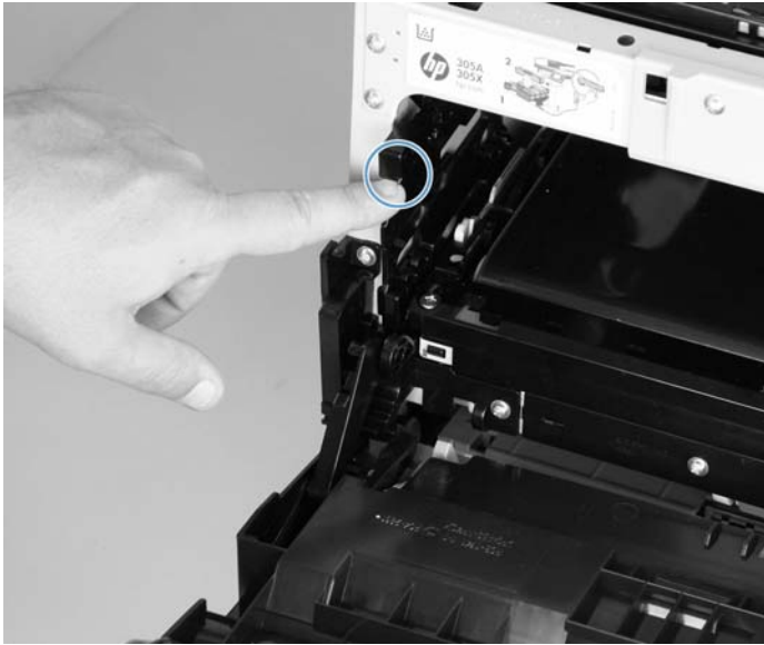
Figure 1-68 Remove the front-door assembly (8 of 10)
