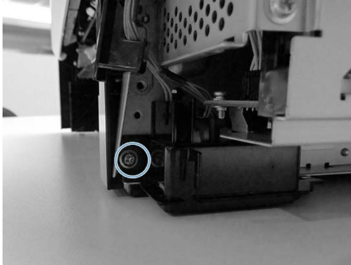
Figure 1-140 Remove the screw holding the tray 3 harness in place
