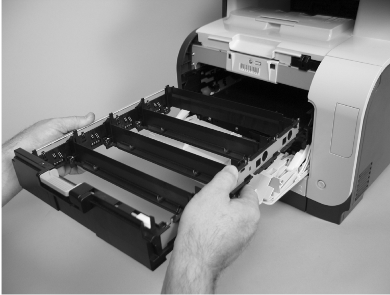
Figure 1-25 Remove the print-cartridge drawer (3 of 3)
