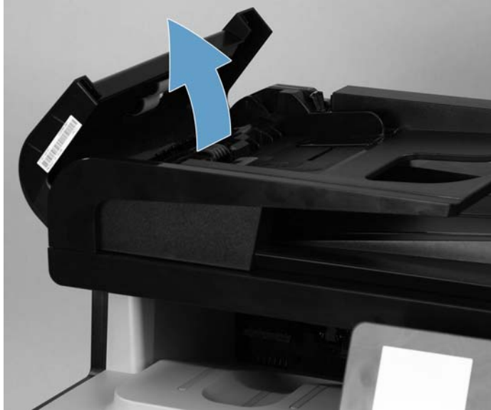
Figure 1-8 Open the jam-access cover
