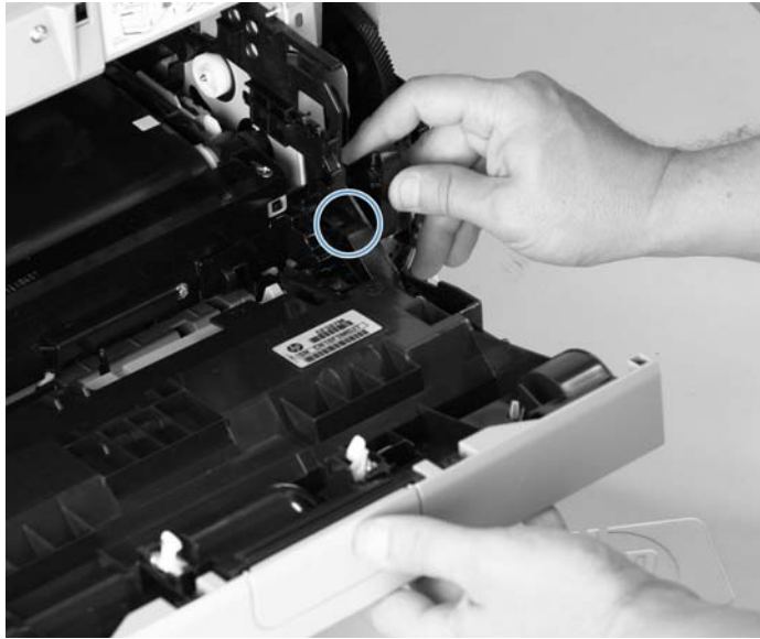
Figure 1-66 Remove the front-door assembly (6 of 10)
