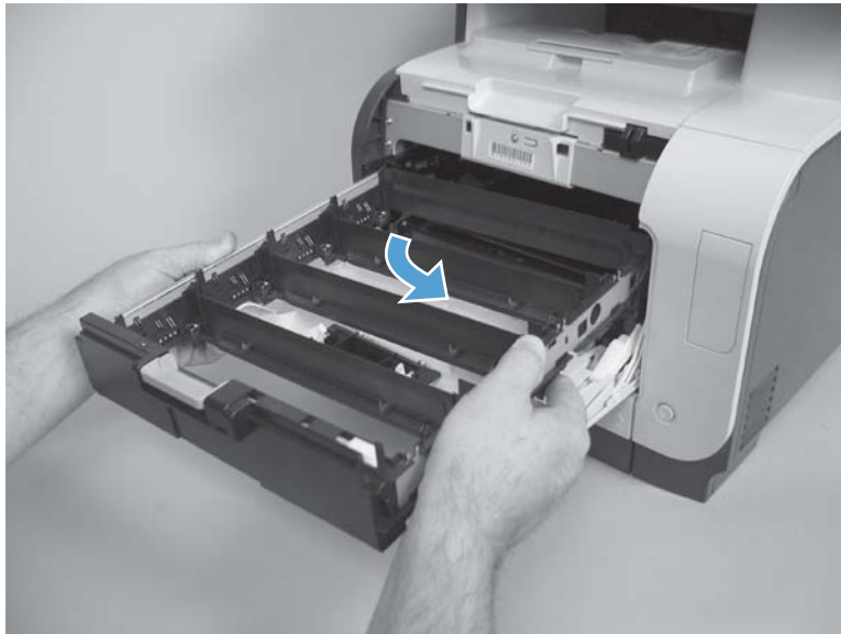
Figure 1-24 Remove the print-cartridge drawer (2 of 3)
