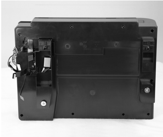
Figure 1-18 Turn the scanner assembly over
