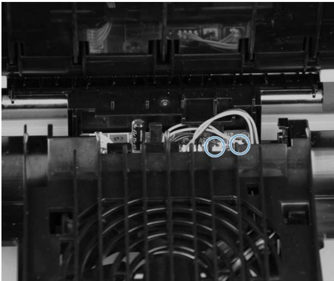
Figure 1-114 Remove the duplex-reverse drive assembly (1 of 4)
