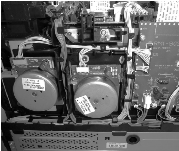
Figure 1-133 DCC plugs disconnected
