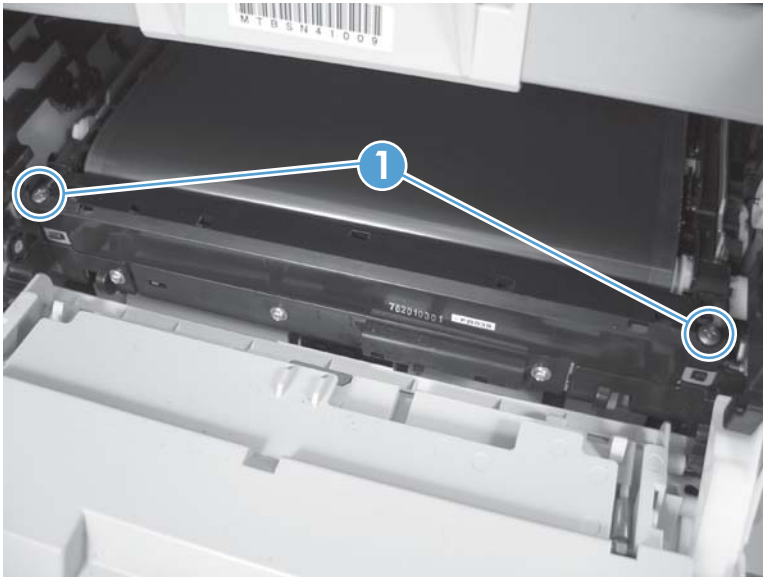
Figure 1-71 Remove the ITB (1 of 6)
