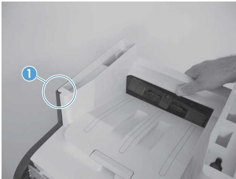
Figure 1-53 Reinstall the upper-cover assembly (1 of 3)
