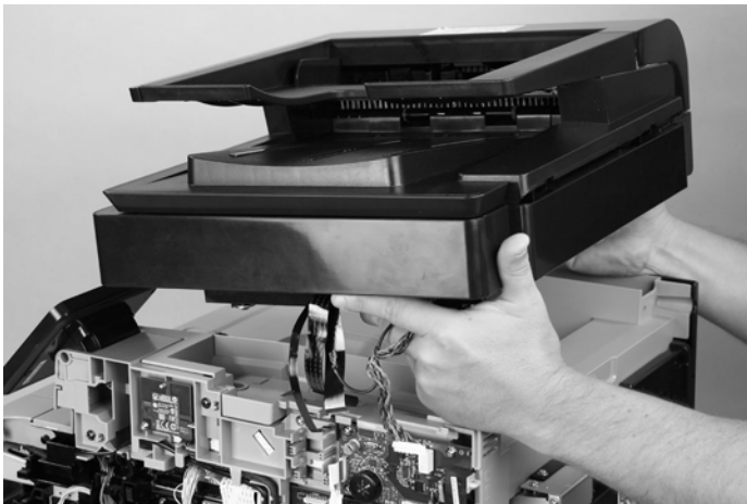
Figure 1-17 Lift the scanner up and off the product
