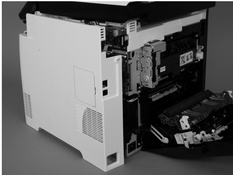
Figure 1-27 Remove the right cover (2 of 2)
