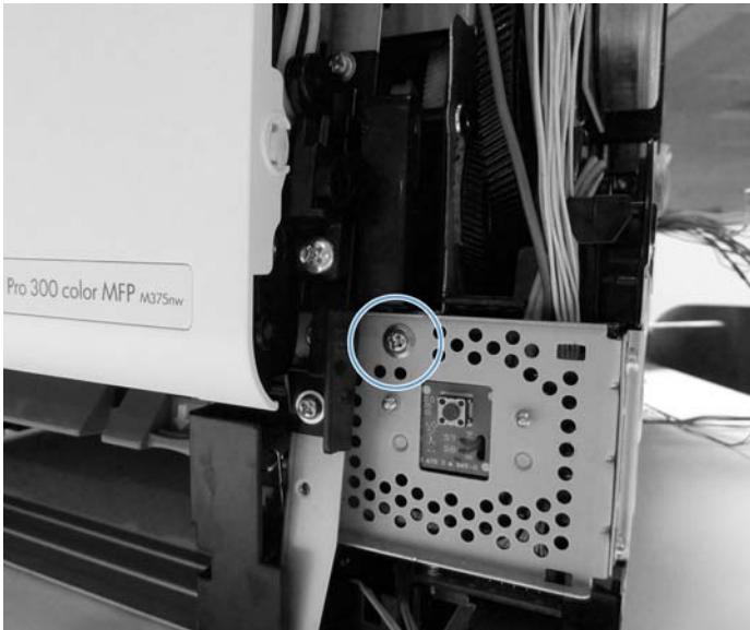
Figure 1-139 Remove one screw above and left of the power switch
