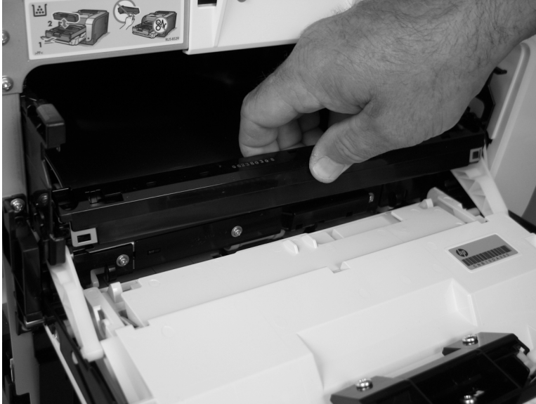
Figure 1-108 Remove the color-misregistration sensor assembly PCA (4 of 4)
