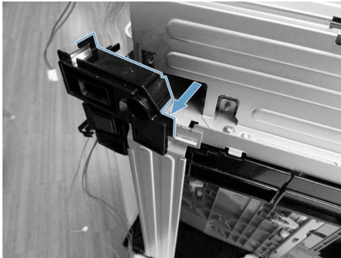
Figure 1-141 Remove the tray 3 harness and pin guide
