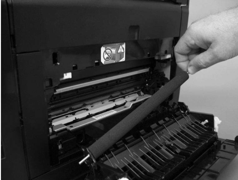
Figure 1-8 Remove the transfer roller (3 of 3)
