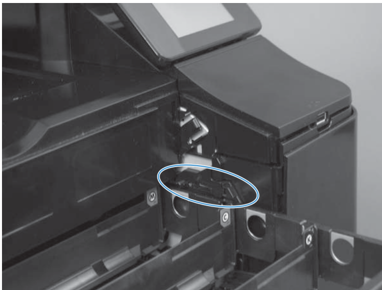
Figure 1-10 Remove the toner-cartridge drawer (2 of 4)
