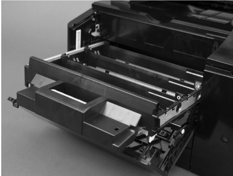
Figure 1-9 Remove the toner-cartridge drawer (1 of 4)
