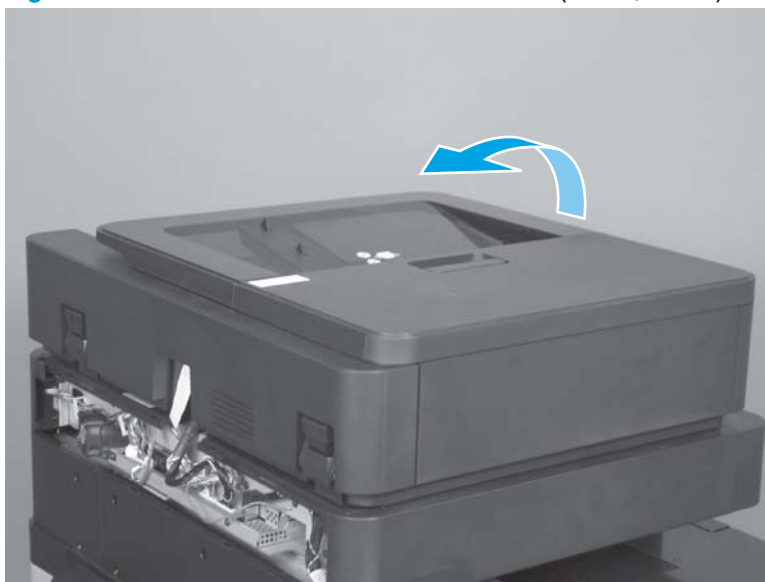
Figure 1-120 Remove the scanner front cover (M880; 1 of 8)
