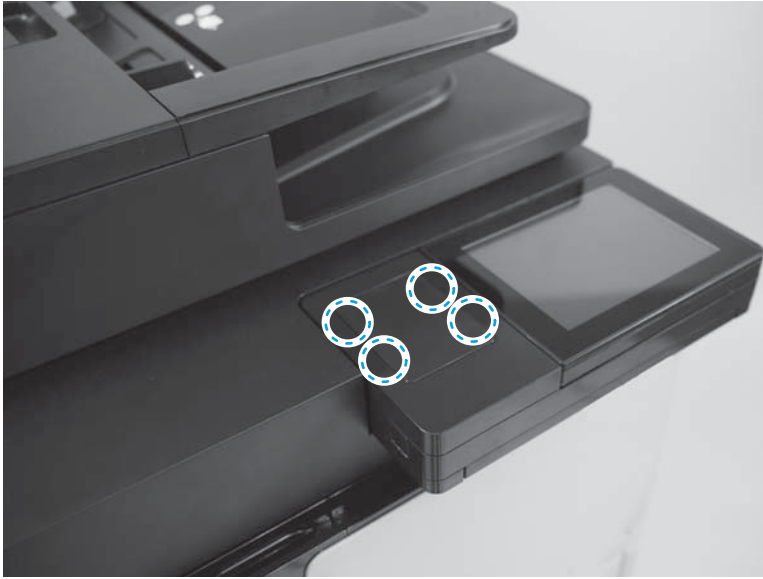
Figure 1-130 Remove the HIP cover (M880; 1 of 3)
