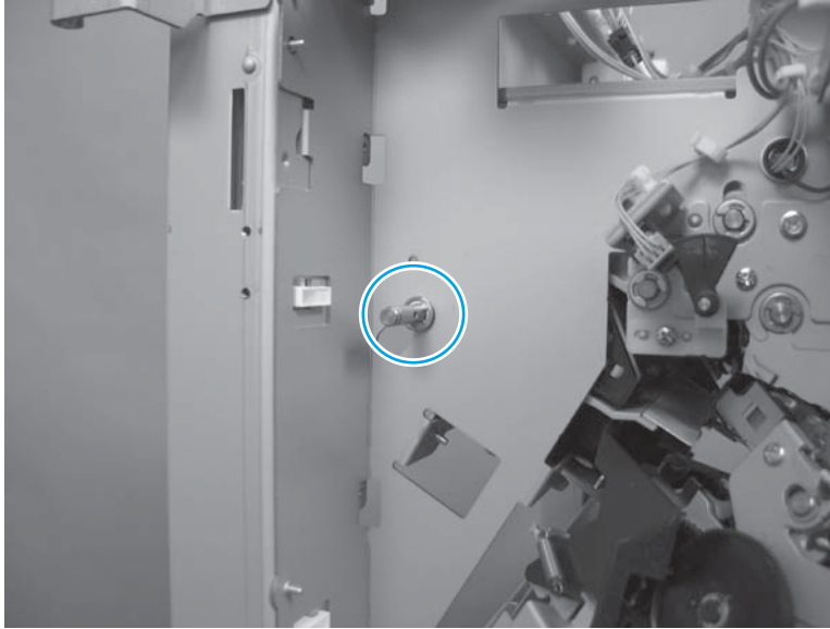
Figure 1-842 Remove the operation tray assembly (3 of 11)
