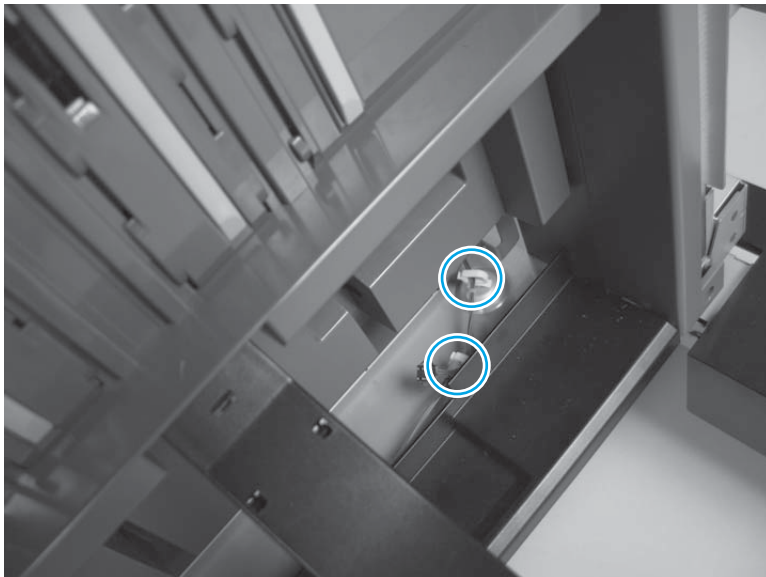
Figure 1-990 Remove the saddle assembly (1 of 13)
