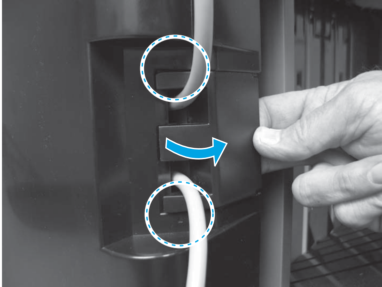
Figure 1-730 Remove the bin cable guide cover (3 of 6)
