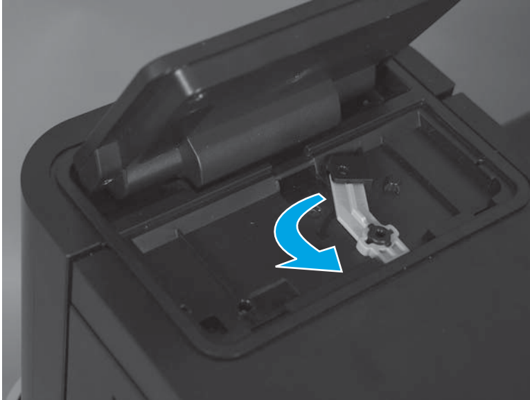
Figure 1-52 Remove the control panel assembly (M855; 4 of 10)
