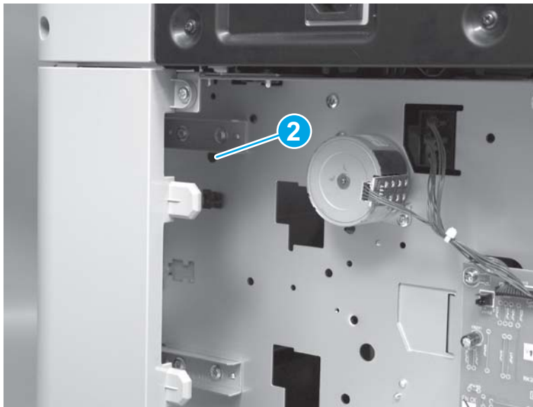
Figure 1-592 Reinstall the 1x500 Tray 3 pickup assembly (2 of 4)
