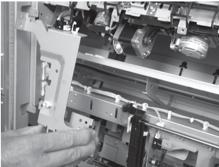
Figure 1-821 Remove the paper face sensor and flag assembly (9 of 9)
