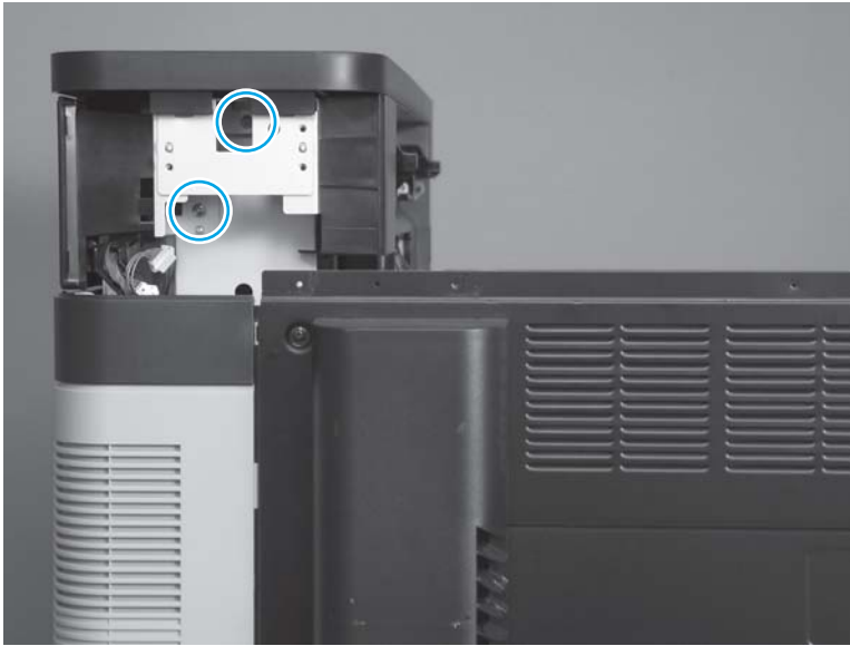
Figure 1-173 Remove the right upper cover (M855; 4 of 9)
