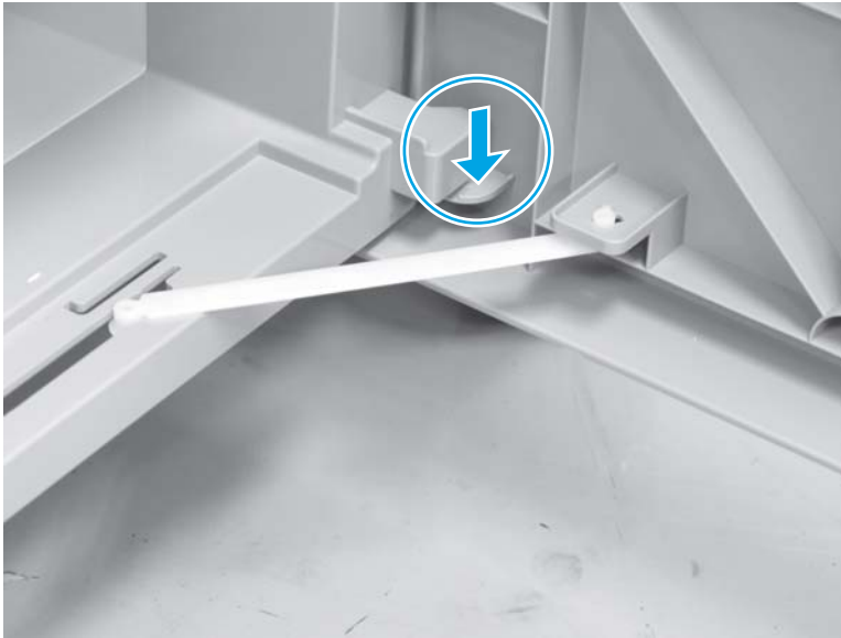
Figure 1-579 Remove the 1x500 storage box door (1 of 3)
