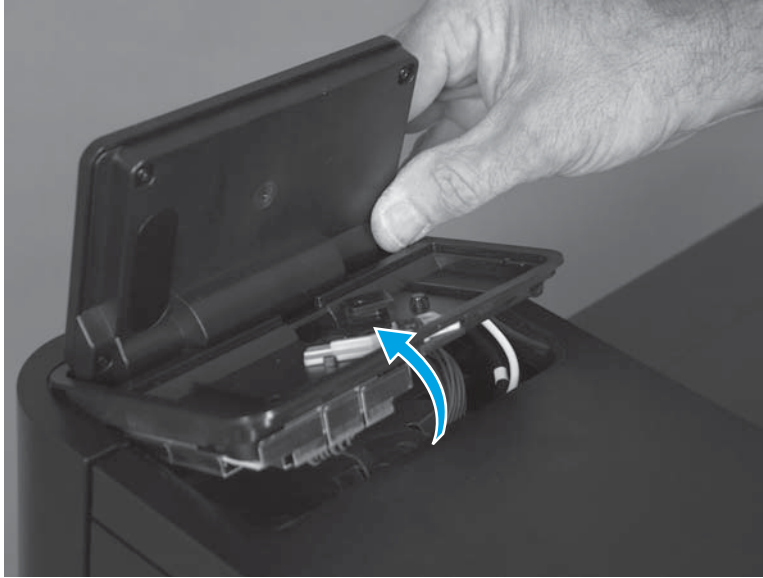
Figure 1-53 Remove the control panel assembly (M855; 5 of 10)
