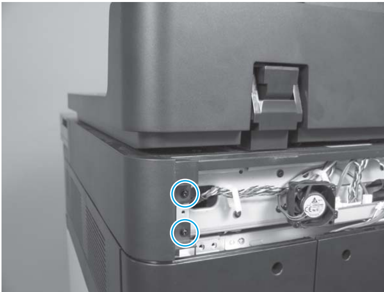
Figure 1-118 Remove the scanner right cover (M880; 1 of 2)
