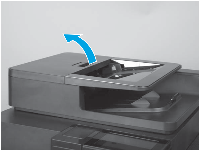
Figure 1-44 Remove the background selector (M880; 1 of 4)
