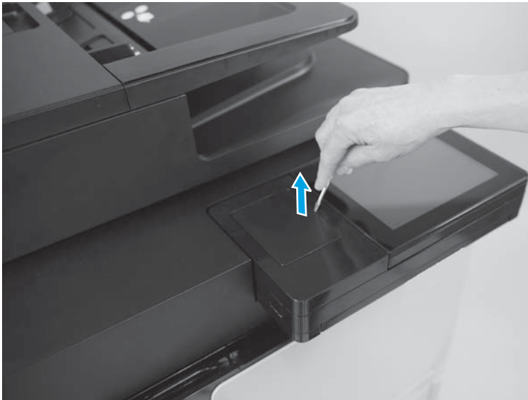
Figure 1-131 Remove the HIP cover (M880; 2 of 3)
