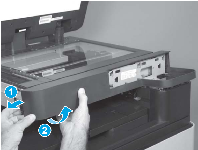
Figure 1-126 Remove the scanner front cover (M880; 7 of 8)
