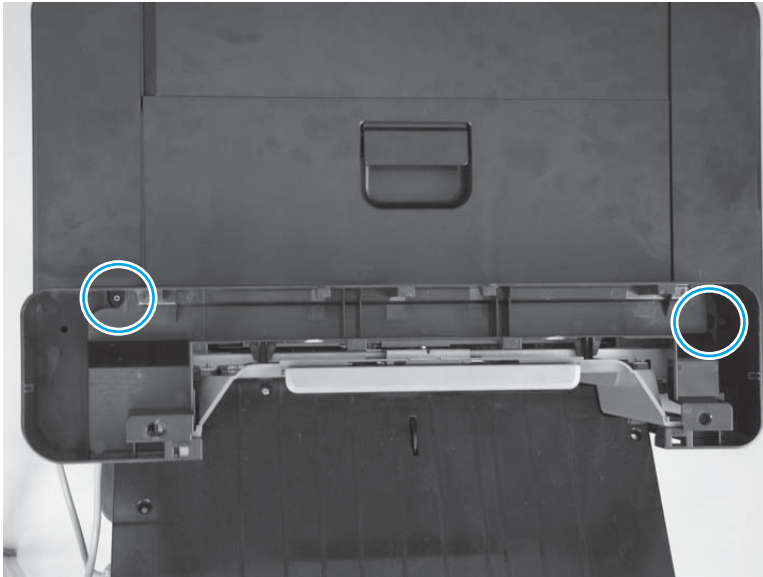
Figure 1-697 Remove the lower stepped cover assembly (1 of 5)
