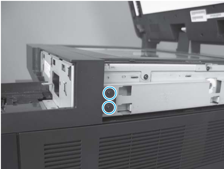
Figure 1-122 Remove the scanner front cover (M880; 3 of 8)
