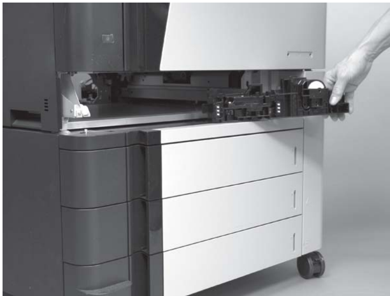
Figure 1-412 Remove the lifter-drive assembly (3 of 3)
