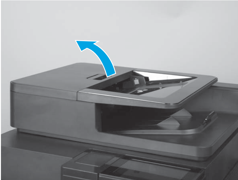
Figure 1-85 Remove the document-feeder roller (M880; 1 of 3)
