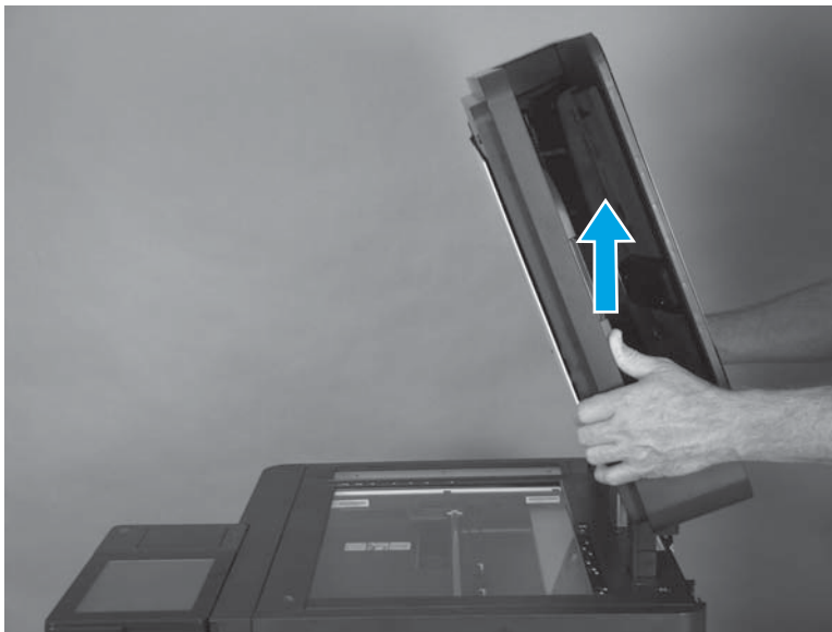
Figure 1-222 Remove the document feeder assembly (M880; 7 of 9)
