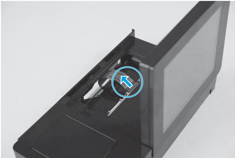
Figure 1-73 Remove the keyboard assembly (M880; 3 of 7)
