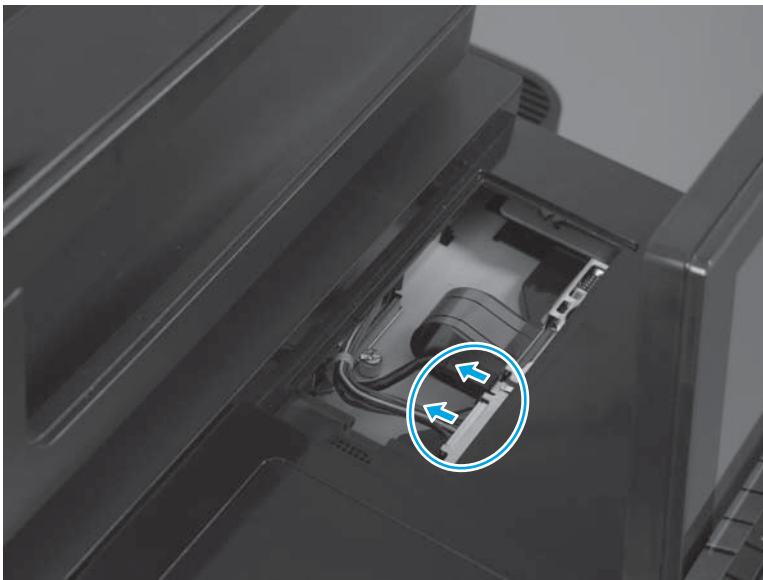
Figure 1-63 Remove the control panel assembly (M880; 4 of 8)
