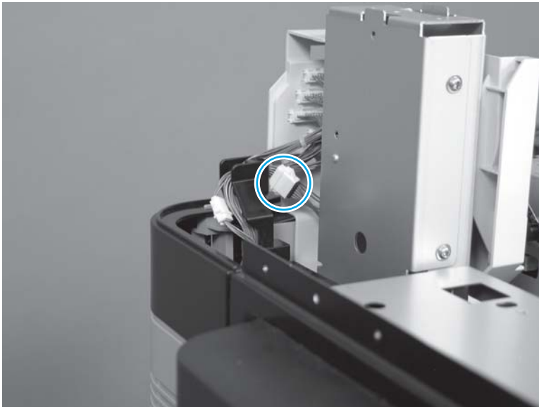
Figure 1-487 Remove the face-down delivery assembly (M855; 7 of 8)
