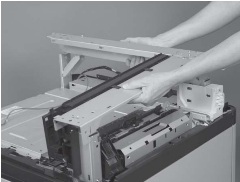
Figure 1-498 Remove the face-down delivery assembly (M880; 10 of 19)
