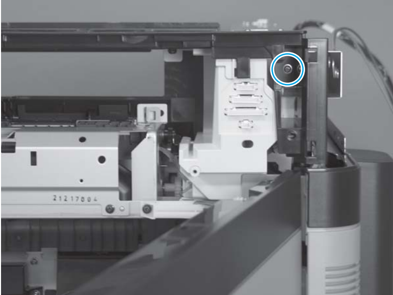
Figure 1-489 Remove the face-down delivery assembly (M880; 1 of 19)
