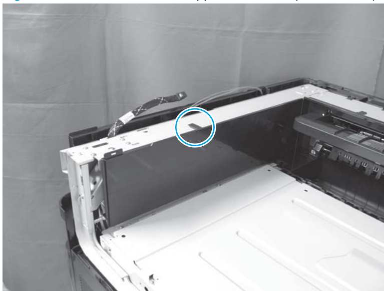
Figure 1-157 Remove the rear upper front cover (M880; 1 of 2)
