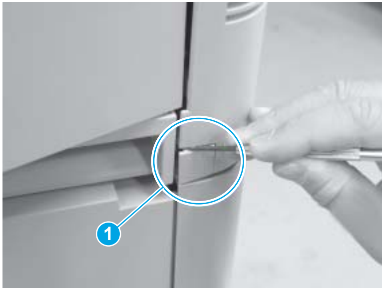
Figure 1-261 Remove the multipurpose tray (Tray 1) drive assembly (1 of 13)
