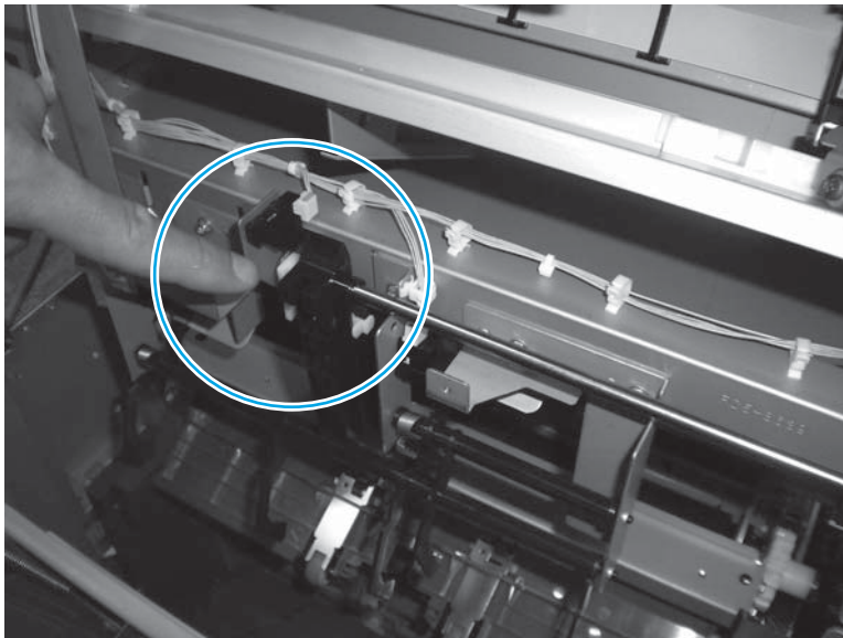
Figure 1-812 Reinstall the height wall assembly
