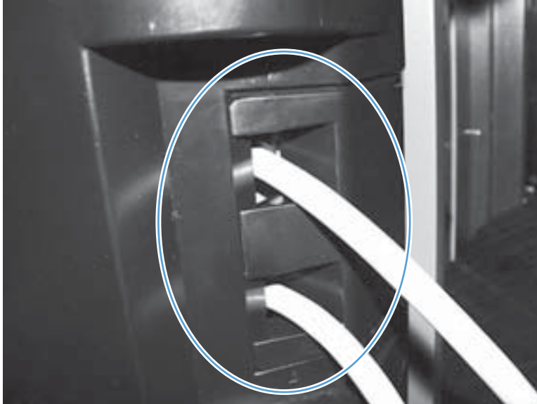
Figure 1-735 Bin cable guide cover incorrectly installed
