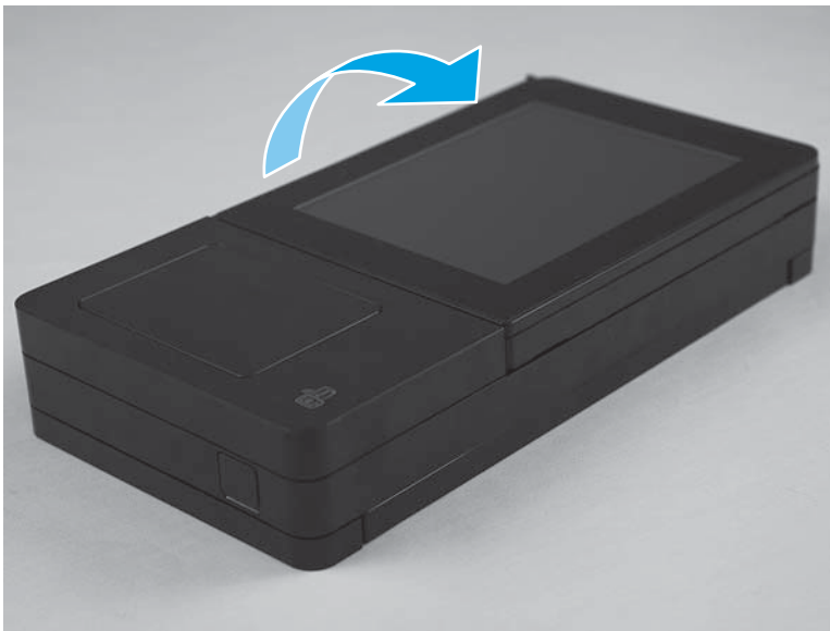
Figure 1-81 Reinstall the keyboard assembly (M880; 4 of 7)
