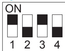
Figure 1-1059 SW601 sensor adjustment settings
