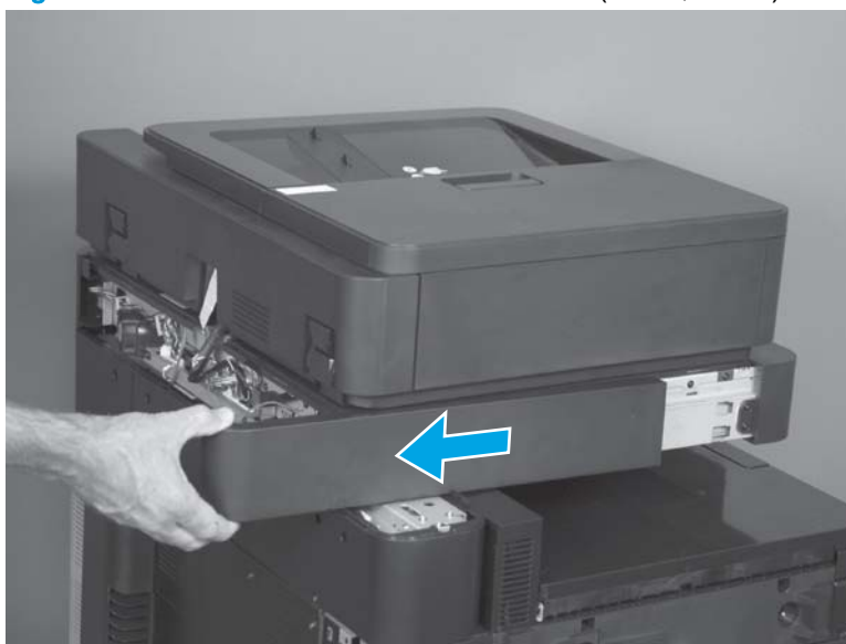
Figure 1-117 Remove the scanner left cover (M880; 2 of 2)
