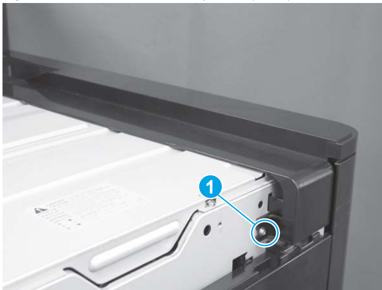
Figure 1-159 Remove the front top cover (1 of 2)
