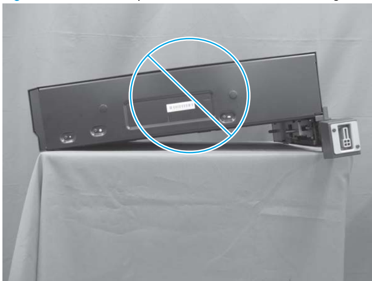
Figure 1-634 Incorrect placement of the IPTU for servicing
