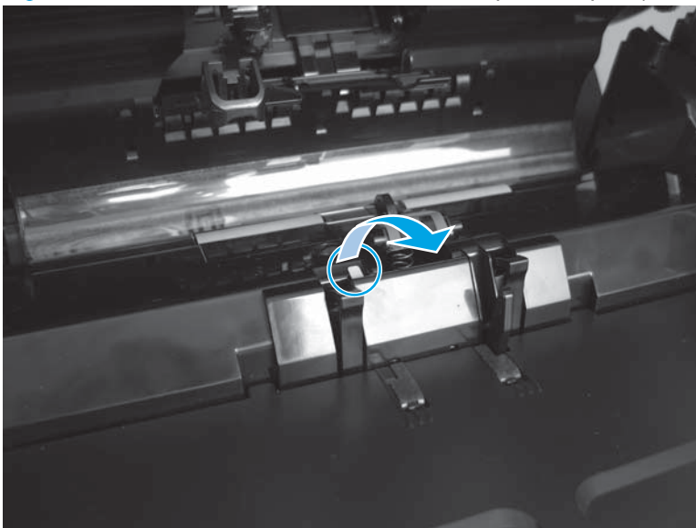
Figure 1-90 Remove the document-feeder separation pad (M880; 2 of 4)
