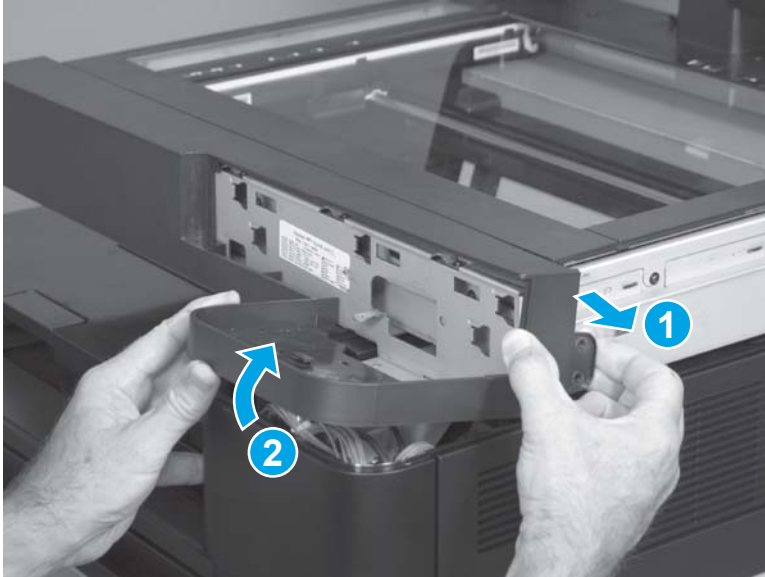
Figure 1-125 Remove the scanner front cover (M880; 6 of 8)
