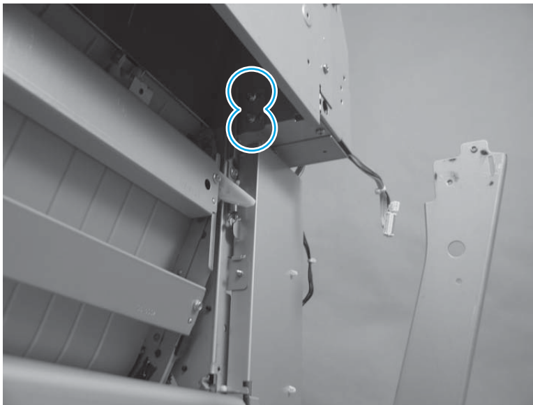
Figure 1-907 Remove the paper pass assembly (5 of 6)
