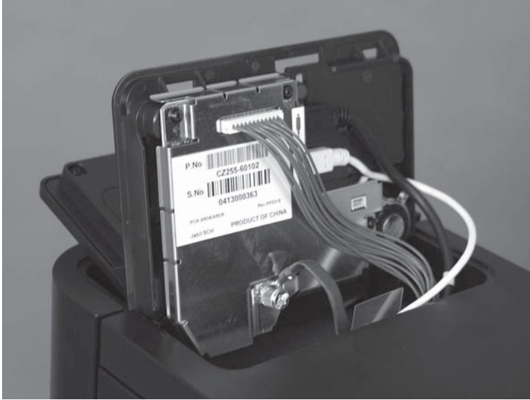
Figure 1-55 Remove the control panel assembly (M855; 7 of 10)
