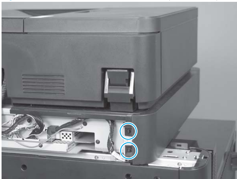
Figure 1-116 Remove the scanner left cover (M880; 1 of 2)
