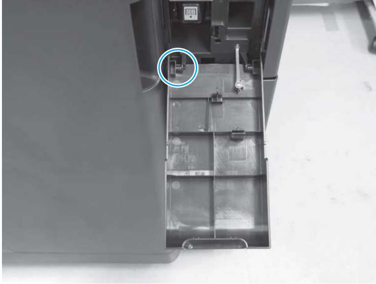
Figure 1-1026 Remove the punch front cover (2 of 2)
