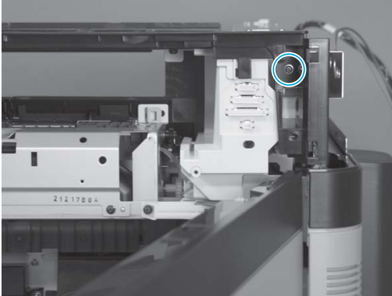
Figure 1-475 Remove the VOC fan (M880; 1 of 6)
