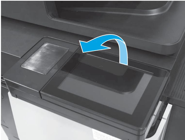
Figure 1-60 Remove the control panel assembly (M880; 1 of 8)
