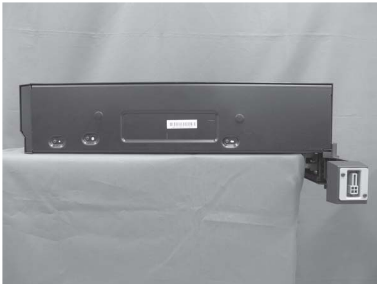
Figure 1-634 Incorrect placement of the IPTU for servicing
