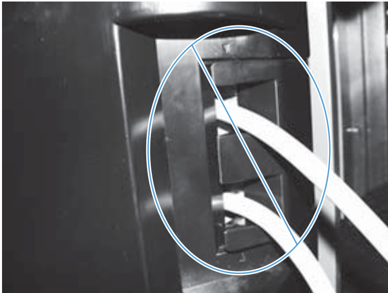
Figure 1-735 Bin cable guide cover incorrectly installed
