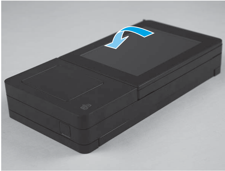
Figure 1-74 Remove the keyboard assembly (M880; 4 of 7)
