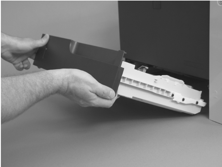
Figure 2-17 Remove the tray (2 of 2)
