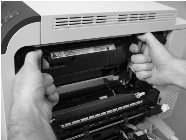
Figure 2-19 Remove the fuser (2 of 2)
