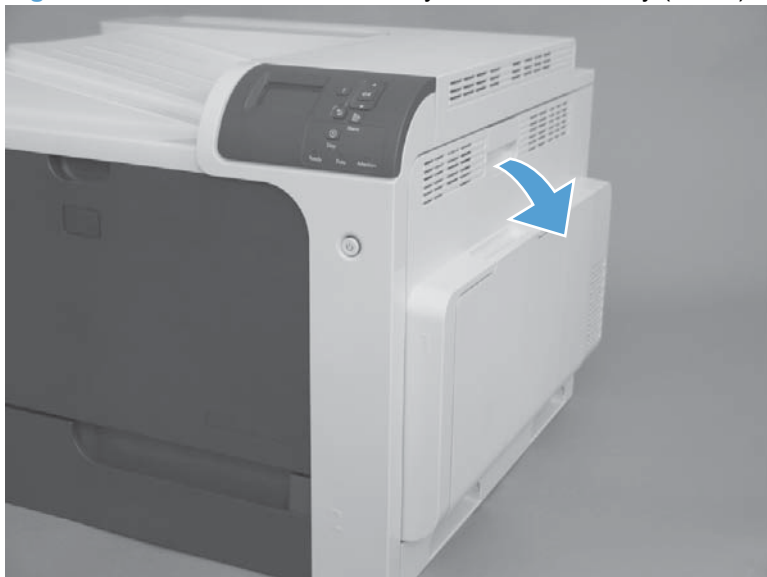
Figure 2-71 Remove the secondary transfer assembly (1 of 3)
