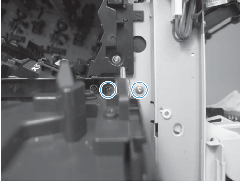
Figure 2-55 Remove the front-door assembly (4 of 5)
