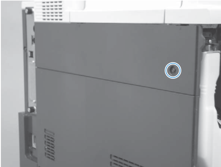
Figure 2-36 Remove the upper-left cover (2 of 3)
