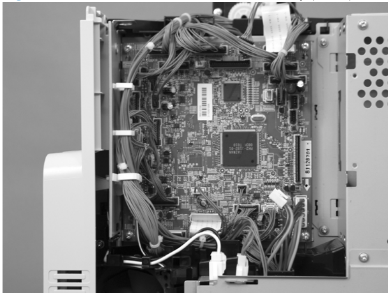
Figure 2-128 Remove the DC controller PCA only (1 of 2)
