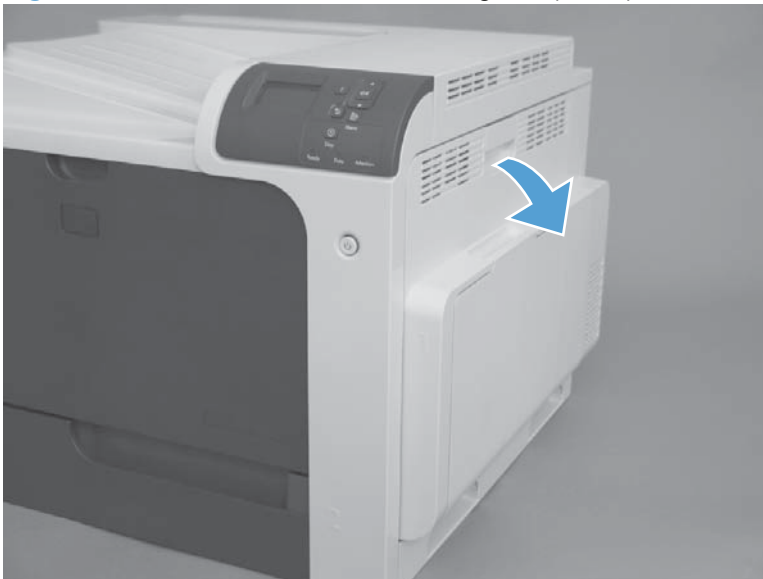
Figure 2-69 Remove the cassette feed guide (1 of 2)
