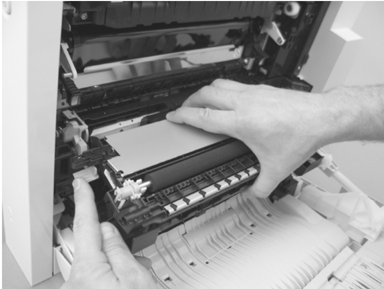
Figure 2-74 Reinstall the secondary transfer assembly
