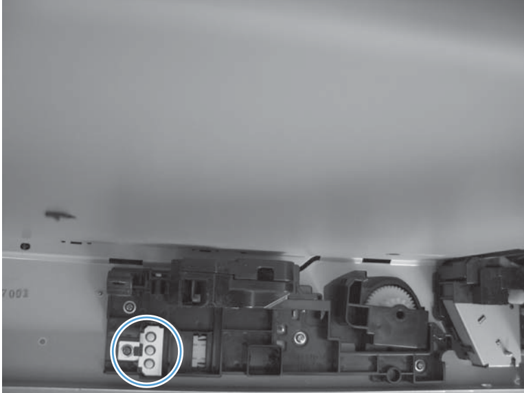
Figure 3-22 Test the Tray 2 paper size switches
