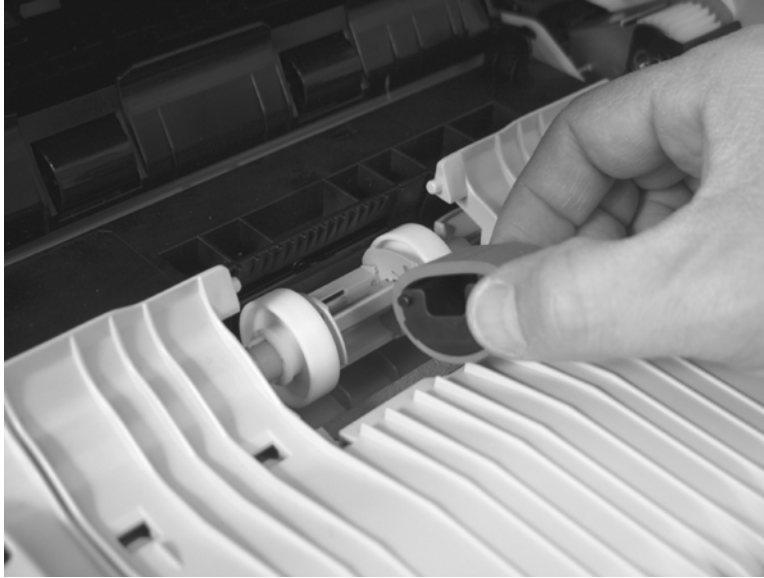
Figure 2-25 Remove the pickup roller (Tray 1) (5 of 5)
