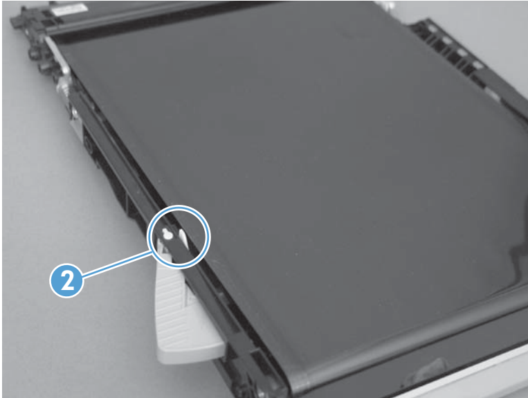
Figure 3-13 Test the primary transfer-roller-disengagement sensor (2 of 4)
