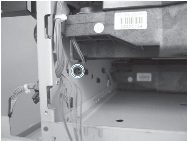
Figure 2-176 Remove the laser/scanner assembly (Y/M) (2 of 5)
