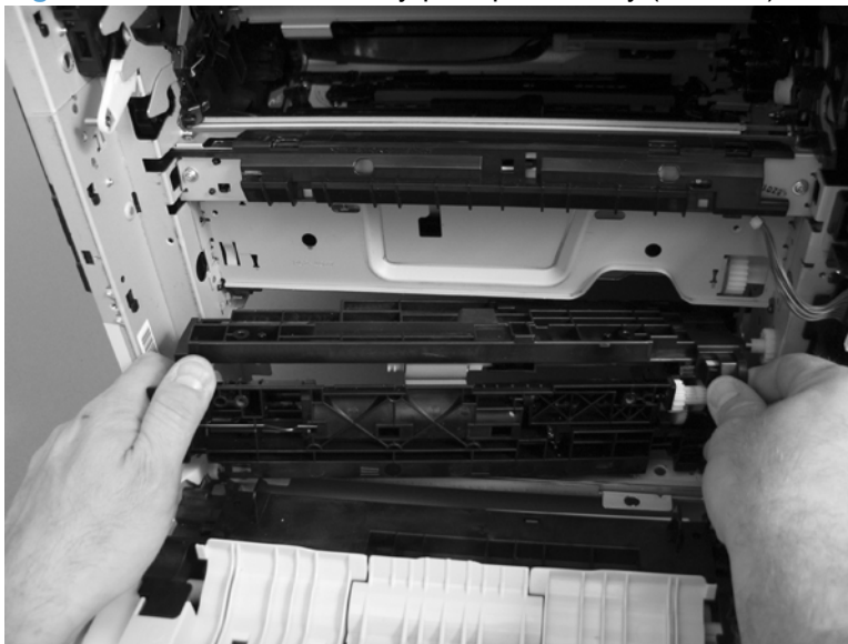
Figure 2-174 Remove the tray-pickup assembly (11 of 11)
