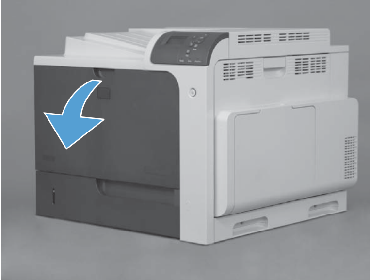
Figure 2-6 Remove the toner-collection unit (1 of 4)
