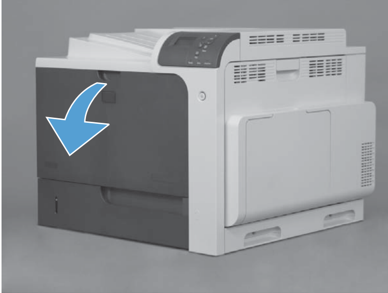
Figure 2-35 Remove the upper-left cover (1 of 3)
