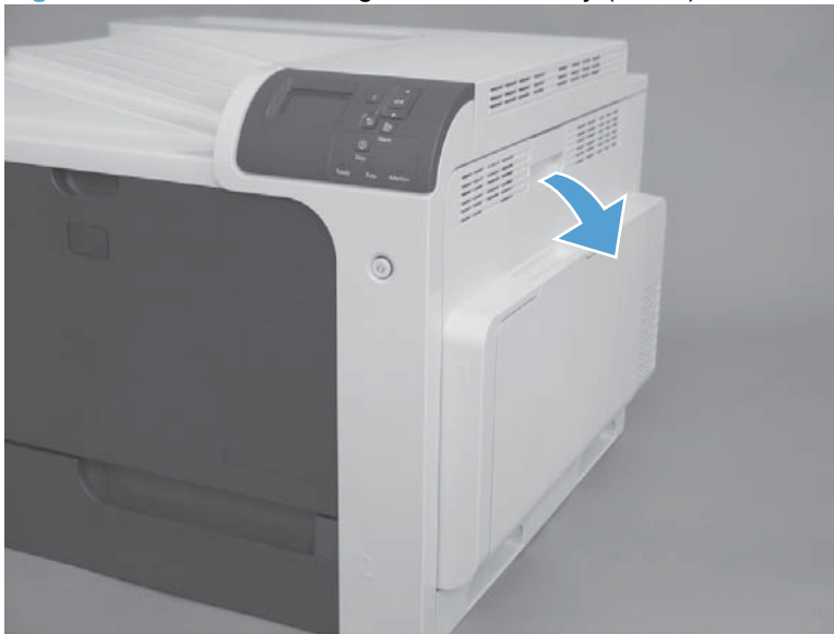
Figure 2-60 Remove the right-door assembly (1 of 9)
