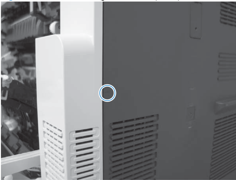
Figure 2-57 Remove the right-rear cover (1 of 2)
