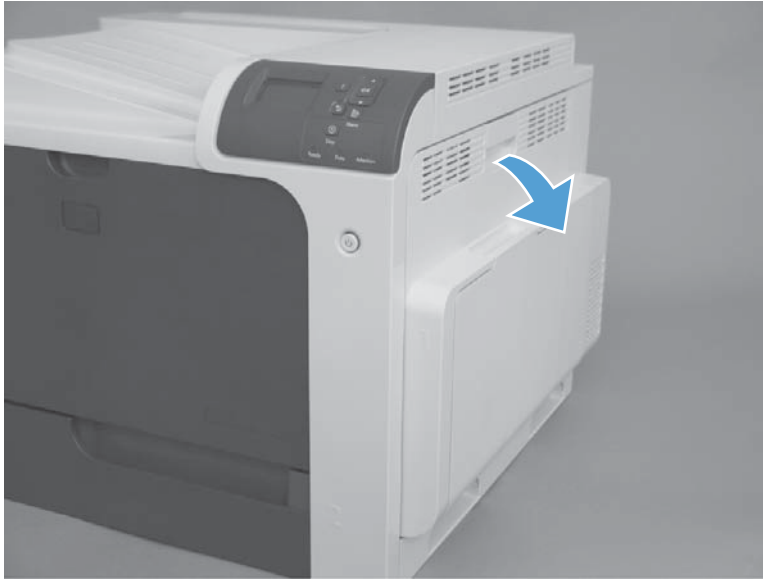
Figure 2-18 Remove the fuser (1 of 2)
