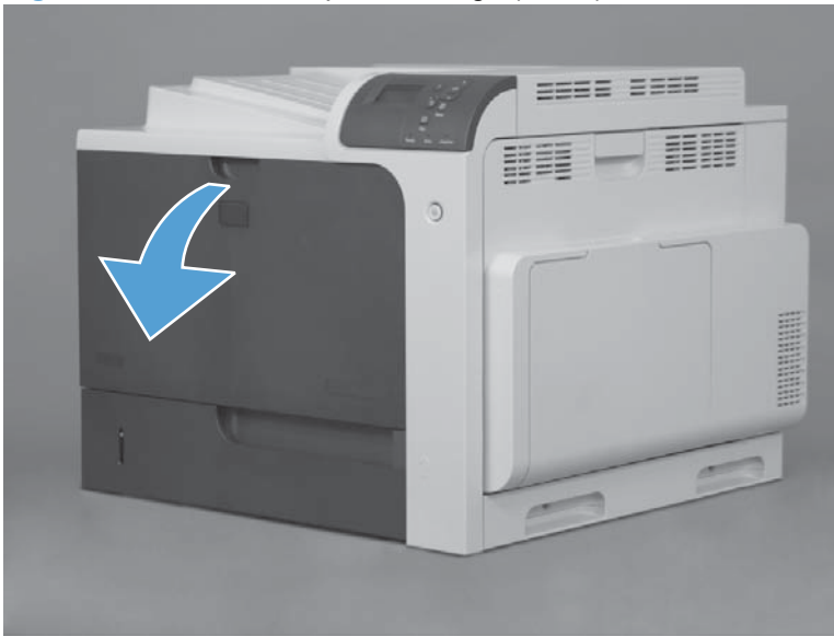
Figure 2-4 Remove the print cartridge (1 of 2)
