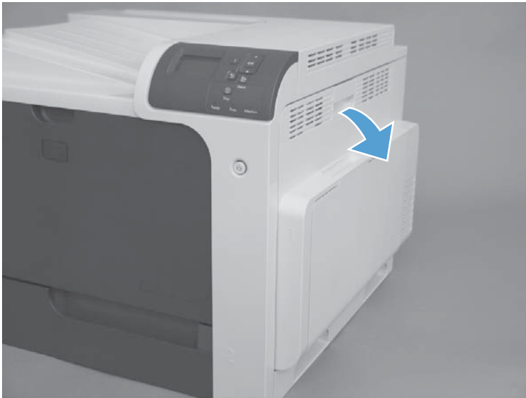
Figure 2-26 Remove the transfer roller (1 of 3)
