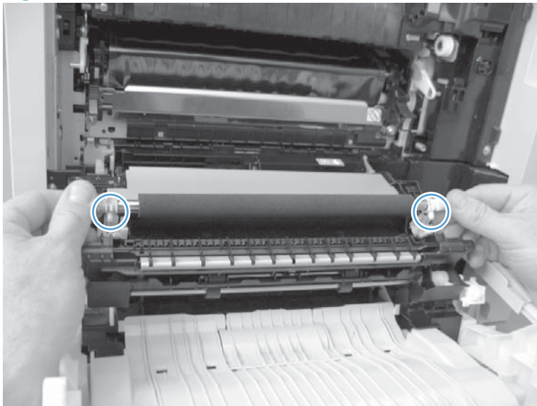
Figure 2-29 Reinstall the transfer roller
