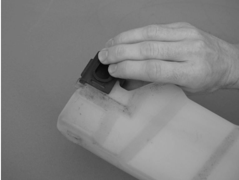
Figure 2-4 Remove the toner-collection unit (3 of 3)
