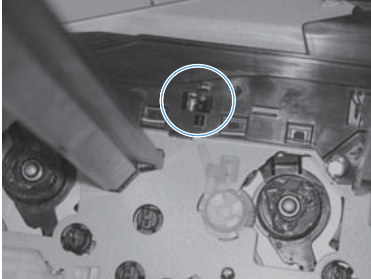
Figure 3-13 Test the ITB alienation switch
