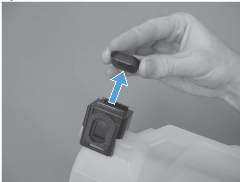
Figure 2-3 Remove the toner-collection unit (2 of 3)
