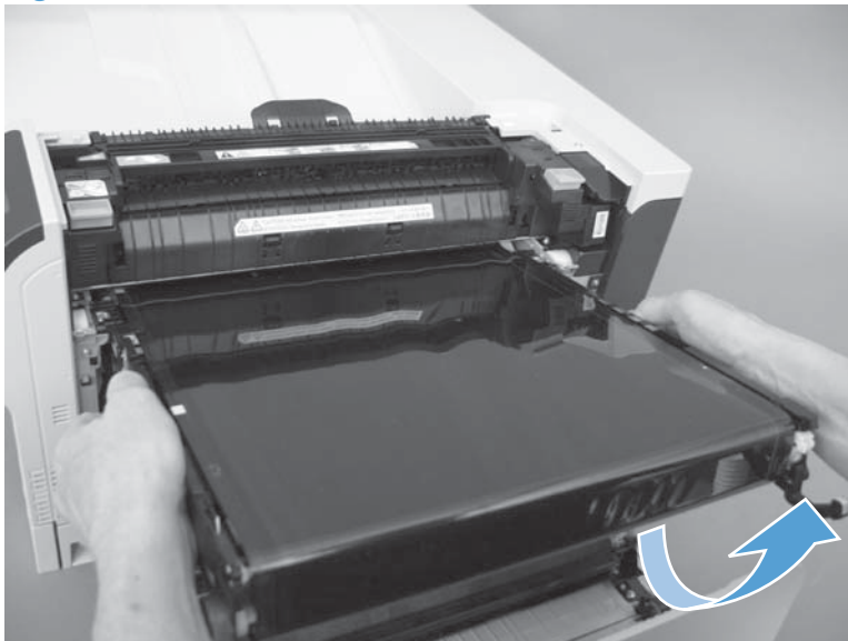
Figure 2-20 Remove the intermediate transfer belt (3 of 3)
