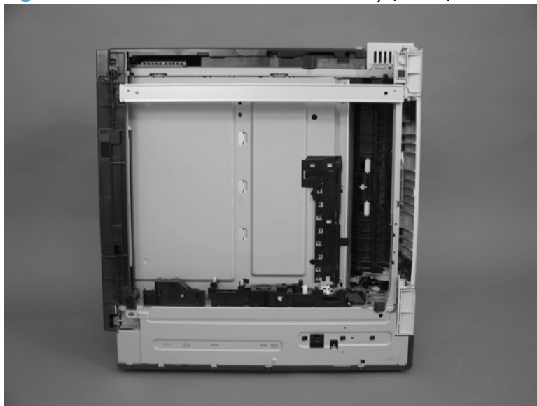
Figure 2-70 Remove the lifter-drive assembly (1 of 3)
