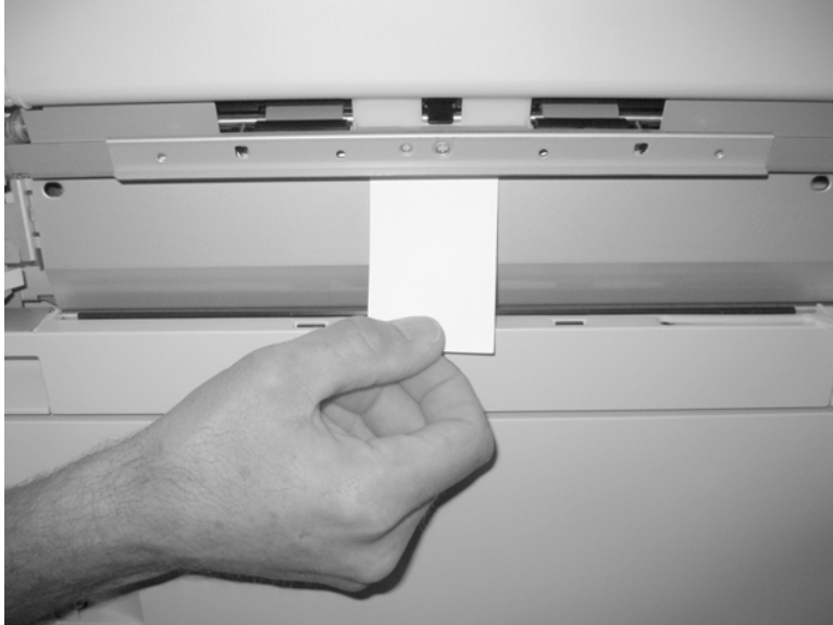
Figure 3-21 Test the Tray 3 feed sensor
