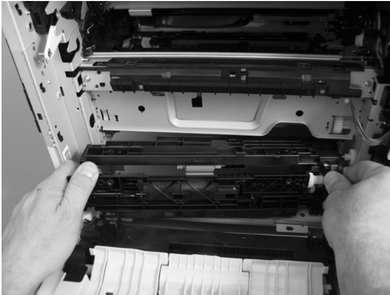
Figure 2-255 Remove the tray-pickup assembly (11 of 11)
