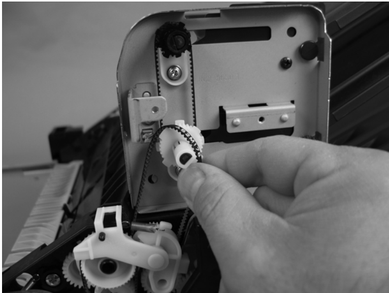
Figure 2-365 Remove the MBM output bin assembly (3 of 3)
