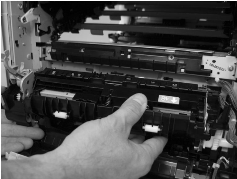
Figure 2-178 Remove the registration assembly (8 of 8)
