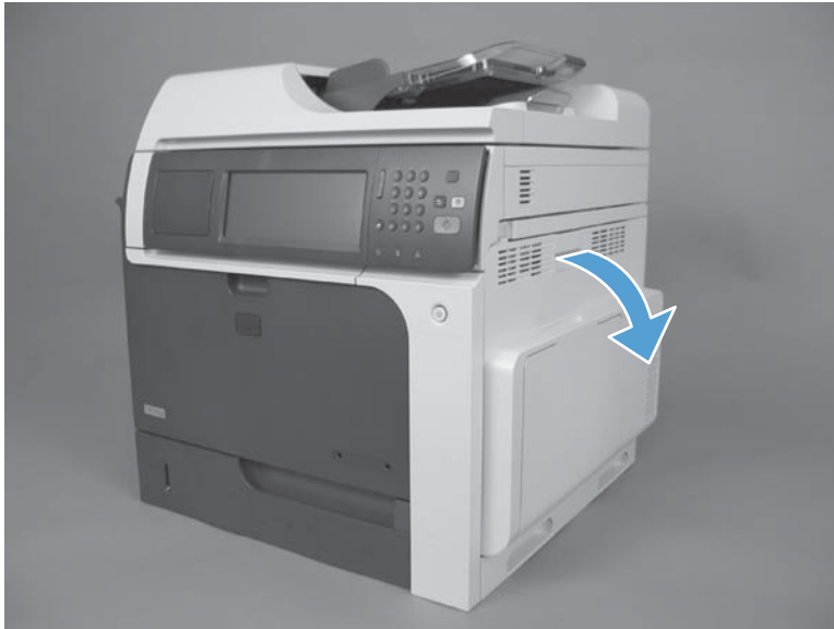
Figure 2-74 Remove the right-door assembly (1 of 9)
