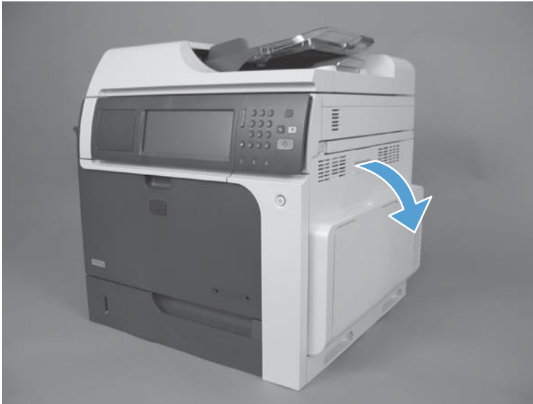
Figure 2-32 Remove the transfer roller (1 of 3)
