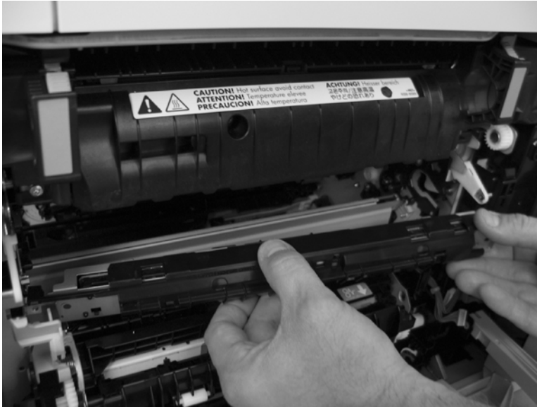
Figure 2-170 Remove the RD sensor assembly (7 of 7)
