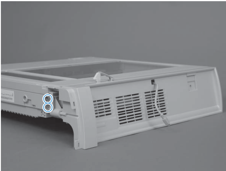
Figure 2-118 Remove the S-ASSY-CP-ADAPTER (CP adapter assembly) (1 of 4)
