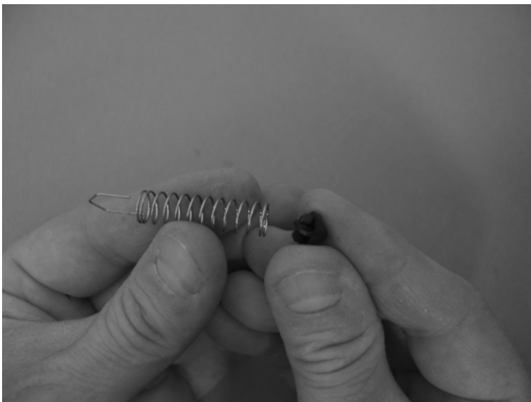
Figure 2-240 Reinstall the lifter base assembly (1 of 2)
