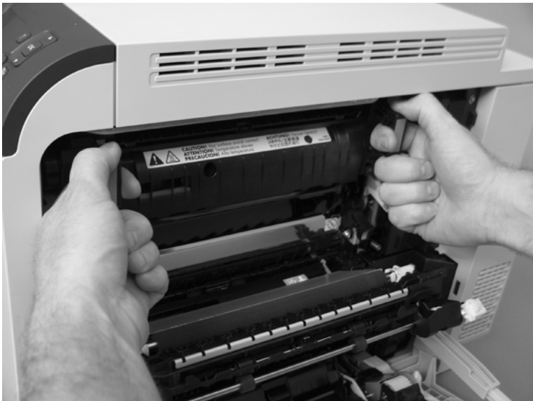
Figure 2-23 Remove the fuser (2 of 2)
