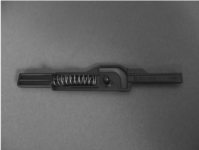
Figure 2-267 Reinstall the PGC actuators (2 of 5)
