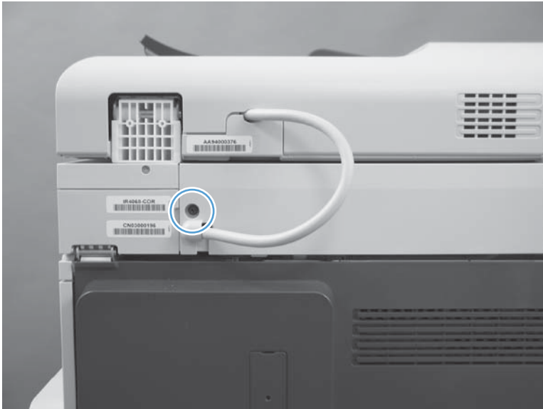
Figure 2-48 Remove S-CVR-REAR (scanner rear cover) (1 of 2)
