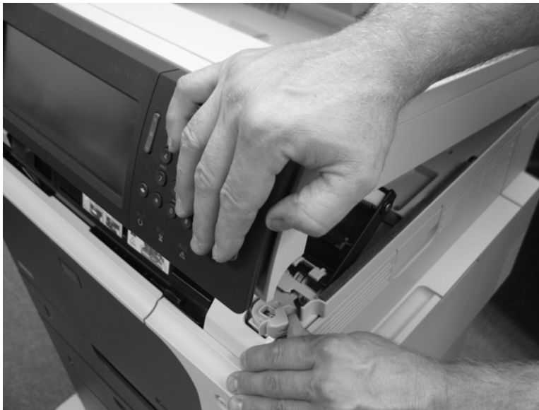
Figure 2-109 Remove the scanner assembly (1 of 6)
