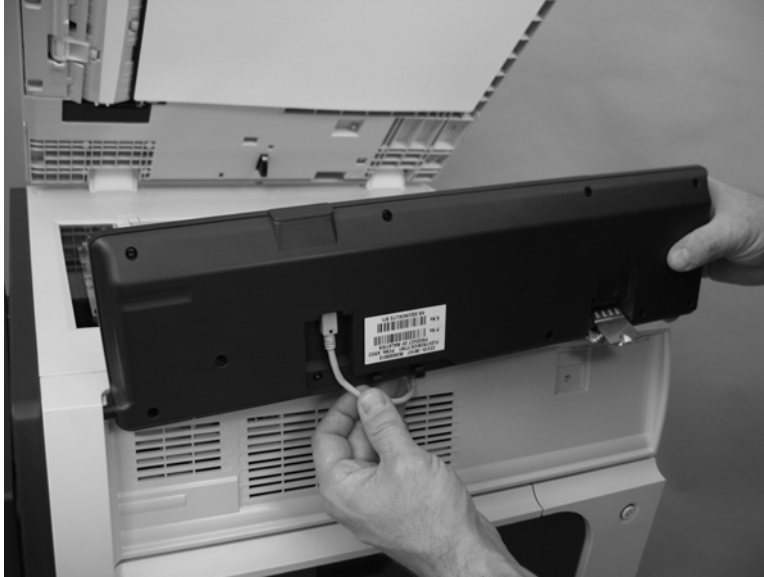
Figure 2-6 Remove the control panel (3 of 3)
