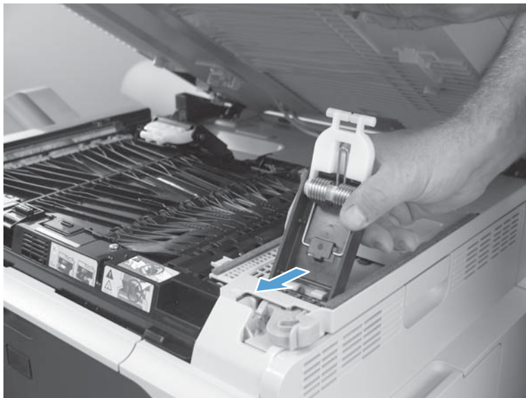
Figure 2-117 Remove the scissor hinge assembly (3 of 3)
