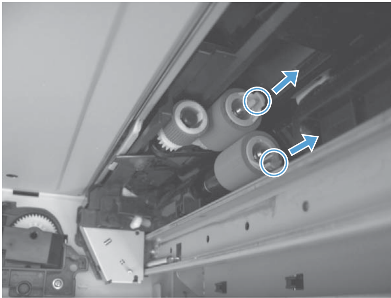
Figure 2-24 Remove the Pickup and feed rollers (Trays 2-5)
