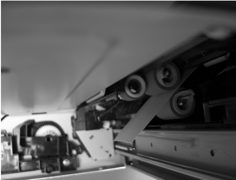
Figure 3-32 Test the Tray 3 feed sensor
