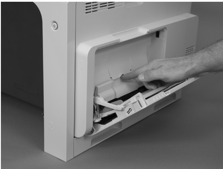
Figure 2-26 Remove the pickup roller (Tray 1) (2 of 5)
