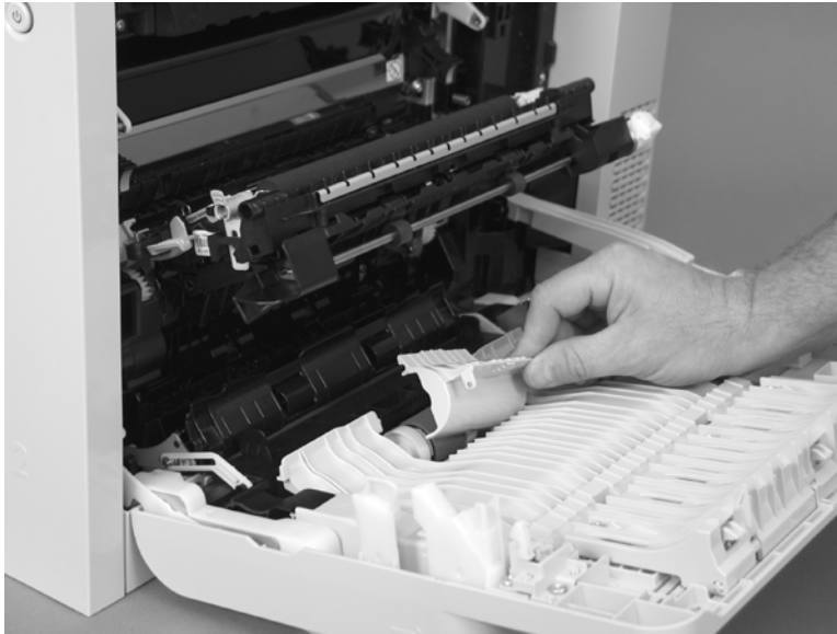
Figure 2-27 Remove the pickup roller (Tray 1) (3 of 5)
