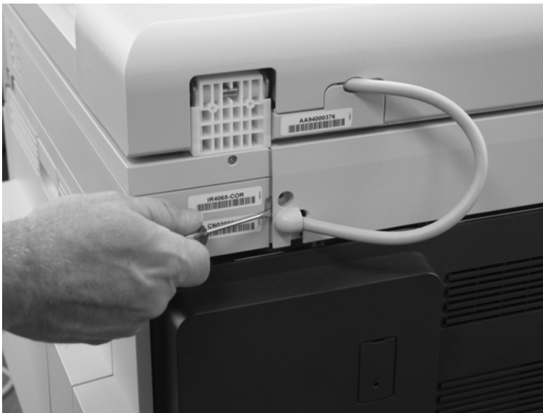
Figure 2-49 Remove S-CVR-REAR (scanner rear cover) (2 of 2)
