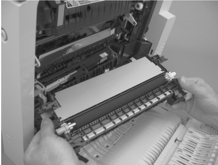
Figure 2-156 Remove the secondary transfer assembly (3 of 3)
