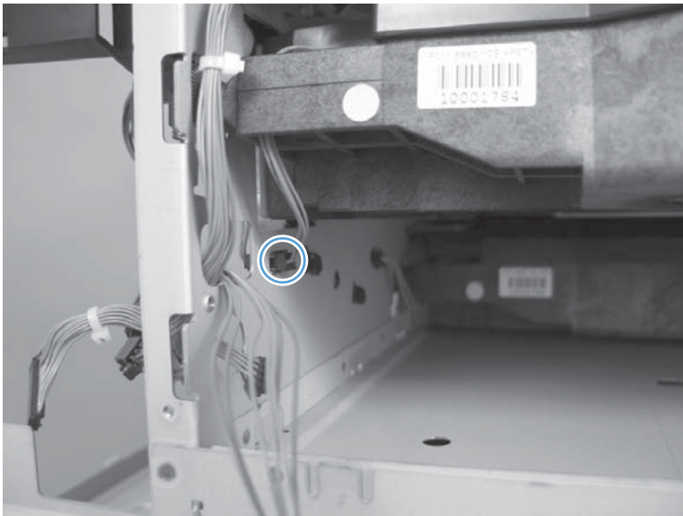
Figure 2-257 Remove the laser/scanner assembly (Y/M) (2 of 5)
