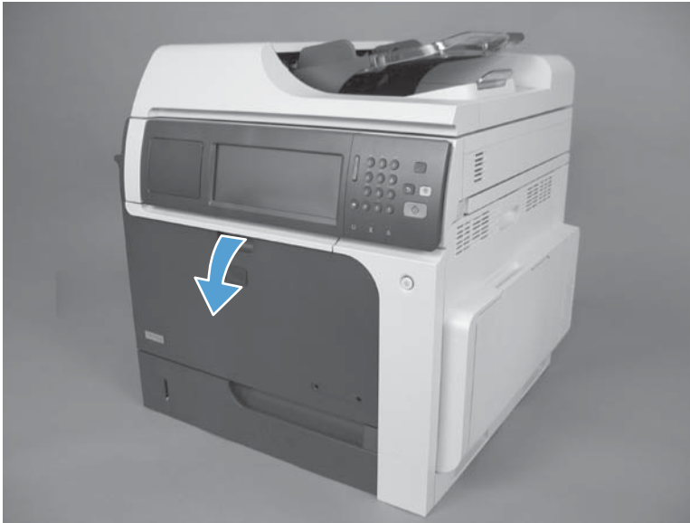
Figure 2-11 Remove the toner-collection unit (1 of 4)
