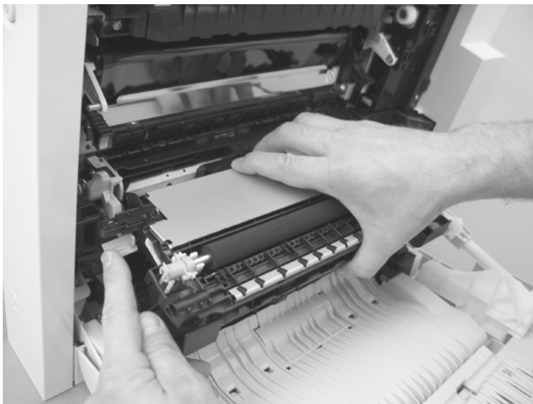
Figure 2-157 Reinstall the secondary transfer assembly
