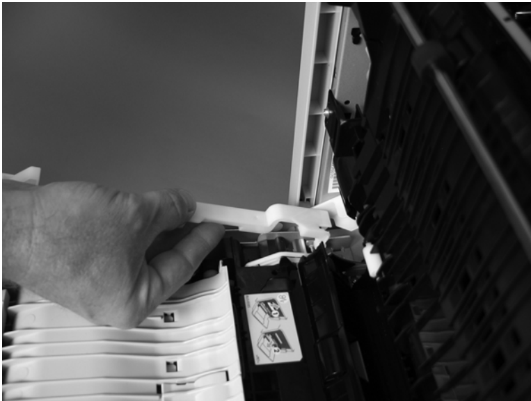
Figure 2-77 Remove the right-door assembly (4 of 9)
