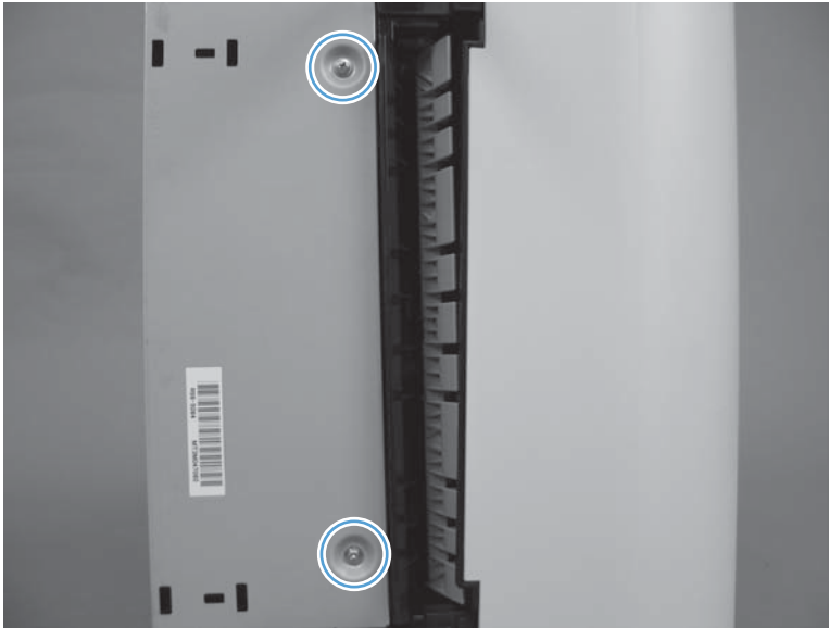
Figure 2-353 Remove the output bin 3 drive assembly (1 of 3)
