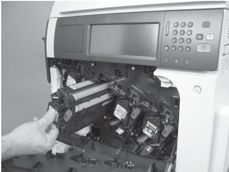
Figure 2-10 Remove the print cartridge (2 of 2)
