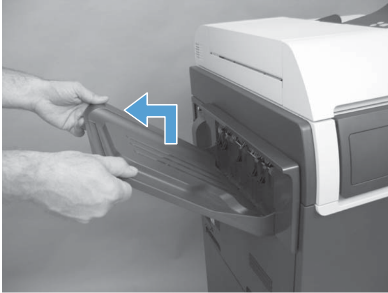
Figure 2-40 Remove the standard output bin
