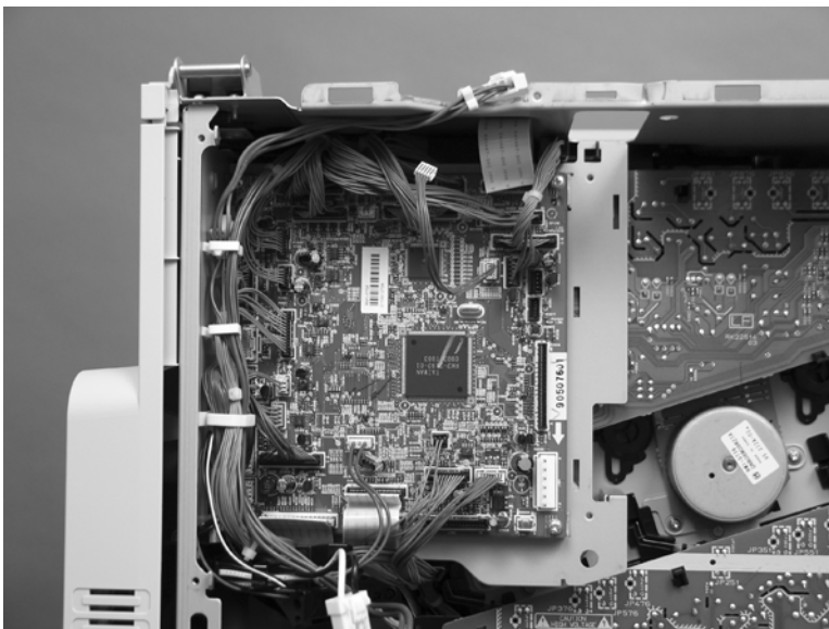
Figure 2-218 Remove the DC controller PCA and tray (1 of 3)
