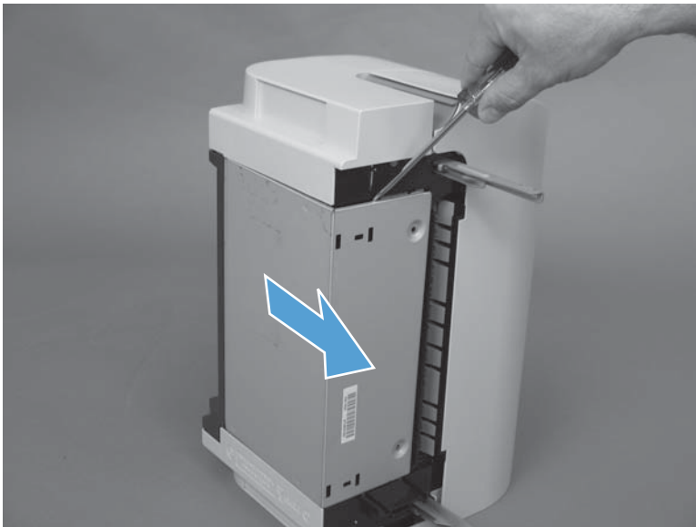
Figure 2-344 Remove the stapling mailbox PCA (2 of 5)
