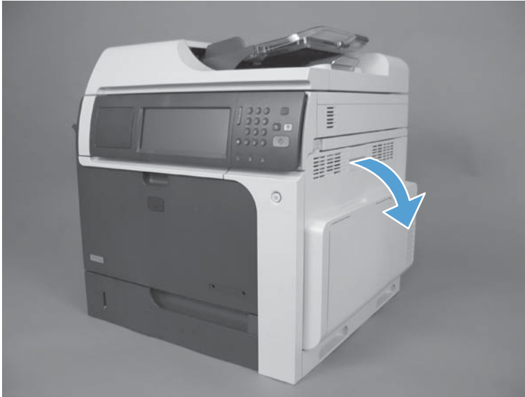
Figure 2-22 Remove the fuser (1 of 2)
