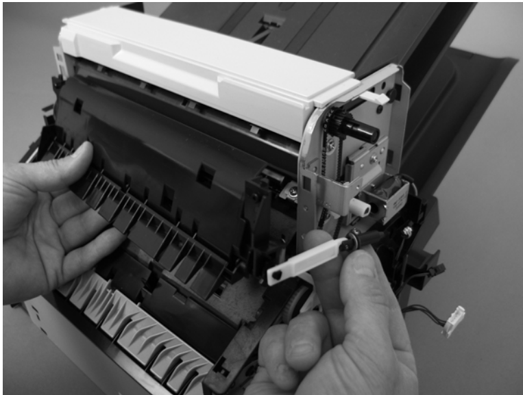
Figure 2-362 Remove the flapper guide assembly (2 of 2)
