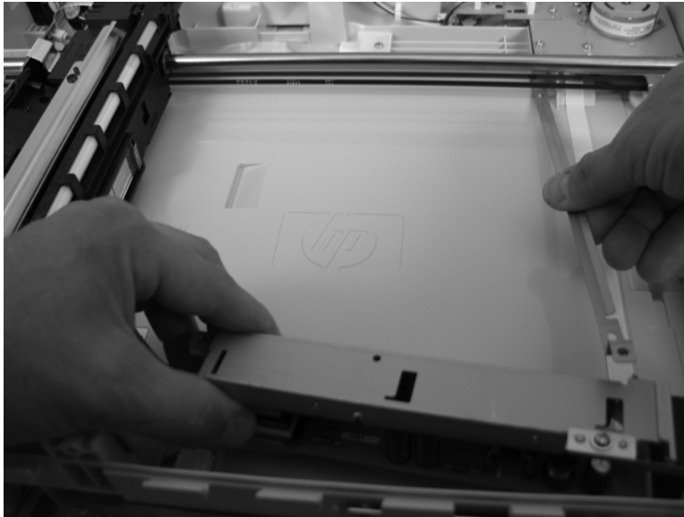
Figure 2-133 Remove the S-ASSY-INV (inverter) (2 of 2)
