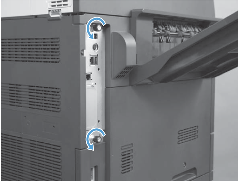
Figure 2-15 Remove the formatter
