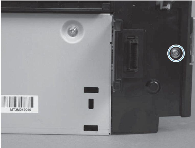
Figure 2-338 Remove the holder connector
