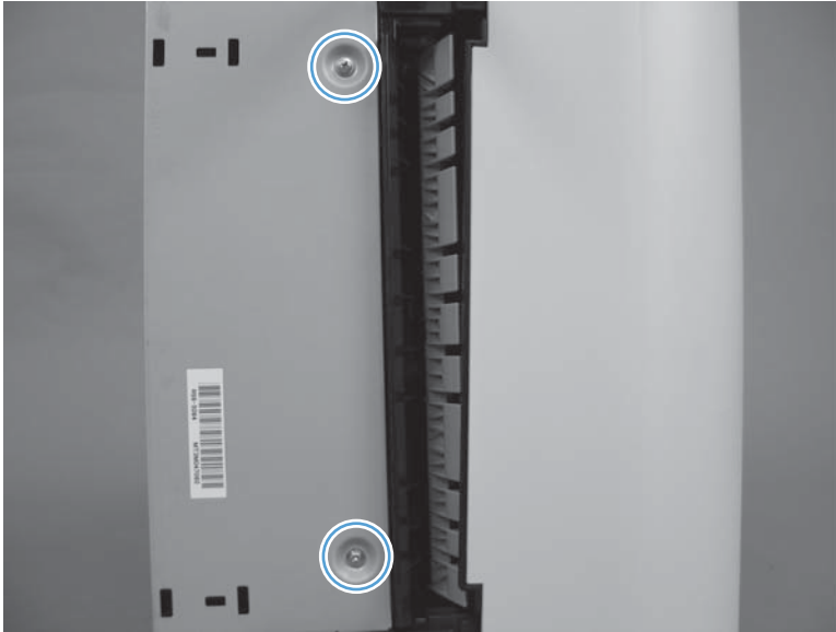
Figure 2-343 Remove the stapling mailbox PCA (1 of 5)
