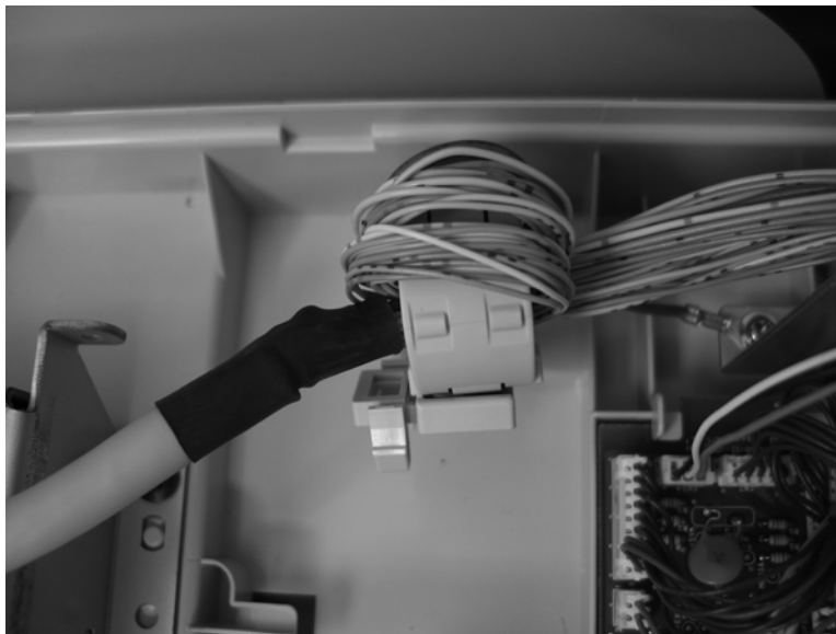
Figure 2-98 Remove the ASM-IF-SP (document feeder cable) (2 of 2)
