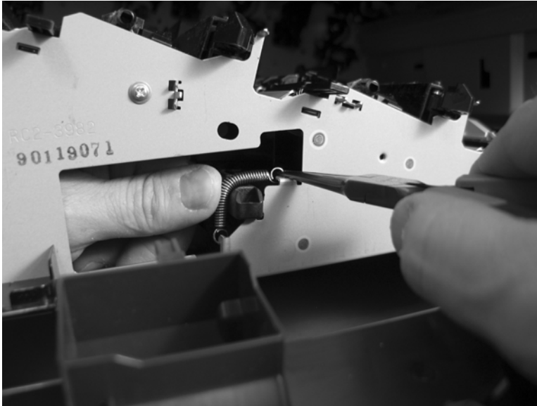
Figure 2-264 Remove the laser/scanner assembly (C/Bk) (4 of 5)
