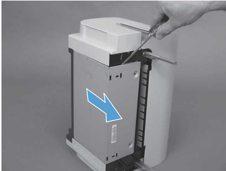
Figure 2-354 Remove the output bin 3 drive assembly (2 of 3)
