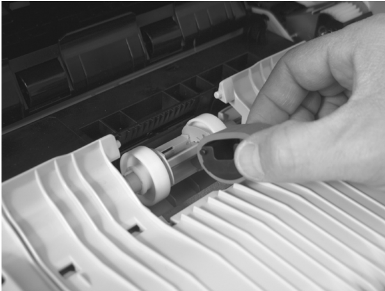
Figure 2-29 Remove the pickup roller (Tray 1) (5 of 5)
