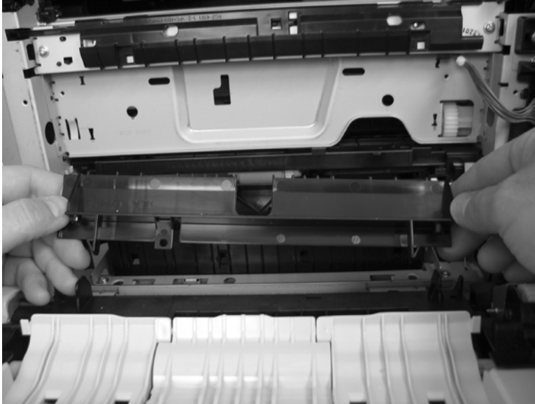
Figure 2-251 Remove the tray-pickup assembly (7 of 11)
