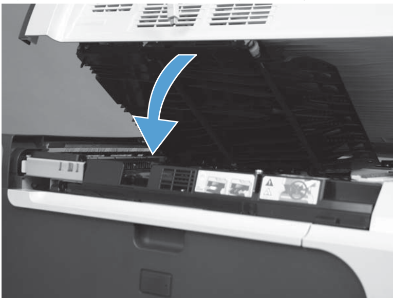
Figure 2-115 Remove the scissor hinge assembly (1 of 3)
