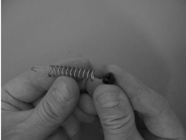
Figure 2-330 Reinstall the lifter assembly (500-sheet paper feeder)
