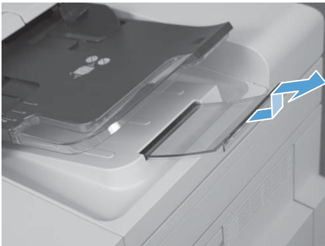
Figure 2-42 Remove the document feeder tray extender
