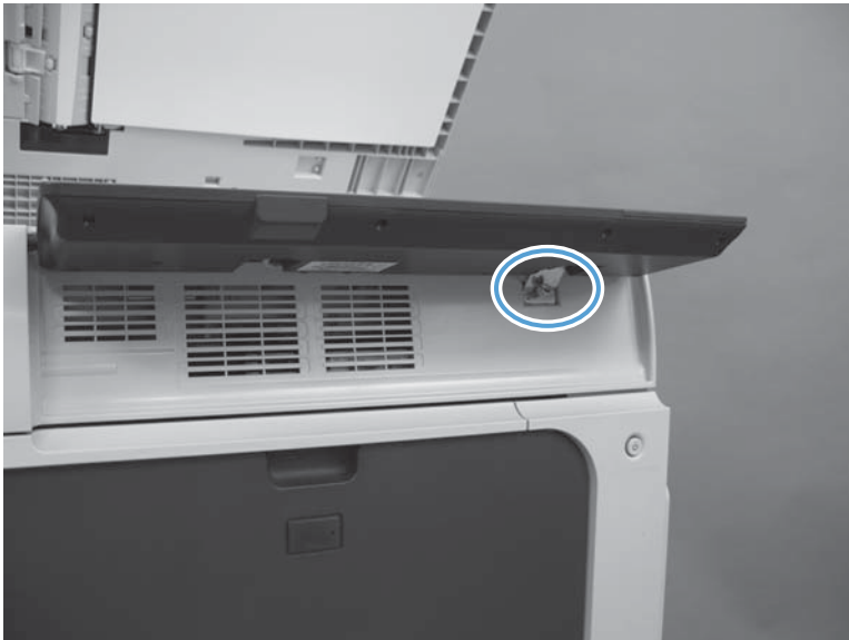
Figure 2-5 Remove the control panel (2 of 3)
