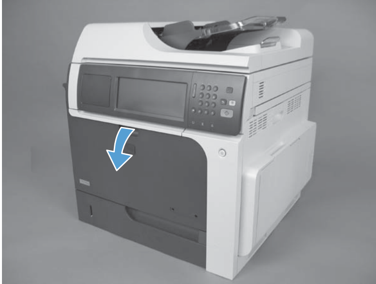
Figure 2-9 Remove the print cartridge (1 of 2)
