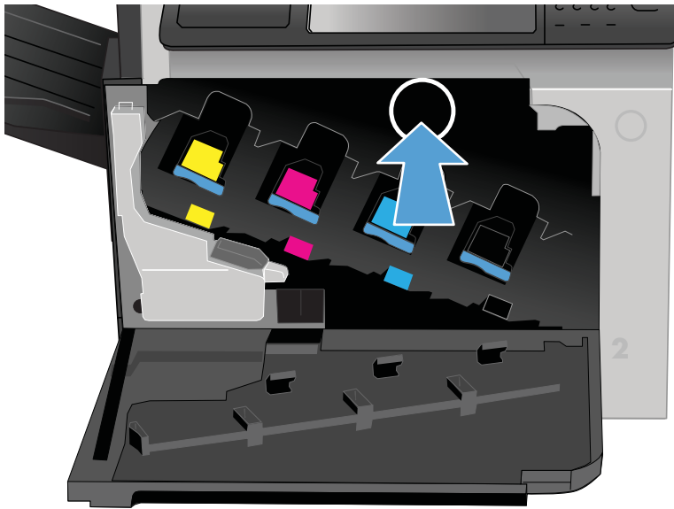
Figure 3-5 Test the front-door switch
