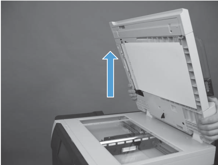
Figure 2-87 Remove the document feeder (3 of 3)
