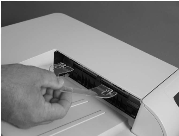
Figure 6-8 Remove the duplex-reverse guide (2 of 2)
