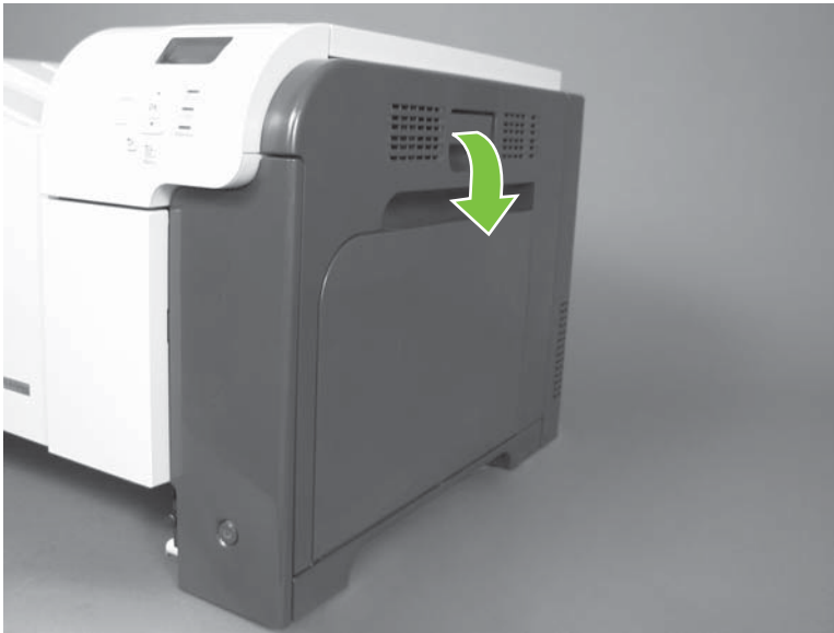
Figure 6-44 Remove the right-door assembly (1 of 8)
