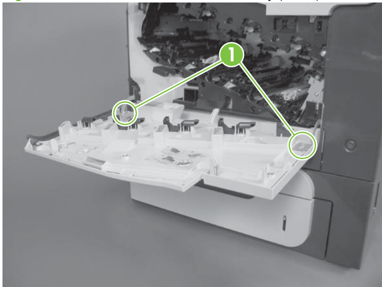
Figure 6-43 Remove the front-door assembly (2 of 2)
