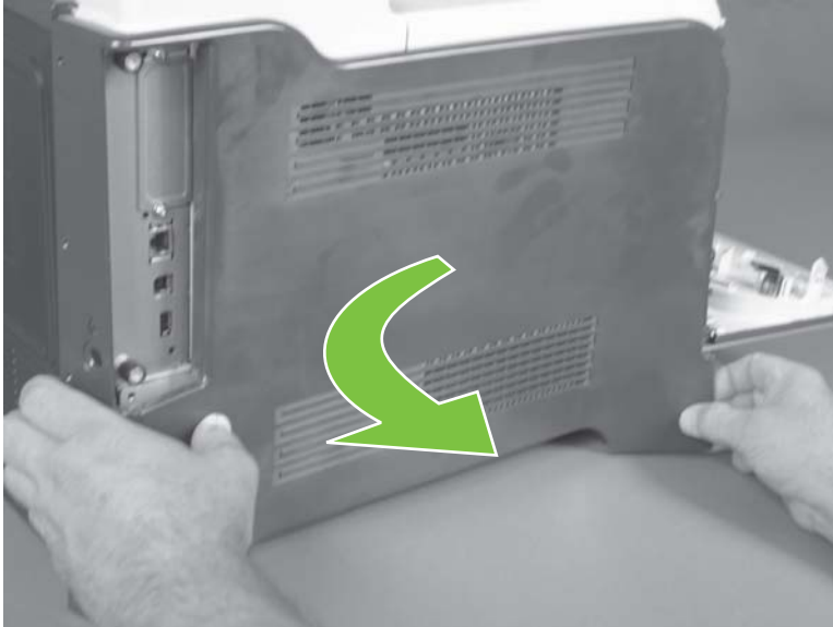
Figure 6-59 Remove the left cover (5 of 5)
