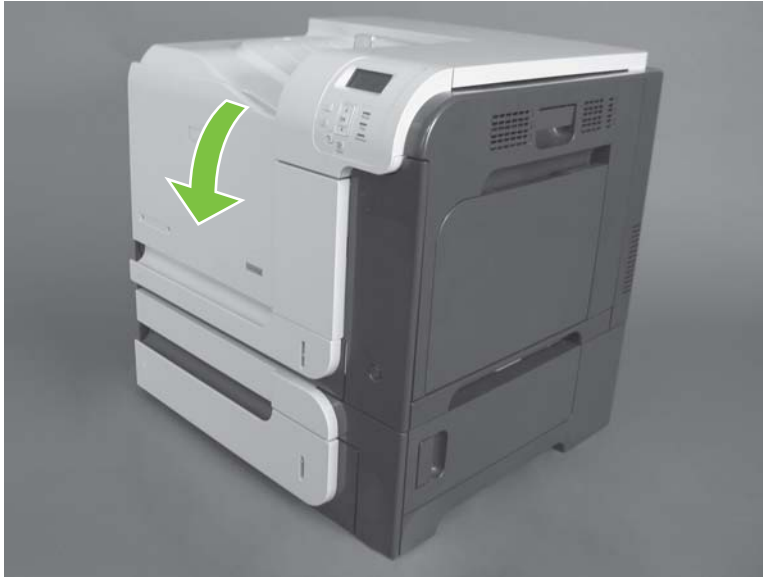
Figure 6-9 Remove the toner-collection unit (1 of 4)
