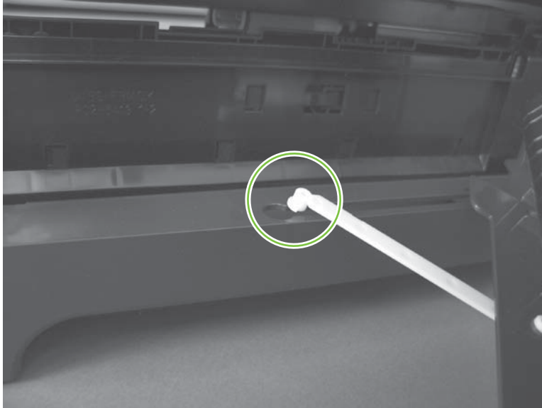
Figure 6-40 Remove the right door; optional paper feeder (3 of 3)
