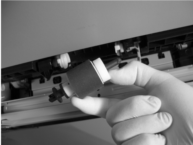
Figure 6-23 Remove the pickup roller (Tray 2) (4 of 4)
