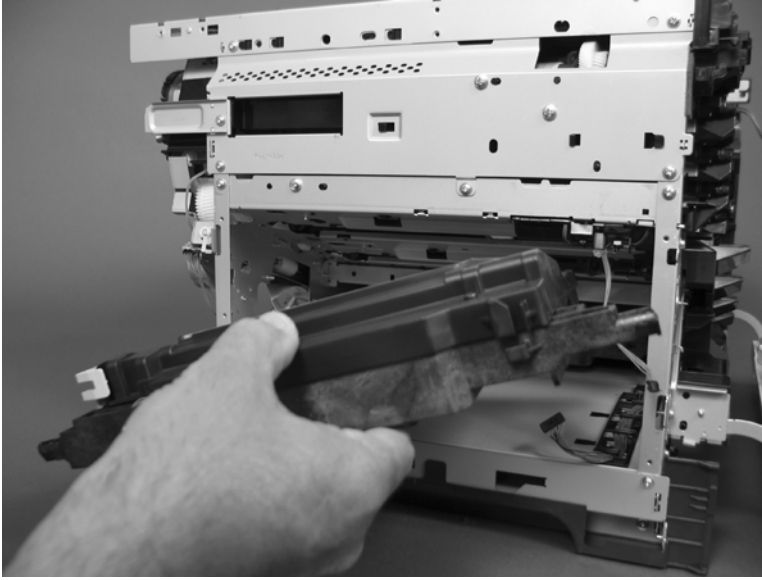
Figure 6-171 Remove the laser/scanner assembly (Y/M) (12 of 12)
