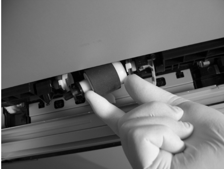
Figure 6-22 Remove the pickup roller (Tray 2) (3 of 4)
