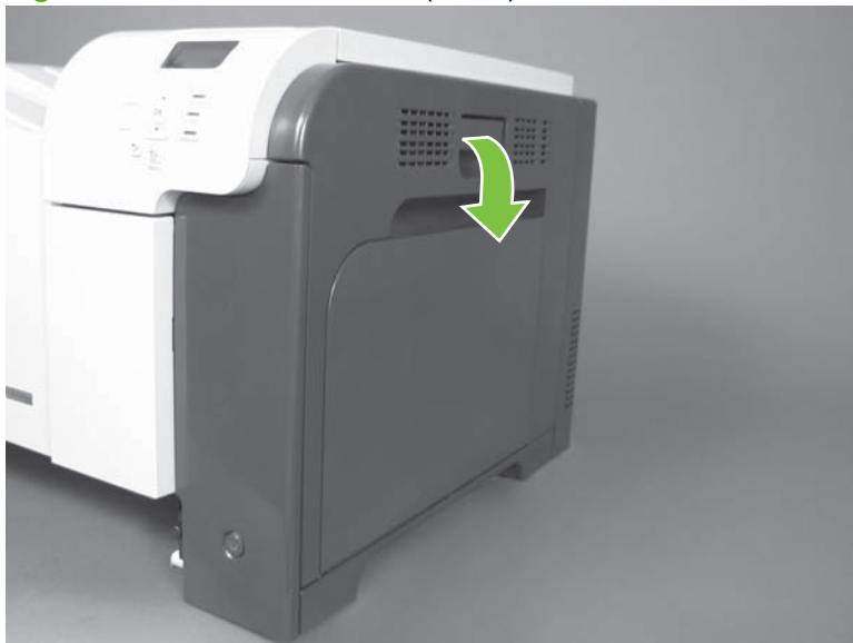
Figure 6-18 Remove the fuser (1 of 2)
