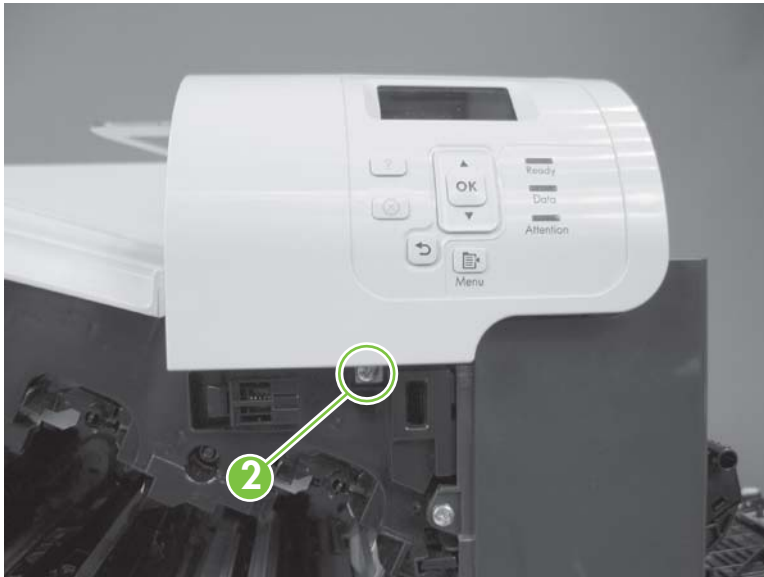
Figure 6-61 Remove the control-panel assembly (2 of 4)
