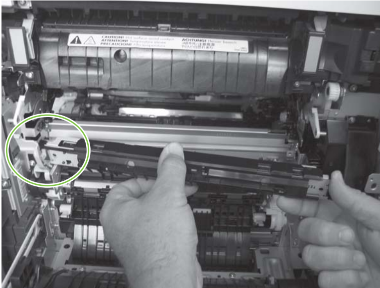
Figure 6-103 Remove the RD sensor assembly (3 of 6)
