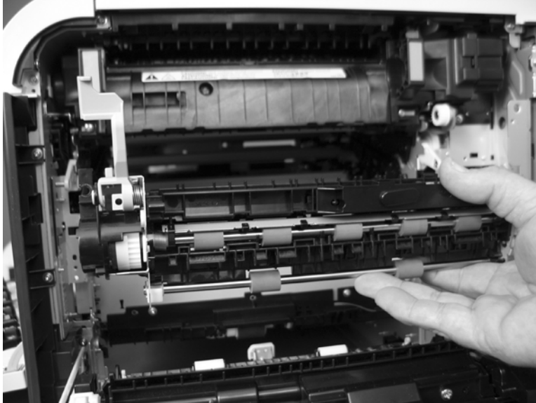
Figure 6-118 Remove the registration assembly (8 of 8)
