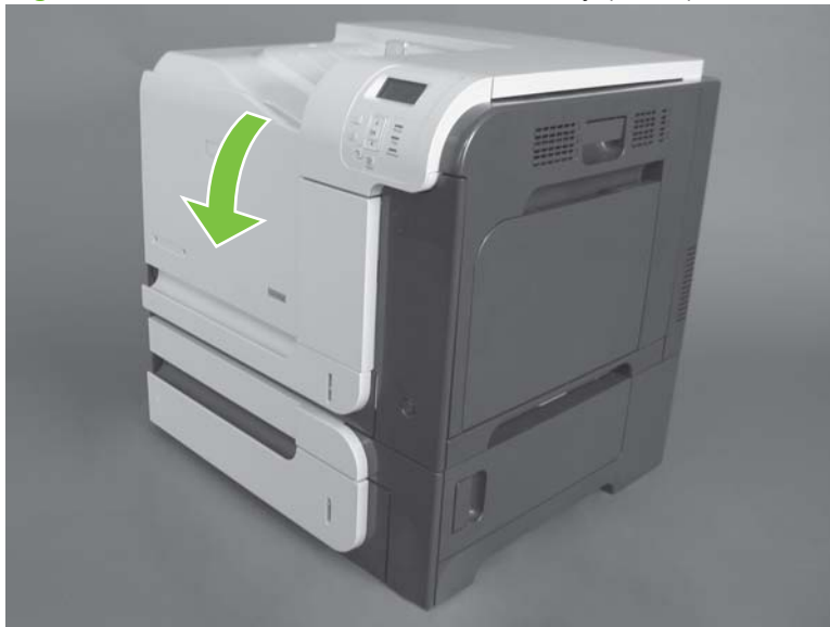
Figure 6-42 Remove the front-door assembly (1 of 2)
