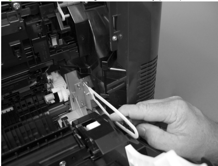
Figure 6-47 Remove the right-door assembly (4 of 8)
