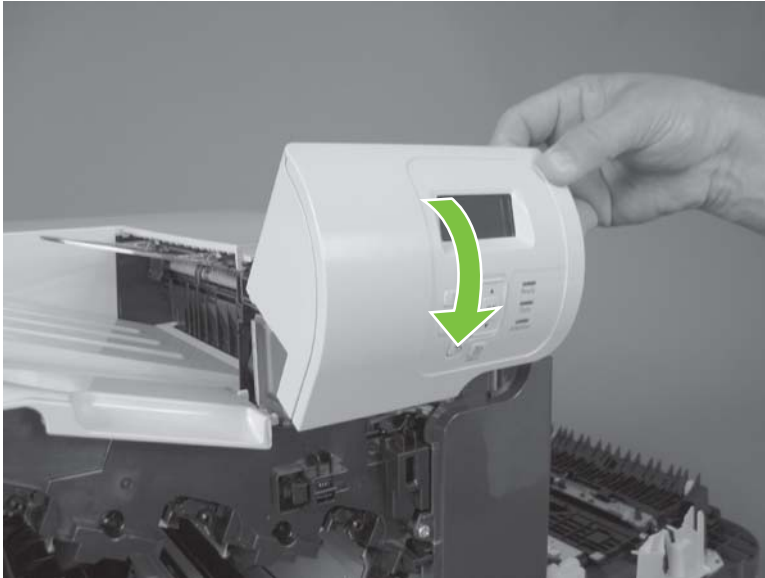
Figure 6-62 Remove the control-panel assembly (3 of 4)
