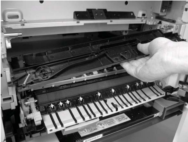
Figure 6-125 Remove the ITB duct (2 of 2)
