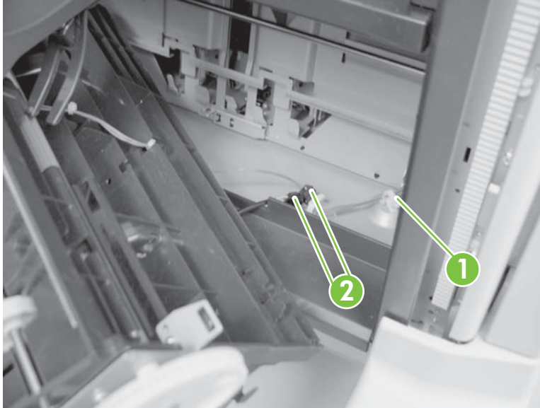
Figure 8-209 Remove the saddle delivery output bin (3 of 3)
