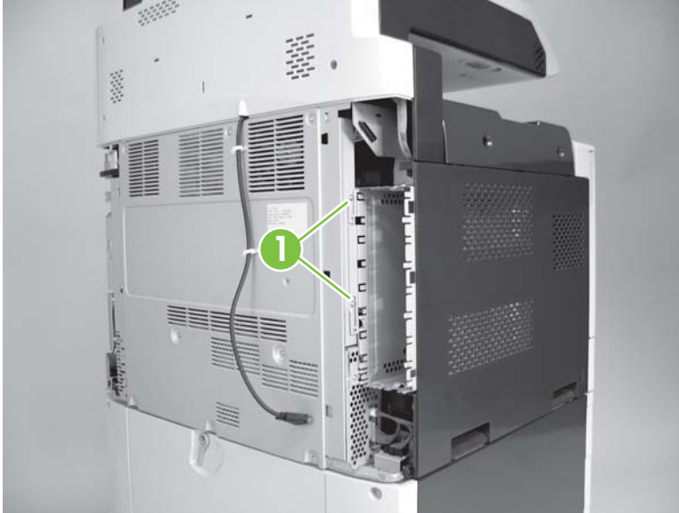
Figure 6-22 Remove rear cover (1 of 2)
