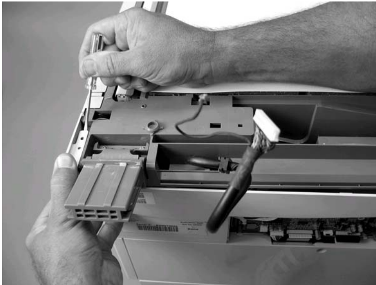
Figure 6-239 Remove the ADF rear end cover (4 of 5)
