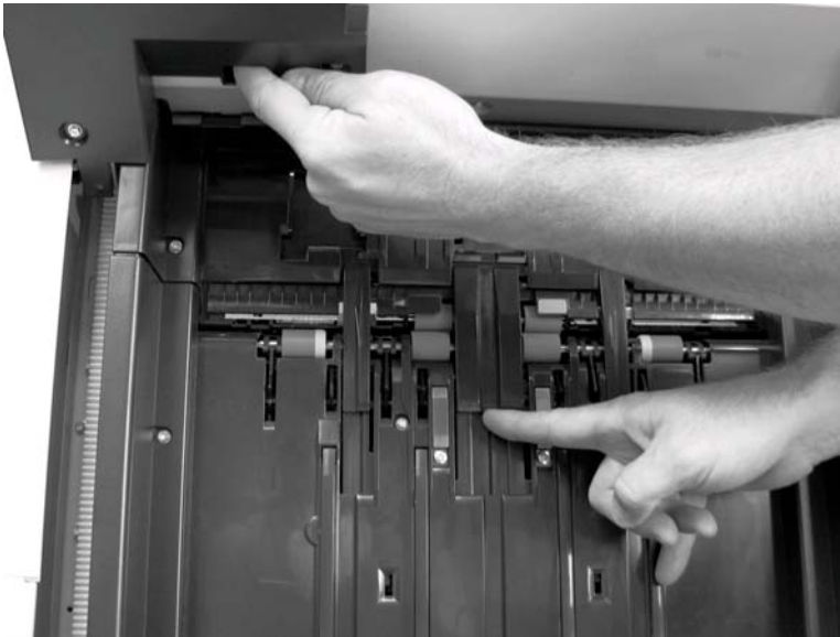
Figure 8-202 Remove output-bin 2 (3 of 3)
