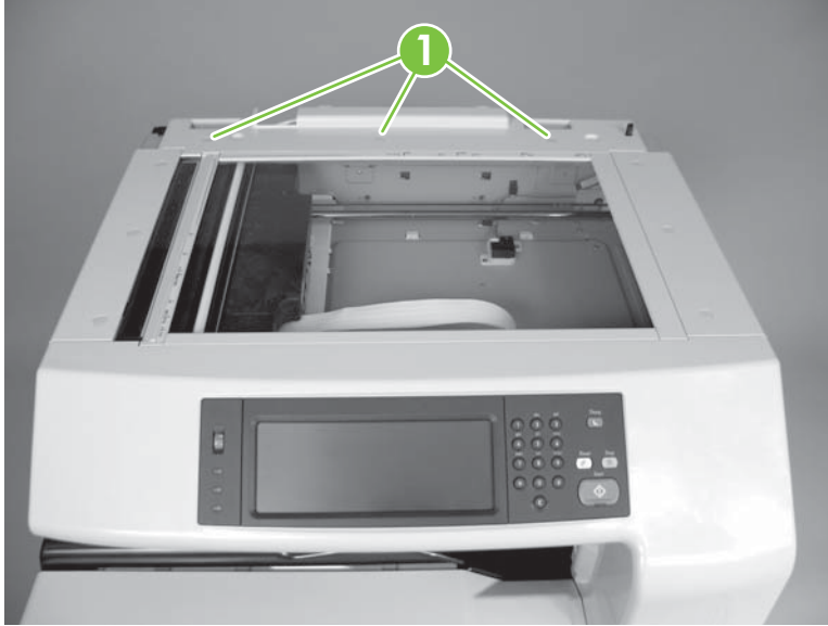
Figure 6-170 Remove top cover (1 of 2)
