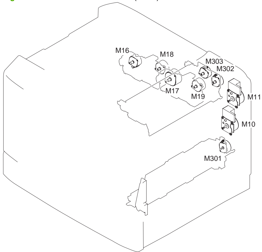
Figure 7-42 Product motor locations (2 of 2)
