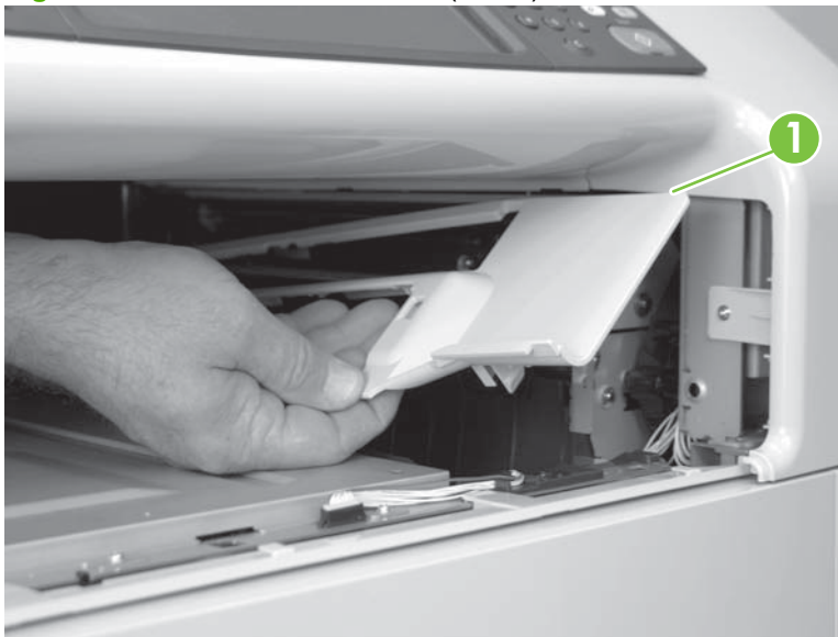
Figure 6-85 Remove inner cover (4 of 4)
