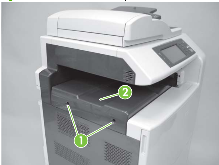
Figure 6-34 Remove face-down output bin
