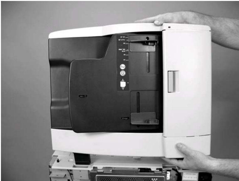
Figure 6-210 Remove the ADF assembly (4 of 4)
