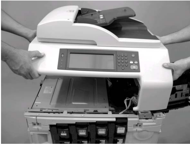
Figure 6-158 Remove optical scanner (6 of 7)
