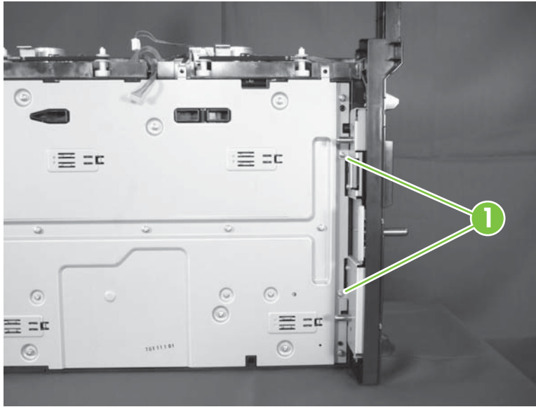
Figure 8-124 Remove the finisher lock-assembly (3 of 4)
