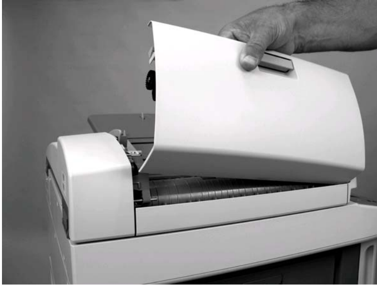
Figure 6-221 Remove the ADF jam cover (3 of 3)
