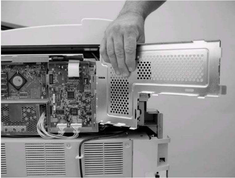
Figure 6-195 Remove SCB and CPB (1 of 5)
