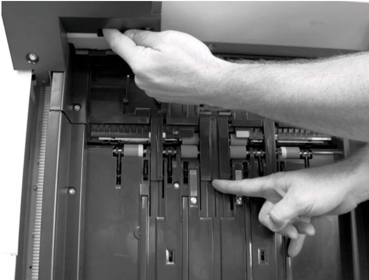
Figure 8-199 Remove output-bin 1 (3 of 3)
