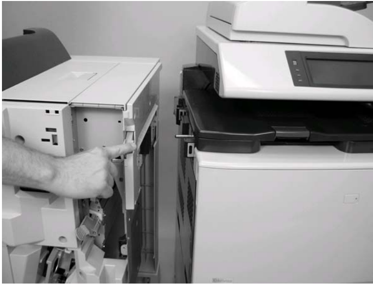
Figure 8-133 Remove output accessory (3 of 5)
