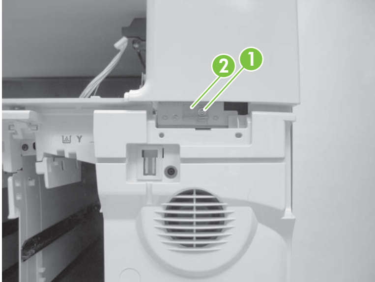
Figure 6-154 Remove optical scanner (2 of 7)
