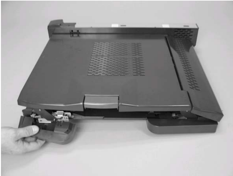
Figure 8-103 Remove upper guide assembly (2 of 5)
