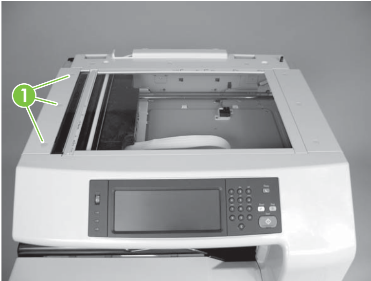
Figure 6-160 Upper-left scanner cover
