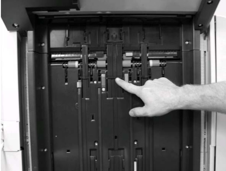
Figure 8-153 Move output bins (1 of 3)
