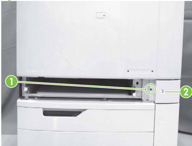
Figure 6-123 Remove front-lower cover
