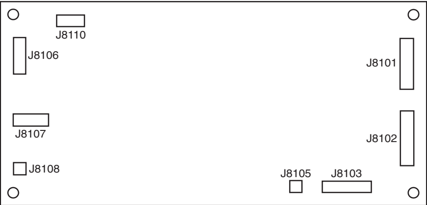
Figure 7-21 Input tray driver PCA
