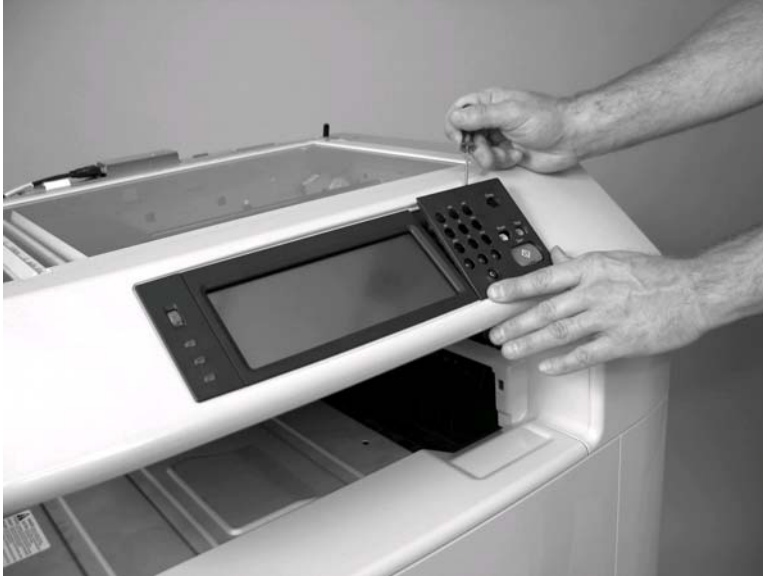
Figure 6-163 Remove control panel (2 of 3)
