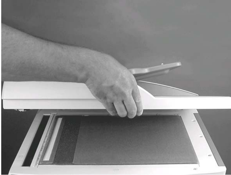
Figure 6-230 Remove the ADF white backing (3 of 4)
