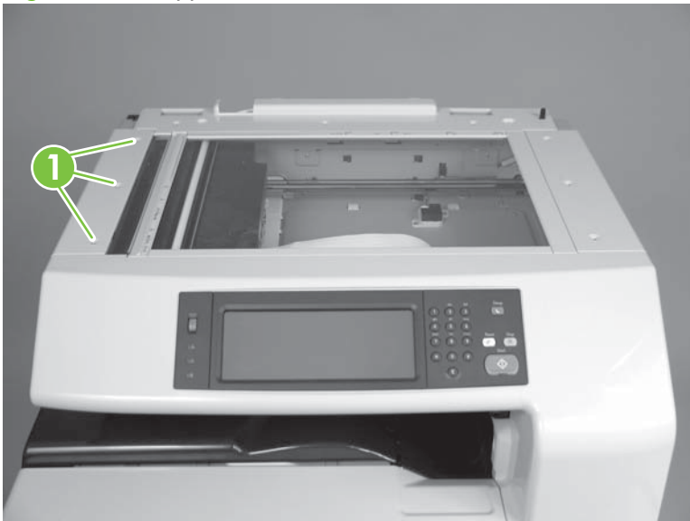
Figure 6-160 Upper-left scanner cover
