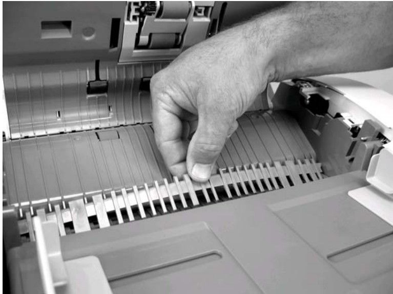
Figure 6-217 Remove the ADF diverter (1 of 2)
