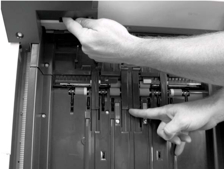
Figure 8-154 Move output bins (2 of 3)
