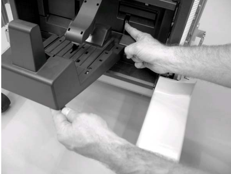
Figure 8-205 Remove booklet-delivery output bin (1 of 2)
