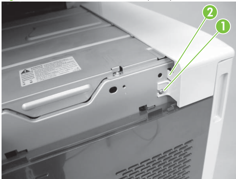
Figure 6-80 Remove front lower cover (1 of 2)
