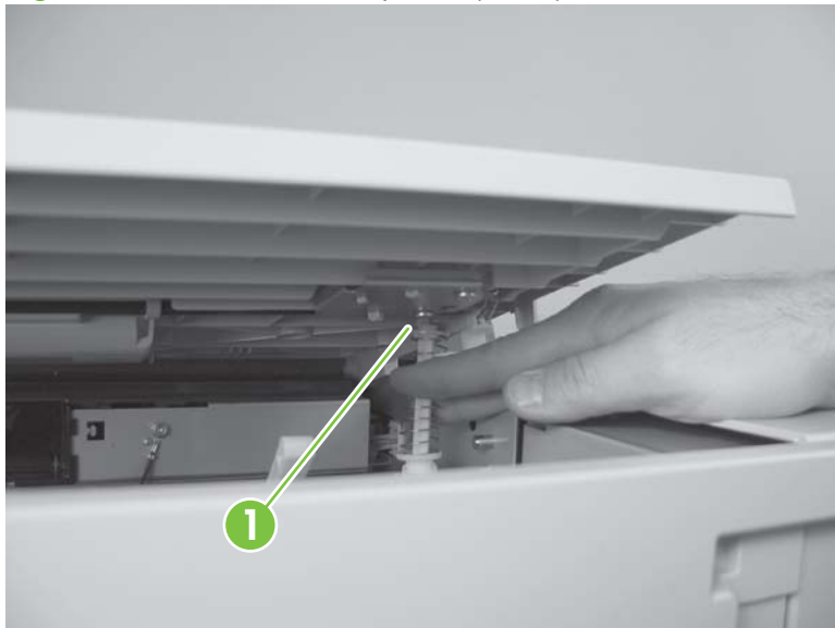
Figure 8-150 Remove the top door (2 of 3)
