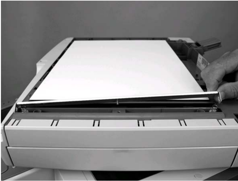
Figure 6-225 Remove the ADF float assembly (3 of 5)
