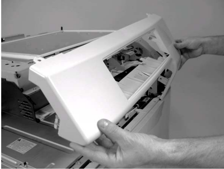
Figure 6-166 Remove front cover (2 of 2)
