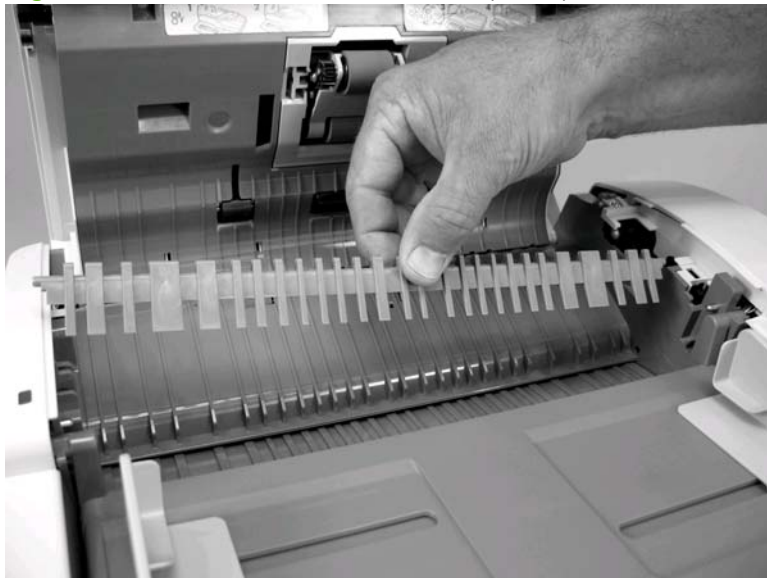
Figure 6-218 Remove the ADF diverter (2 of 2)
