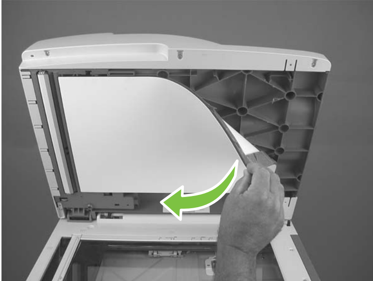
Figure 6-228 Remove the ADF white backing (1 of 4)
