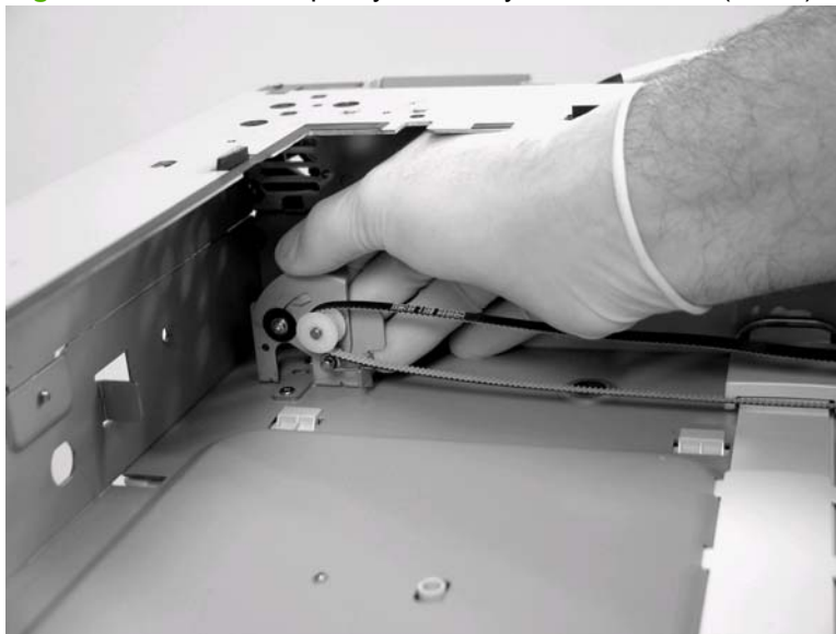
Figure 6-185 Remove pulley assembly and motor unit (3 of 5)
