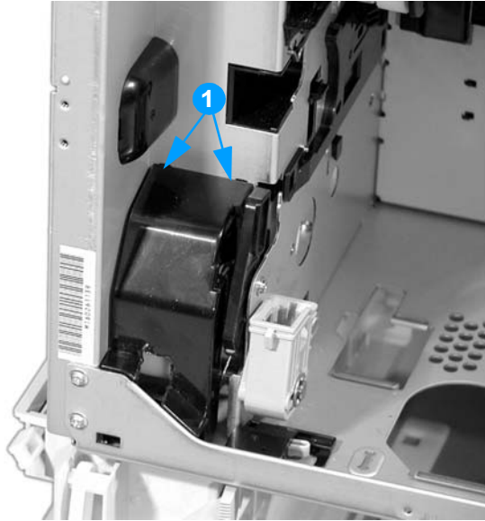
Figure 6-37 Removing and replacing the drum drive assemblies (1 of 4)
