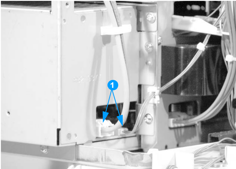
Figure 6-49 Removing and replacing the low-voltage power supply, left side of printer (1 of 4)
