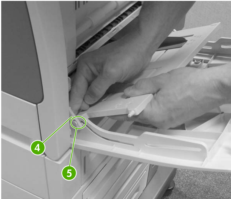
Figure 6-20 Remove the multipurpose tray (4 of 7)
