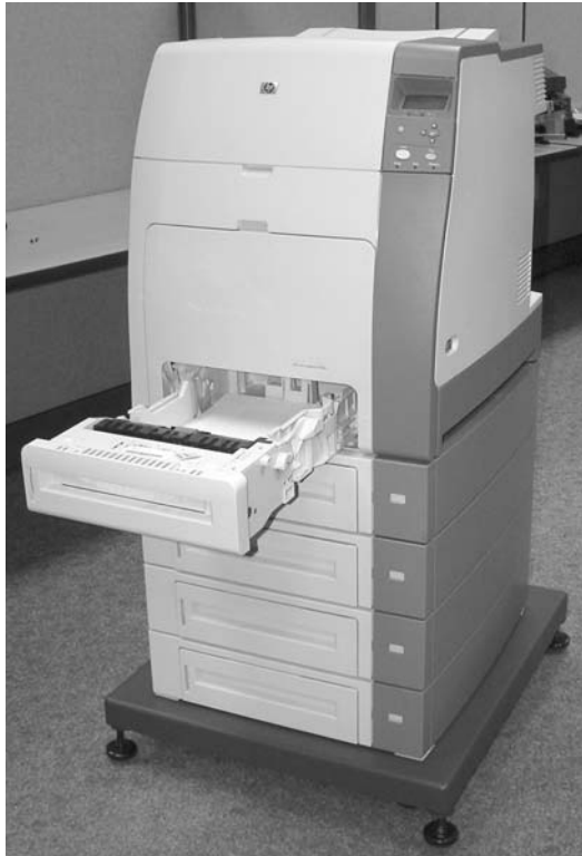
Figure 6-16 Remove the paper tray
