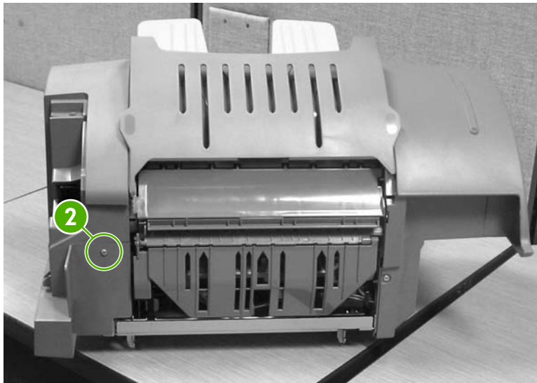
Figure 6-175 Remove the left cover (2 of 2)
