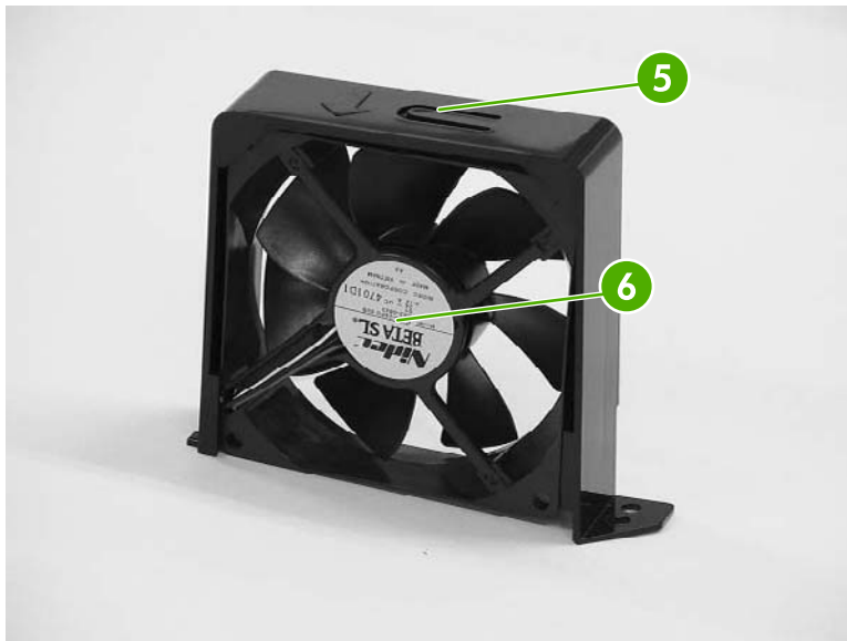
Figure 6-121 Remove the upper exhaust fan (2 of 3)
