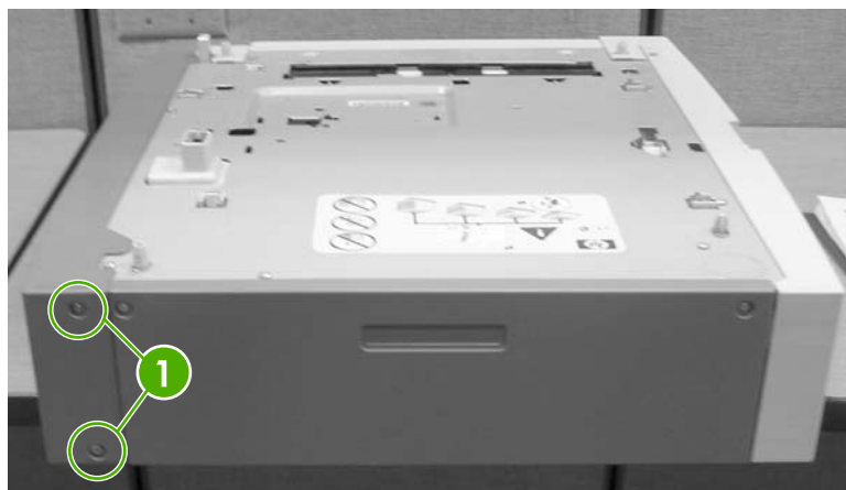
Figure 6-150 Remove the right cover (1 of 2)
