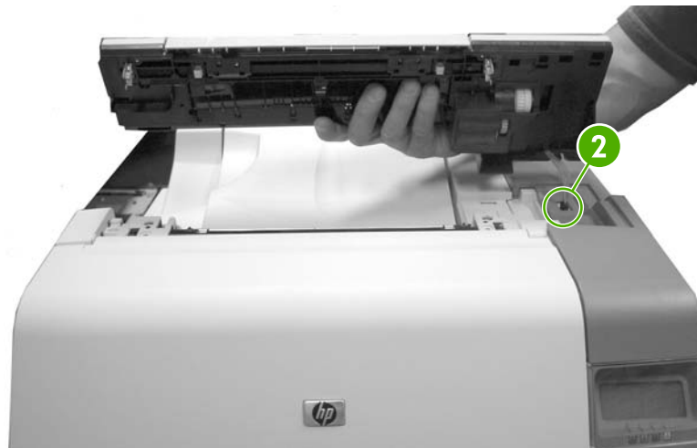
Figure 6-187 Remove the top duplexing assembly (2 of 2)
