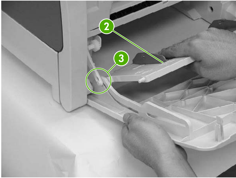
Figure 6-19 Remove the multipurpose tray (3 of 7)
