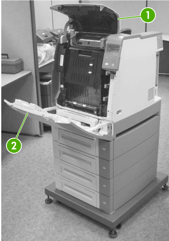
Figure 6-24 Remove the front cover (1 of 6)
