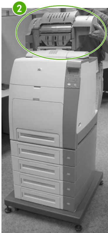
Figure 6-171 Remove the stapler/stacker from the printer (2 of 2)
