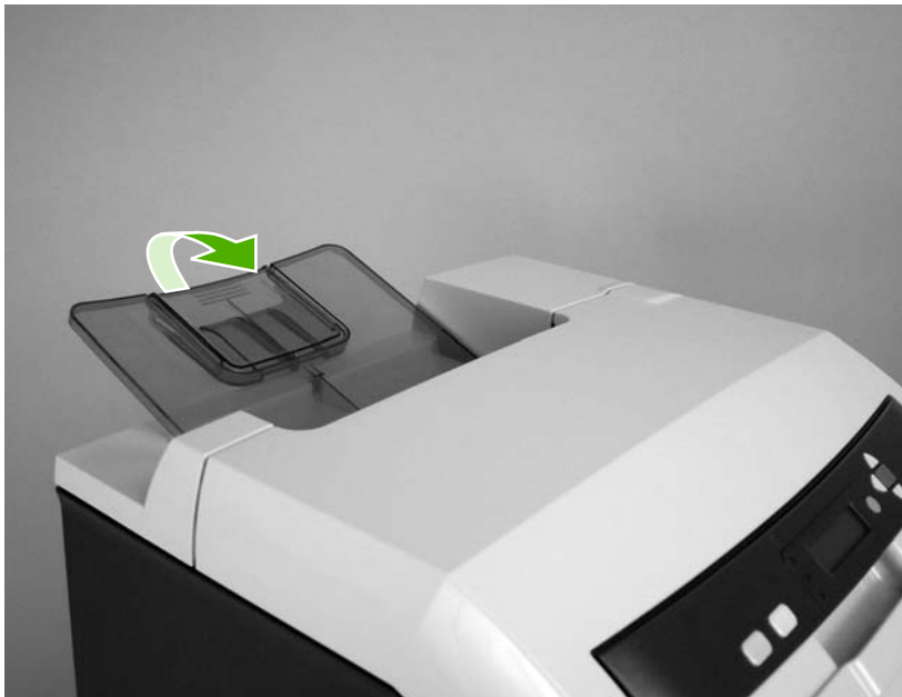
Figure 5-11 Remove the upper cover (1 of 5)
