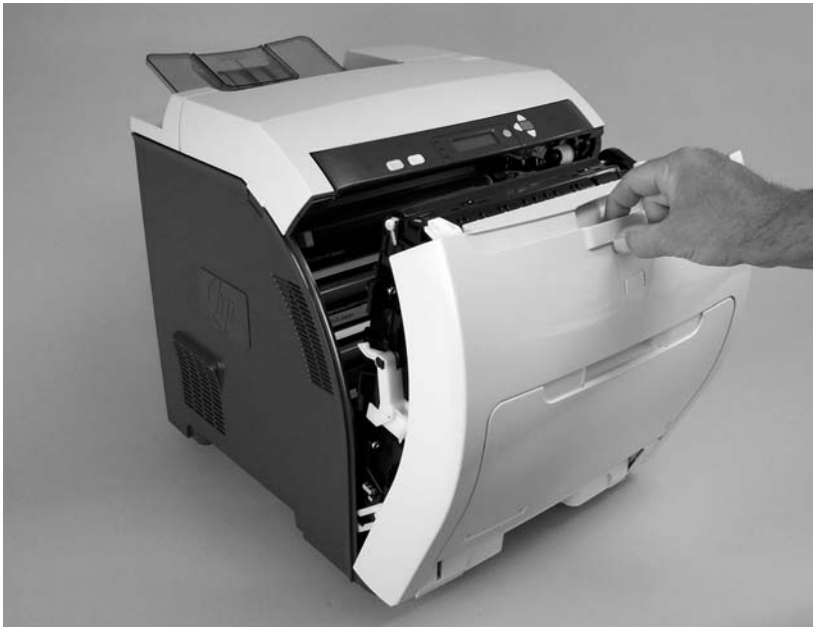
Figure 5-2 Remove the print cartridges (1 of 2)
