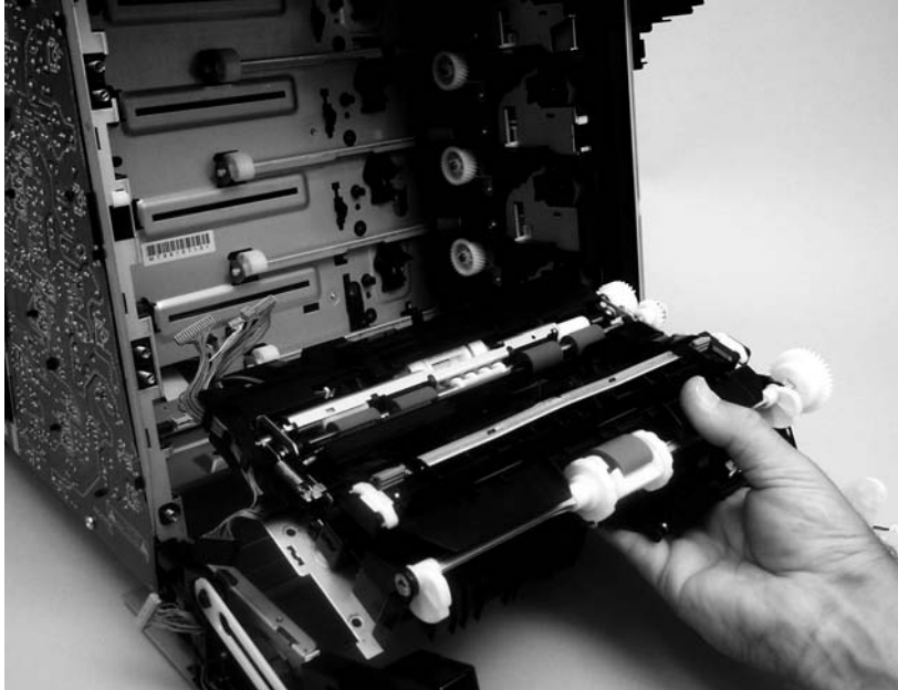
Figure 5-57 Remove the pickup-and-feed assembly (8 of 8)
