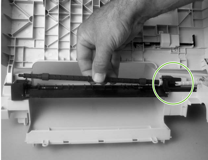
Figure 5-36 Remove the duplex-reverse-drive assembly (2 of 5)
