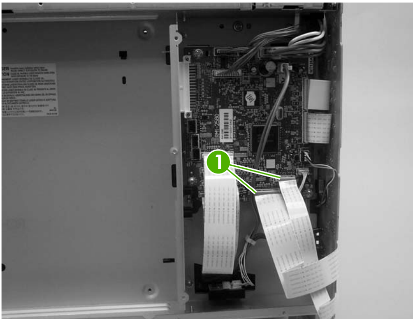
Figure 5-88 Remove the high-voltage power supply (1 of 3)
