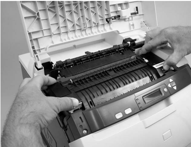
Figure 5-12 Remove the upper cover (2 of 5)
