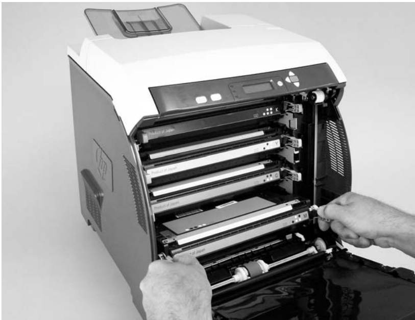
Figure 5-3 Remove the print cartridges (2 of 2)
