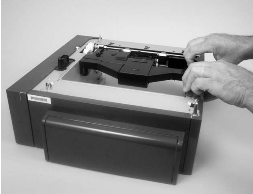
Figure 5-115 Remove the 500-sheet feeder left cover (2 of 5)
