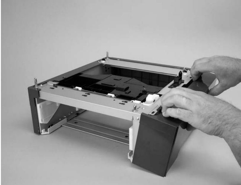
Figure 5-112 Remove the 500-sheet feeder right cover (2 of 3)
