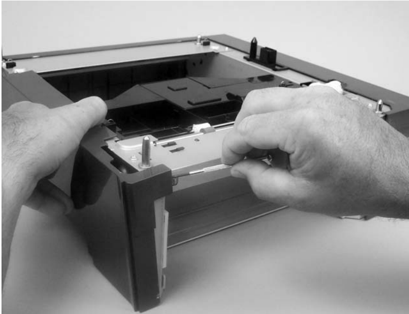
Figure 5-116 Remove the 500-sheet feeder left cover (3 of 5)
