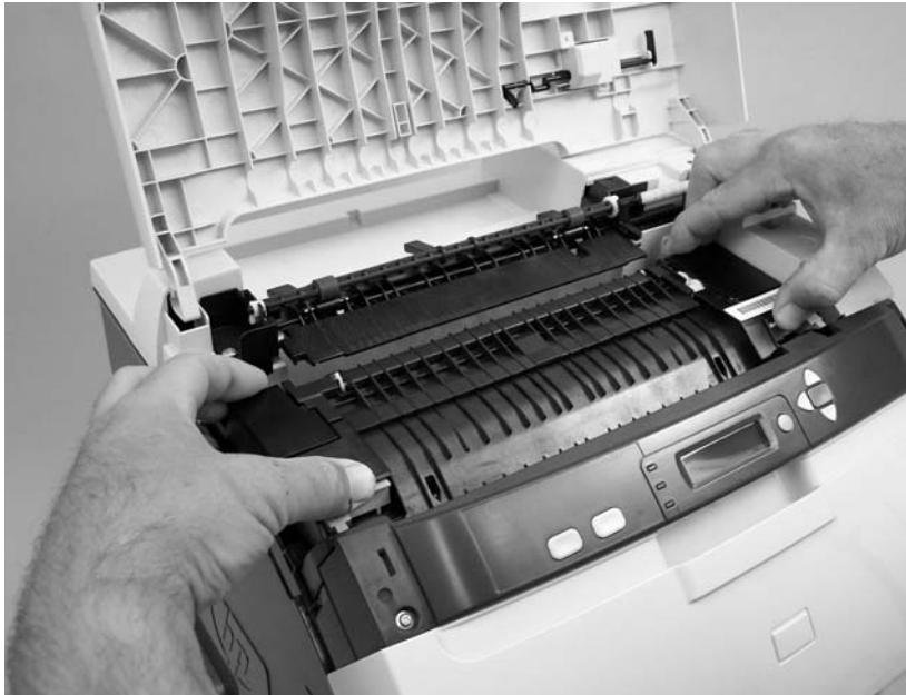
Figure 5-30 Remove the fuser
