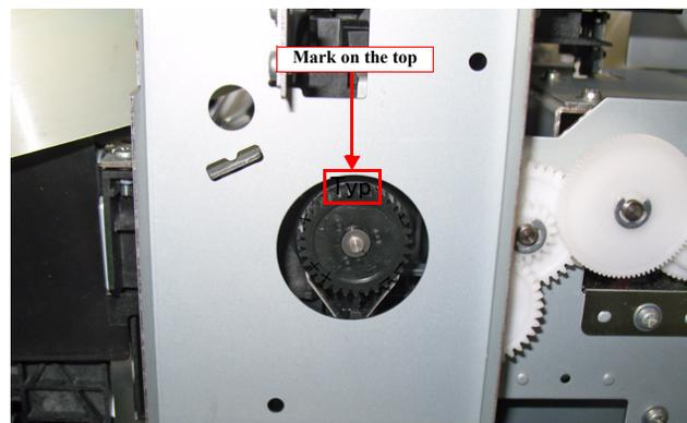
Figure 4-31. APG cam position checking point
