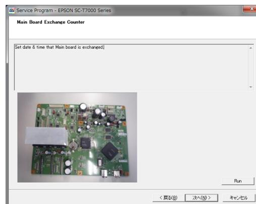
Figure 4-75. [Main Board Exchange Counter] Screen
