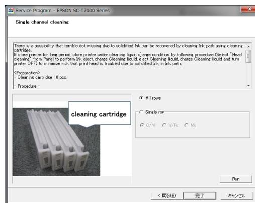
Figure 4-55. [Single channel cleaning] Screen
