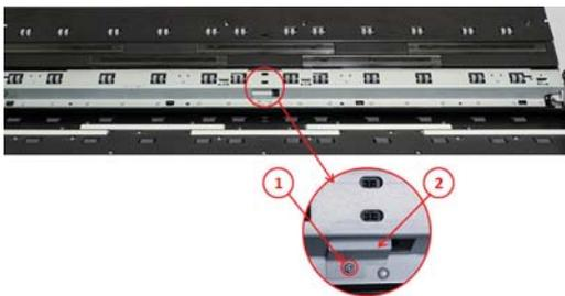
6. Open the CIS unit. See [Scanner Controller Unit \(SUP\) on page 328](#).
