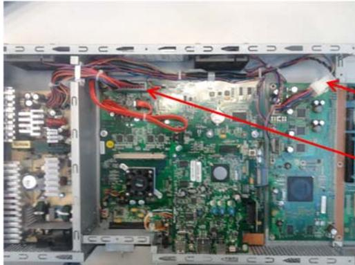
3. Unroute the cables and remove one T-10 screw.
