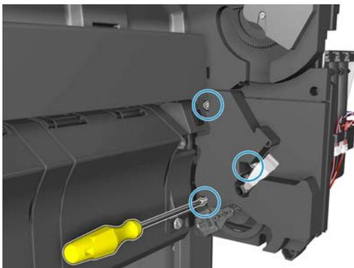
6. Remove the bottom tip support.
