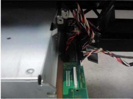
6. Remove the E-Box from the printer.
