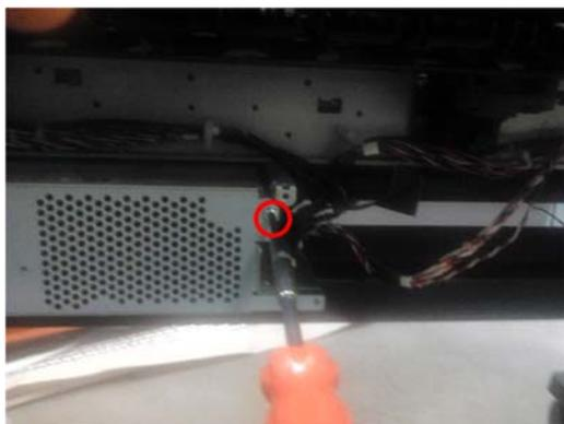
4. Remove the front panel cable and the T-10 screw.
