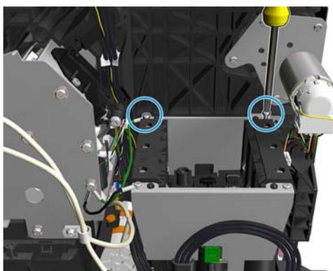
4. Remove the bracket and side plate.
