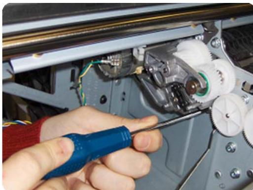
3. Loosen the encoder sensor adjustment screw.
