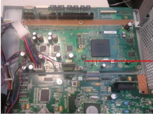
**⚠ WARNING!** If the engine PCA is not removed before the formatter, the bridge connections may be damaged.
