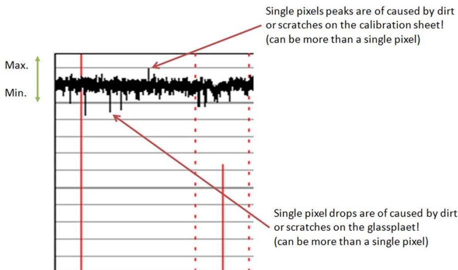
Peaks will show up in a scan as a lighter color and not necessarily in all colors, it depends on which color channels are being affected by the dirt/ scratch.
