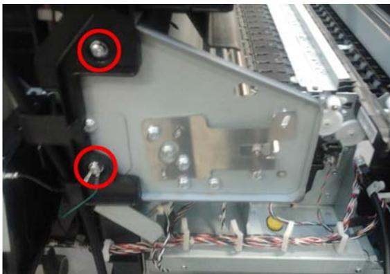
8. Remove the Scan Axis Motor. See [Scan Axis Motor on page 244](#).
