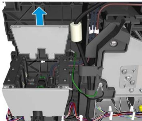
5. Remove 2 screws and the side plate.
