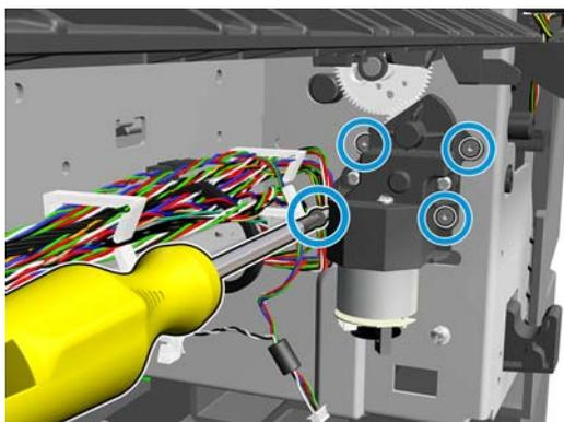
4. Remove the valves motor.
