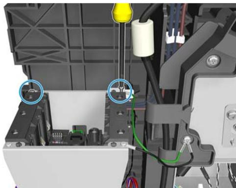
4. Remove the bracket and side plate.
