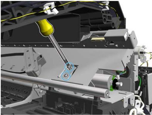
10. Slide out the auto pinch lifter, and disconnect the sensor.
