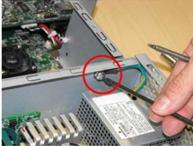
6. Remove the power supply unit.
