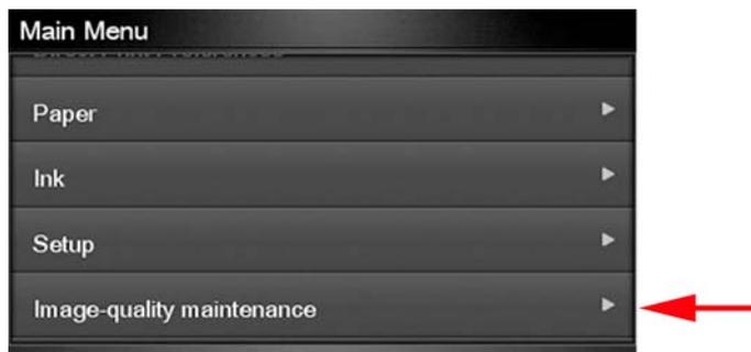
4. From the Image-quality maintenance menu, scroll down and select the **Scanner IQ plot** to print.
