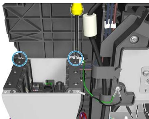
4. Remove the bracket and side plate.
