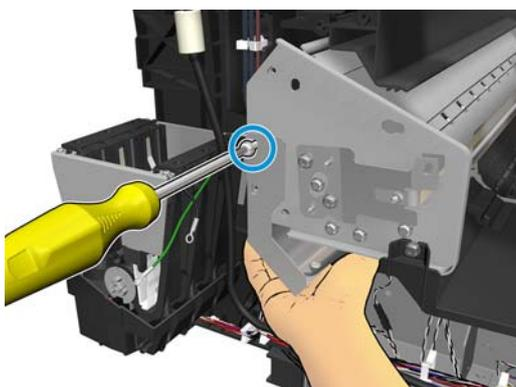
**8. Remove the Scan Axis Motor.**
