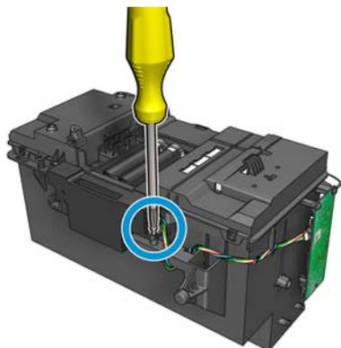
4. Remove the Drop Detector from the service station.
