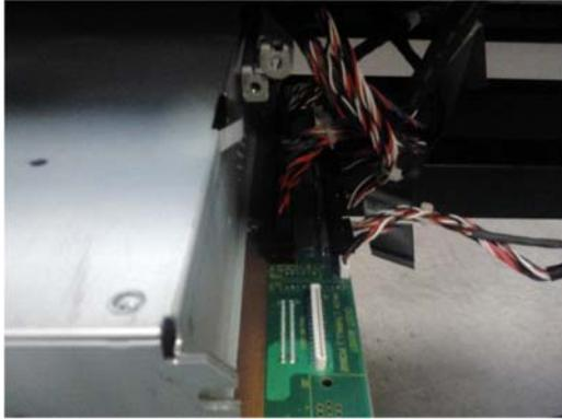
6. Remove the E-Box from the printer.
