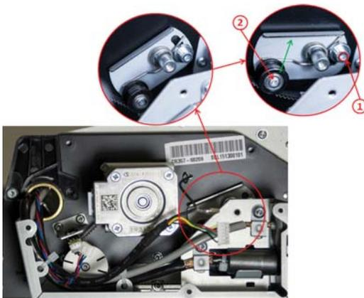
7. Remove the motor screws.
