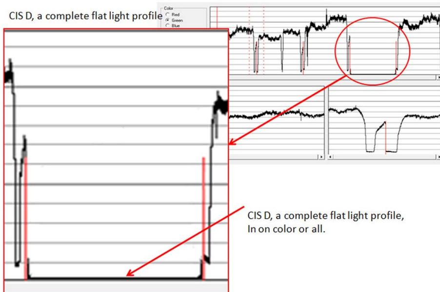
A completely flat light profile in one color or all colors can either be one specific LED or the entire CIS module that is faulty.
