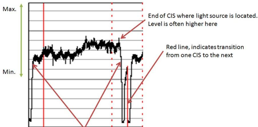
A drop in the light level in the active part of the CIS is often caused by dirt or scratches on the glass plate
