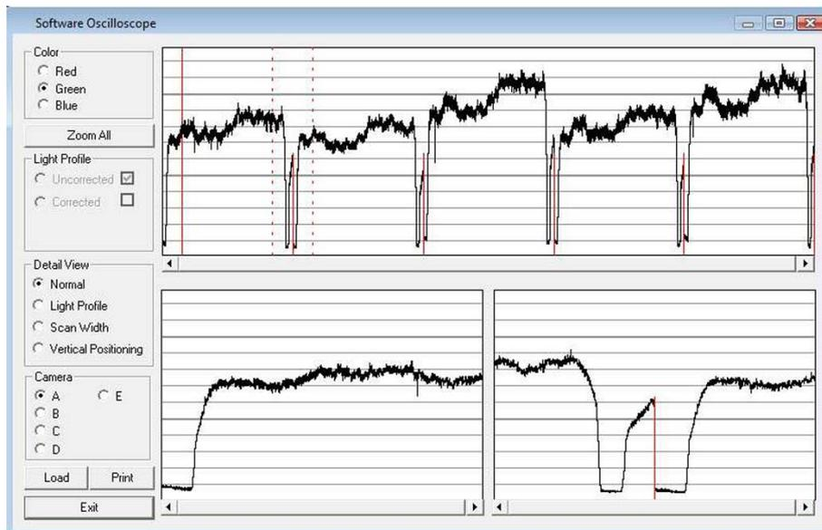
The Adjusted light profile is corrected according to the calibration sheet, in other words, the calibration sheet has been used as a reference to correct the imperfection of the CIS elements.
