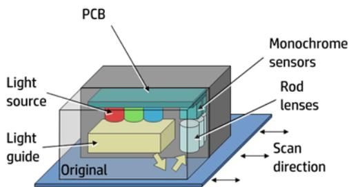
The purpose of the lens is to channel the light from the “pixels” on the image to the sensors. There is no magnification in the lens (1x1).
