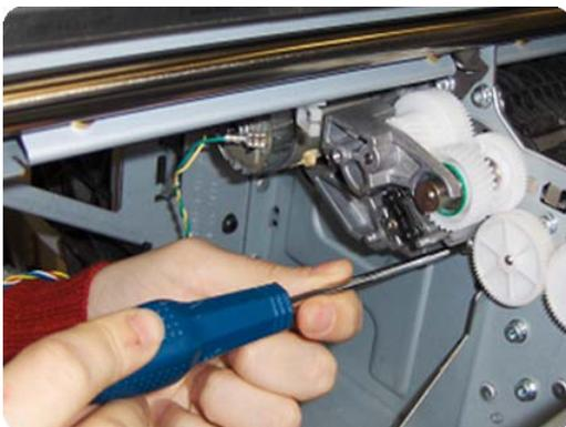
3. Loosen the encoder sensor adjustment screw.
