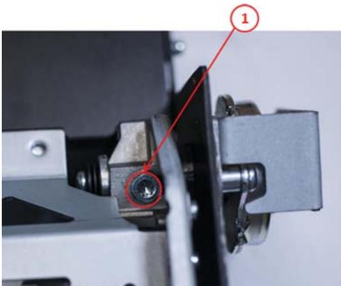
5. Tilt open the CIS bridge to decrease the spring tension (1), and remove CIS damper (2).
