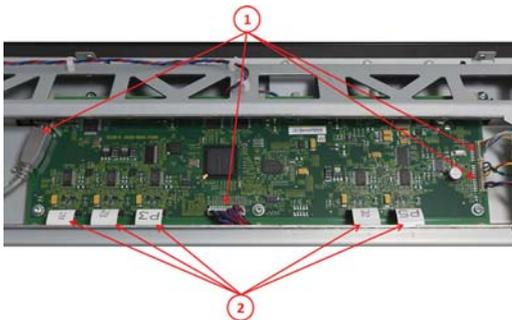
4. Remove the Screws (Torx 10), and remove the Scanner Controller Board.
