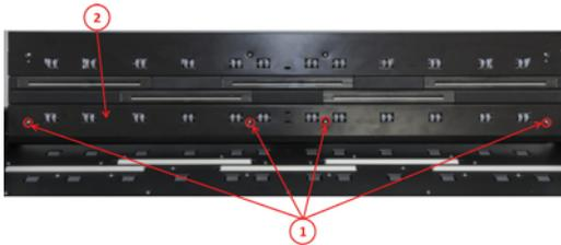
5. Remove the screw (1), and the sensor bracket (2).
