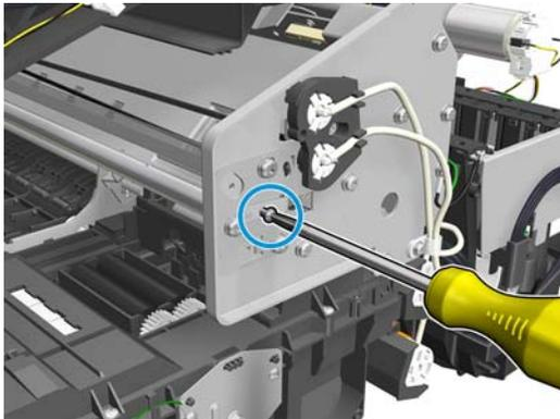
4. Press the bracket to release the encoder strip tension.
