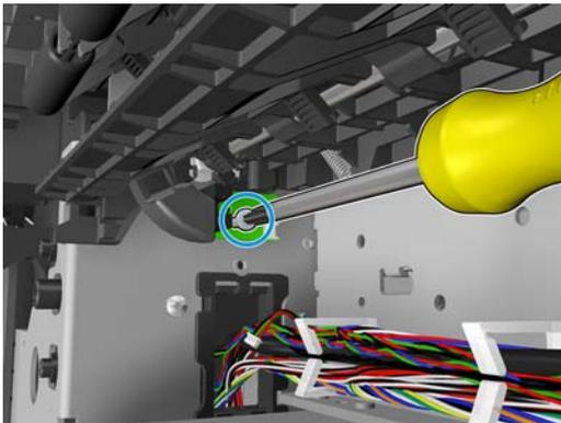
5. Remove the sensor valves.
