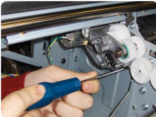
4. Position the Media Advance Drive Adjustment Tool on the end Media Advance Roller shaft, push it firmly onto the shaft and maintain a constant pressure to ensure it is flush to the Media Advance Drive.
