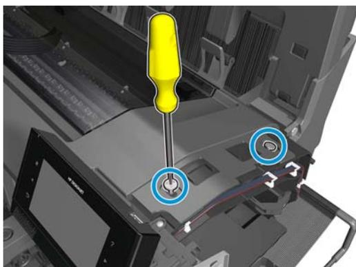
6. Lift up the center cover, and remove it from the printer.
