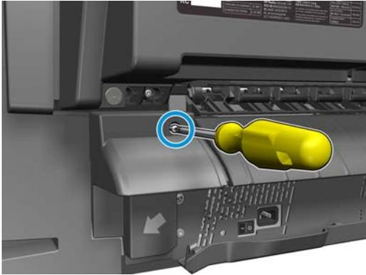
2. Remove the arch sidewall cover from the front panel side.
