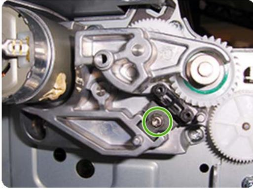
4. Add the Encoder Sensor Tool to the Media Drive Adjustment Tool.
