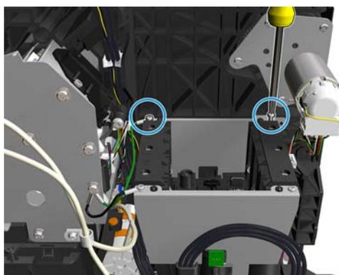
4. Remove the bracket and side plate.
