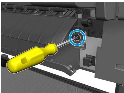
3. Remove the output platen.
