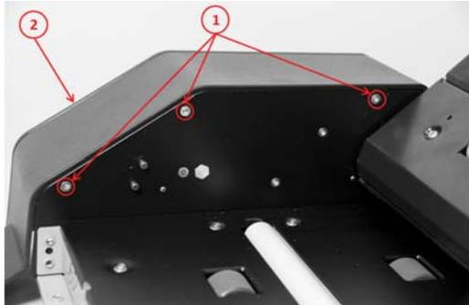
3. Remove the screws (1), and then the motor cover (2).
