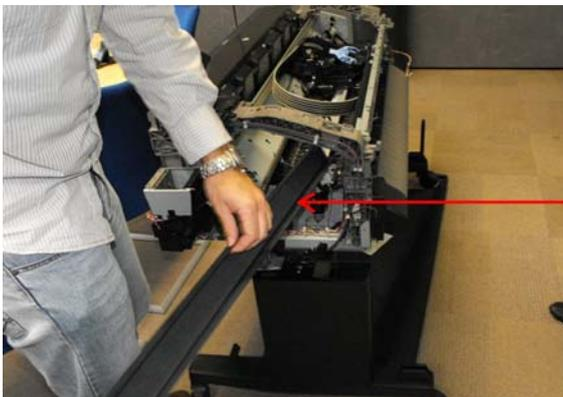
11. Remove 5 screws and the printheads.
