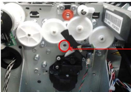
2. Install the new gears that came with the kit reversing the removal process.
