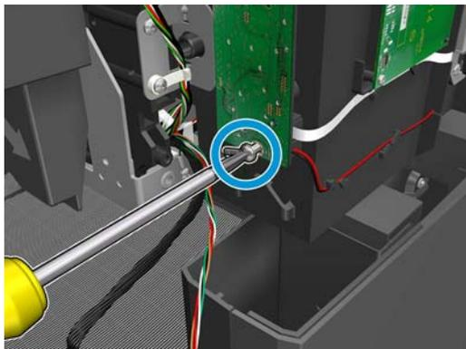
5. Remove the 2 allen screws from the Slider Rod.
