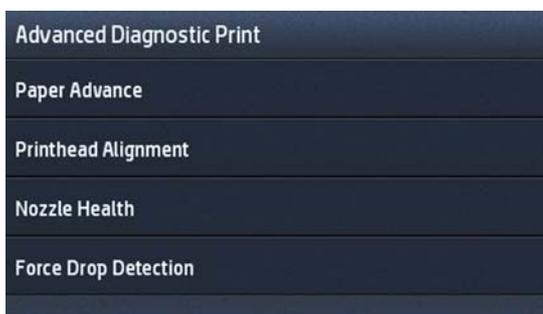
All the diagnostic Prints (except **Force Drop Detection**) require that the printer be ready to print (paper loaded, printhead and supplies installed). At the beginning of each diagnostic, you will see the following screen:
