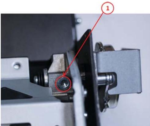
5. Tilt open the CIS bridge to decrease the spring tension (1), and remove CIS damper (2).
