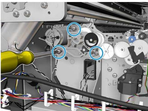
7. Remove the paper axis motor.
