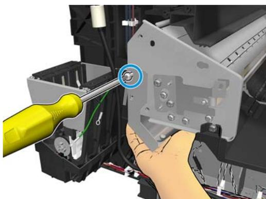
**8. Remove the Scan Axis Motor.**
