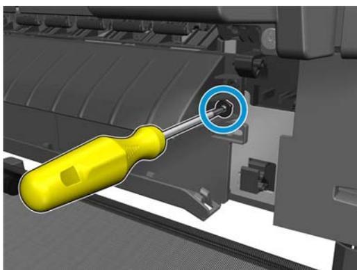
3. Remove the output platen.
