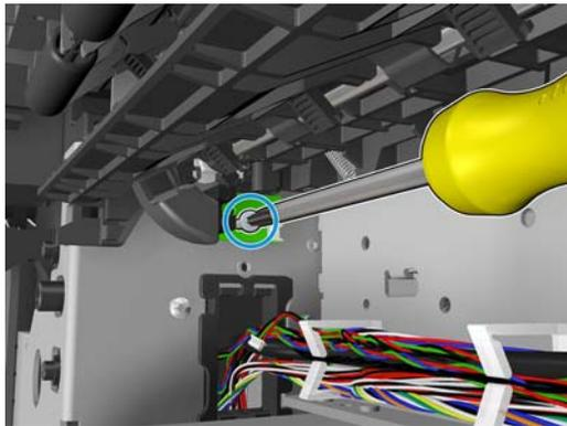
5. Remove the sensor valves.
