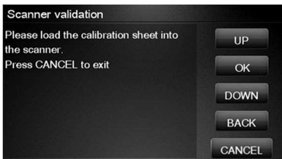
4. Hold the calibration sheet from both sides and place it facing the arrow in the centre of the sheet in front of the Page icon present on the input tray of the scanner. Push the sheet with both hands on both sides at the same time to load the sheet with no skew. Press OK to continue with the test.
