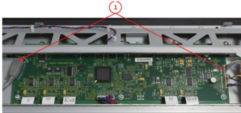
4. Unclip the USB Cable and pull it gently out of the CIS bridge (1). Remove the screws and unclip the cable (2).
