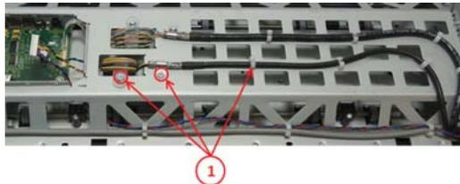
3. Cut the cable tie, and push the cable into the CIS unit.
