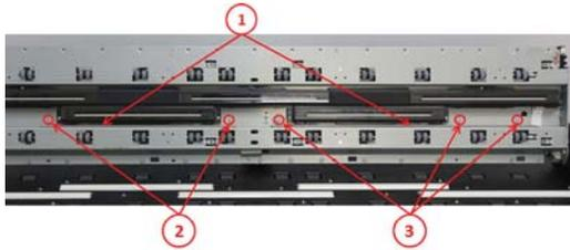
4. Unplug only the FFC cables that need to be replaced.
