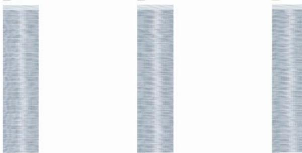
The most uniformly centered will be the white/lightest band; better the media advance the printer has.
