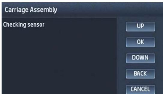
6. After the line sensor has been checked, you're asked to insert the printheads again. To do so, open the printer window, open the carriage cover, and insert the printheads into the carriage. Then, close the carriage cover, printer window, and then press **OK**.
