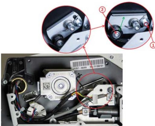
7. Remove the motor screws.
