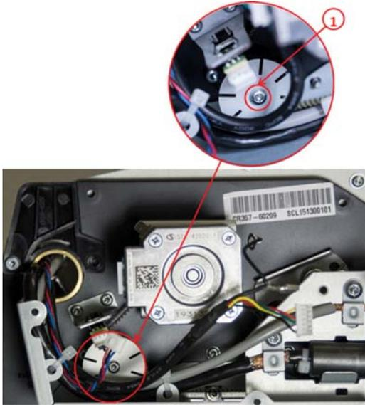
6. Release belt tension by loosening the screw (don't remove it), and push the tension wheel upwards and tighten the screw.
