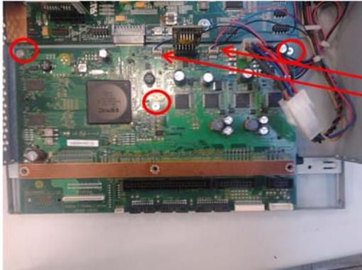
3. Slide out and remove the engine PCA (which is connected to the formatter PCA).
