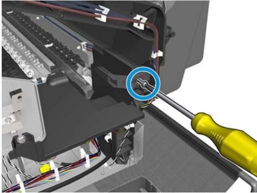
3. Remove the bump cutter actuator.
