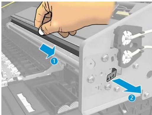
5. Remove 2 screws, and remove the primer tubes.
