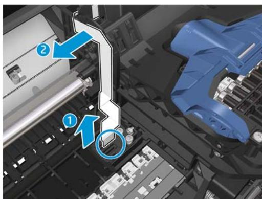
3. Unclip the mylar, and disconnect trailing cable.
