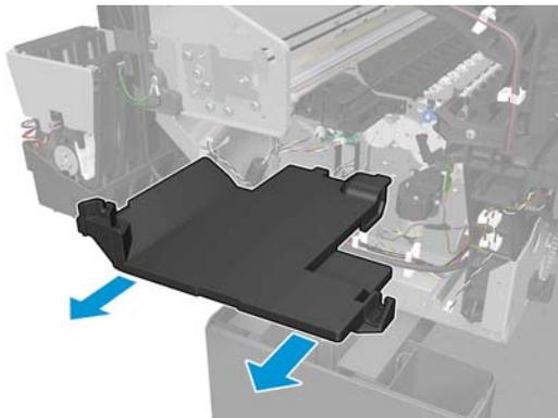
3. Remove the first starwheel rail. See [Customer Self Repair Flyers on page 353](#).
