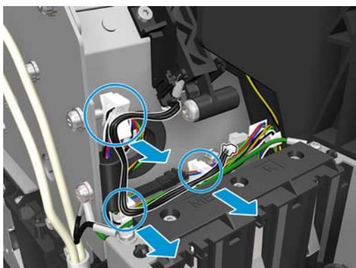
3. Remove the 2 T-20 screws, and the PRS actuator.
