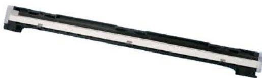
2. Remove the CIS tiles, and mark them for repositioning if necessary.
