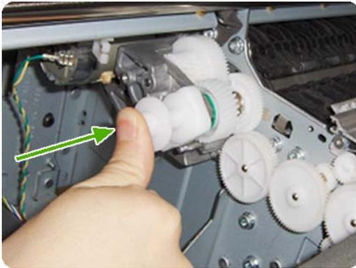
5. While maintaining pressure on the Media Advance Drive Adjustment Tool, fully tighten the three T-15 attachment screws in the order shown.
