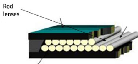
Due to the very short focal length, the focus depth is limited. The original has to be in contact with the surface of the glass plate in order to be in focus.
