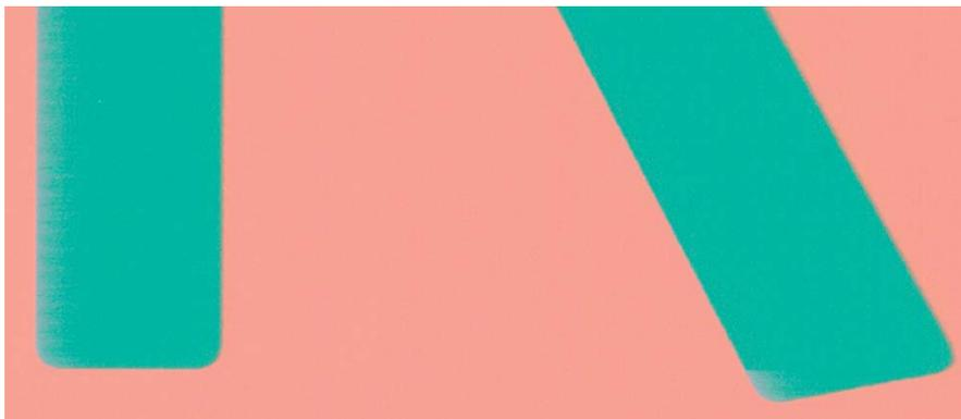
If edges of objects or lines appear to be poorly defined or lighter in density, and you have already set the print-quality slider to **Quality** in the driver dialog, select the custom print-quality options, and try setting the quality level to **Normal**. See users guide.
