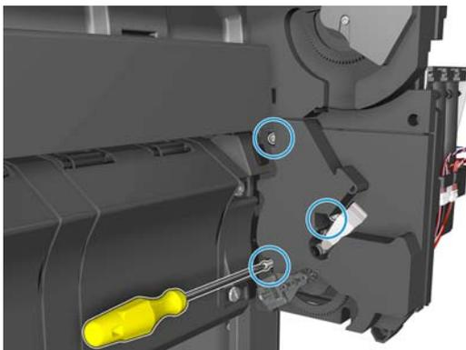
6. Remove the bottom tip support.
