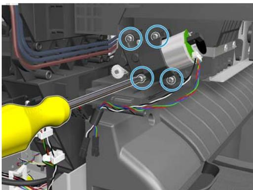
4. Remove the ramps motor.
