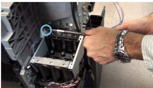
7. Remove the service station. See [Service Station with Drop Detector on page 248](#).
