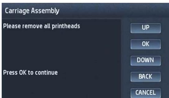
If the printheads were not correctly removed after pressing the **OK** button, a message appears asking to remove them. To do so, repeat the previous steps. If the printheads were correctly removed (it is clear there are no printheads installed in the carriage), and the message still appears, press the Cancel (X) key; the test will finish, and the appropriate error code will appear.
