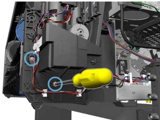
8. Remove the ISS Front Panel Side.
