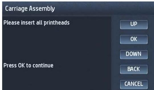
If the printheads were not correctly installed after pressing the **OK** button, a message appears asking to install them. To do so, repeat the previous steps. If on checking, the printheads were correctly installed (it is clear there are printheads installed in the carriage), and the message still appears, press the Cancel (X) key; the test will finish, and the appropriate error code will appear.
