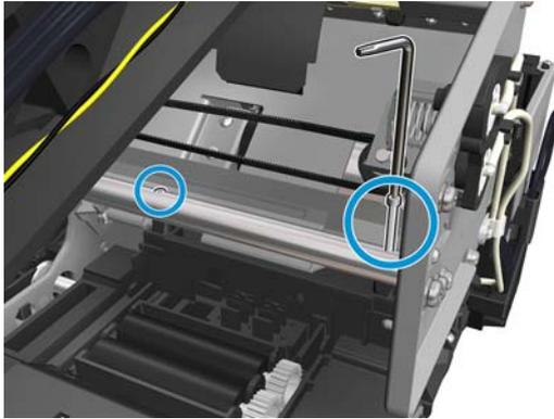
6. Remove the 2 T-15 screws and the left bracket.
