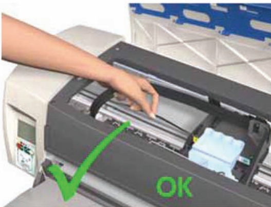
Correct: move using the belt.
