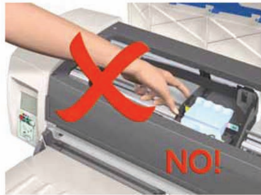
Incorrect: never move using Carriage Assembly.
