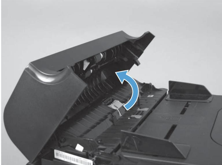
2. Hold the scanner cover down, and then pull up on the document feeder tray to release two tabs, lift the document feeder tray up, and then remove it.
