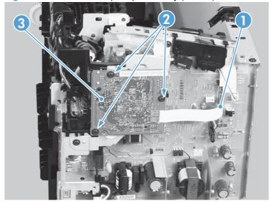
4. Remove three screws (callout 1), and then remove the sheet-metal plate (callout 2).
