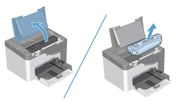
Keep the print cartridge door open, and then with both hands, grasp the side of the jammed paper that is most visible (this includes the middle), and carefully pull it free from the product.
