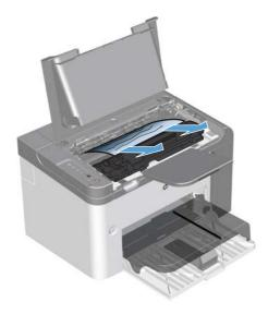
3. Reinstall the print cartridge, and then close the print-cartridge door.
