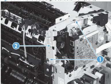
3. Remove three screws (callout 1), and then remove the sheet-metal plate (callout 2).
