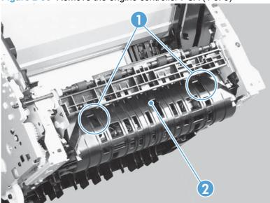
2. Remove two screws (callout 1), and then remove the sheet-metal corner brace (callout 2).
