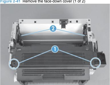
Figure 2-41 Remove the face-down cover (1 of 2)
