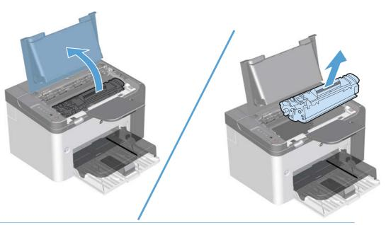
△ CAUTION: To prevent damage, do not expose the print cartridge to light. Cover it with a piece of paper.
