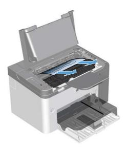
3. Press the green tab and then open the jam-access door, carefully grasp the jammed paper and slowly pull it out of the product.
