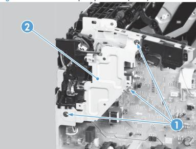
5. Disconnect one connector (callout 1), and then remove the wire harness (callout 2) from the guide (callout 3).
