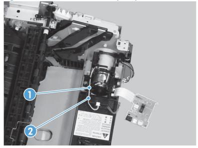
8. Remove one screw (callout 1), and then remove the motor cover (callout 2).
