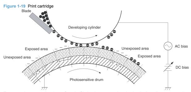
Toner acquires a negative charge from the friction that occurs when the developing roller rotates against the developing blade. The developing bias is applied to the developing roller to make a potential difference between the developing roller and the photosensitive drum. The negatively charged toner is attracted to the latent image on the photosensitive drum because the drum surface has a higher potential.
