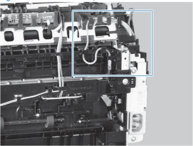
Figure 2-76 Reinstall the fuser; incorrect wire harness installation
