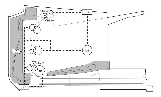
Table 1-8 Photo sensors, motor, and solenoid
