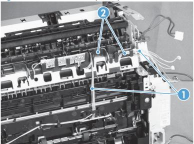
9. Remove two screws (callout 1) and the sheet-metal brace (callout 2), and then remove one bushing (callout 3).
