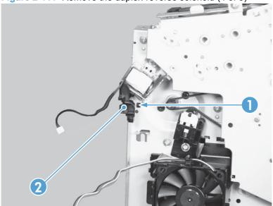
Remove one screw (callout 1), and then remove the duplex-reverse solenoid (callout 2).
