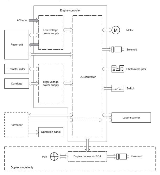
Table 1-7 DC controller controlled components
