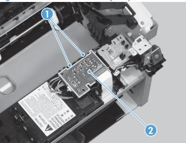
5. **Duplex models only**: Release one tab (callout 1), and then remove the duplex-connector PCA (callout 2).
