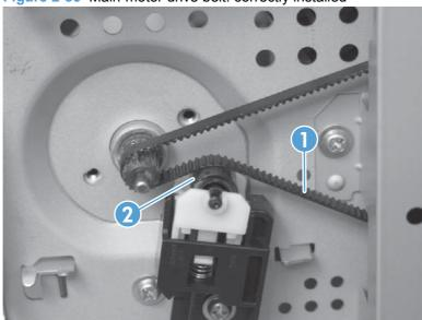
Figure 2-87 Main-motor drive belt: incorrectly installed
