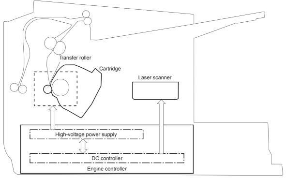
The DC controller rotates the main motor to drive the following components:
