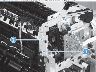
Remove one FFC (callout 1), remove three screws (callout 2), and then remove the formatter (callout 3).
