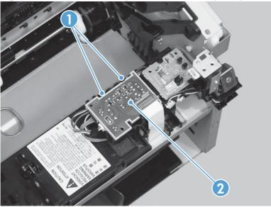
5. Release one tab (callout 1), and then remove the duplex-connector PCA (callout 2).
