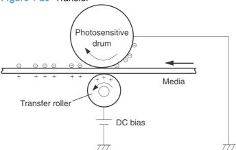
**Step 5**: The elasticity of the paper causes its separation from the photosensitive drum. A static charge eliminator aids separation by weakening any electrostatic adhesion.
