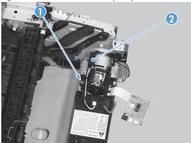
9. Remove two screws (callout 1), and then remove the motor (callout 2).
