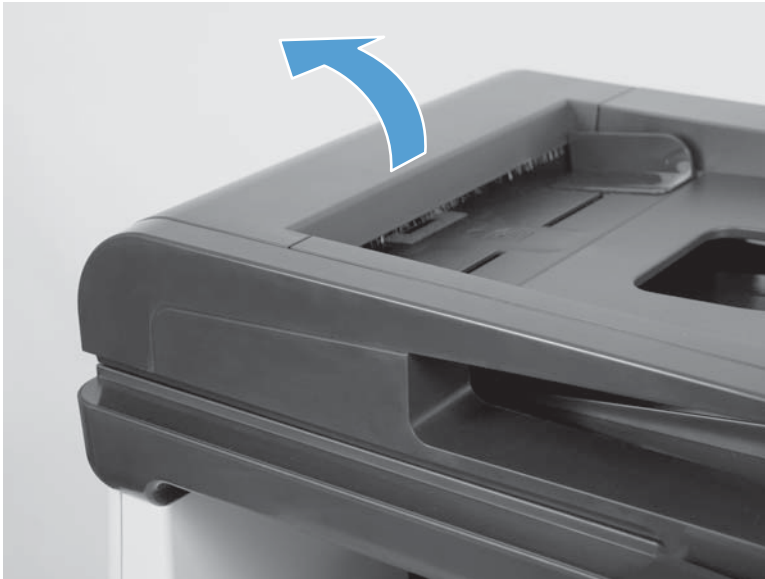
Figure 1-10 Remove the document feeder separation roller (1 of 2)
