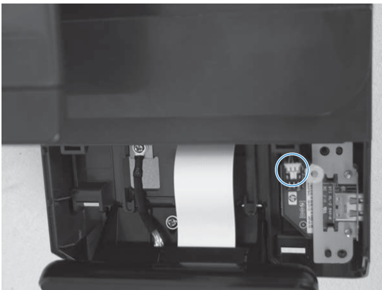
Figure 1-82 Remove the USB PCA (2 of 4)
