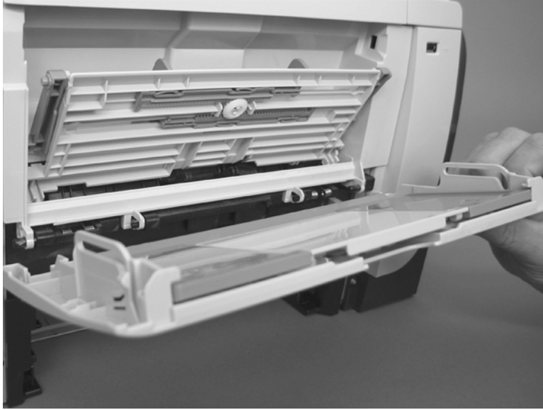
Figure 1-40 Remove Tray 1 cover (3 of 3)
