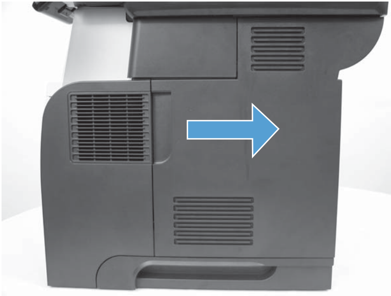
Figure 1-14 Remove the formatter cover
