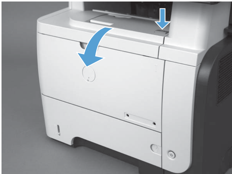
Figure 1-105 Remove the Tray 1 separation pad (1 of 2)
