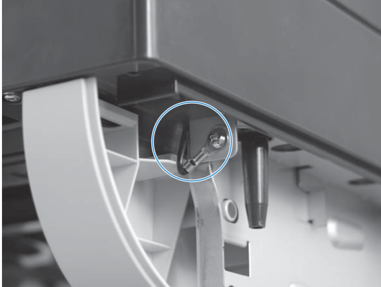
Figure 1-68 Reinstall the document feeder/scanner assembly (3 of 3)
