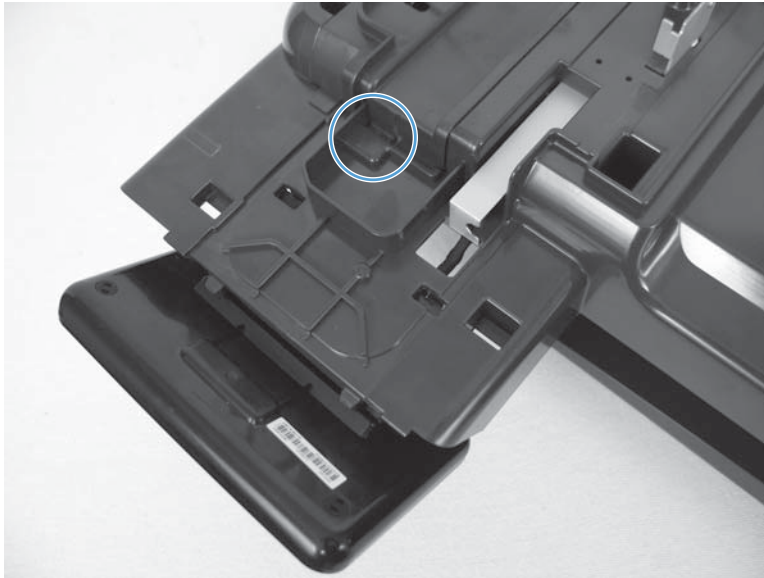
Figure 1-87 Remove the control-panel FFC (3 of 6)
