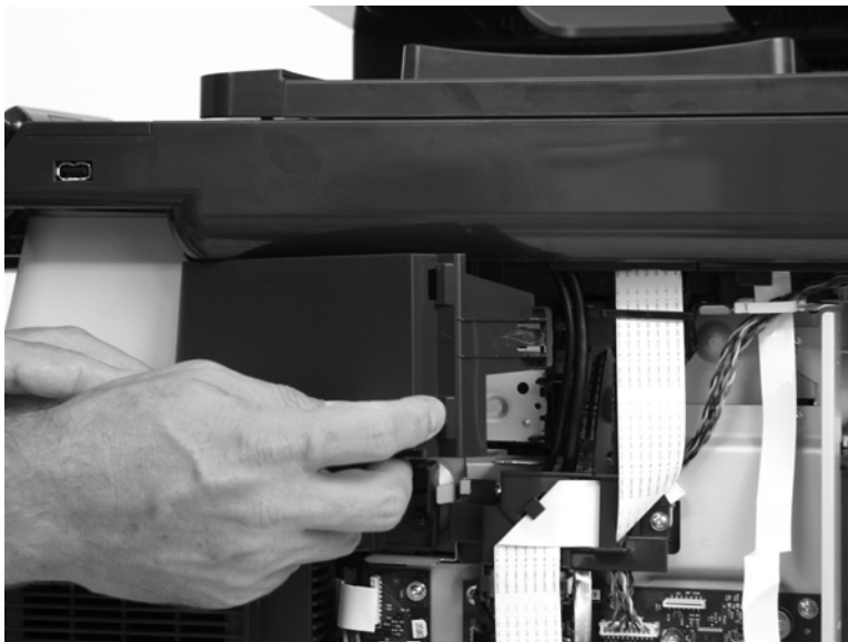
Figure 1-23 Remove the dummy cover (2 of 2)
