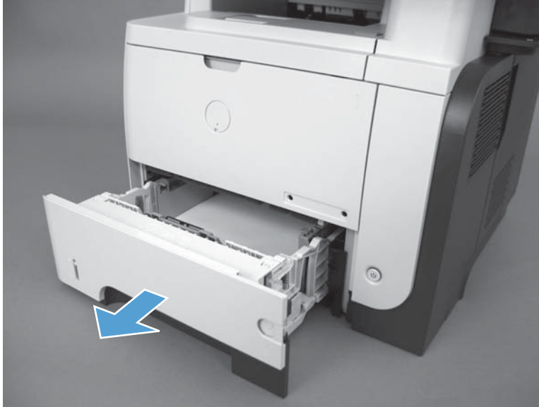
Figure 1-7 Remove the tray
