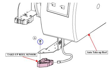
Figure 3-151. Removing the TAKE-UP REEL SENSOR
