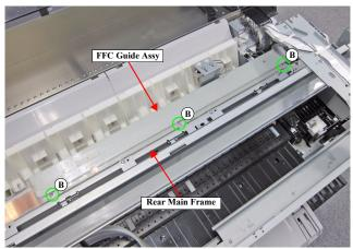
Figure 3-65. Removing the FFC (Top of the Rear Main Frame)
