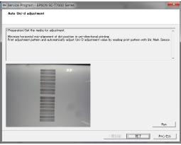
Figure 4-25. [Auto Uni-d adjustment] Screen
