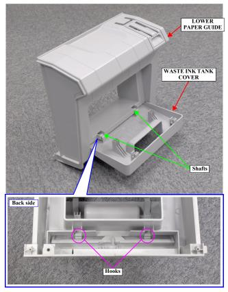
Figure 3-19. Removing the WASTE INK TANK COVER
