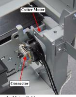
Figure 3-144. Releasing the Motor Cable
