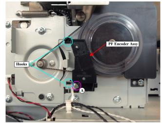
Figure 3-119. Removing the PF Encoder Assy
