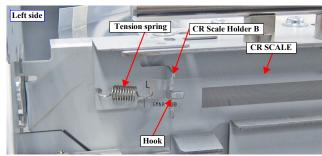
Figure 3-78. Removing the CR SCALE (Left side)
