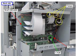
Figure 3-37. Releasing the Cable (MAIN BOARD)
