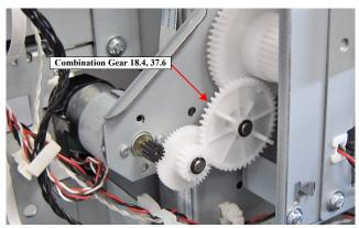
Figure 3-123. Rotate the Combination Gear 18.4, 37.6
