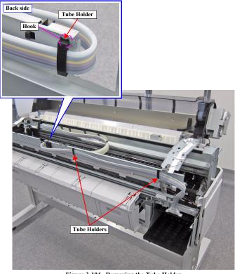
Figure 3-104. Removing the Tube Holder
