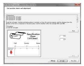
Figure 4-64. [Cut position check and adjustment] Screen
