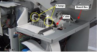
Figure 3-38. Releasing the Cable (Top of the Board Box)
