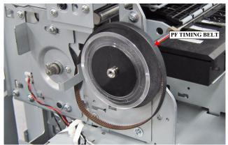
Figure 3-122. Removing the PF TIMING BELT
