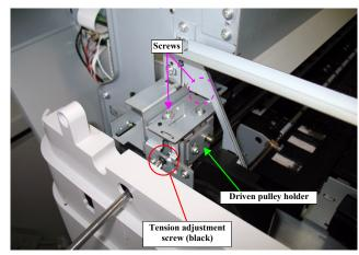
Figure 4-17. Tension adjustment screw
