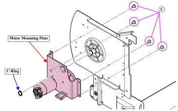
Figure 3-164. Removing the Motor Mounting Plate
