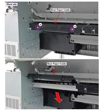
Figure 3-138. Removing the Rear Paper Guide
