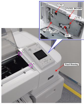
Figure 3-51. Removing the Panel Housing
