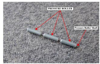
Figure 3-125. Removing the PRESSURE ROLLER (2)
