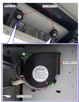
Figure 3-148. Removing the SUCTION FAN
