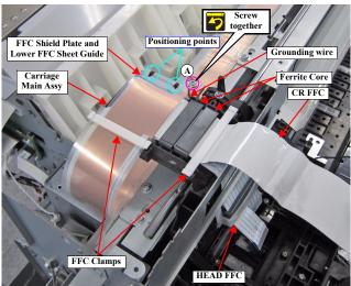
Figure 3-69. Removing the CR FFC (Top of the CR UNIT)
