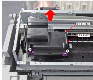
Figure 3-53. Removing the CR COVER
