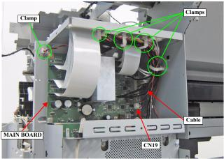
Figure 3-87. Releasing the Cable
