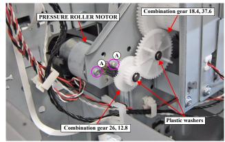
Figure 3-127. Removing the Combination gear 26, 12.8 and Combination gear 18.4, 37.6
