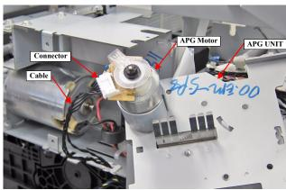
Figure 3-92. Removing the Cable
