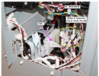
Figure 3-96. Disconnecting the Relay connectors and FFC
