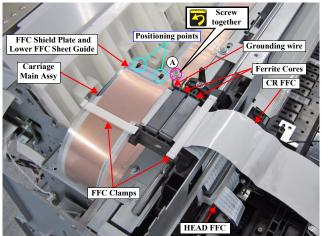
Figure 3-62. Removing the HEAD FFC (Top of the CR UNIT)
