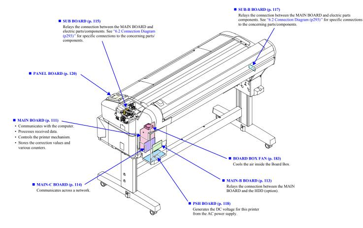
Figure 3-4. Electric Circuit Components
