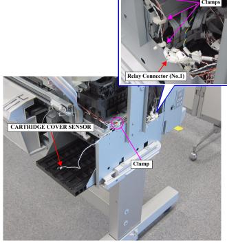
Figure 3-33. Removing the CARTRIDGE COVER SENSOR
