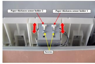
Figure 4-67. Adjusting the Positions
