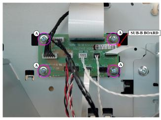
Figure 3-47. Removing the SUB-B BOARD
