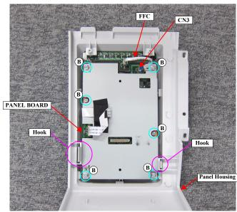
Figure 3-52. Removing the PANEL BOARD
