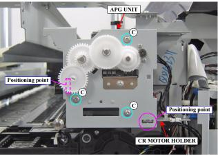
Figure 3-91. Removing the APG UNIT
