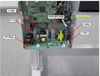
Figure 3-49. Removing the PS Plate
