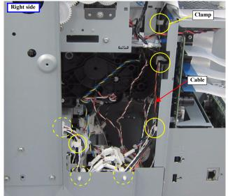
Figure 3-39. Releasing the Cable (Right side)
