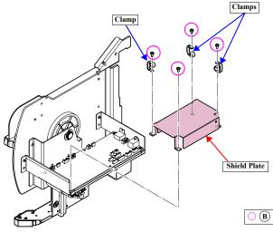
Figure 3-168. Removing the Removing the Shield Plate
