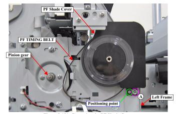
Figure 3-121. Removing the PF Shade Cover
