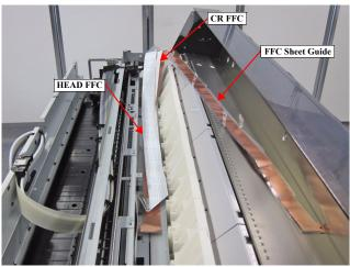
Figure 3-64. Removing the FFC Sheet Guide
