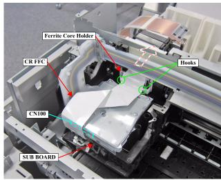
Figure 3-56. Releasing the CR FFC
