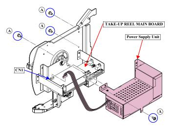
Figure 3-167. Removing the Power Supply Unit
