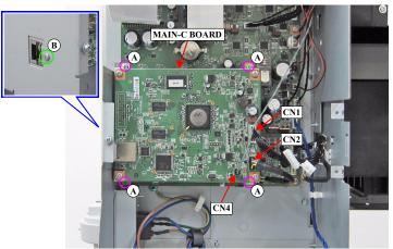
Figure 3-40. Removing the MAIN-C BOARD
