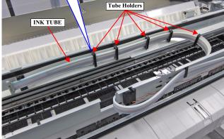
Figure 3-102. Removing the INK TUBE (Left side)
