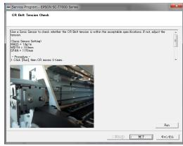
Figure 4-14. [CR Belt Tension Check] Screen
