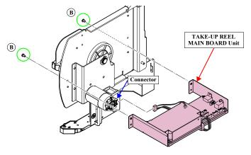
Figure 3-163. Removing the TAKE-UP REEL MAIN BOARD Unit
