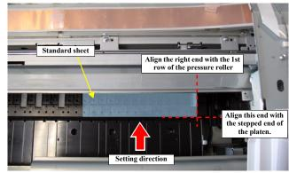
Figure 4-68. Setting Position of the Standard Sheet
