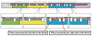
Figure 4-32. The measurement position for SC-T7000 Series
