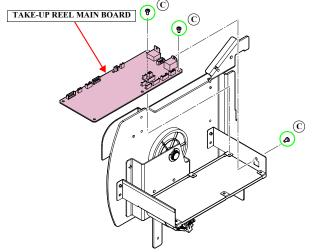
Figure 3-170. Removing the TAKE-UP REEL MAIN BOARD
