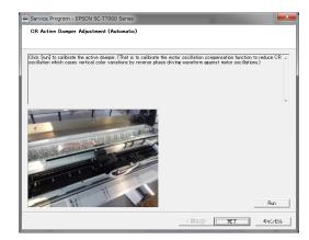
Figure 4-24. [CR Active Damper Adjustment] Screen
