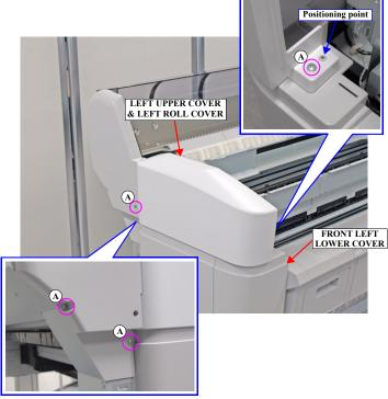
Figure 3-28. Removing the LEFT UPPER COVER & LEFT ROLL COVER
