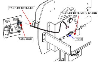
Figure 3-154. Removing the TAKE-UP REEL LED
