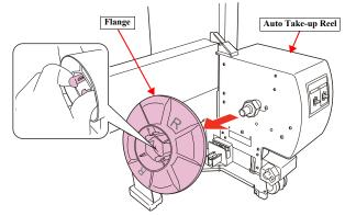
Figure 3-161. Removing the Flange
