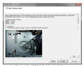
Figure 4-58. [PF Belt Tension check] Screen
