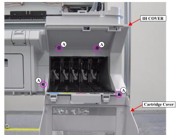
Figure 3-16. Removing the IH COVER
