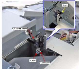
Figure 3-89. Removing the CR HP SENSOR
