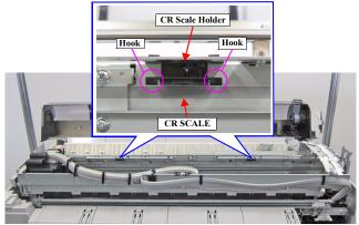
Figure 3-79. Removing the CR SCALE (Center)
