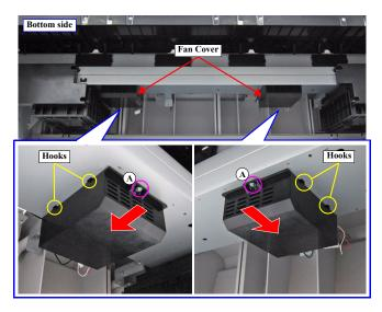
Figure 3-147. Removing the Fan Cover
