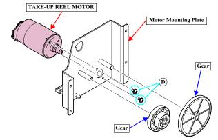
Figure 3-165. Removing the TAKE-UP REEL MOTOR
