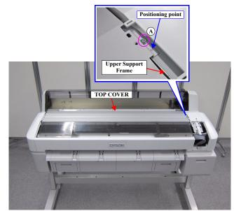
Figure 3-11. Removing the TOP COVER
