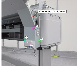
Figure 3-31. Removing the REAR LEFT LOWER COVER
