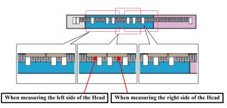
Figure 4-34. The measurement position for SC-T3000 Series
