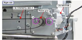
Figure 3-86. Removing the CR TIMMING BELT
