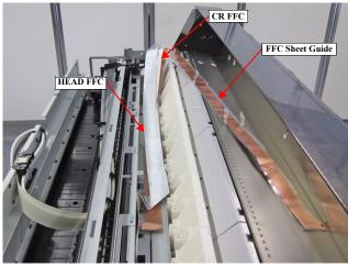
Figure 3-71. Removing the FFC Sheet Guide
