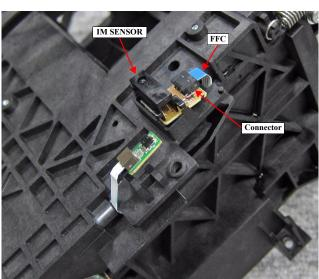
Figure 3-112. Removing the IM SENSOR
