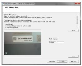
Figure 4-71. [MAC Address Input] Screen
