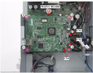
Figure 3-43. Removing the MAIN-C BOARD
