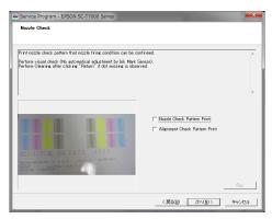
Figure 4-40. [Nozzle Check] Screen
