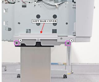
Figure 3-29. Removing the LEFT BASE COVER
