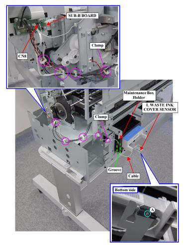
Figure 3-35. Removing the L WASTE INK COVER SENSOR
