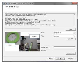
Figure 4-70. [RTC&USB ID Input] Screen
