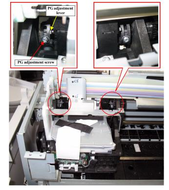
Figure 4-36. PG Adjustment Levers and PG Adjustment Screws
