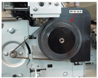
Figure 3-118. Removing the PF SCALE
