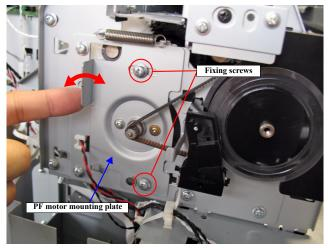
Figure 4-57. Softening the PF TIMING BELT
