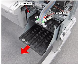
Figure 3-100. Removing the IC HOLDER (2)
