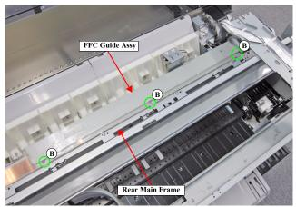
Figure 3-72. Removing the CR FFC (Top of the Rear Main Frame)
