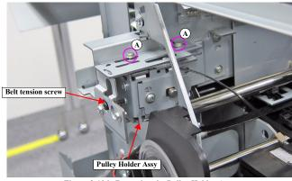
Figure 3-106. Removing the Pulley Holder Assy
