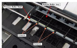
Figure 3-124. Removing the PRESSURE ROLLER (1)
