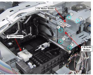
Figure 3-109. Removing the CR Scale Holder
