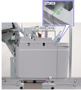
Figure 3-25. Removing the LEFT LOWER COVER  $\,$
