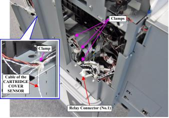
Figure 3-15. Releasing the Cable
