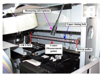
Figure 4-15. Measuring the belt tension
