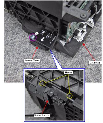
Figure 3-111. Removing the Sensor Cover
