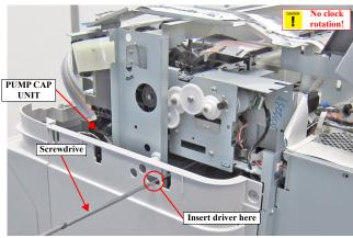
Figure 3-9. Unlocking the CR Unit
