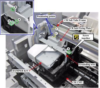
Figure 3-55. Removing the CR Sub Fixing Plate
