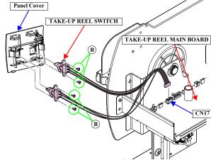
Figure 3-157. Removing the TAKE-UP REEL SWITCH
