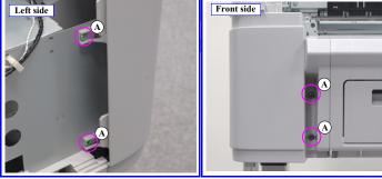
Figure 3-30. Removing the FRONT LEFT LOWER COVER
