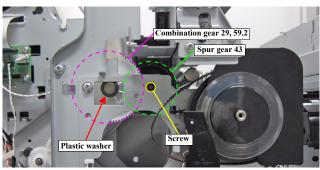
Figure 3-130. Removing the PRESSURE ROLLER SENSOR (1)
