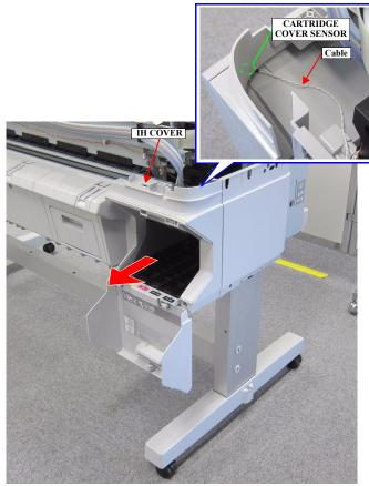
Figure 3-17. Removing the IH COVER
