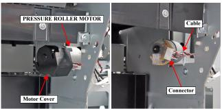
Figure 3-128. Removing the PRESSURE ROLLER MOTOR
