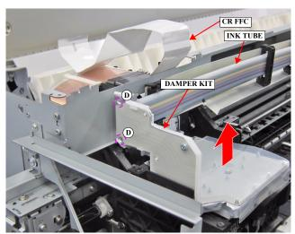
Figure 3-57. Removing the INK TUBE
