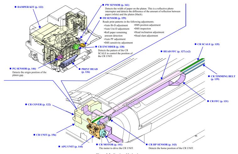
Figure 3-5. Carriage Mechanism
