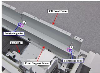
Figure 3-44. Removing the CR Front Frame
