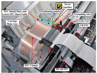
Figure 3-108. Removing the HAED FFC and CR FFC (Top of the CR UNIT)
