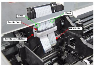
Figure 3-107. Removing the HEAD FFC
