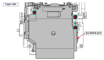
Figure 3-58. Removing the DAMPER KIT
