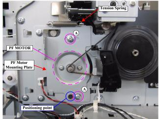
Figure 3-115. Removing the PF Motor Mounting Plate
