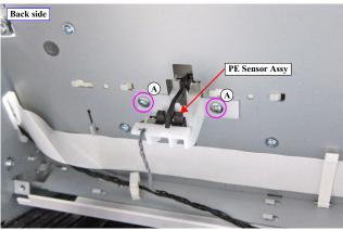
Figure 3-136. Removing the PE Sensor Assy
