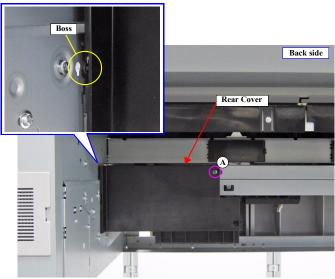
Figure 3-97. Removing the Rear Cover
