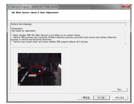
Figure 4-20. [Ink Mark Sensor check & Auto Adjustment] Screen
