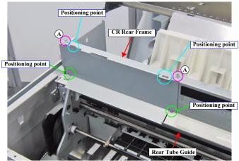
Figure 3-54. Removing the CR Rear Frame
