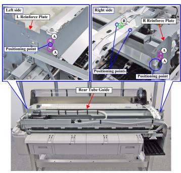
Figure 3-77. Removing the Rear Tube Guide
