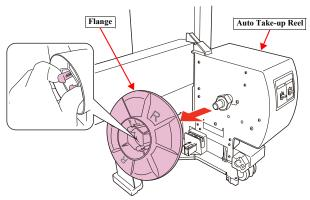
Figure 3-158. Removing the Flange
