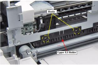
Figure 3-45. Removing the Upper EJ Holder
