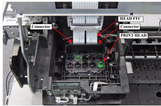
Figure 3-59. Removing the HEAD FFC
