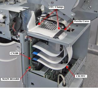
Figure 3-75. Removing the CR FFC (Around the Board Box)
