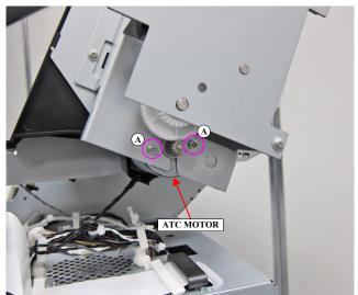
Figure 3-133. Removing the ATC MOTOR
