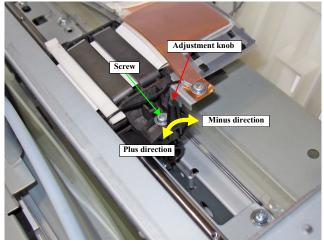
Figure 4-52. Correcting the Head Slant
