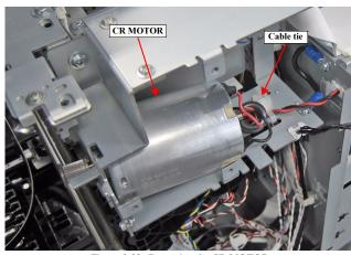
Figure 3-88. Removing the CR MOTOR
