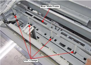
Figure 3-66. Releasing the FFC (2)
