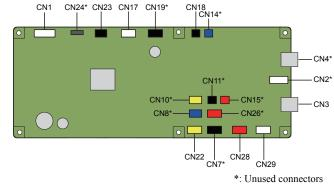
Figure 3-169. Connector location
