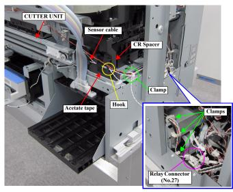
Figure 3-143. Releasing the Sensor Cable
