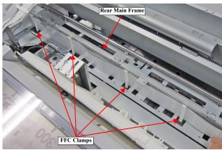
Figure 3-73. Releasing the FFC (2)
