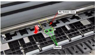
Figure 3-139. Removing the PE Sensor Assy
