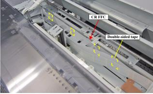
Figure 3-74. Releasing the FFC (3)
