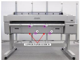
Figure 3-14. Removing the LOWER PAPER GUIDE B
