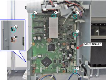
Figure 3-41. Removing the MAIN BOARD
