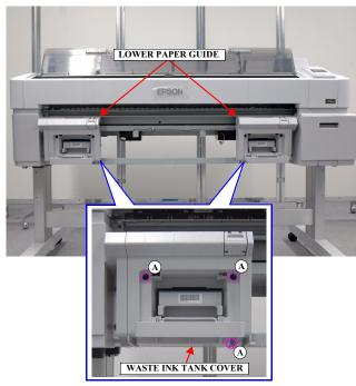
Figure 3-13. Removing the LOWER PAPER GUIDE
