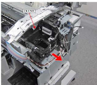
Figure 3-110. Removing the CR UNIT
