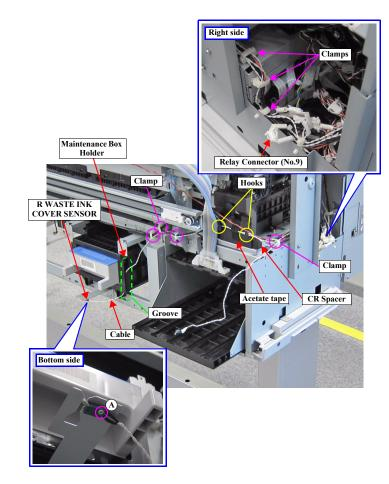
Figure 3-34. Removing the R WASTE INK COVER SENSOR
