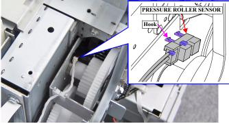
Figure 3-131. Removing the PRESSURE ROLLER SENSOR (2)
