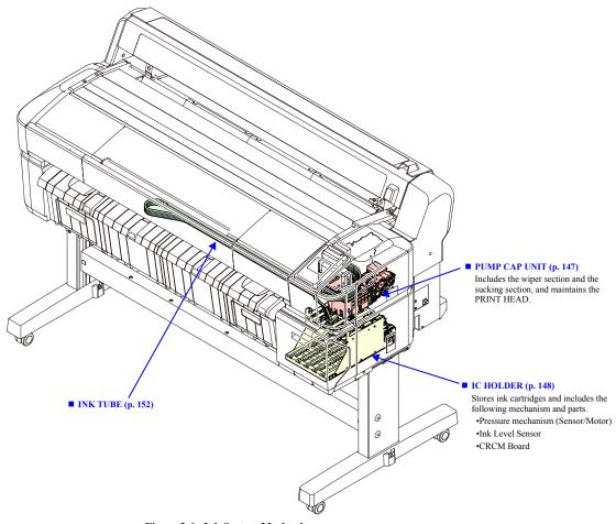
Figure 3-6. Ink System Mechanism
