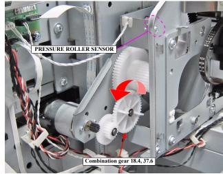
Figure 3-129. Rotate the Combination gear 18.4, 37.6
