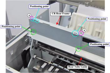
Figure 3-76. Removing the CR Rear Frame
