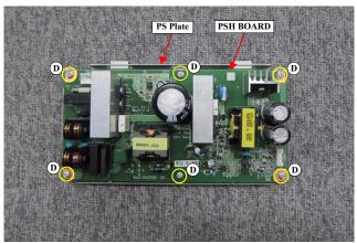
Figure 3-50. Removing the PSH BOARD
