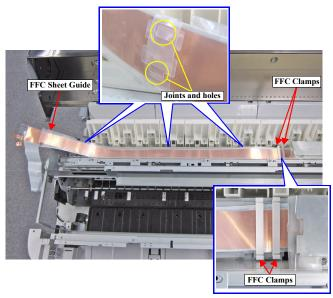
Figure 3-63. Releasing the FFC (1)
