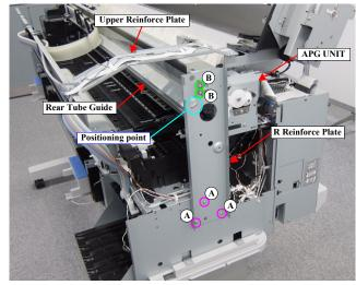
Figure 3-90. Removing the R Reinforce Plate
