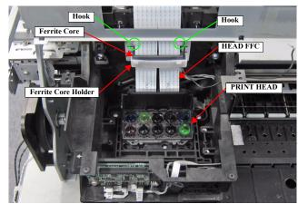
Figure 3-68. Removing the HEAD FFC
