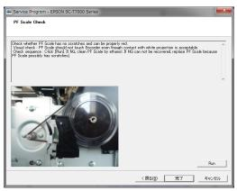
Figure 4-60. [PF Scale Check] Screen
