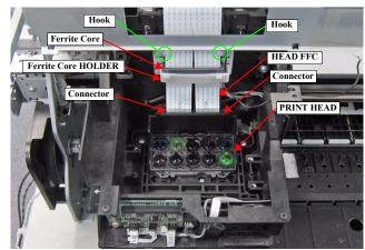
Figure 3-61. Removing the HEAD FFC
