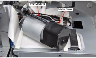
Figure 3-134. Removing the Motor Cover
