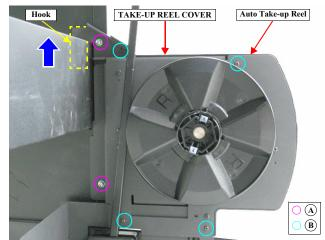
Figure 3-149. Removing the Auto Take-up Reel
