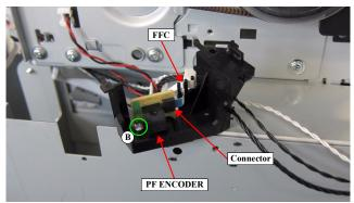
Figure 3-120. Removing the PF ENCODER
