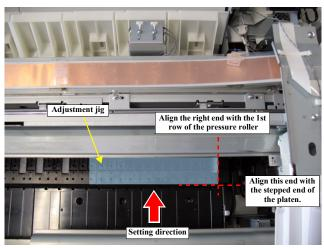
Figure 4-66. Setting position of the adjustment jig
