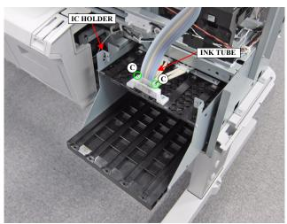
Figure 3-105. Removing the INK TUBE (2)
