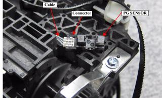
Figure 3-94. Removing the Cable
