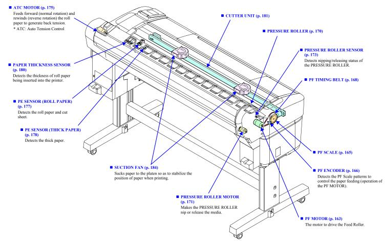
Figure 3-7. Paper Feed Mechanism / Cutter
