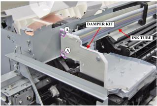
Figure 3-101. Removing the INK TUBE (1)
