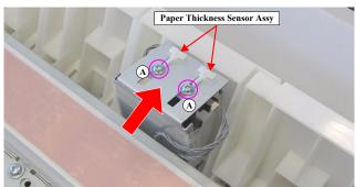
Figure 3-141. Removing the Paper Thickness Sensor Assy
