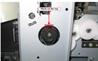
Figure 4-31. APG cam position checking point
