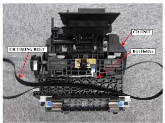
Figure 3-84. Removing the CR TIMING BELT
