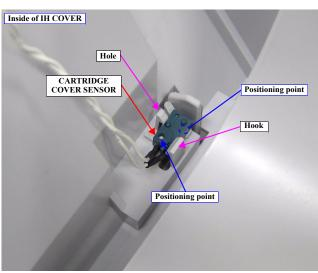
Figure 3-18. Removing the CARTRIDGE COVER SENSOR
