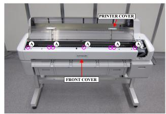
Figure 3-12. Removing the FRONT COVER
