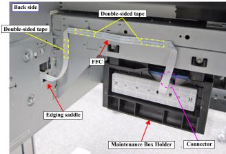
Figure 3-98. Releasing the FFC
