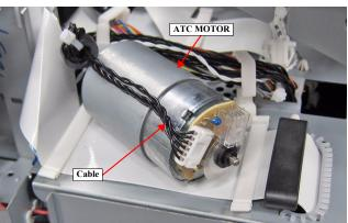
Figure 3-135. Removing the Cable
