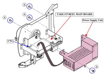
Figure 3-156. Removing the Power Supply Unit
