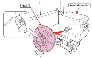
Figure 3-155. Removing the Flange
