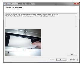
Figure 4-76. [Suction Fan Adjustment] Screen
