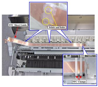
Figure 3-70. Releasing the FFC (1)
