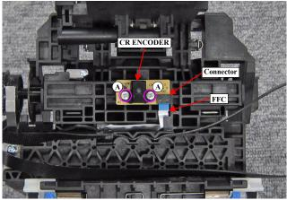
Figure 3-82. Removing the CR ENCODER
