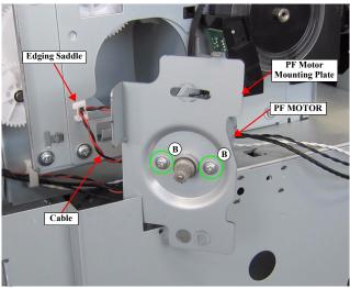
Figure 3-116. Removing the PF MOTOR
