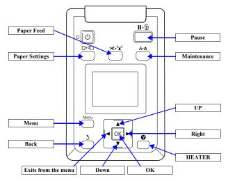
Figure 4-79. Buttons and Their Names Displayed on the Panel
