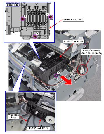
Figure 3-95. Removing the PUMP CAP UNIT
