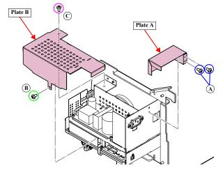
Figure 3-159. Removing the Plate A/B
