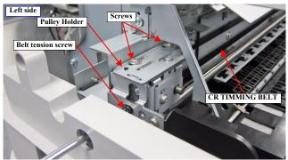
Figure 3-85. Loosening the CR TIMMING BELT tension
