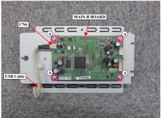
Figure 3-42. Removing the MAIN-B BOARD
