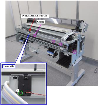
Figure 3-36. Removing the INTERLOCK SWITCH
