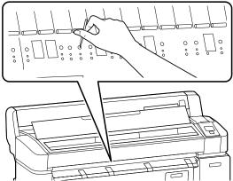
Figure 5-4. Cleaning the Suction Holes on the Platen
