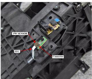
Figure 3-114. Removing the PW SENSOR
