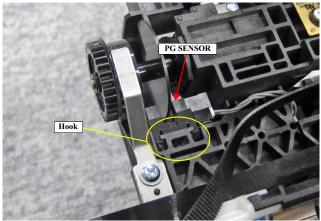
Figure 3-93. Removing the PG SENSOR
