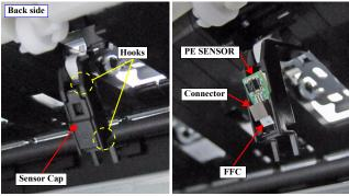
Figure 3-140. Removing the PE SENSOR (THICK PAPER)
