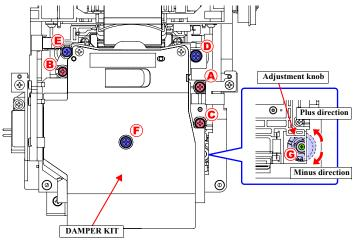
Figure 4-47. Correcting the Head Inclination
