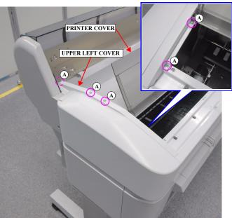
Figure 3-27. Removing the UPPER LEFT COVER
