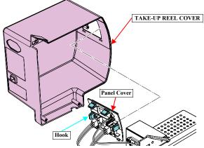
Figure 3-150. Removing the TAKE-UP REEL COVER
