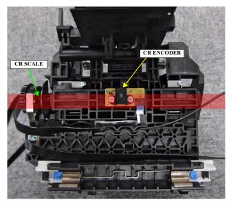
Figure 4-23. CR Encoder and Scale Check
