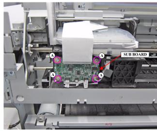
Figure 3-46. Removing the SUB BOARD
