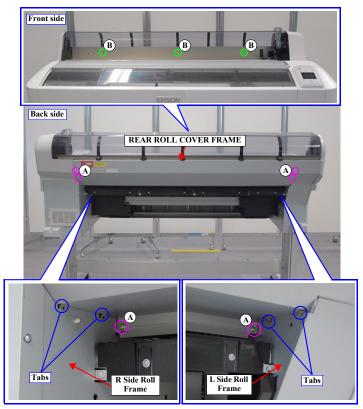
Figure 3-32. Removing the REAR ROLL COVER FRAME
