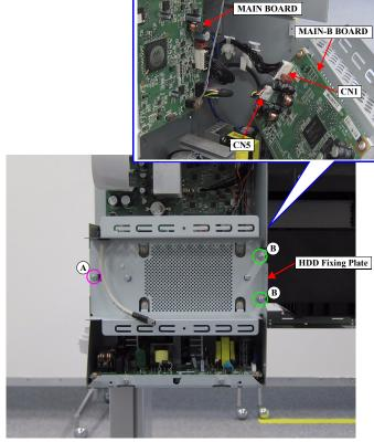
Figure 3-48. Removing the HDD Fixing Plate
