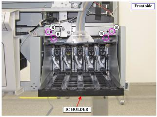
Figure 3-99. Removing the IC HOLDER (1)
