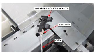
Figure 3-132. Removing the PRESSURE ROLLER SENSOR (3)
