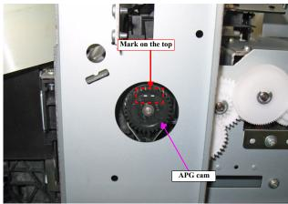
Figure 4-19. Checking the APG cam
