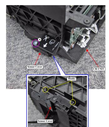
Figure 3-113. Removing the Sensor Cover
