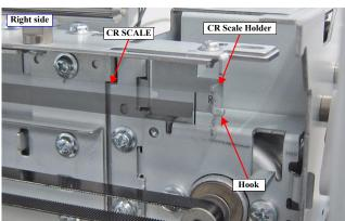
Figure 3-80. Removing the CR SCALE (Right)
