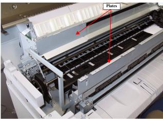
Figure 4-35. Removing the plate
