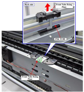
Figure 3-103. Releasing the INK TUBE (Front side)
