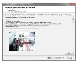
Figure 4-50. [Head slant manual adjustment (PF direction)] Screen
