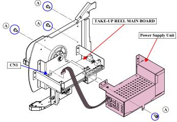
Figure 3-153. Removing the Power Supply Unit
