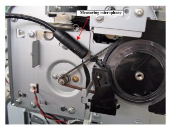
Figure 4-59. PF Belt Tension Check
