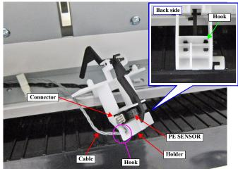
Figure 3-137. Removing the PE SENSOR (ROLL PAPER)
