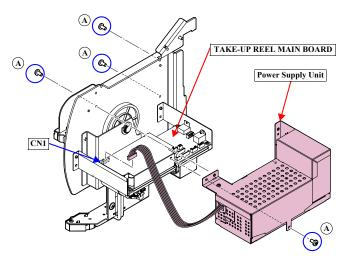
Figure 3-162. Removing the Power Supply Unit
