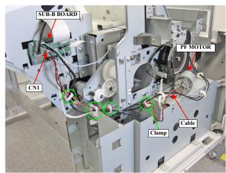
Figure 3-117. Releasing the Cable
