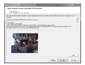
$Figure\ 4-45.\ [Head\ inclination\ manual\ adjustment\ (CR\ direction)]\ Screen$
