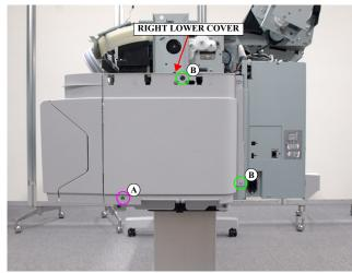
Figure 3-23. Removing the RIGHT LOWER COVER
