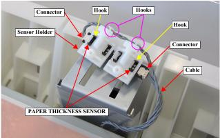
Figure 3-142. Removing the PAPER THICKNESS SENSOR
