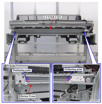
Figure 3-145. Removing the CUTTER UNIT
