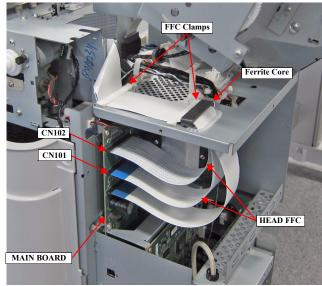
Figure 3-67. Removing the HEAD FFC (Around the Board Box)
