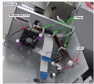
Figure 3-146. Removing the BOARD BOX FAN
