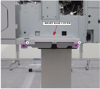
Figure 3-24. Removing the RIGHT BASE COVER
