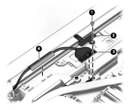
**16.** Release the wireless antenna cables from the routing channels built into the base enclosure.
