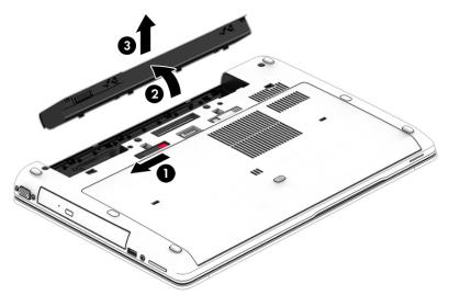
Reverse this procedure to install the battery.
