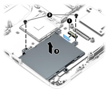
Reverse this procedure to install the smart card reader and cable.
