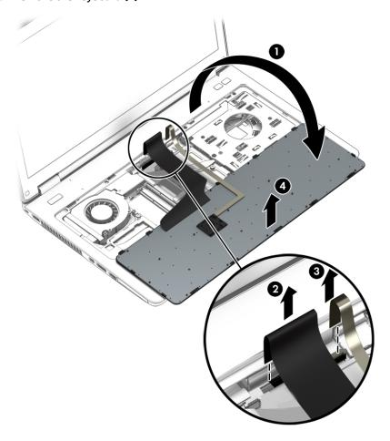
Reverse this procedure to install the keyboard.
