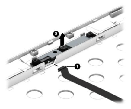
c. Remove the webcamera/microphone module.
