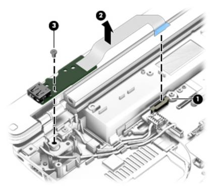
4. Remove the USB board and cable.
