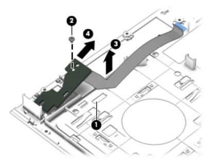
Reverse this procedure to install the function button board.
