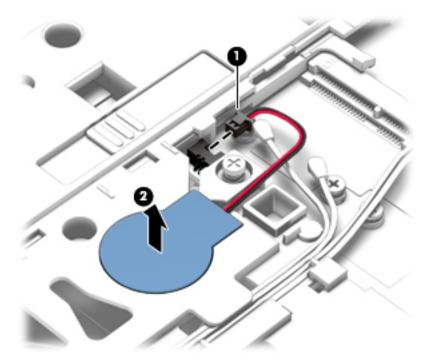
Remove the RTC battery and cable.
