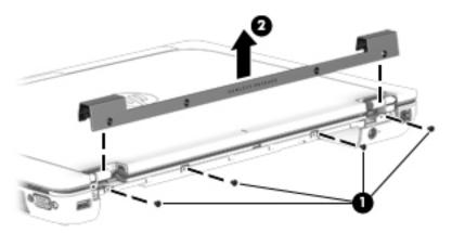
9. Remove the two Torx T8M2.5×4.5 screws that secure the display assembly to the base enclosure.
