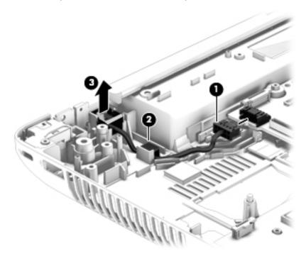
4. Remove the power connector cable.
