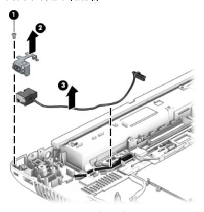
Reverse this procedure to install the RJ-45 (network) cable.
