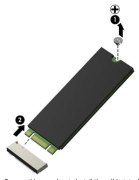
Reverse this procedure to install the solid-state drive.
