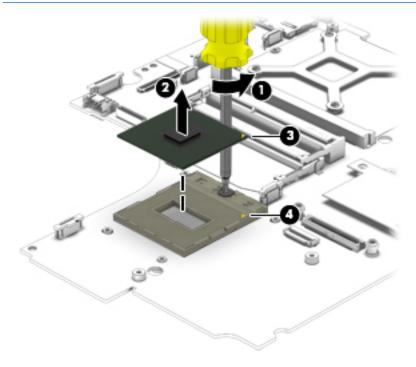
Reverse this procedure to install the processor.
