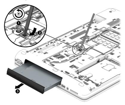
Reverse this procedure to install the optical drive.
