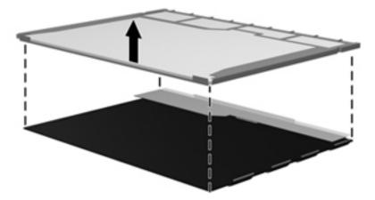
24. Recycle the LCD panel and backlight.
