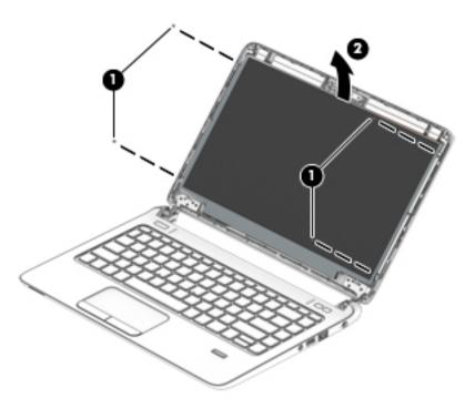
7. Rotate the display panel all the way over (1), disconnect the display cable from the rear of the panel (2), and then remove the display panel (3) from the enclosure.
