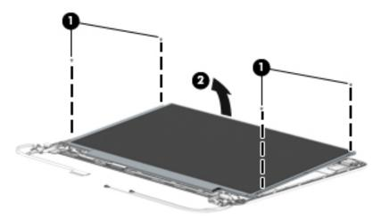
**13.** Rotate the display panel all the way over **(1)**, disconnect the display cable from the rear of the panel **(2)**, and then remove the display panel **(3)** from the enclosure.
