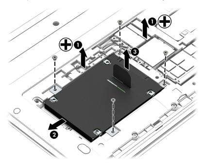
To remove the hard drive cover from the hard drive, remove the 4 Phillips PM3.0×3.0 screws (1) that secure the cover to the drive, and then lift the cover off the drive (2).
