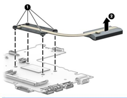
NOTE: Thoroughly clean thermal material from the surfaces of the system board component (1) and the heat sink (2) each time you remove the heat sink. All heat sink and processor spare part kits include thermal material.
