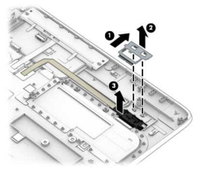
Reverse this procedure to install the fingerprint reader assembly.
