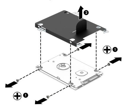
Reverse this procedure to install a hard drive.
