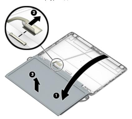
**14.** If it is necessary to replace the display hinges, remove the 6 Phillips PM2.5×3.0 screws **(1)** that secure the display hinges to the display enclosure.
