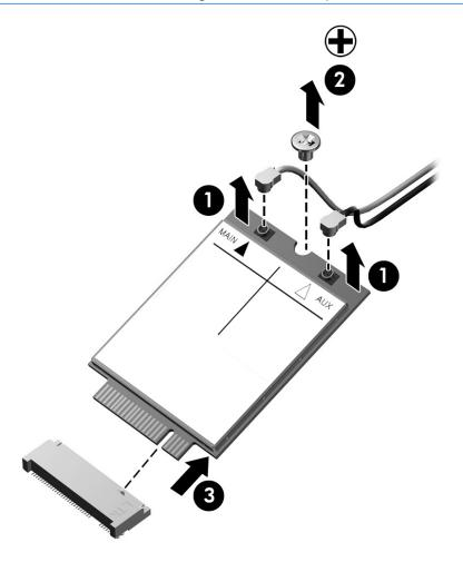
NOTE: If the WWAN antennas are not connected to the terminals on the WWAN module, the protective sleeves must be installed on the antenna connectors, as shown in the following illustration.
