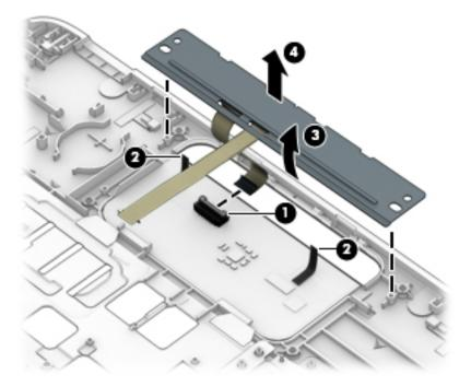
Reverse this procedure to install the touchpad board.
