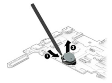
Reverse this procedure to install the RTC battery.
