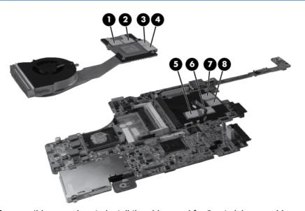
Reverse this procedure to install the video card fan/heat sink assembly.
