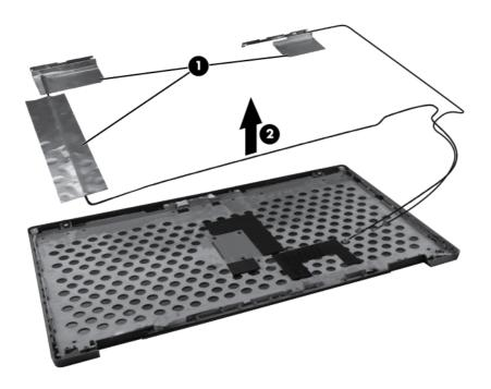
19. If it is necessary to replace the WLAN antenna cables, detach the WLAN antenna transceivers (1) from the adhesive on the back cover, and then release the cables from the clips (2) that secure the cables to the display back cover.
