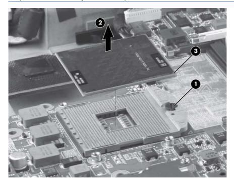
Reverse this procedure to install the processor.
