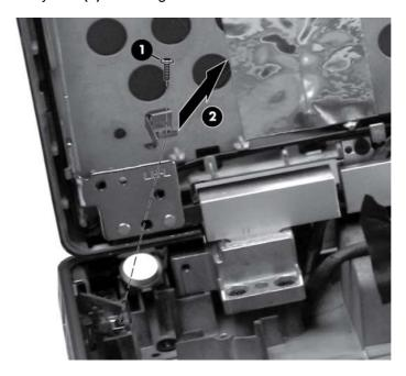
Reverse this procedure to install the security lock.
