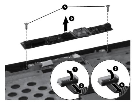
17. If it is necessary to replace the webcam/ambient light sensor cable, disconnect the cable from the ambient light sensor board (1), and then remove the cable (2).
