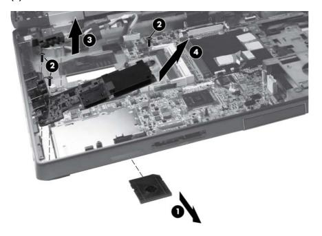
Reverse this procedure to install the Secure Digital (SD) card/USB 2.0 assembly.
