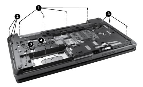
Pull up the back edge (1) of the top cover, and then lift the cover (2) away at an angle.
