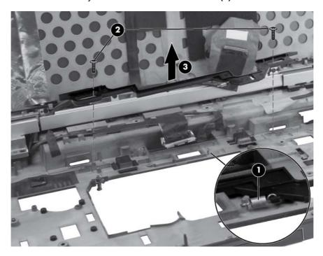
Reverse this procedure to install the battery latch.
