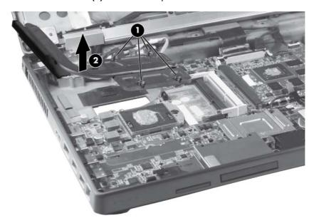
NOTE: The thermal material must be thoroughly cleaned from the surfaces of the processor heat sink components (1) and system board components (2) each time the processor heat sink is removed. Thermal material is included with all heat sink and processor spare part kits.
