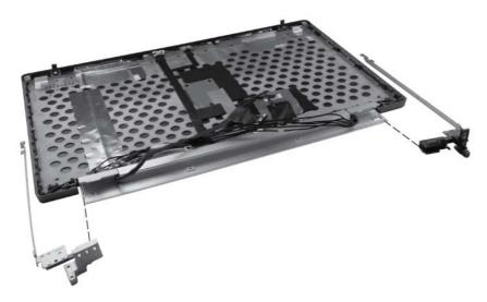
13. If it is necessary to remove the cable routing tray, remove the five Phillips M2.0×3.0 screws (1) that secure the cable routing tray to the display enclosure. The cable routing tray is available in the Raw Panel Support Kit, spare part number 657408-001.
