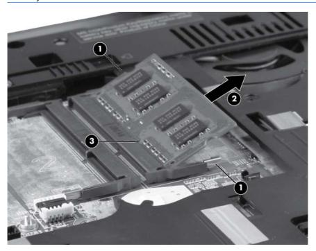
Reverse this procedure to install a primary expansion memory module.
