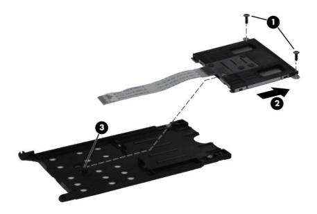
Reverse this procedure to reassemble and install the smart card reader.
