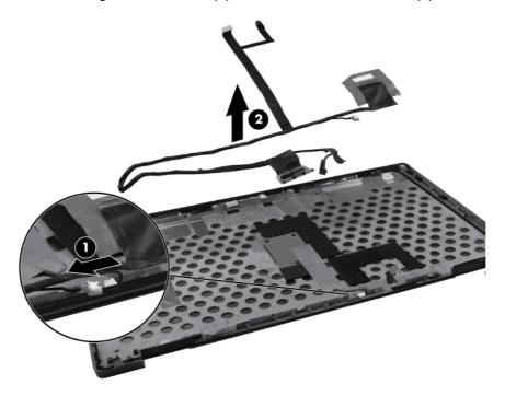
18. If it is necessary to replace the WWAN antenna cables, detach the WWAN antenna transceivers (1) from the adhesive on the back cover, and then release the cables from the clips (2) that secure the cables to the display back cover.
