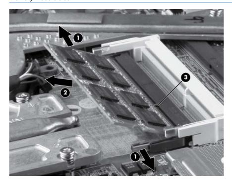
Reverse this procedure to install a primary memory module.
