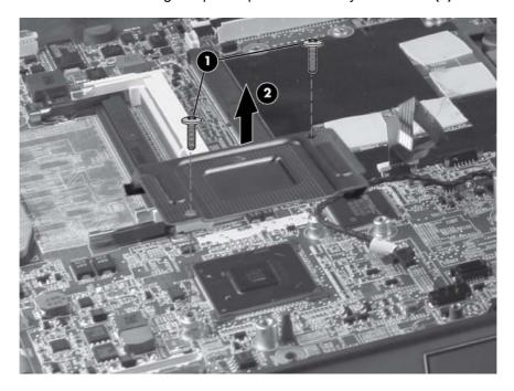
Reverse this procedure to install the Northbridge chip heat plate.
