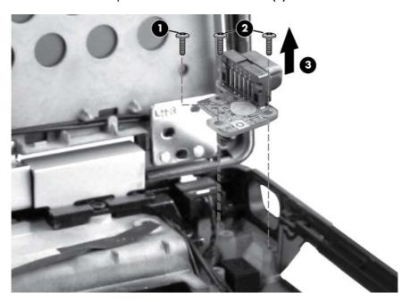
Reverse this procedure to install the VGA port.
