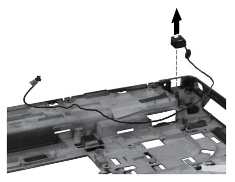
Remove the RJ-11 connector cable from the base enclosure.
