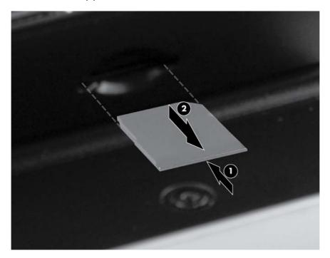
Reverse this procedure to install the SIM.
