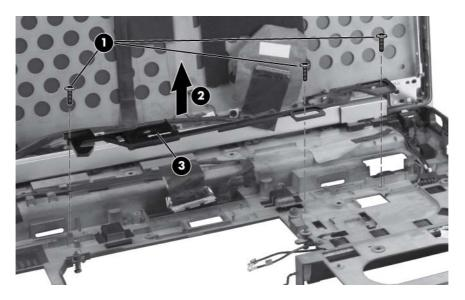
Reverse this procedure to install the service access cover latch.
