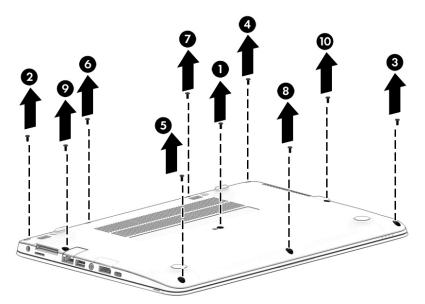
**b.** After you remove the PM2.5×5.0 screws (1), remove the 1 PM2.0×7.0 screw (2).
