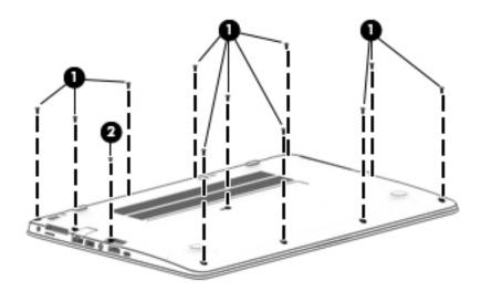
4. Pry up on the top (near the display hinge) of the bottom cover to disengage it from the computer.
