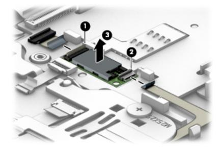
Reverse the removal procedures to install the NFC module.
