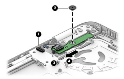
Remove the power button board from a 15" computer:
