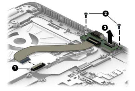
Reverse this procedure to install the USB/audio board.
