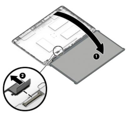
**11.** If it is necessary to replace the display hinges, remove the 1 Phillips PM2.0×3.0 screw **(1)** that secure the hinge covers to the display enclosure, and then remove the hinge covers **(2)**.
