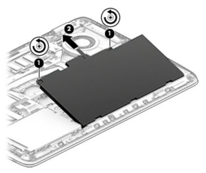
Reverse the removal procedures to install the battery.
