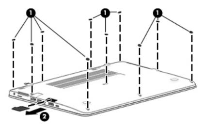
3. Remove the screws that secure the bottom cover to the computer.
