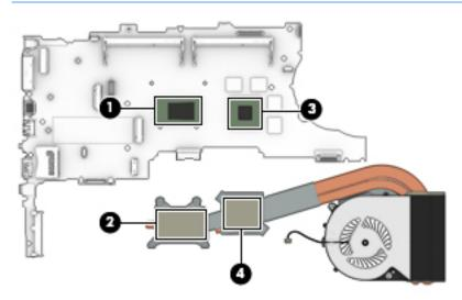
Reverse this procedure to install the heat sink/fan assembly.
