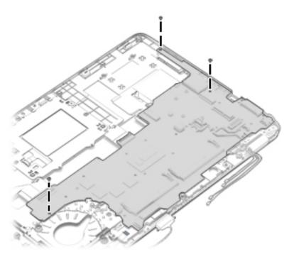
**14.** Lift the left side of the system board **(1)** until it rests at an angle.
