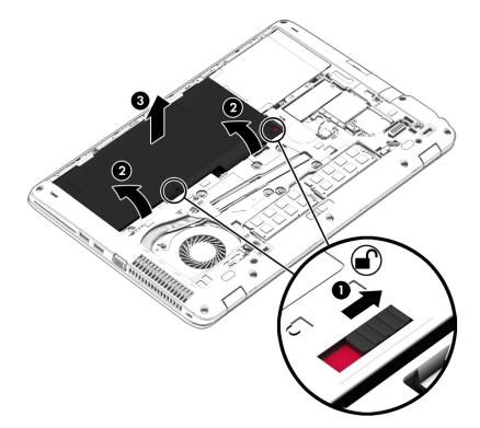
Reverse this procedure to install the battery.
