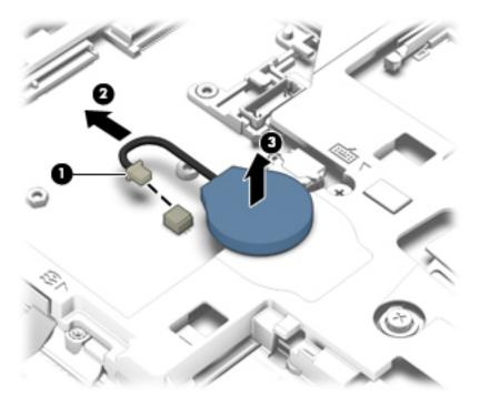
**3.** Remove the RTC battery.
