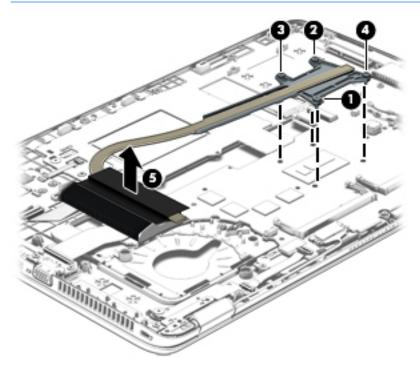
The following illustration shows the replacement thermal material locations on the system board and the heat sink on computer models equipped with a graphics subsystem with discrete memory. The thermal material must be thoroughly cleaned from the surfaces of the system board and the heat sink components each time the heat sink is removed. Replacement thermal material is included with the system board and heat sink spare part kits.
