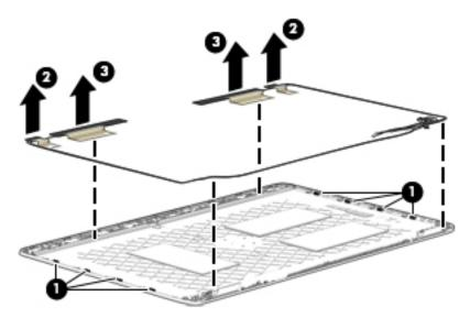
c. Remove the WLAN and WWAN antenna cables and transceivers.
