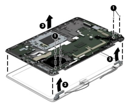
6. To remove the display bezel, flex the inside edges of the bottom edge (1), the left and right sides (2), and the bottom edge (3) of the bezel until the bezel disengages from the display enclosure.
