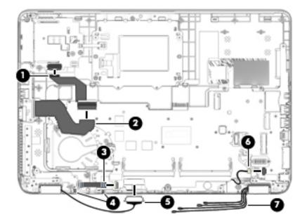
**13.** Remove the three Phillips PM2.5×5.0 screws that secure the system board to the top cover.
