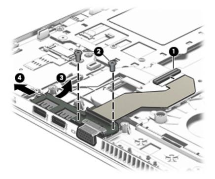
Reverse this procedure to install the USB/VGA connector board.
