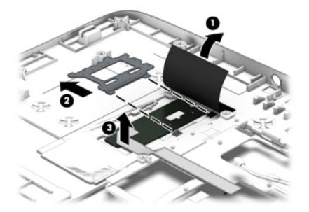
Reverse this procedure to install the fingerprint reader board.
