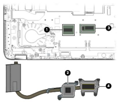
The following illustration shows the replacement thermal material locations on computer models equipped with a graphics subsystem with UMA memory. The thermal material must be thoroughly cleaned from the surfaces of the heat sink and the system board components each time the heat sink is removed. Replacement thermal material is included with the heat sink, processor, and system board spare part kits.
