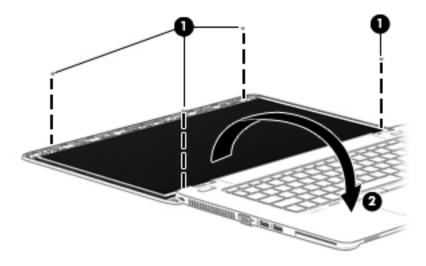
5. Release the adhesive support strip (1) that secures the display panel cable to the display panel.
