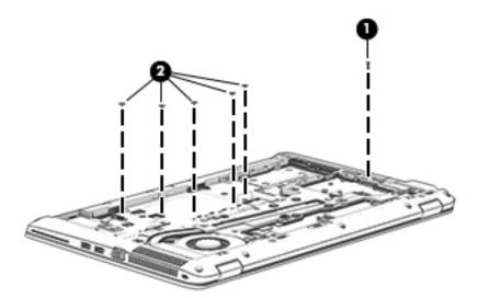
7. Lift the base enclosure off the computer.
