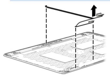
**10.** To remove the WLAN/WWAN antenna cables and transceivers:
