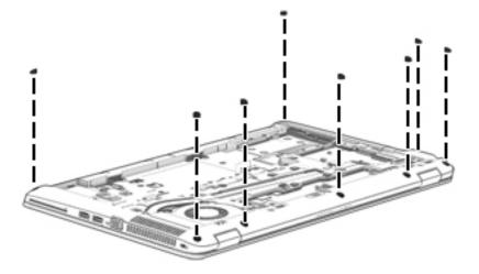
4. Remove the 21 Torx T8M2.5×5.0 screws that secure the base enclosure to the computer.
