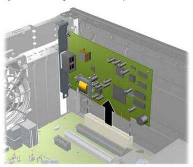
If you are removing a PCI Express x16 card, pull the retention arm on the back of the expansion socket away from the card and carefully rock the card back and forth until the connectors pull free from the socket. Pull the expansion card straight up from the socket then away from the inside of the chassis to release it from the chassis frame. Be sure not to scrape the card against the other components.
