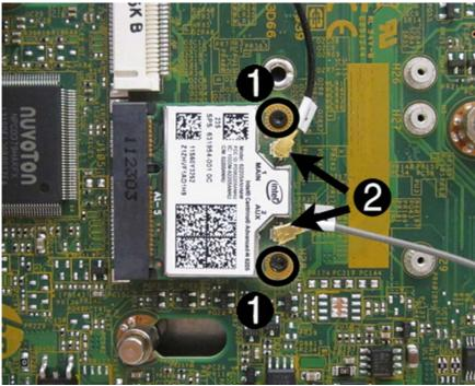
Lift the module to a 45 degree angle (3), and then remove the module from the connector by pulling it away at an angle (4).
