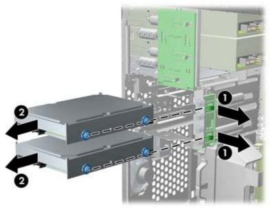
5. Remove the four guide screws (two on each side) from the old drive. You will need these screws to install a new drive.
