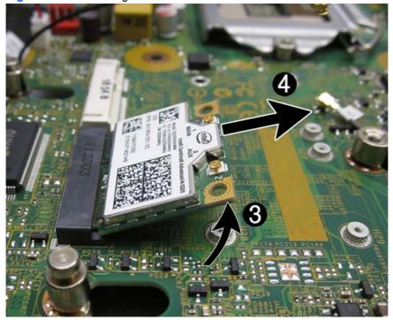
To install the WLAN module, reverse the removal procedure. Make sure the antenna cables are correctly routed.
