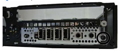
**b.** Press the tab on right side of the panel **(1)**, and then swing the right side of the cage away from the chassis to remove it **(2)**.
