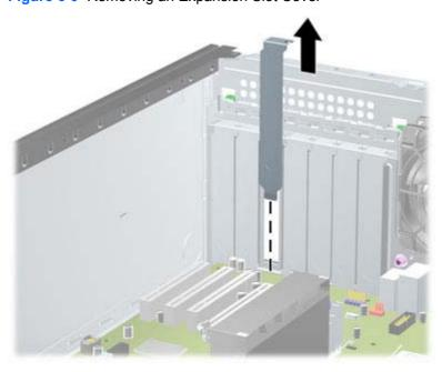
If you are removing a standard PCI card or PCI Express x1 card, hold the card at each end and carefully rock it back and forth until the connectors pull free from the socket. Lift the card straight up to remove it. Be sure not to scrape the card against other components.
