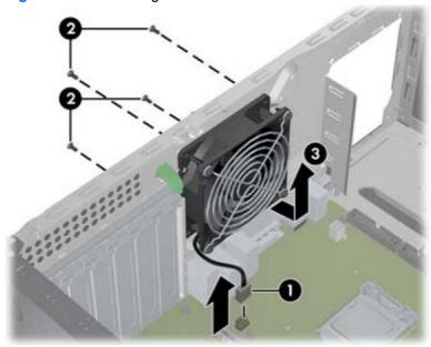
To install the fan, reverse the removal procedure. Be sure to orient the air flow out of the unit.
