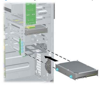
• If you are installing a hard drive into the upper bay (bay 4), slide the hard drive into the drive bay (1) then secure the drive in place with a standard 6-32 screw (2).
