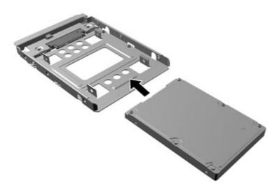
Secure the drive to the bay adapter bracket by installing four black M3 adapter bracket screws through the sides of the bracket into the drive.
