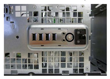
Rotate the right side of the assembly away from the chassis.
