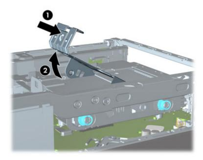
5. Lift the hard drive carrier straight up and out of the chassis.
