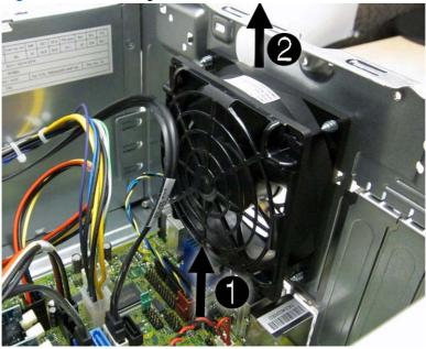
To install the fan assembly, reverse the removal procedure. Be sure to orient the air flow out of the unit.
