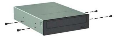
Position the guide screws on the drive into the J-slots in the drive bay. Then slide the drive toward the front of the computer until it locks into place.
