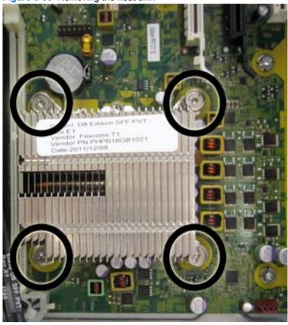
Lift the heat sink from atop the processor, and set it on its side to keep from contaminating the work area with thermal grease.
