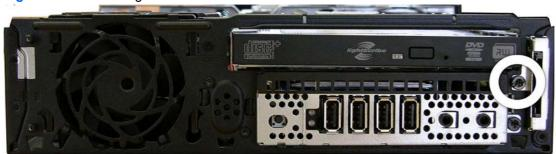
9. Pull the reader away from the front of the chassis while threading the cable through the slot in the front of the chassis.
