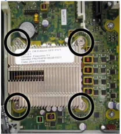
Lift the heat sink from atop the processor.
