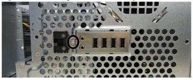
Rotate the left side of the assembly to the right .
