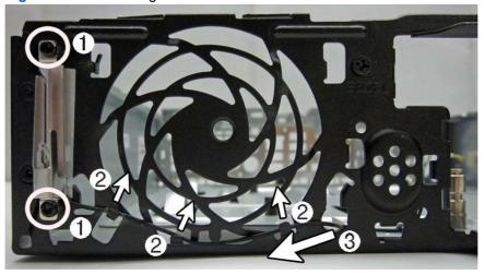
13. To remove the rear antenna, from the inside of the front of the chassis, remove the antenna from the plastic clips attached to the side of the chassis.
