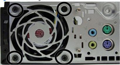
**10.** From the inside of the chassis, slide the fan out from underneath the chassis lip, and then remove the fan.
