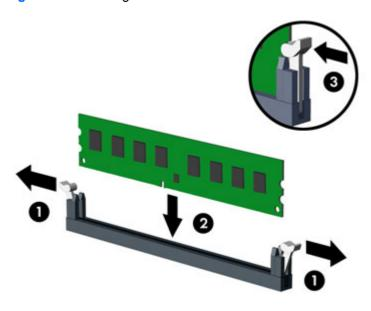
NOTE: A memory module can be installed in only one way. Match the notch on the module with the tab on the memory socket.
