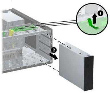
• To remove a hard drive from one of the two lower internal hard drive bays, pull up on the green hard drive drivelock mechanism (1) for that drive and slide the drive from the drive bay (2).
