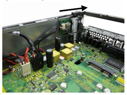
To install the card reader, reverse the removal procedure.
