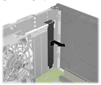
If you are removing a standard PCI card or PCI Express x1 card, hold the card at each end, and carefully rock it back and forth until the connectors pull free from the socket. Pull the expansion card straight up from the socket then away from the inside of the chassis to release it from the chassis frame. Be sure not to scrape the card against the other components.
