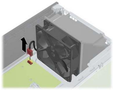
Press the tabs that secure the fan assembly to the front of the chassis (1).
