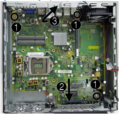
To install the system board, reverse the removal procedure.
