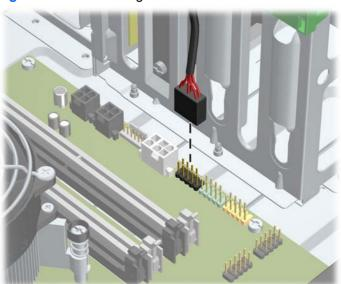
Figure 6-21 Connecting the Media Card Reader USB Cable
