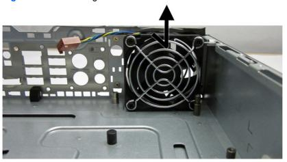
To install the rear fan, reverse the removal procedure.
