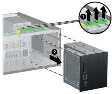
**9.** Gently slide the drive into the uppermost available bay until it snaps into place. When the drive is properly inserted, the drivelock will secure it. Repeat this step for each drive.
