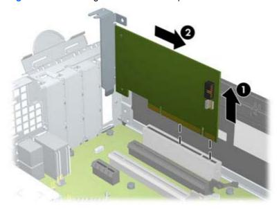
If you are removing a PCI Express x16 card, pull the retention arm on the back of the expansion socket away from the card and carefully rock the card back and forth until the connectors pull free from the socket. Pull the expansion card straight up from the socket then away from the inside of the chassis to release it from the chassis frame. Be sure not to scrape the card against the other components.
