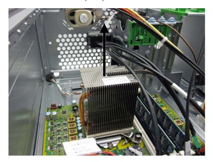
When reinstalling the heat sink, make sure that its bottom has been cleaned with an alcohol wipe and fresh thermal grease has been applied to the top of the processor.
