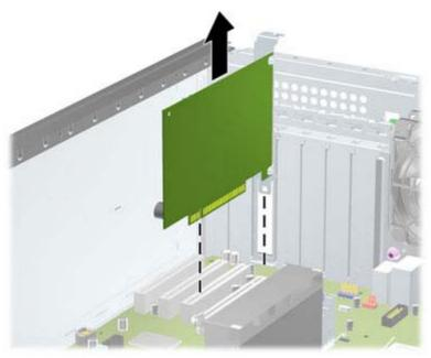
If you are removing a PCI Express x16 card, pull the retention arm on the back of the expansion socket away from the card and carefully rock the card back and forth until the connectors pull free from the socket. Lift the card straight up to remove it. Be sure not to scrape the card against other components.
