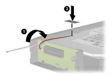
Slide the cover on the carrier (1) and replace the screw on the rear of the carrier to secure the cover in place (2).
