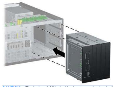
A CAUTION: The bottom 5.25-inch drive bay has a shorter depth than the upper two bays. The bottom bay supports a half-height drive or other device that is no more than 14.5 cm (5.7 inches) in depth. Do not try to force a larger drive, such as an optical drive, into the bottom bay. This could cause damage to the drive and the system board. The use of unnecessary force when installing any drive into the drive bay may result in damage to the drive.
