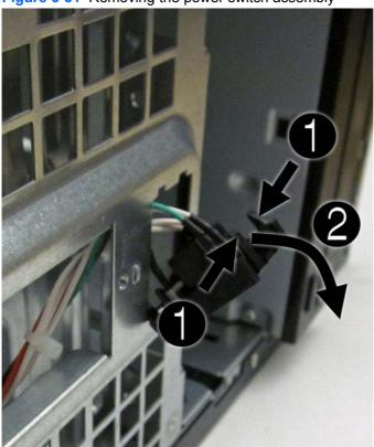
Figure 6-31 Removing the power switch assembly
