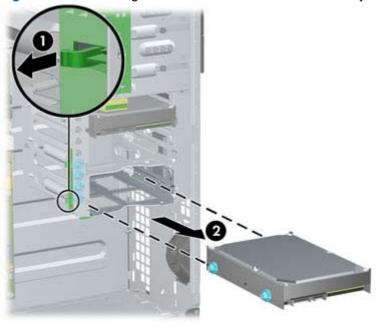
• To remove a hard drive from the upper internal hard drive bay, remove the screw on the side of the bay that secures the drive in place (1), then slide the drive out of the bay (2).
