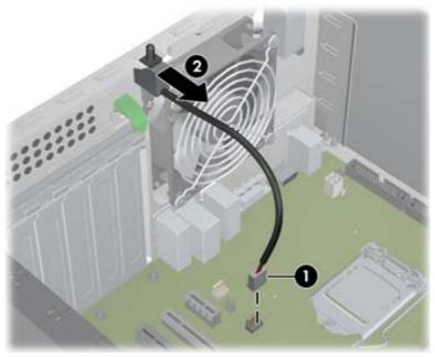
To reinstall the hood sensor, reverse the removal procedure.
