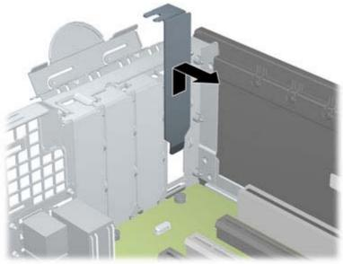
If you are removing a standard PCI card or PCI Express x1 card, hold the card at each end, and carefully rock it back and forth until the connectors pull free from the socket. Pull the expansion card straight up from the socket (1) then away from the inside of the chassis to release it from the chassis frame (2). Be sure not to scrape the card against the other components.
