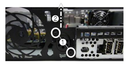
To install the speaker, reverse the removal procedure.
