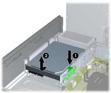
To install a hard drive, you must transfer the silver and blue isolation mounting guide screws from the old hard drive to the new hard drive.
