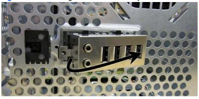
Pull the assembly away from the computer while threading the wires through the hole in the front of the chassis.
