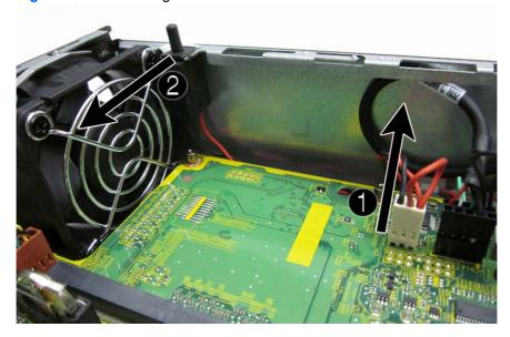
To install the hood sensor, reverse the removal procedures.
