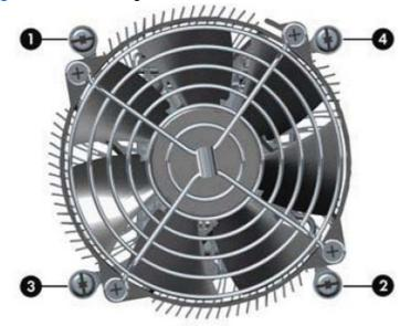
Disconnect the fan cable from the white system board connector labeled CPUFAN (1).
