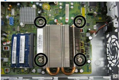
Lift the heat sink from the system board.
