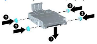
10. To place the hard drive carrier back in the chassis, align the guide screws with the slots on the drive bay, drop the carrier straight down into the drive bay (1), and press the handle on the carrier all the way down (2) so that the drive is properly seated and locked in place.
