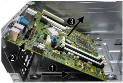
When reinstalling the system board, first insert the I/O panel back into the slots in the rear of the chassis, and then align the board with the chassis screw holes.
