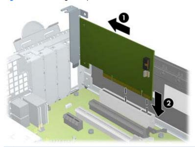
When installing an expansion card, press firmly on the card so that the whole connector seats properly in the expansion card slot.
