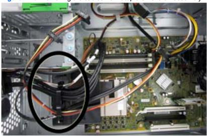
Unplug the fan cable from the system board connector labeled CHFAN.
