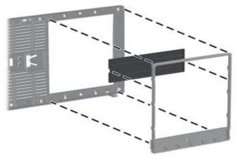
NOTE: When replacing the subpanel, ensure that the aligning pins and any remaining bezel blanks are in their proper orientation. The logo on the subpanel should be located at the bottom of the subpanel when properly oriented.
