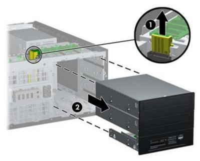
9. Gently slide the drive into the uppermost available bay until it snaps into place. When the drive is properly inserted, the drivelock will secure it. Repeat this step for each drive.
