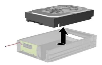
Place the new hard drive in the carrier then slide the hard drive back so that it seats in the SATA connector on the carrier's circuit board. Be sure the connector on the hard drive is pressed all the way into the connector on the carrier's circuit board.
