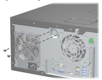
Figure C-2 Removing the Smart Cover Lock Screws from the Microtower
