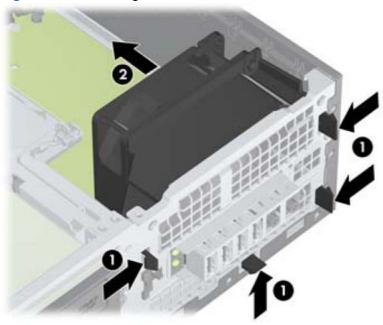
To install the front fan, reverse the removal procedure. Be sure to orient the air flow into the unit.
