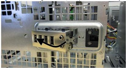
Pull the assembly toward the right and away from the chassis while threading the wires through the slot between the drive cage and chassis front and the hole in the front of the chassis.
