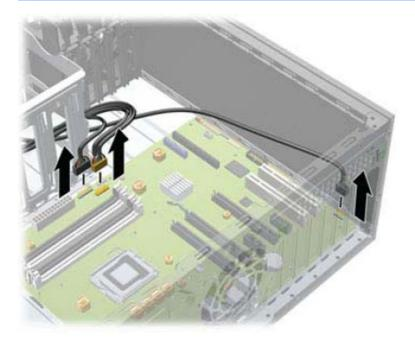
Remove the Torx T15 screw that secures the assembly to the front of the chassis.
