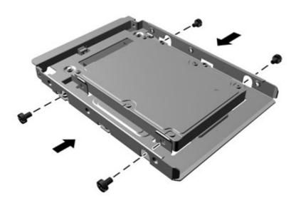
• Install four 6-32 silver and blue isolation mounting guide screws in the adapter bracket (two on each side of the bracket).
