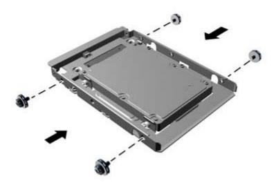
• If you are installing the drive in the upper bay (bay 4), install three standard 6-32 silver guide screws (two on the right side and one on the left side in the screw hole closest to the power and data connectors).
