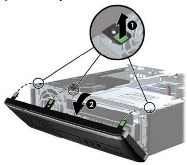
To install the front bezel, reverse the removal procedure.
