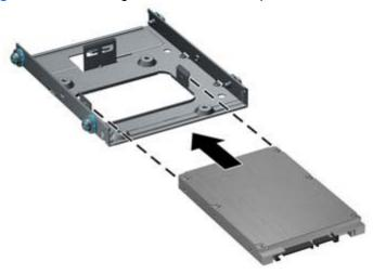
Hold the drive and bracket firmly together and turn the assembly over. Install four M3 screws to secure the drive to the bracket.
