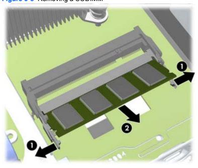
5. Slide the new SODIMM into the socket at approximately a 30° angle (1) then press the SODIMM down (2) so that the latches lock it in place.
