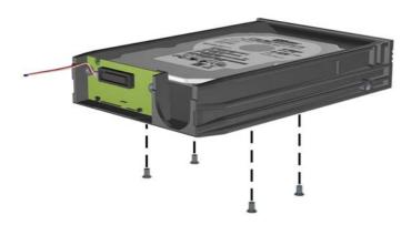
Slide the hard drive back to disconnect it from the carrier then lift it up and out of the carrier.
