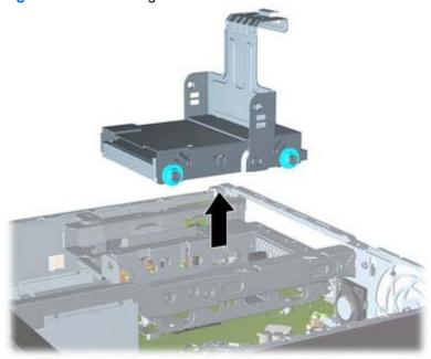
Remove the four guide screws from the sides of the hard drive carrier.
