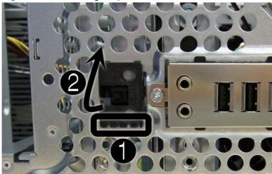
Pull the assembly away from the chassis while threading the cable through the hole in front of the chassis.
