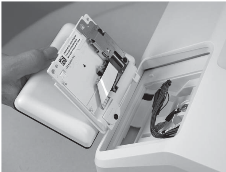
Figure 1-367 Remove the control panel
