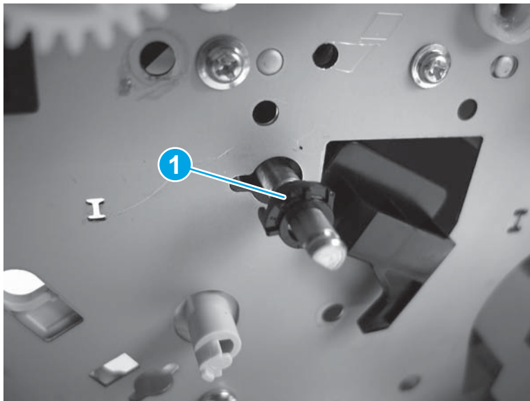
Figure 1-1665 Install one bushing
