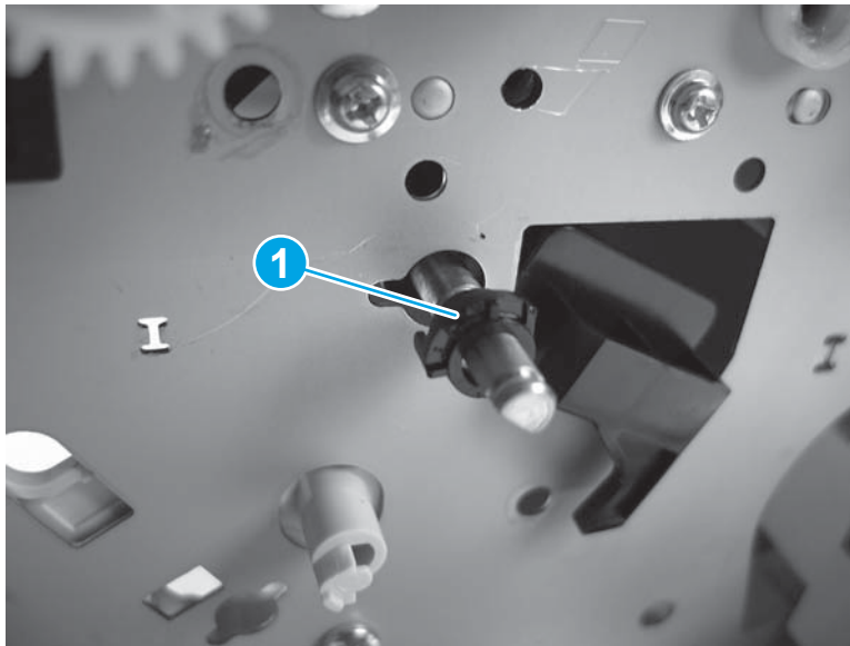
Figure 1-1652 Remove one bushing
