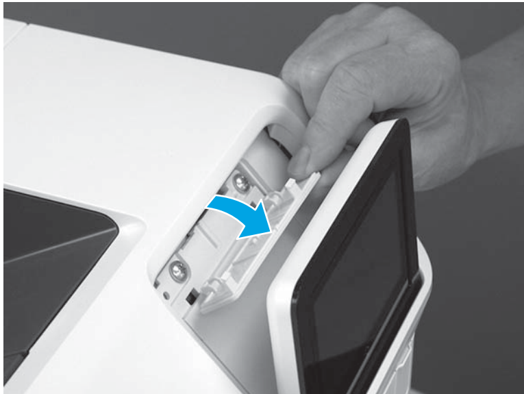
Figure 1-363 Rotate cover away
