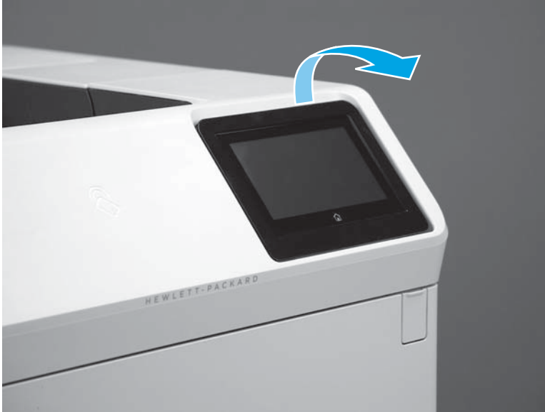
Figure 1-123 Tilt the control panel up
